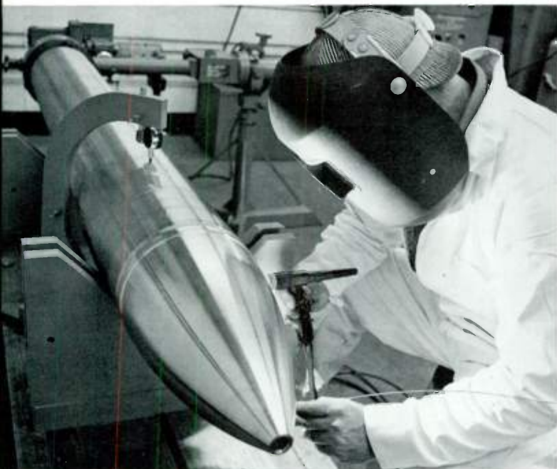
ONE OF THE END PIECES of the new Westinghouse Time Capsule is welded to the center section. The capsule will be filled with the documentary evidence of man's progress in the past 25 years, and then the other end piece will be welded on. The stainless-steel capsule will be buried at the New York World's Fair to supplement the record left there, for people 5000 years from now, at the close of the 1939-40 Fair.
