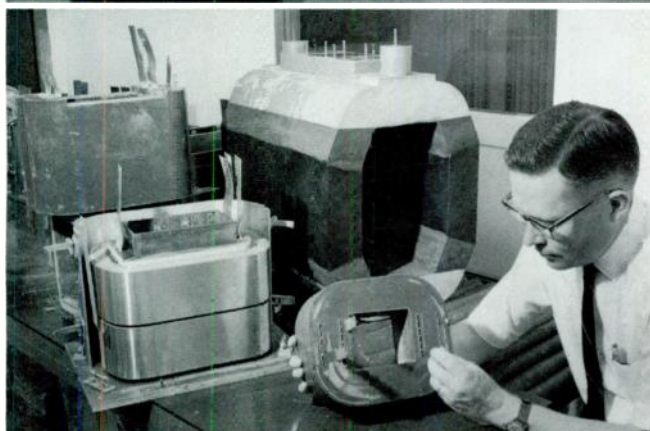
A COMPLETED 25-KVA, 7200-VOLT UNIT (top photo) is placed in its tank. In the bottom photo, the author is holding a 10-kva solid insulation unit. Limited quantities of 10, 15, 25, 50, 100, and 167 kva units are now being produced.
