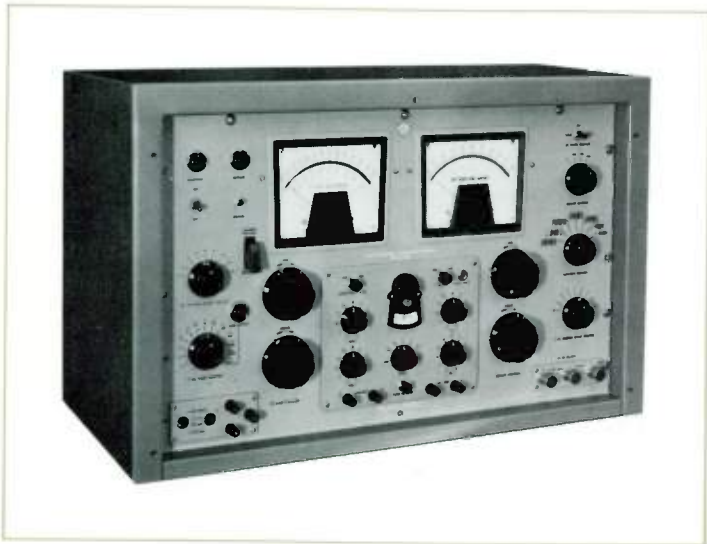
TBS ac and dc ammeters and voltmeters are used as comparison standards in a \pm 0.25 percent accuracy, direct-reading Instrument Calibration Standard for voltages from 0.25 millivolt to 2000 volts, and currents from 2 microamperes to 20 amperes.
