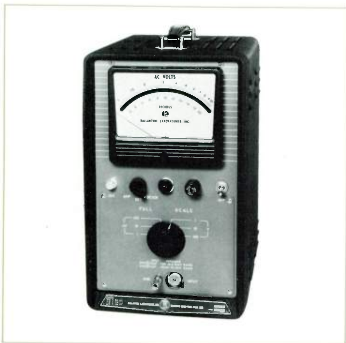
Sensitive video electronic voltmeter with logarithmic scale having ranges from 100 microvolts to 100 volts over a frequency span from 2 cps to 6 mc. All scale divisions of the taut-band suspension instrument are individually calibrated and marked making possible unusually high accuracy and repeatability.
