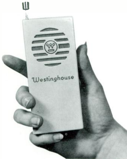
1) Single-side-band command receiver miniaturized with monolithic integrated circuitry.
