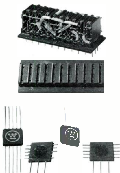
11) Stacked-array submodule holds flat-packs and other components in a specially designed plastic frame structure.
