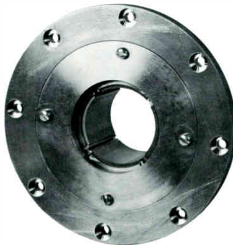
4—Rotor bearings are of pivoted-pad type designed for use with liquid potassium as the lubricant. Pads can be adjusted individually to control clearances and concentricity.
