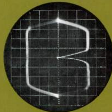
Vertical Current Limit, Full IR Droop
