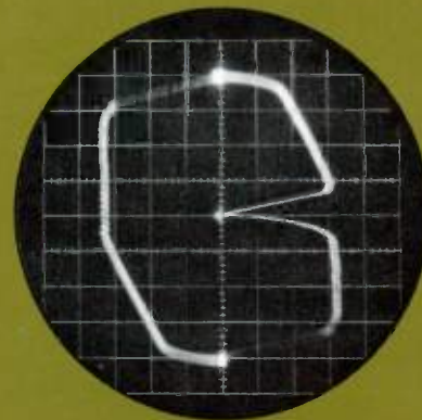
Full Current Limit Slope, One-Half IR Droop
