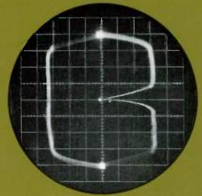
Vertical Current Limit, One-Half IR Droop
