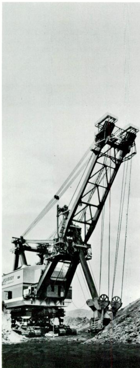
Shovel of 150 cubic-yard capacity is used for stripping overburden from coal deposits. It, like other large excavators, is powered by a number of dc motors energized by m-g sets. Motor speed and torque control must be precise and fast acting for maximum productivity and safe operation of the massive machinery. This control, effected by regulating the generator fields, has been greatly improved by application of the parallel control technique. (The shovel illustrated was built by Bucyrus-Erie Company for Peabody Coal Company.)
