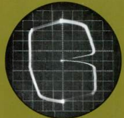
One-Half Current Limit Slope, One-Half IR Droop
