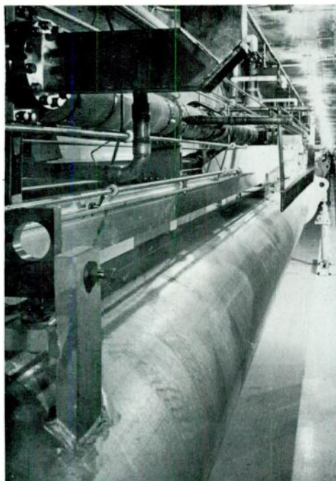
Accelerator tube stretches two miles down a tunnel. Waveguides, one of which is seen at upper left, bring microwave energy from 240 klystrons to accelerate electrons through the tube for high-energy physics research.
