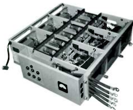
3—Thyristors and fuses are located in a vertical central duct in the power case for forced-air cooling. Continuous rating of the case is 460 amperes.
