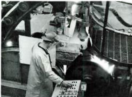
Continuous casting produces copper bar of virtually unlimited length. The molten metal pours into a cavity formed by a steel belt and a groove in the rotating casting wheel seen behind the operator.
