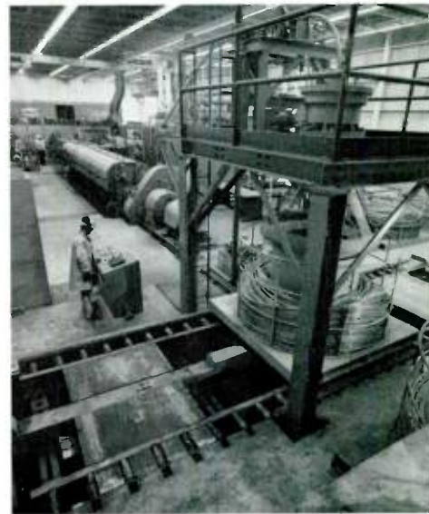
After rolling, rod is cooled in its passage through a tube that elevates it to a coiling device, which lays it evenly in large baskets. When one is filled, it is removed and another put into its place without stopping the process. The rolling train is seen in the background and, behind that, the casting facilities and a railroad car in which copper plates are brought in for melting.
