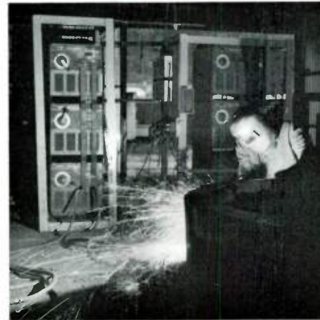
Solid-state welders are connected in threes to form power supplies for arc-air gouging.
