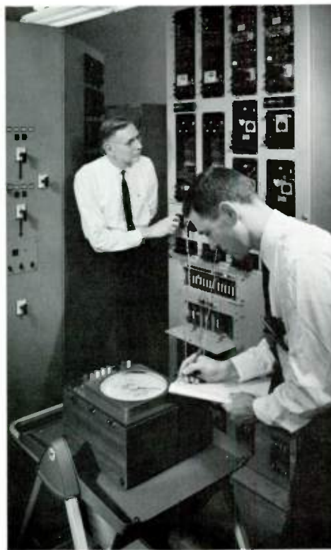
Photo—Portable phase-angle meter is designed for use as a field instrument for checking relay connections and other applications where the relationship between current and voltage must be known.
