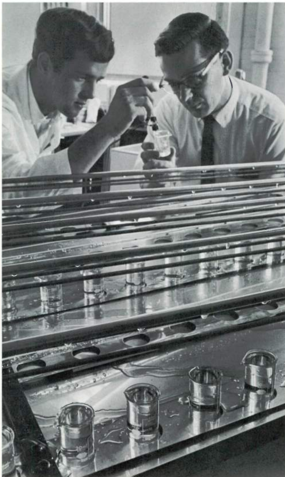
Pure water from brine is the product of experiments with reverse osmosis being conducted at the Westinghouse Research Laboratories. Water molecules pass through a semipermeable membrane in this process, but the salt is left behind. The development work is aimed primarily at purification of water of relatively low salt content—"brackish" water.
