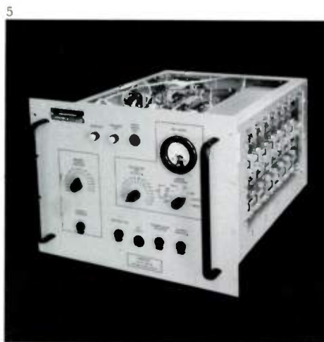
4—The modular concept is illustrated by this solid-state power amplifier. Each 5-kw module is automatically disconnected from the input
