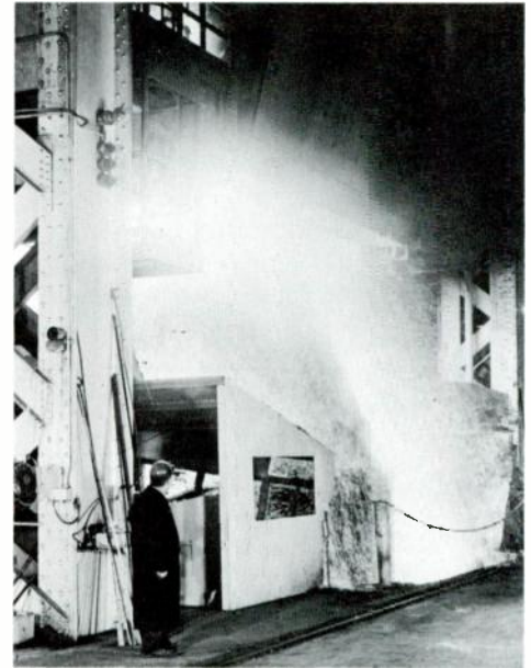
More pyrotechnics result when oxygen is blown through a water-cooled lance lowered into the open top of the BOF vessel. By burning carbon and impurities out of the molten metal, the oxygen converts the bath to steel. Blowing time is critical because too little or too much necessitates adjustments that reduce plant productivity.
