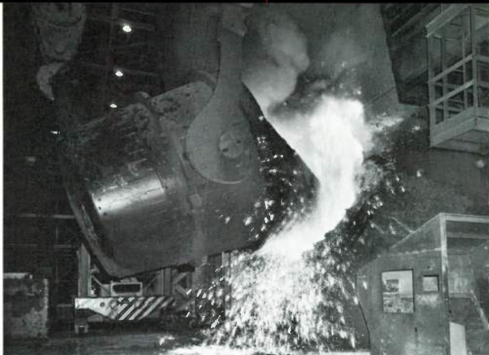
Molten iron is charged into a BOF steelmaking vessel, one of two 230-ton furnaces at Jones & Laughlin Steel Corporation's Cleveland Works. Scrap metal is the other main component of the vessel's charge. Scrap and hot-
