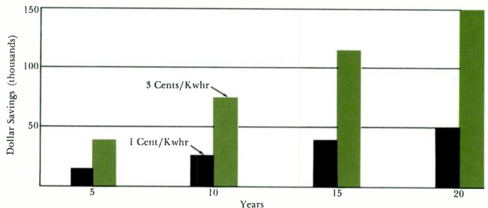
5 —Typical savings in operating costs for a solid-state transmitter compared to a vacuum tube transmitter.
