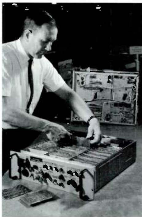
3—This demodulator chassis for an ultrareliable low-frequency receiver contains 439 integrated molecular units, the equivalent of more than 11,000 discrete components.
