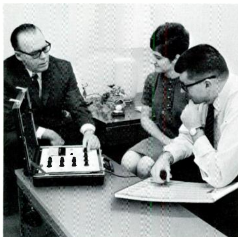
A compact analog computer provides fast and realistic estimates of heat loss from a house, the contributions of various parts of the structure to heat loss, and the cost of electric heating for that house. The computer can also indicate the effects of changes in insulation on heat loss and heating cost.
