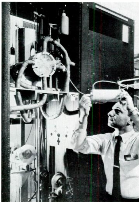
Pulmonary simulator takes the place of one or more human subjects for such purposes as testing and calibrating medical devices and life-support systems. An oxygen gauge is being connected here.
