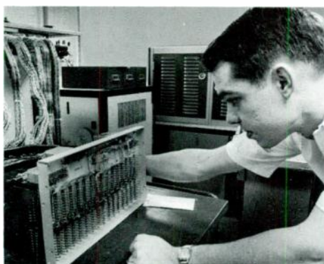
2—Testing is automated in the Hagan/Computer Systems Division manufacturing shop by using a small digital computer (seen in the background) to check various assemblies that will go into other computers. Here a wired panel into which electronic circuit cards will later be plugged is checked for short circuits, open circuits, bad connections, and wiring errors. The computer prints out its test findings to guide any corrections required.
