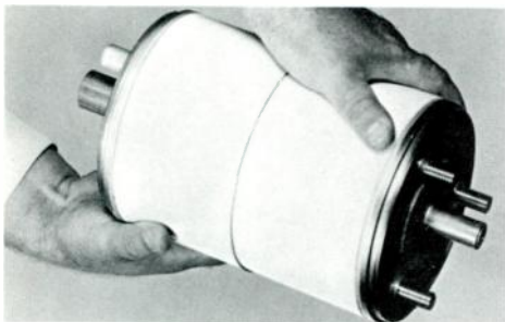
1—The vacuum interrupter (WL-23223) is designed for 15.5-kV circuit breaker service. The interrupter is rated at 600 amperes rms continuous current and is capable of interrupting up to 12,000 amperes rms.
