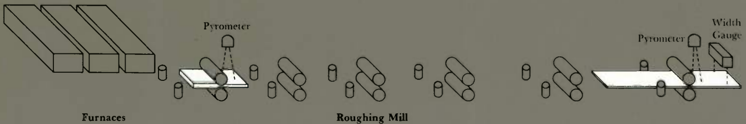
2—The Armco hot strip mill is represented here in greatly simplified form. It was started up one area at a time, beginning with the roughing mill, after the subsystems had been verified.
