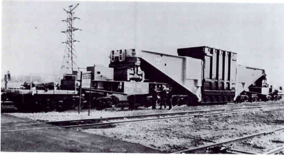
The latest Schnabel car for transporting power transformers handles the really big fellows. Its capacity is a million pounds.
