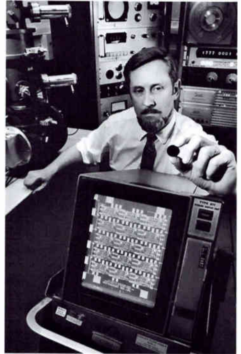
The design displayed on the monitor is a detail from one of the electron-emitting masks used to form an interconnected array of ultra-small integrated circuits on a silicon wafer such as the one in the man's hand. The highly detailed masks are "written" by the scanning electron microscope at left, with the electron beam controlled by magnetic tapes prepared from drawings.
