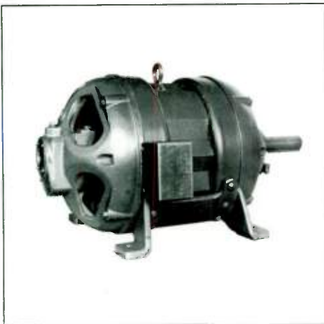
3—Early version of Type CS 1920 motor had a frame consisting of two rings joined by heavy cast feet riveted to them. Cooling air was drawn in through large openings in each end bracket and discharged through clearances between each end ring and the stator core.
