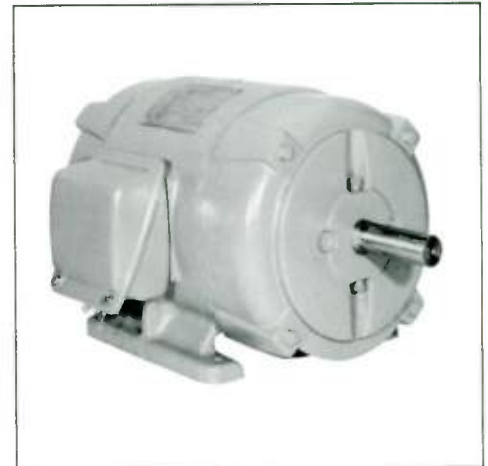
5—U-frame motors came out in mid-1950's. This Life-Line A machine was single end ventilated in the smaller sizes; the ventilation opening in each end bracket is virtually invisible, being confined to the lower quadrant. Larger sizes were double end ventilated.
