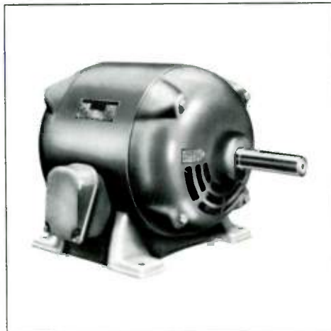
4—Type CSP motor of 1940 vintage had a dripproof housing for greatly improved protection of windings. It was single end ventilated and had sealed prelubricated ball bearings instead of the sleeve bearings that had been standard in the earlier motors.
