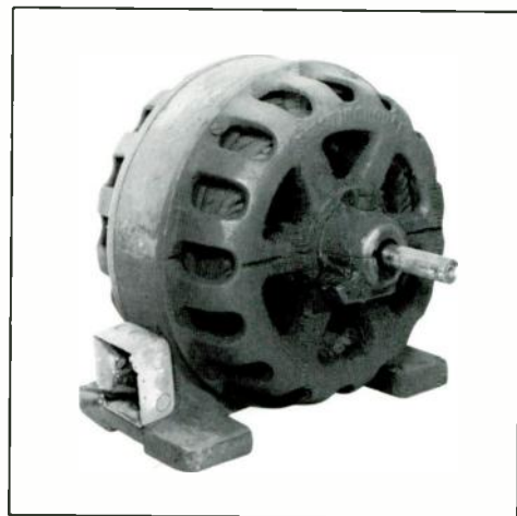
2—Type CCL 1910 motor was photographed as it was retired early this year. It had been used in a machine shop from about 1913 to 1960 to drive several machines via an overhead lineshaft; then, to soften the transition to retirement, it was assigned to blower-drive duty.
