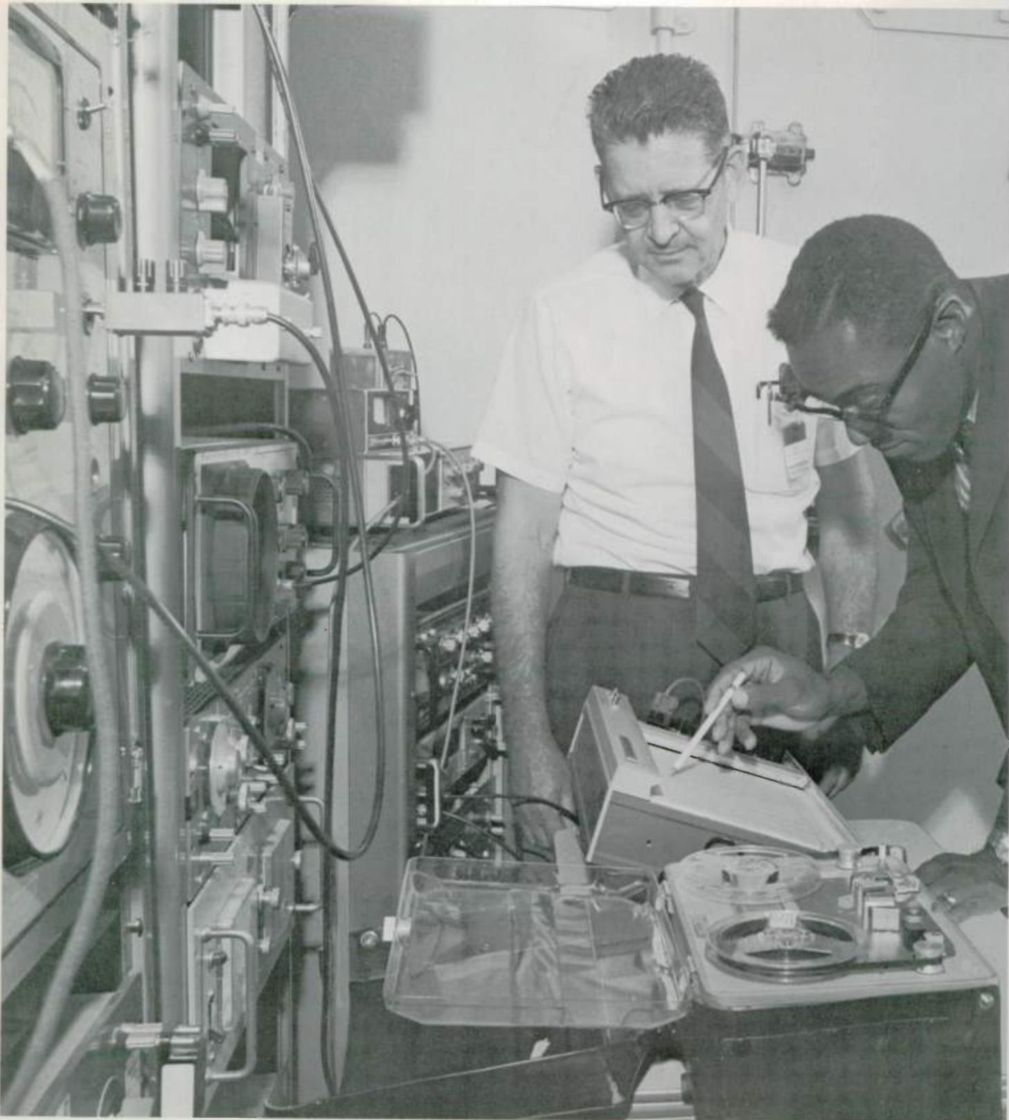
Noise measured in an industrial plant is analyzed as part of a service that helps industries comply with government regulations. (See page 188.)
