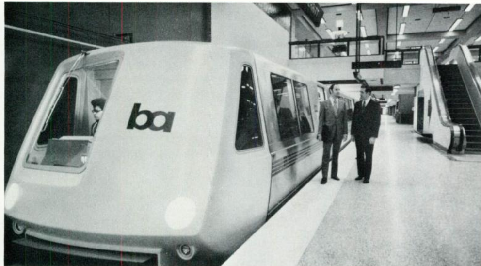
BART trains are designed for high speed and high passenger volume. Although an operator is present in the head car, operation normally is completely automatic.
