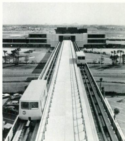
Tampa International Airport Passenger Transport System connects a central terminal building with satellite buildings. Similar vehicles and technology are used in the Transit Expressway system designed for public transportation in smaller cities and for feeder service in large cities.
