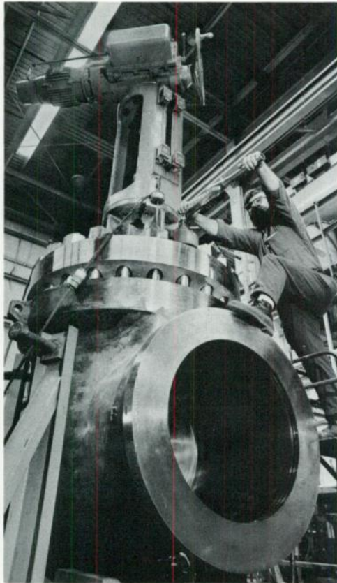
Large stop valves for PWR power plants isolate loops from the reactor when service is required on the loops. They are designed for reliable operation and sealing. The valve in the photograph is of 27½-inch port diameter. Shown being prepared for testing, it has since been installed in Commonwealth Edison's second plant at the Zion, Illinois, site. The two plants there each have eight of the valves.
