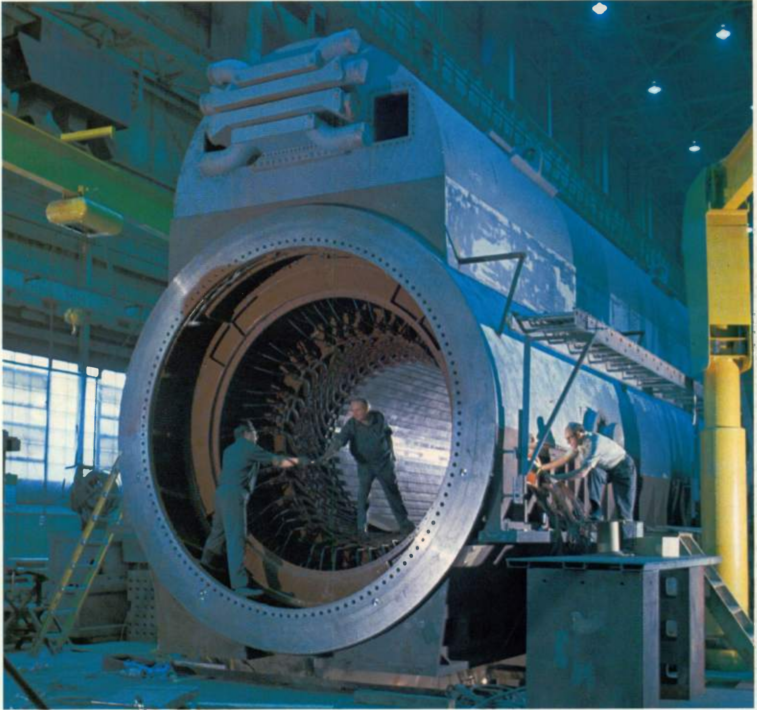
This large stator is a part of one of two 1200-MW generators built for Tennessee Valley Authority. The completed machines are each 40 feet long, and each can supply the electrical requirements of a city the size of Nashville, Tennessee.
