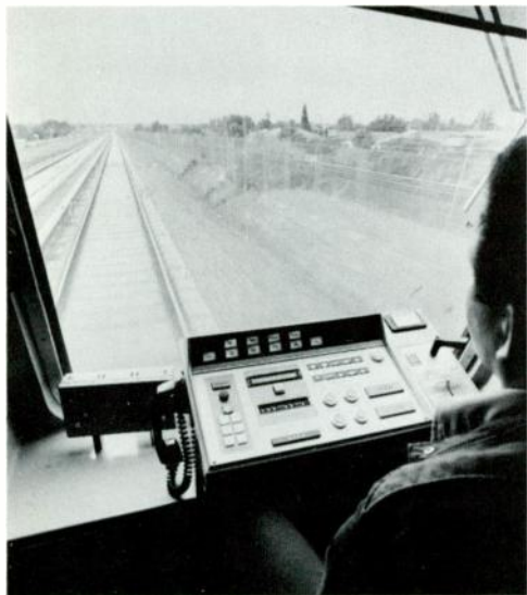
A BART train races down the track at 80 miles per hour under automatic control, which is the normal mode of operation. The control panel enables an attendant to operate the train manually, if necessary, at low speed.
