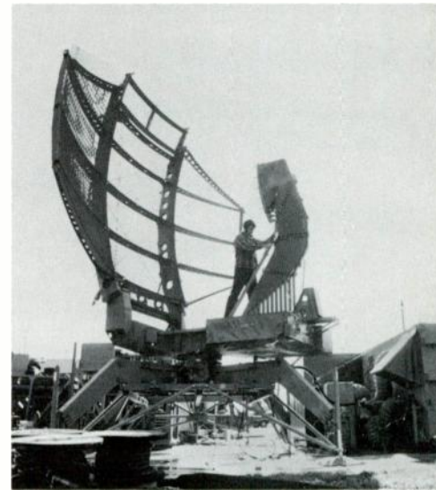
This radar is part of a tactical air defense system, shown undergoing field tests. The AN/TPS-43 three-dimensional radar provides the necessary information for both aircraft warning and control capability.
