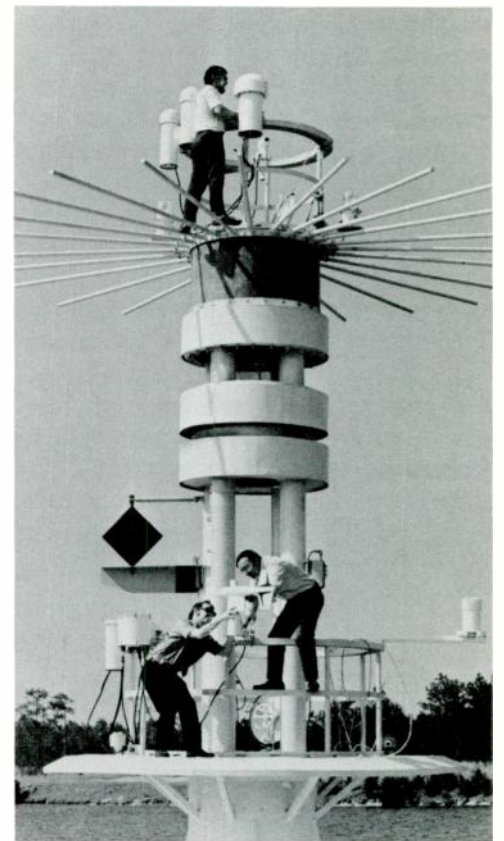
2—Meteorological sensors are mounted at two levels, 5 and 10 meters above sea level. The sensors for the six meteorological parameters are identified by the drawing (the atmospheric pressure and electronics package at the 10-meter level was not installed when the photograph was taken).
