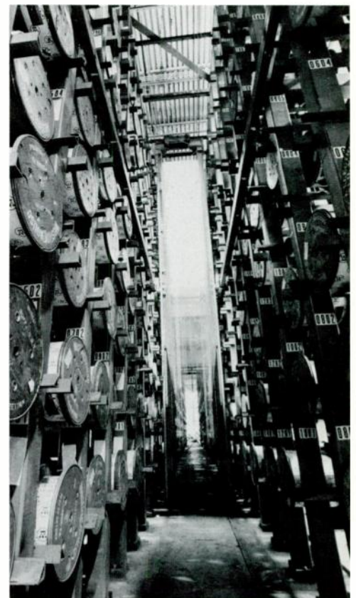
9—Stacker cranes store and retrieve finished reels of wire. The blur in the center here is the crane cab moving quickly upward to retrieve a reel for shipment.
