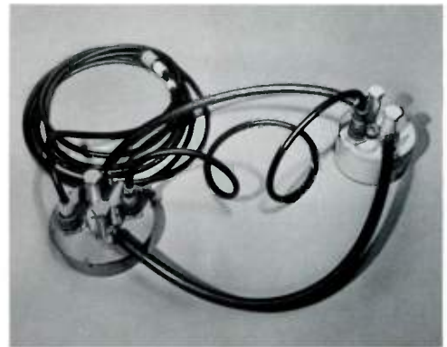
3—(Above) The Westinghouse Periguard system consists of a pair of fluid-filled hoses buried along parallel paths several feet apart. As an intruder approaches, a larger pressure change is generated in the hose nearer the intruder. Piezoelectric crystals in the buried detector sense the pressure differential between hoses and trigger an alarm.
