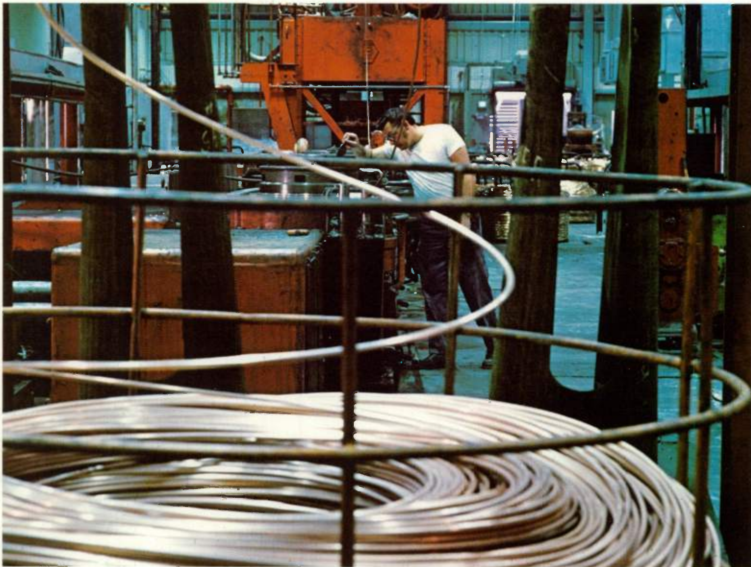
Copper rod is shaved before being drawn or rolled into magnet wire. (See page 58.) Shaving removes oxides and surface imperfections that could degrade the quality of the finished wire.
