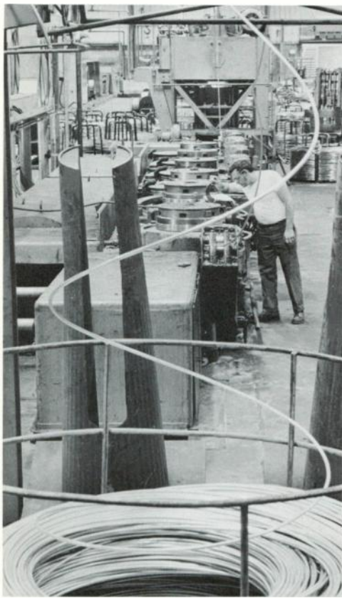
5—Shavers such as this one cut the skin off CMCB rod and perform a preliminary draw to prepare it for final wire drawing or rolling. Aluminum rod is also shaved and drawn.
