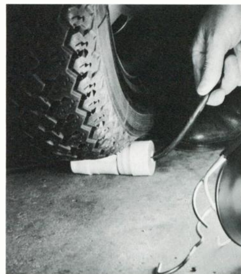
9—Plugs and connectors with nylon bodies are so strong that they can withstand such abuse as being run over by vehicles.
