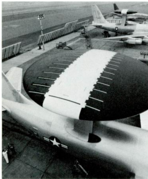
AWACS radar subsystem includes the antenna mounted in the structure on these test aircraft that were used to prove the engineering model.
