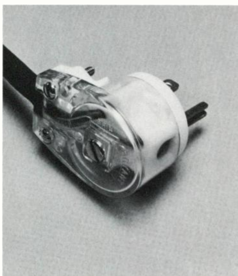
2—Proper attachment of the grounding conductor in this three-wire plug can be verified visually because the back is transparent. Also, the right-angle cord attachment permits equipment to be placed against the plug without having to bend the cord sharply.
