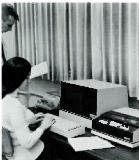
Warehouse operations system employs a keyboard, display monitor, and teleprinter to enable an operator to communicate with a remote computer. The new system produces shipping tickets and purchase orders, keeps track of inventory, produces accounting reports and statements, gives management operating reports, and provides a host of other information at selected intervals.
