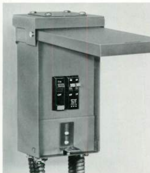
3—The GFCB breaker is applied in place of a standard 1-inch-wide breaker in a load center, and it then provides ground fault protection for all the outlets on that circuit. It is the device on the left in this typical load center; the one on the right is an ordinary duplex breaker that protects two circuits against overload and short-circuit currents.
