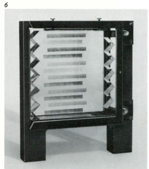
4—Two views of a rectangular delay line illustrate how internal reflection of acoustic signals increases the effective length of the acoustic path and thus increases the storage capacity of the delay line. Incident processing light illuminates the acoustic paths of a radar return signal and its reference.
