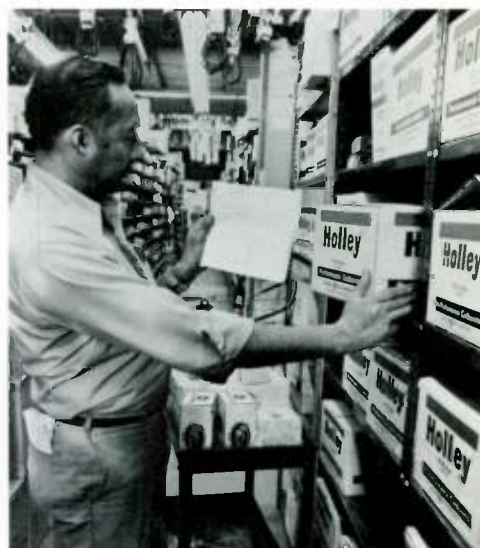
An order picker uses one of the shipping tickets produced by the system to assemble an order. The ticket tells in which zones and bins the parts will be found, and it lists them in the sequence that requires the least walking. Both photos show operations at Cleveland Ignition Company, Cleveland, Ohio.
