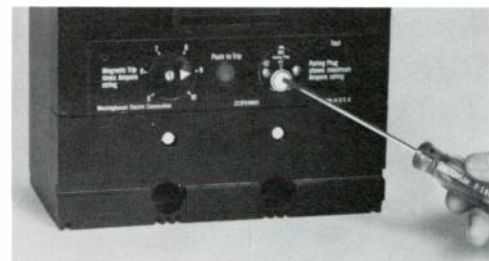
2—(Top) Easily changed plugs determine the continuous current rating of each breaker. A fixed rating plug is being installed here.
