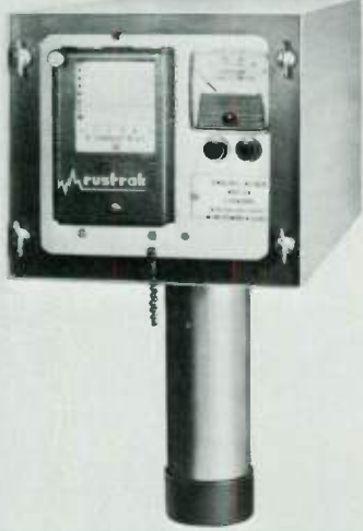
This combustible limit relay monitors the percent of combustible gases in the gas space of a transformer.
