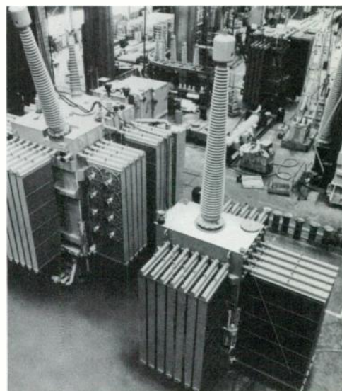
This 500-kV single-phase autotransformer (left) and shunt reactor (right) were tested together before being shipped to Arizona Public Service Company for the Navajo Project. The autotransformer is rated 200/266/333/444 MVA, 525/230 kV, 1425/825 kV BIL, and it has a load tap changer to regulate voltage. The shunt reactor is rated 70 MVAR, 525 kV, 1550 kV BIL.
