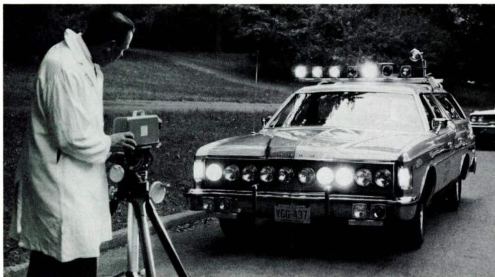
Shown lighted on the test car are the three lamps that provide the mid beam for a proposed new three-beam headlight system.
