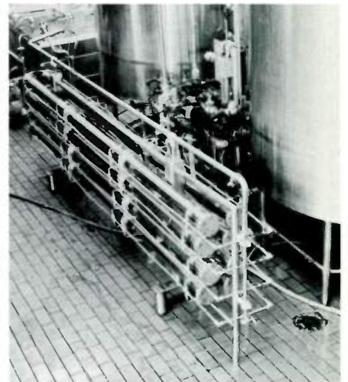
A typical configuration for a cheese whey fractionator/concentrator system is illustrated by the simplified diagram. The system has been used on a pilot-plant basis, as shown in the photograph, at a number of dairies to provide operating data and to assure conformance with dairy industry regulations. It economically reclaims valuable products while cleaning up dairy plant wastes.
