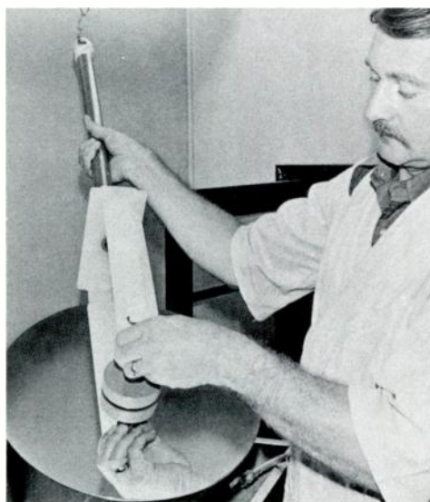
(Top)—Wafers for disc memories are cleaned, before plating, in an alkaline bath in this two-station six-kW ultrasonic unit at Sperry Univac's Bristol, Tennessee, plant.
