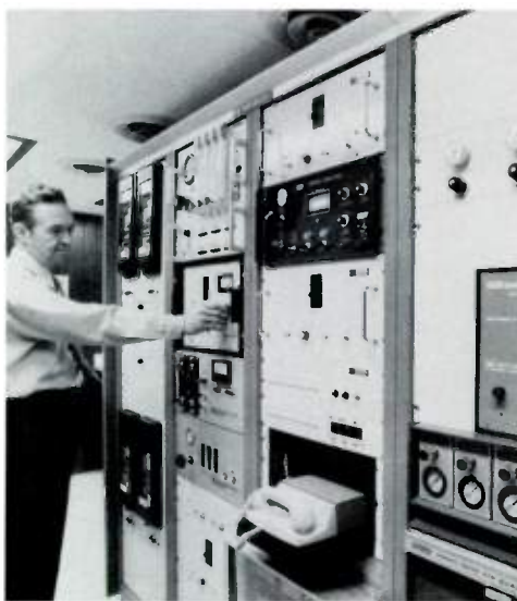
Environmental monitoring system includes one or more mobile monitoring stations. The tower, which carries meteorological sensors, is lowered when the station is to be moved. Sensors and analyzers inside the station continuously monitor air pollutants and meteorological conditions. All instrumentation is located in a central island to provide accessibility to the front and back of each rack.
