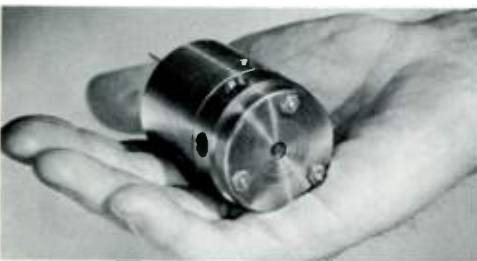
3—The cathode is a tungsten rod contained in a plug-in assembly that is readily replaceable (above). The assembly also contains the auxiliary filaments that heat the cathode by electron bombardment (right). The cathode's operating characteristics are much more constant than those of resistively heated types, and it has much longer life.
