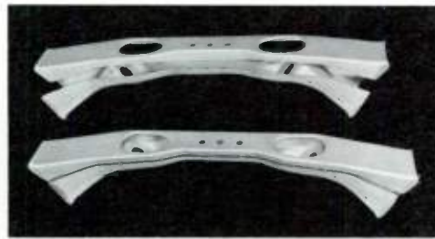
8—This component of an automotive frame was welded in a prototype EB welding system that can make the butt welds at 280 inches per minute. The component is 36 inches long. It is held stationary while two welding heads, one on each side, follow the seams and make the welds.
