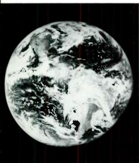
Views of the western hemisphere with its weather patterns are transmitted from the SMS-1 satellite and recorded at ground stations by laser-beam recorders. A picture can be made every half hour for close monitoring of weather movements.
