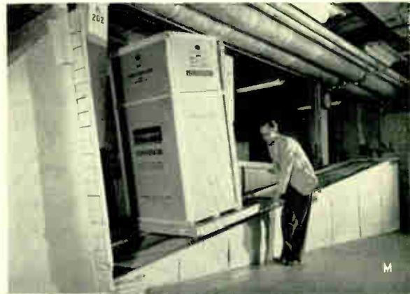
K—Some products, like electronic control, can be developed as readily on the breadboard as on the drafting board. L—Manufacturing engineers also have laboratories for creating better ways of making things—such as better cutting methods. M—In the appliance shipability laboratory the product and its container as a unit are given preshipment trials.
