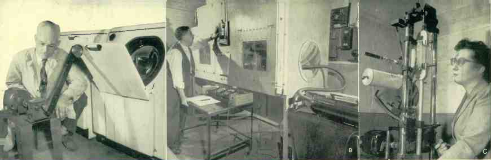
A —Engineers learn how many “bangings” a Laundromat door will take. B —The “drawing power” of a tank-type cleaner is tested. C —Strength of washed fabric is measured.
