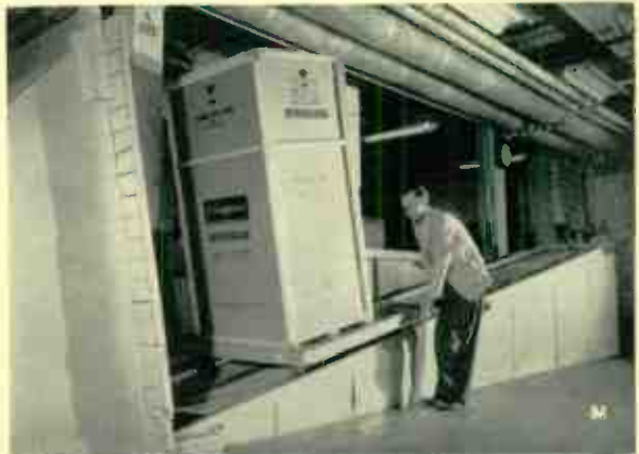
K—Some products, like electronic control, can be developed as readily on the breadboard as on the drafting board. L—Manufacturing engineers also have laboratories for creating better ways of making things—such as better cutting methods. M—In the appliance shipability laboratory the product and its container as a unit are given preshipment trials.
