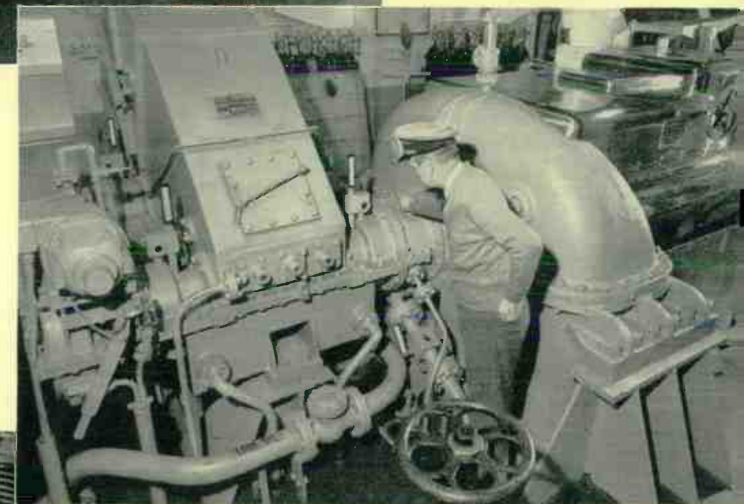
Two of these 3800-kw turbines furnish all propulsion, pumping, and auxiliary power for this seagoing dredge.
