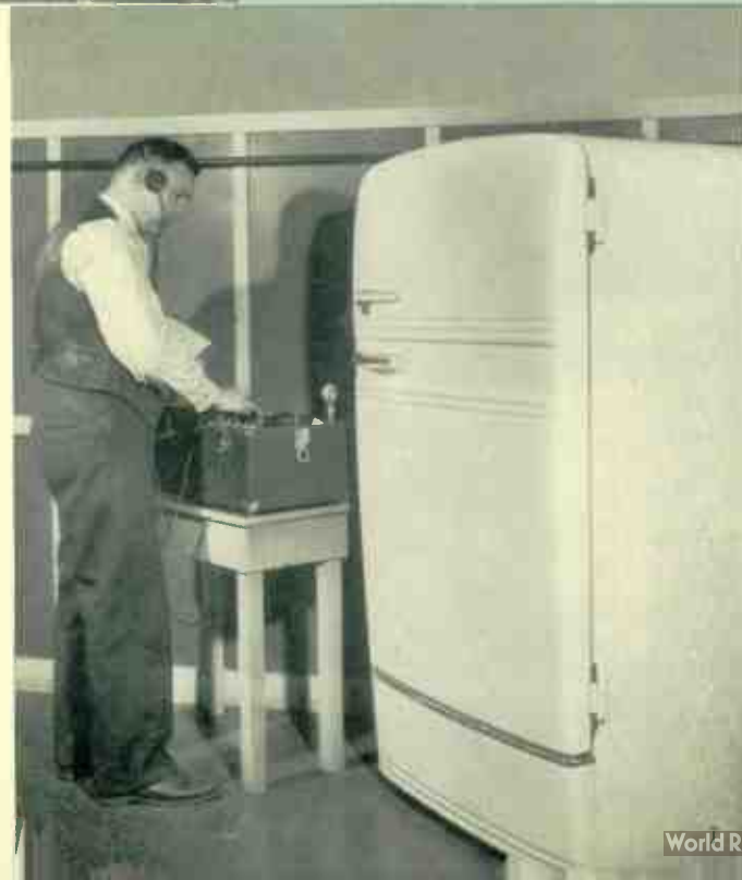
H —Electric-range elements must be able to take the ordeal of cold, corrosive liquids. Here, measured quantities of cold salt water are poured on hot cooking elements. I —In the quiet room, a refrigerator proves that it will not create noise.
