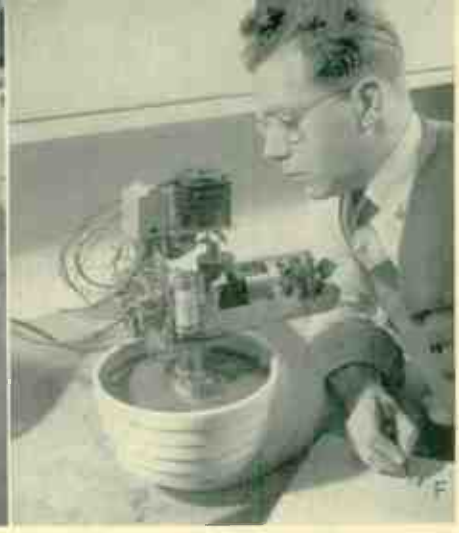
E —To test washing techniques, fabric must be made dirty. Here is the machine that soils cloth. F —Asbestos shavings and heavy oil simulate stiff cake batter.
