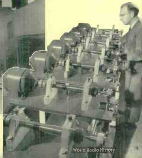
N —Fatigue machines provide essential data for turbine designers. O —Giant arcs provide the best laboratory shows.
