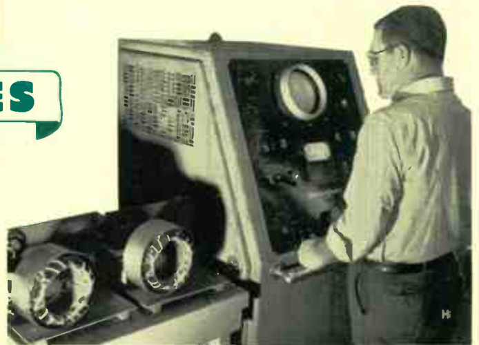
E —Beside the engineer is a frequency standard accurate to 0.01 part per million. F —Many rooms isolate noise, high frequency, x-rays, or nuclear radiation. This is a radio-noise room.
