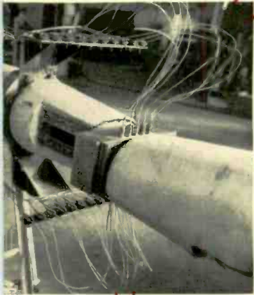
Combustion equipment will be used to measure the relative rate of corrosion of various turbine-blade metals. Hot exhaust gases from a residual oil combustor pass over test specimens at approximately the same velocity as gases entering turbine nozzles. Corrosion is measured by weight loss of the blade.
