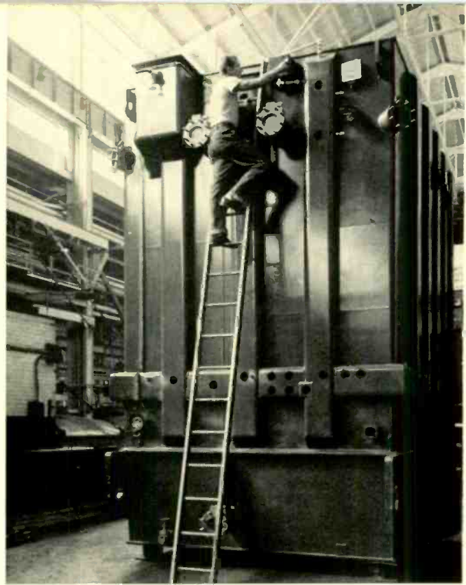
This is a 315-mva generating-station transformer under construction. Both this transformer and a larger 360-mva unit will be shipped upright in a single piece, minus coolers and bushings.
