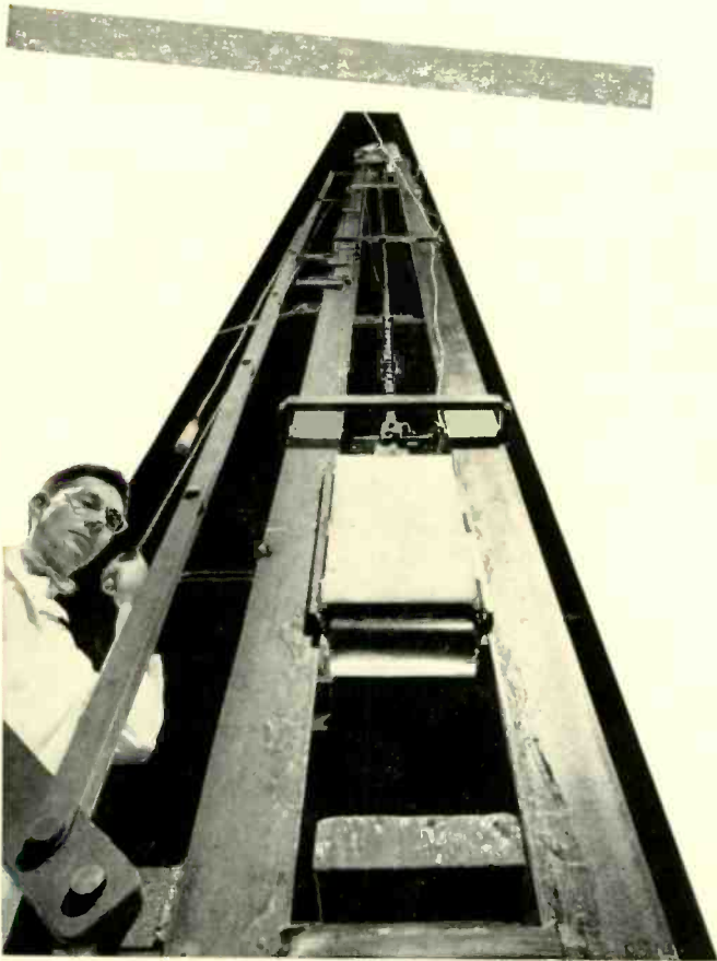
This guillotine tests shock resistance of metals.
