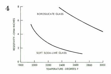
ELECTRICAL RESISTIVITY OF GLASS varies inversely with temperature, and it also depends on the chemical composition of the glass. This wide variation in resistivity encountered among various glasses and at various temperatures necessitates careful design of electric furnaces and their power supplies. The characteristics illustrated here are for a borosilicate glass (for ovenware) and a soda-lime glass (common container glass).
