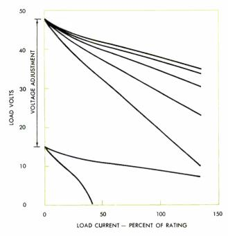
CONSTANT-VOLTAGE DC WELDERS have volt-ampere eurves that are nearly flat. In some, the slope of the curves can be adjusted as shown. Voltage also is adjustable over a wide range.
