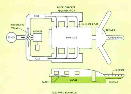
CONTINUOUS ELECTRIC GLASS FURNACE occupies much less space and is simpler than a fuel-fired furnace of the same capacity. The latter requires flues, regenerators to heat the combustion air, a stack, and a blower. In the electric furnace,
