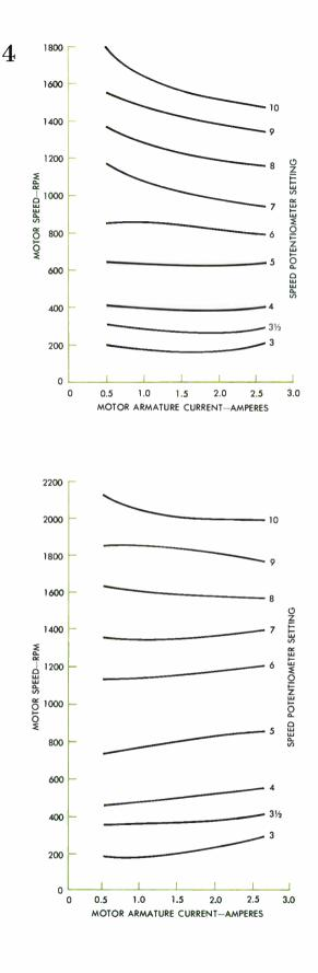
SPEED REGULATION with the type 902 thyristor drive in the *low* speed range (top) and the *high* range (bottom). Excellent control is provided over a range of seven to one or greater. The curves are based on the performance of a dc shunt-wound motor rated at 1/4 horsepower, 2.5 amperes, and 1725 rpm.
