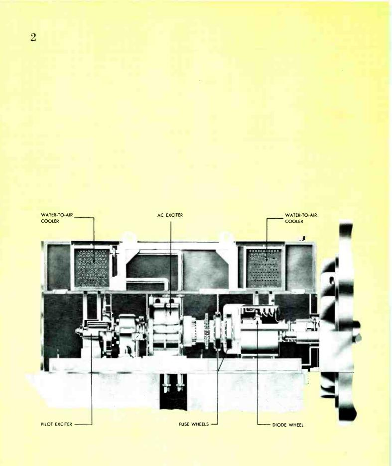
COMPONENT ARRANGEMENT of the brushless excitation system is shown in this artist's drawing of the 1350-kw unit.
