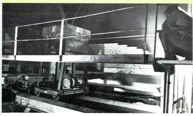
BATCH CHARGER for the continuous electric furnace at the Jeannette Glass Company travels along the side of the furnace.
