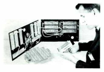
The system detects heat radiated from any target within its field of view and generates a coarse errortracking signal that can be used to center the system on the target. When the target is brought into the center of the field of view, the center four detectors in the mosaic generate a precise angle-tracking signal accurate to less than one milliradian.
