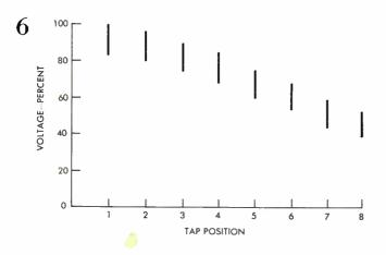
VOLTAGE CONTROL available at each transformer tap position by reactor adjustment overlaps that available at the adjacent positions. This reduces the amount of tap changing required.
