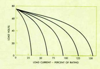
AC ARC WELDERS of the transformer type usually have capacitors for power-factor correction, giving electrical performance illustrated by these typical curves. Because the capacitors draw the same corrective kva under all load conditions, power factor increases with decreasing current output. Idling input is approximately 1.5 kva per 100 amperes of rating, and power factor is 100 percent leading.
