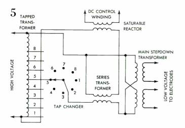
SERI-ACTROL FURNACE POWER SUPPLY includes a transformer tap changer for coarse power adjustments and saturable reactors for fine adjustments. For simplicity, a single-phase unit is illustrated rather than the two- or three-phase type actually used for continuous-furnace melting.
