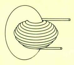
THE CHOKE configuration chosen for the illustrative problem is of the form of two interlocking doughnuts, the core comprising one doughnut, and a coil of N turns making up the other.
