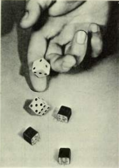
Fig. 11 Dice-cube-size miniature relays used in equipment where weight and space are at a premium. (Courtesy: Hi-G, Inc.)
