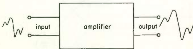
Fig. 14 An amplifier enlarges the input signal, but does not change its shape.
