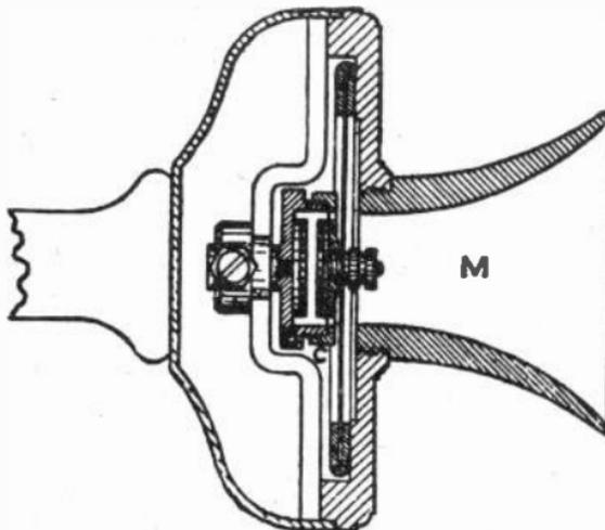
Fig. 9. Sectional view of a common type of telephone transmitter.
