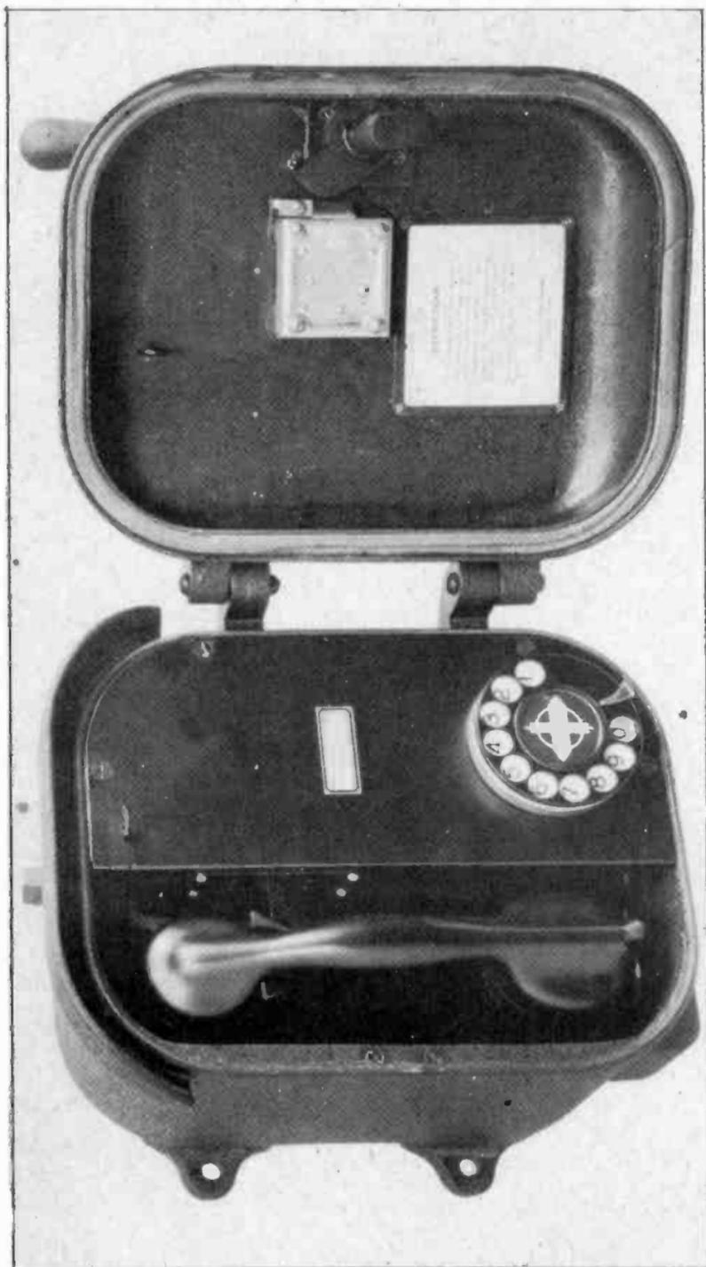
**This photo shows the latest type of outdoor MONOPHONE. Rugged equipment of this type is used in mines and other places where a communications system must be maintained both in and out of the buildings.**
