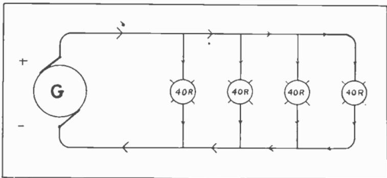
Fig. 39. Equal Resistances In Parallel.
