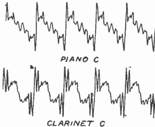
Fig. 2. These waves are typical of various musical notes, having the small variations in frequency and volume occurring at regular intervals, forming groups or large variations in the general note.
