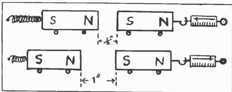
Fig. 82.-A. & B. Doubling the distance between two magnets, decreases their pull to  $\frac{1}{4}$  of what it was.
