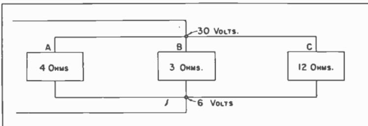
Fig. 37. Three Resistances Connected In Parallel.
