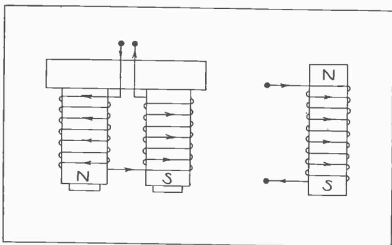
Fig. 104. Double and single electro-magnets.
