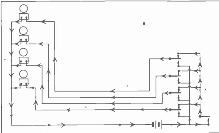
Fig. 21. Another type of selective call system with Master Control
