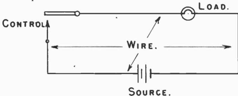
Current designated by this sign ( $I$ ) is needed to operate any piece of electrical equipment and the rate of flow of current in the circuit supplying such equipment will depend on the voltage ( $E$ ) applied to the circuit and the resistance ( $R$ ) of the circuit.
