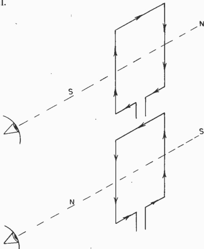
We already know that the flux around a wire will reverse if we reverse the current flow. This is equally true then of the flux around a coil or group of wires. So we can reverse the polarity of a solenoid or electro-magnet at will, merely by reversing the current supply wires to it.
