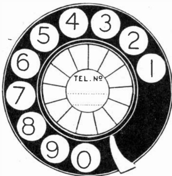
Fig. 5. Front view of dial, showing finger plate, holes, numbers and finger stop.
