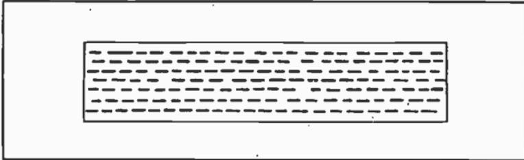
Fig. 77. Molecules lined up, in a fully magnetized bar.
