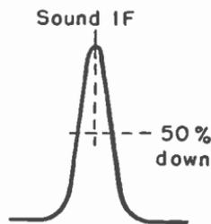
Fig. 4-6.—Response curve of a sound i-f amplifier.
