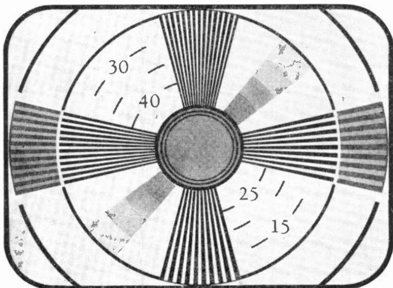
Fig. 1-1.—Test patterns are designed to help make service adjustments and locate troubles
