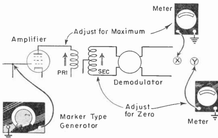
Fig. 7-6.—Connections for generator and output indicator for alignment of demodulator.
