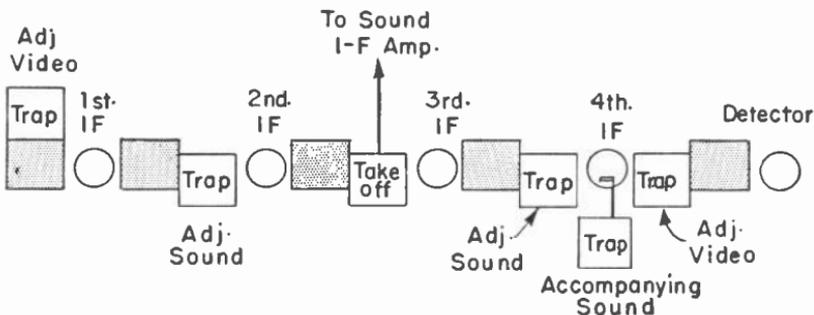
Fig. 6-6.—Locations of the six traps in the video-sound i-f amplifier.
