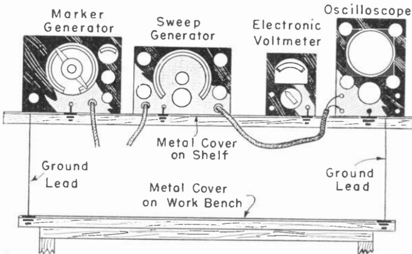
Fig. 2-19.—Service instruments on a shelf above the work bench.
