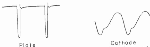
Fig. 14-20.—Oscilloscope traces taken from a diode damper tube.
