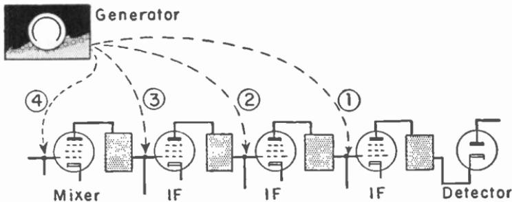
Fig. 6-3.—The generator coupling may be moved back toward the mixer, stage by stage, as alignment proceeds.
