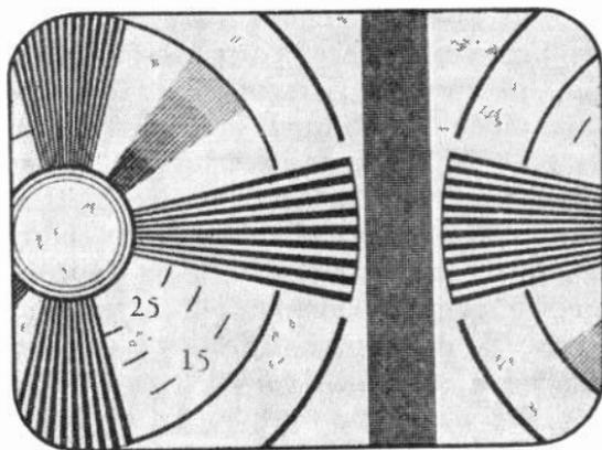
Fig. 13-5.—A blanking bar in the picture area indicates misadjustment of the discriminator phasing control.
