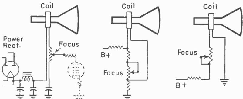
Fig. 15-9.—Circuits for control of magnetic focusing.
