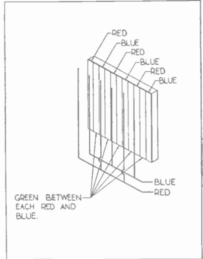
Fig. 4.—Grid structure for single-gun tube.
