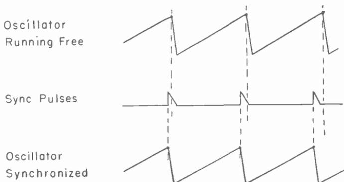
Fig. 12-11.—How sync pulse voltages bring the oscillator into time with the received signal.
