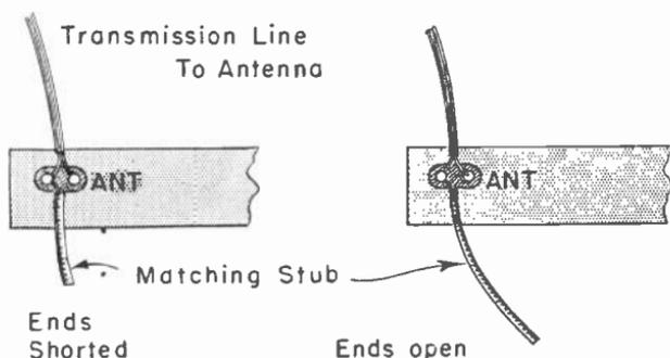
Fig. 17-13.—Matching stubs on antenna terminals of receiver.
