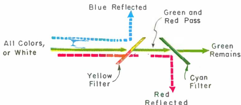
Fig. 18-14.—The principle of three-color separation by means of filters of colors complementary to the primary color bands.
