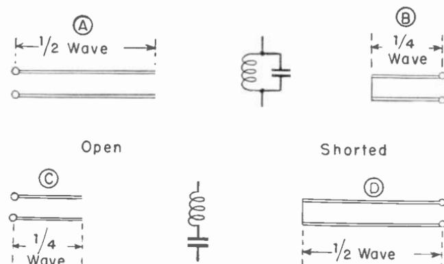
Fig. 18-26.—Half-wave and quarter-wave resonant lines act like parallel and series tuned circuits at the resonant frequencies.
