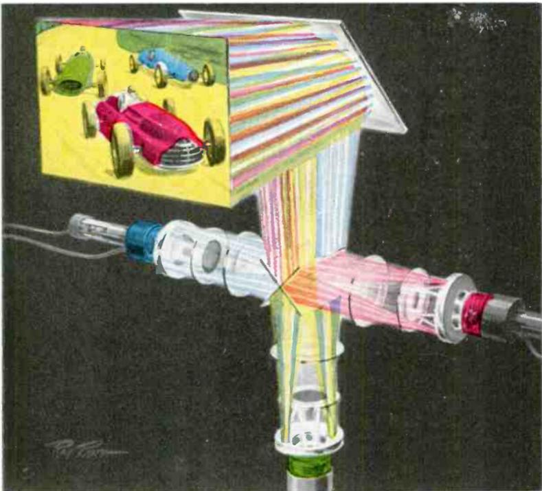
Fig. 18-12.—RCA full color reproduction method employing three projection kinescopes, a pair of dichroic mirrors, and a reflective optical system.
