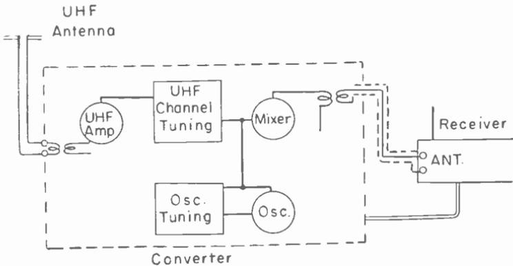
Fig. 18-28.—Principal parts for one style of uhf converter used with a vhf television receiver.
