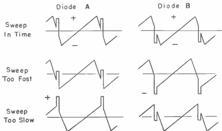
Fig. 13-7.—How sync pulse voltages and a sawtooth voltage from the sweep output combine in the phase detector.
