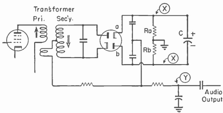
Fig. 7-4.—Ratio detector circuit showing points at which the output is measured.
