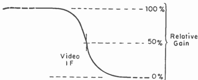
Fig. 5-4.—High-frequency end of a typical video i-f response curve.
