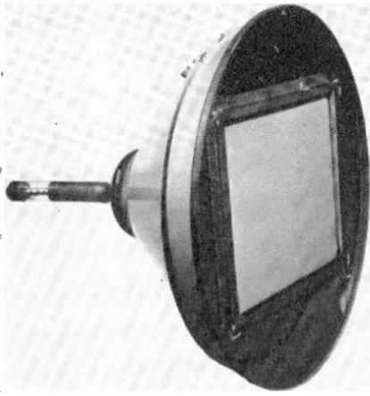
Fig. 1.—Front view shows 18.5-in. color face.
