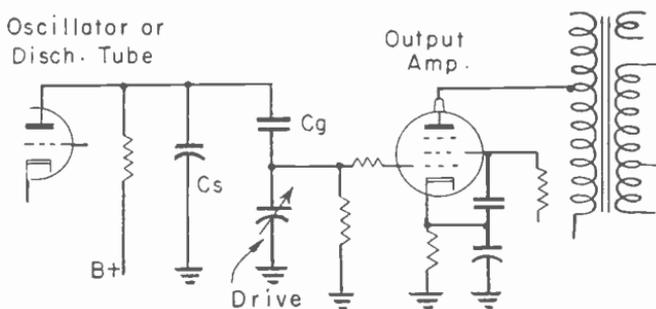
Fig. 14-13.—An adjustable capacitor as a drive control.
