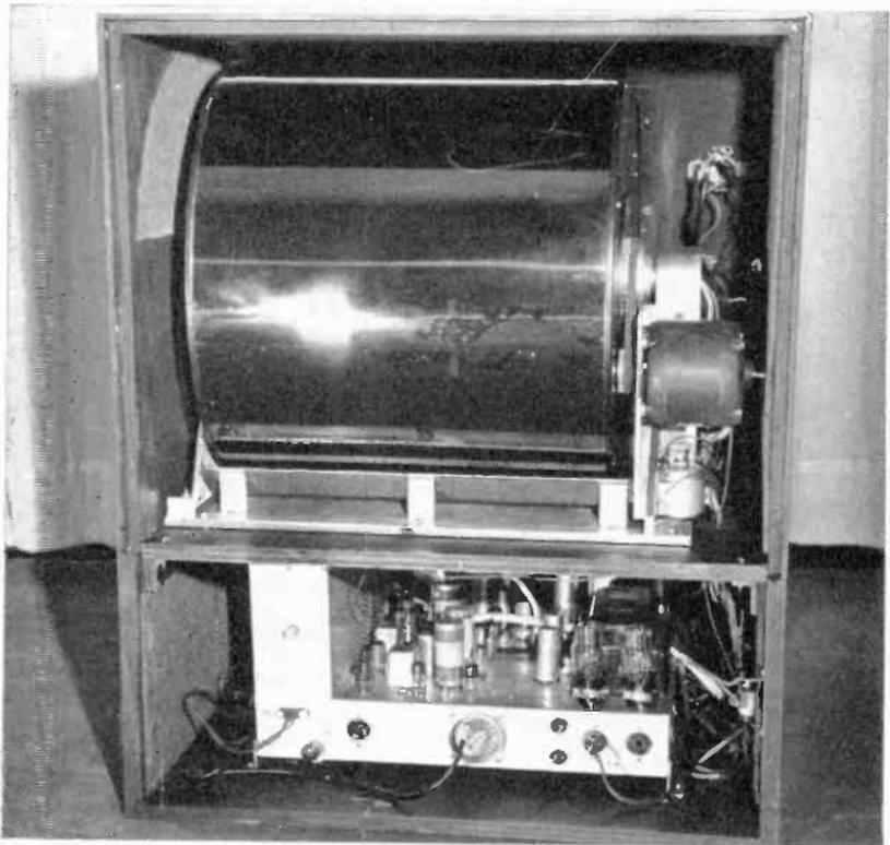
*Closeup of the rear of a TV set with new CBS color drum. Note drive at right of drum used to drive the drum around stationary picture tube. Connections to photo tube are made through hollow shaft on axle of drum color filter.*
