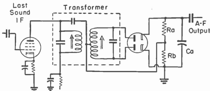
Fig. 4-11.—Typical circuit of Foster-Seeley discriminator for f-m sound.
