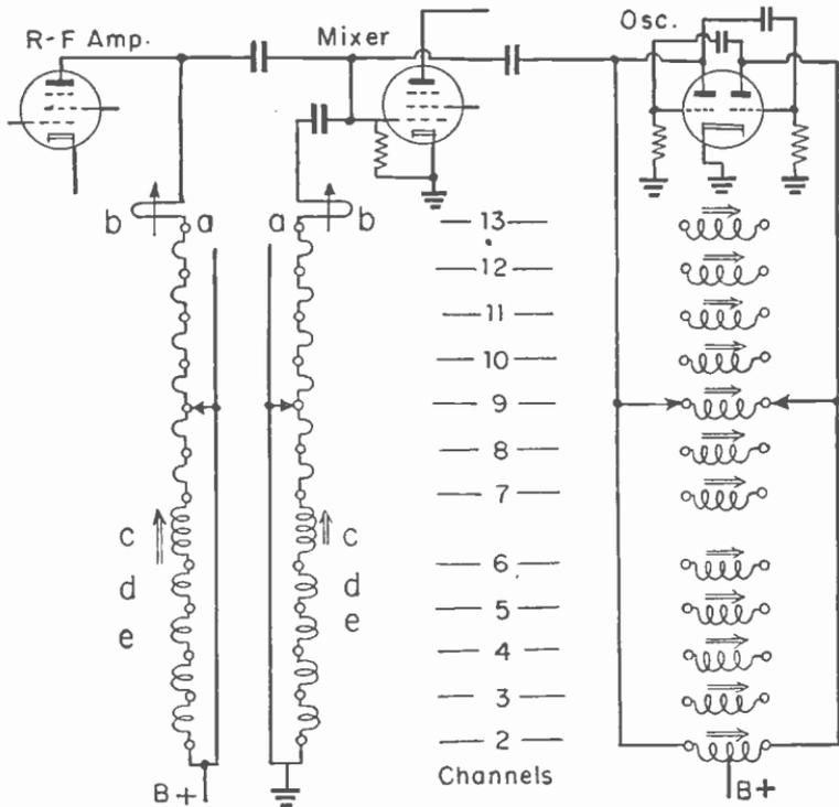
Fig. 8-1.—Rotary switch tuner with r-f adjustments for some channels and oscillator adjustments for all channels.
