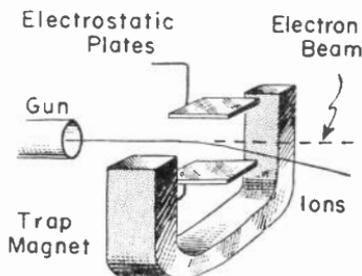
Fig. 15-14.—Ion traps which require only a single magnet.
