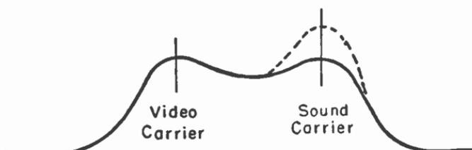
Fig. 4-3.—Frequency response of an r-f stage or a tuner.
