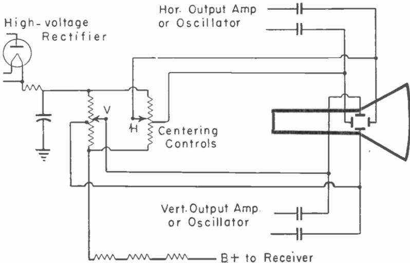
Fig. 15-11.—Circuits in general use for electrostatic centering.
