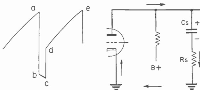
Fig. 12-10.—How a negative square wave is added to the sawtooth wave when the picture tube is operated with magnetic deflection.
