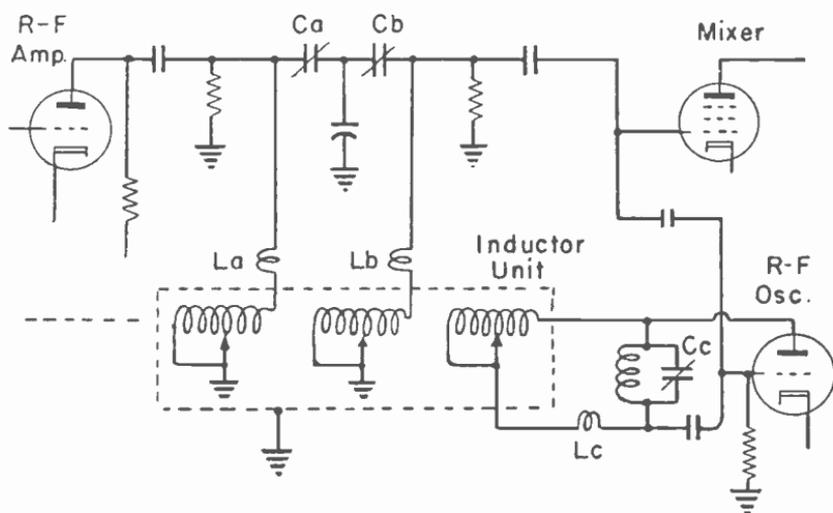
Fig. 3-5.—How a continuous tuner may be used between r-f amplifier and mixer tubes
