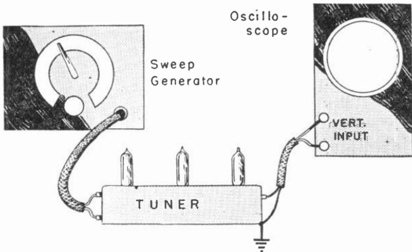
Fig. 2-5.—Voltage from the sweep generator is amplified in the tuner and applied to the oscilloscope.
