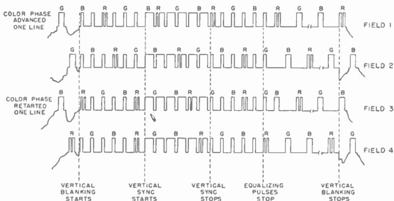
Fig. 18-20.—How a standard signal is modified for color scanning with the CTI method.
