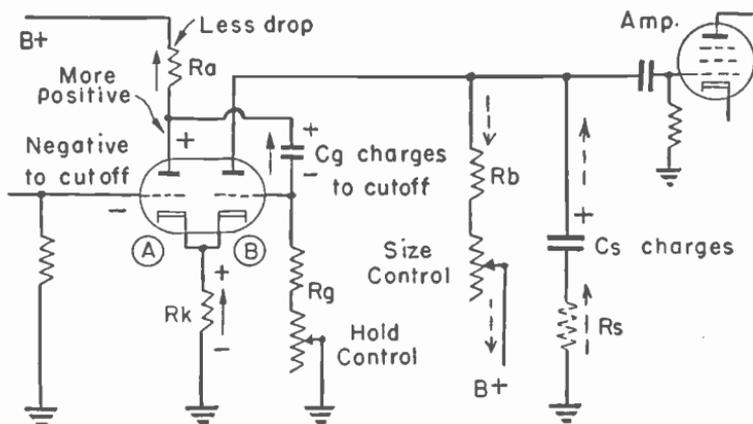
Fig. 12-6.—Connections for a multivibrator sweep oscillator.
