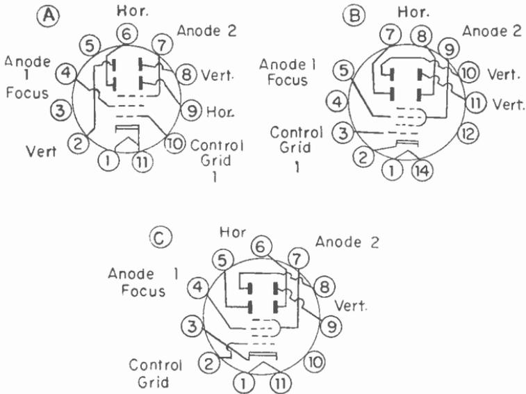
Fig. 15-2.—Basing connections for picture tubes having electrostatic deflection and focusing. A, 7EP4. B, 7GP4 and 7JP4. C, 3KP4.
