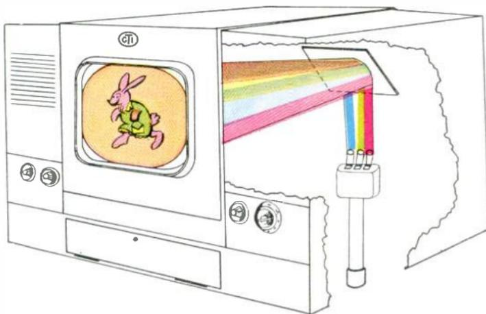
Fig. 18-18.—How the three color bands are combined on the projection screen.
