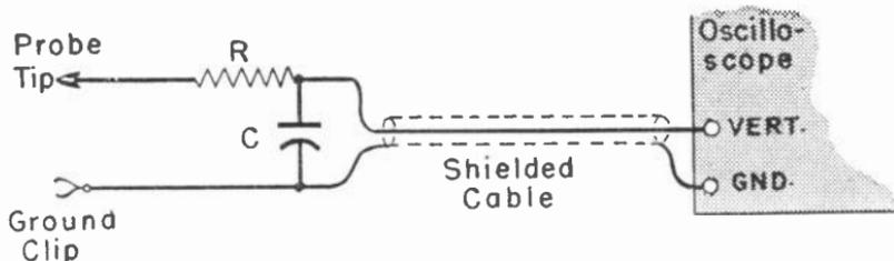
Fig. 2-15.—A low-pass filter probe for the vertical input of the oscilloscope.
