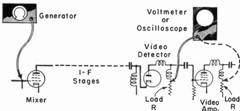
Fig. 6-7.—How the instruments are connected for alignment of traps.
