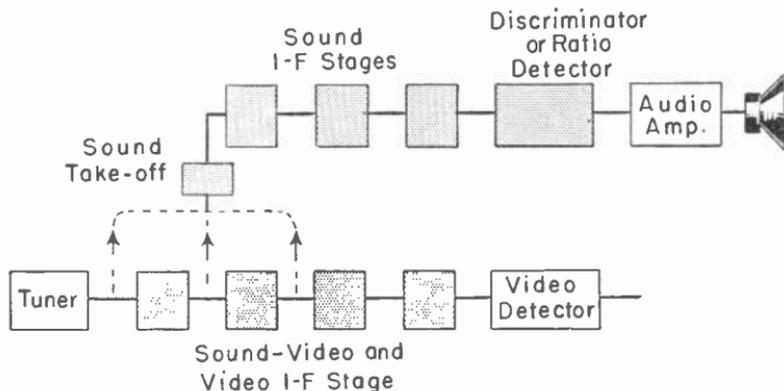
*Fig. 7-1.—A sound section operating at the sound intermediate frequency, with takeoff ahead of the video detector.*
