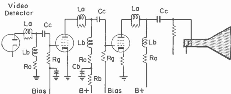
Fig. 9-9.—Connections in a typical two-stage video amplifier.
