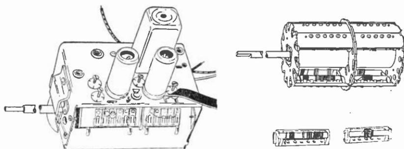
Fig. 3-4.—The parts of one style of turret tuner. (Stewart-Warner)
