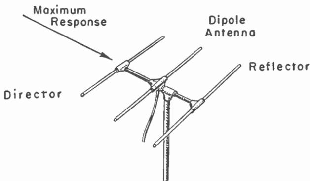
Fig. 17-5.—A simple dipole with director and reflector elements
