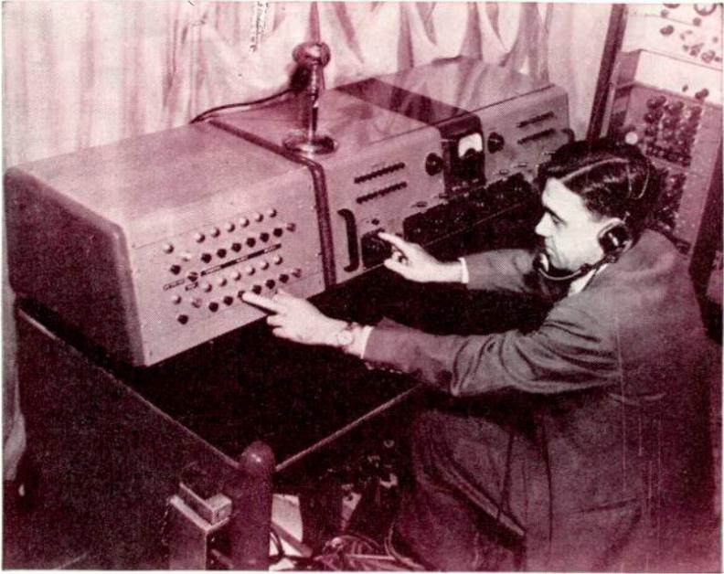
Fig. 18-23.—A studio control panel for the RCA color television system.
