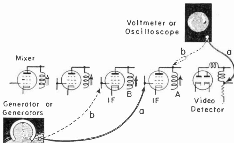
Fig. 6-13.—Instrument connections for observing the response and making alignment adjustments in individual stages.
