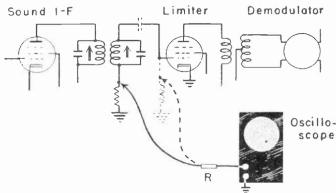
Fig. 7-8.—Oscilloscope connections to limiter grid circuits.
