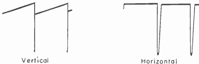
Fig. 15-7.—Oscilloscope traces taken from terminals of deflection coils.
