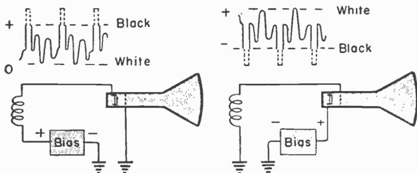
Fig. 1-13.—The television signal may be applied either to the cathode of the picture tube (left) or to the control grid (right).
