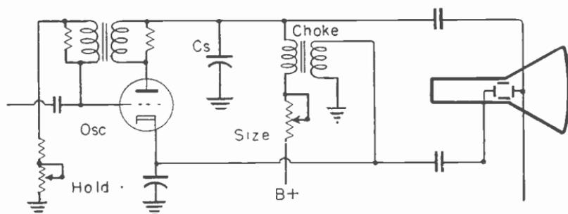
Fig. 14-5.—Electrostatic deflection system employing no amplifier.
