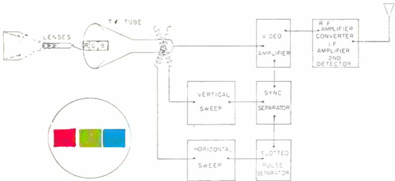
Fig. 18-17.—Principal parts of the CTI color receiver.
