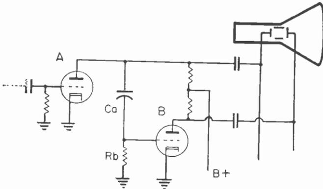
Fig. 14-2.—Capacitor coupling to the inverter for electrostatic deflection.
