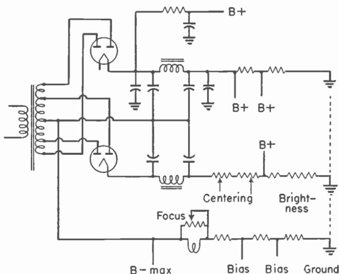
Fig. 16-11.—A low-voltage B-supply employing two rectifiers.
