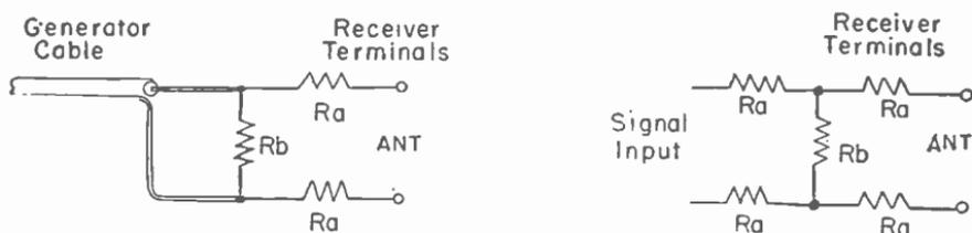
Fig. 8-6.—Impedance matching pad (left) and attenuator pad (right).
