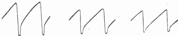
Fig. 14-16.—Oscilloscope traces showing the effect of adjusting a drive capacitor when there is feedback for production of negative pulses.
