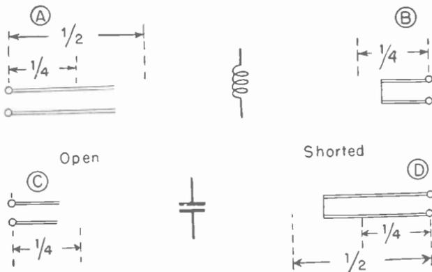
Fig. 18-27.—Lines less than half- or quarter-wavelengths long may act like inductance or capacitance added to tuned circuits.
