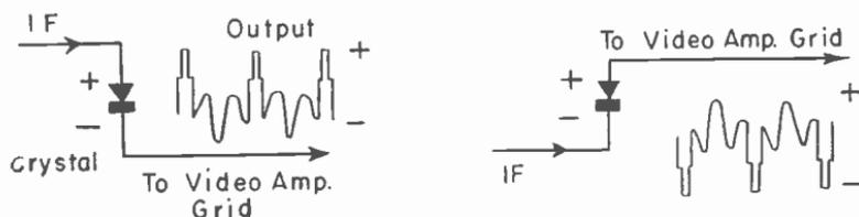
Fig. 9-5.—Signal polarities in the output of a crystal diode detector.
