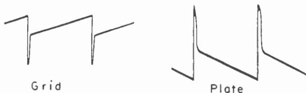
Fig. 14-8.—Oscilloscope traces from a vertical amplifier for magnetic deflection.
