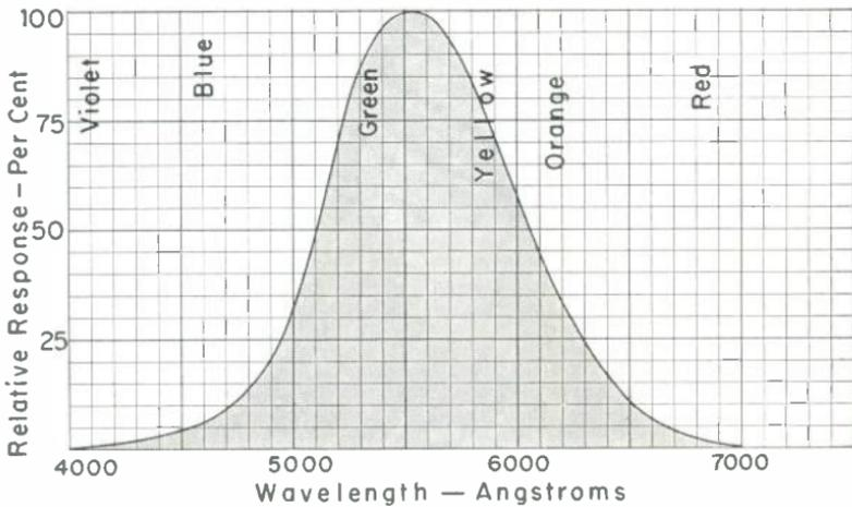
Fig. 18-2.—Relative average sensitivity of the human eye to radiation of equal intensity throughout the visible spectrum.
