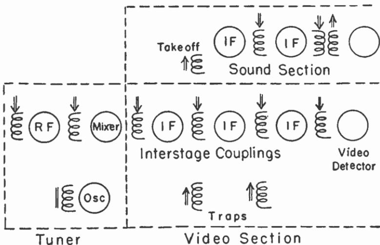
Fig. 6-1.—Points at which alignment may be required.
