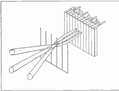
Fig. 3.—Three-gun electron beams through grid.
