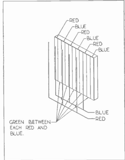
Fig. 4.—Grid structure for single-gun tube.
