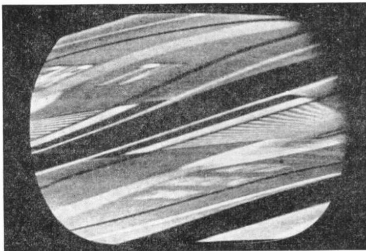
*Fig. 1-5.—This pattern indicates that the horizontal sweep oscillator is slightly out of synchronization.*
