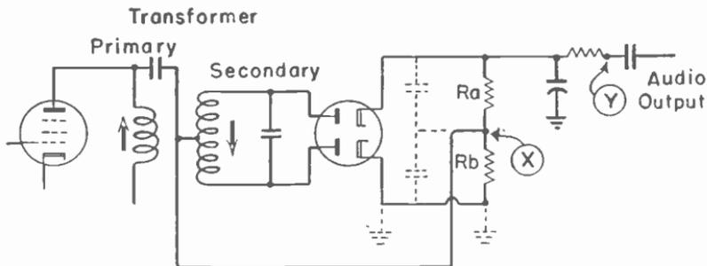
Fig. 7-3.—Discriminator circuit showing points at which the output is measured.
