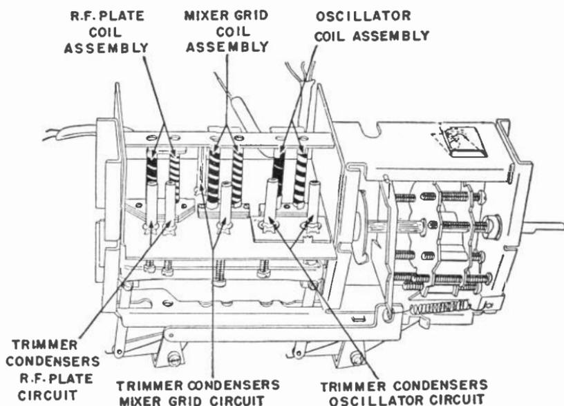
Fig. 3-6.—Construction of one style of two-band continuous tuner.
