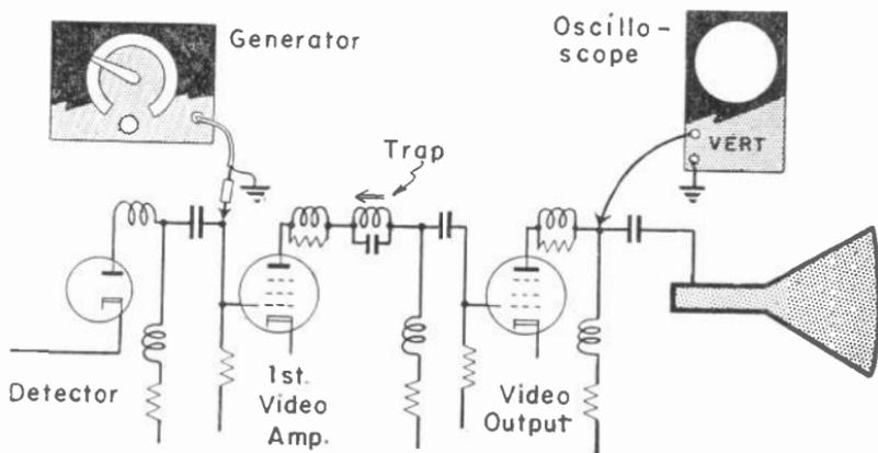
Fig. 9-10.—Alignment of trap for intercarrier beat frequency.
