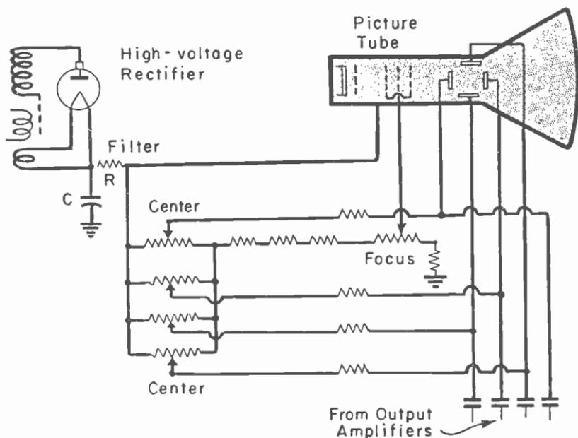
Fig. 2-21.—Circuits and parts at high voltage with an *r-f* voltage supply used with electrostatic deflection in the picture tube.
