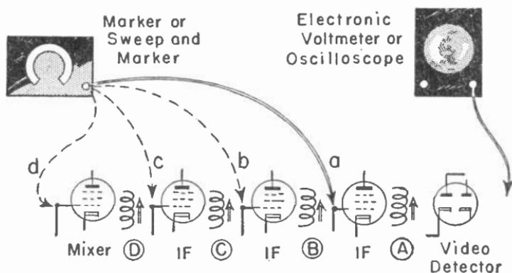
Fig. 6-12.—Connection from the generators may be moved back from grid to grid during alignment of successive stages.
