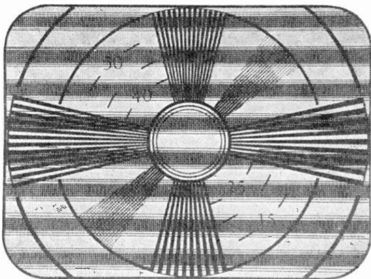
Fig. 6-8.—Sound bars on the screen of the picture tube.
