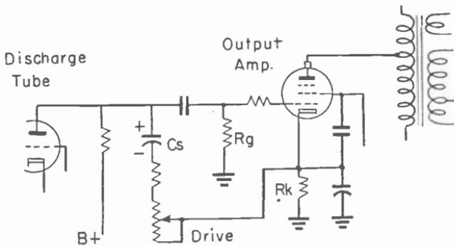
Fig. 14-10.—An adjustable resistor as drive control.
