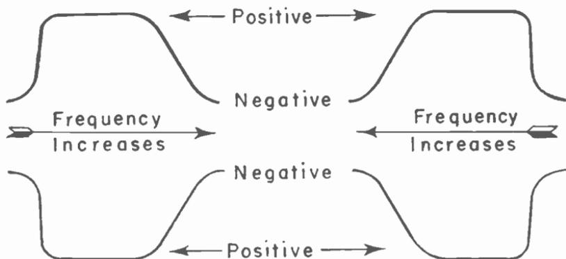
Fig. 2-16.—Responses and waveforms may be reversed and inverted in various ways as they appear on the oscilloscope trace.
