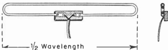
Fig. 17-2.—A half-wave folded dipole, a broad band antenna.
