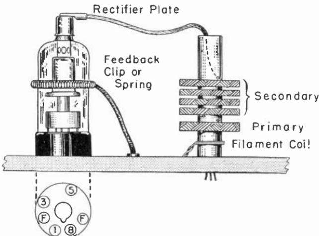
Fig. 16-8.—The 1B3 rectifier and the transformer for an oscillator type high-voltage supply system.
