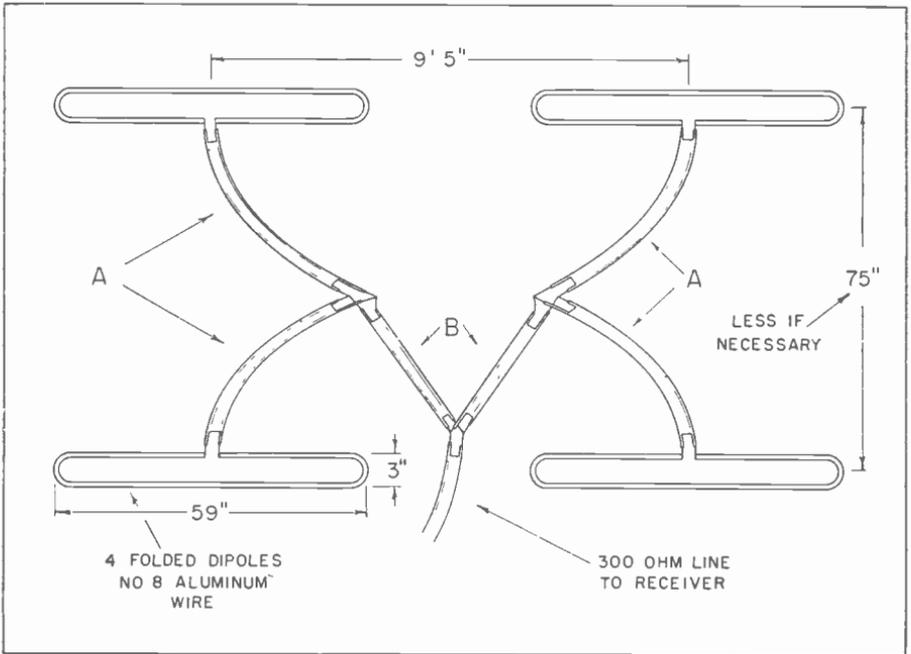
Figure 1. Four Dipole Receiving Array. Elevation View. Orient broadside to the direction of the desired signals. LEGEND: All connections made with 300 ohm twin lead. Leads "A"—Four equal length leads, any convenient length. Leads "B"—Two quarter-wavelength impedance matching sections, 26" long. Phase connections as shown. (Rightside of all dipoles connected together.)
