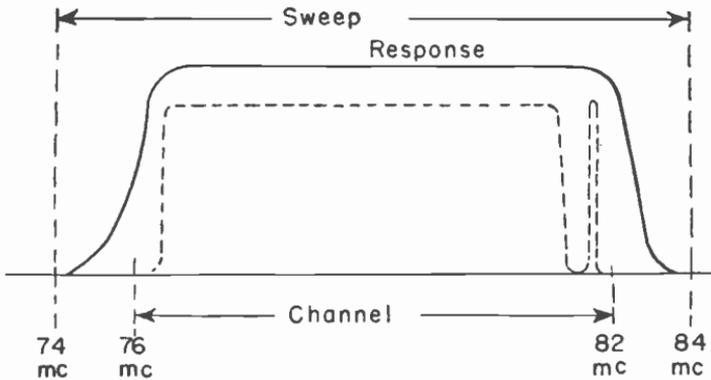
Fig. 2-2.—The frequency from the sweep generator shifts back and forth over a range somewhat greater than that of channel frequencies.
