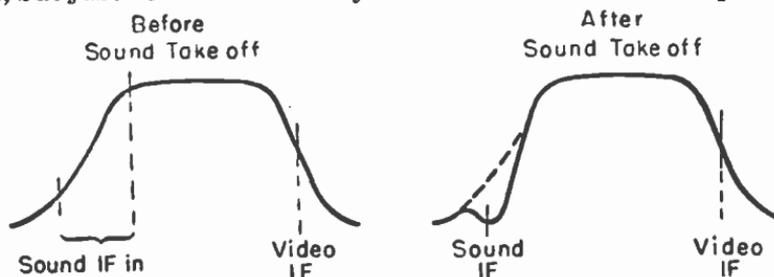
Fig. 4-4.—Video i-f responses where the sound system operates at the sound intermediate frequency.
