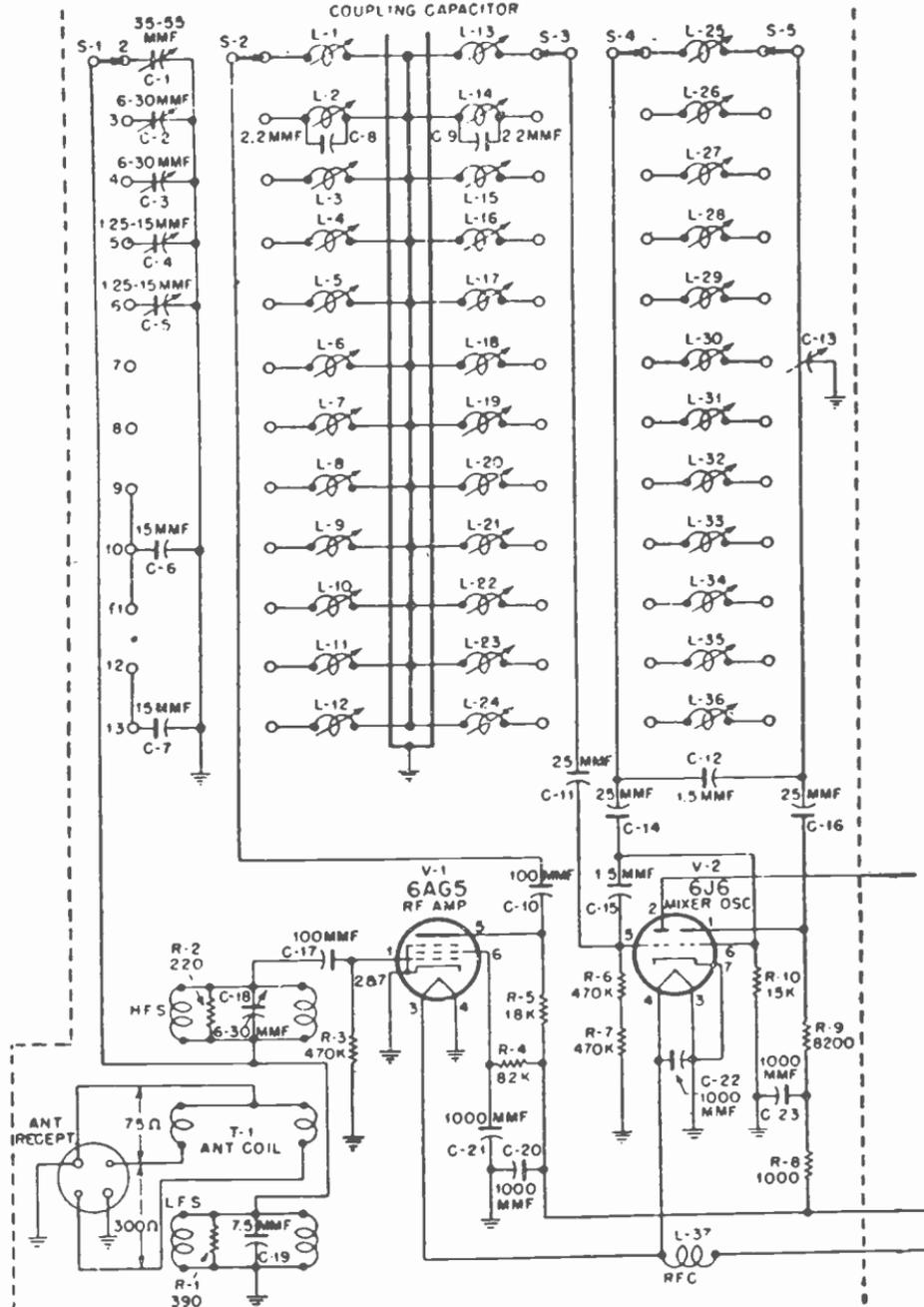
Fig. 3-7.—R-f input with tuning in two bands and connections for either of two types of transmission line. (Motorola)
