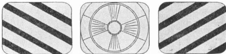
Fig. 12-12.—Changes produced in a pattern during adjustment of a horizontal hold control.
