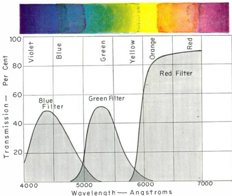
Fig. 18-3.—Transmissions of filters for separating the visible spectrum into three wavelength bands or color bands.
