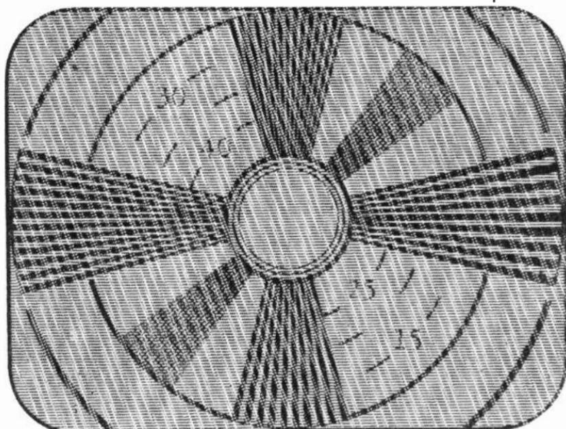
Fig. 5-16.—Effect of high-frequency interference experienced in some television channels.
