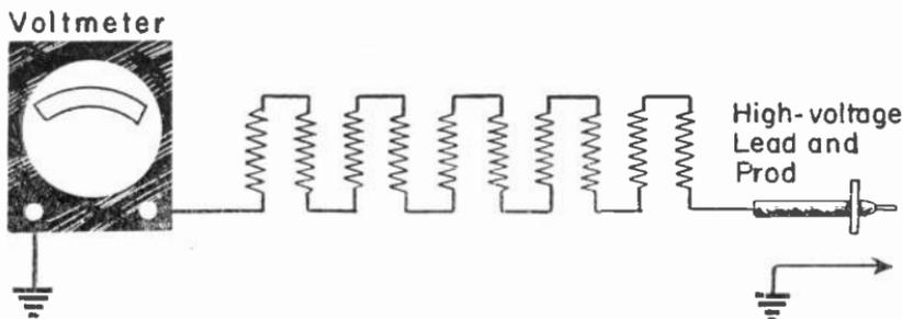
Fig. 2-22.—High-voltage multiplier assembled with resistors.
