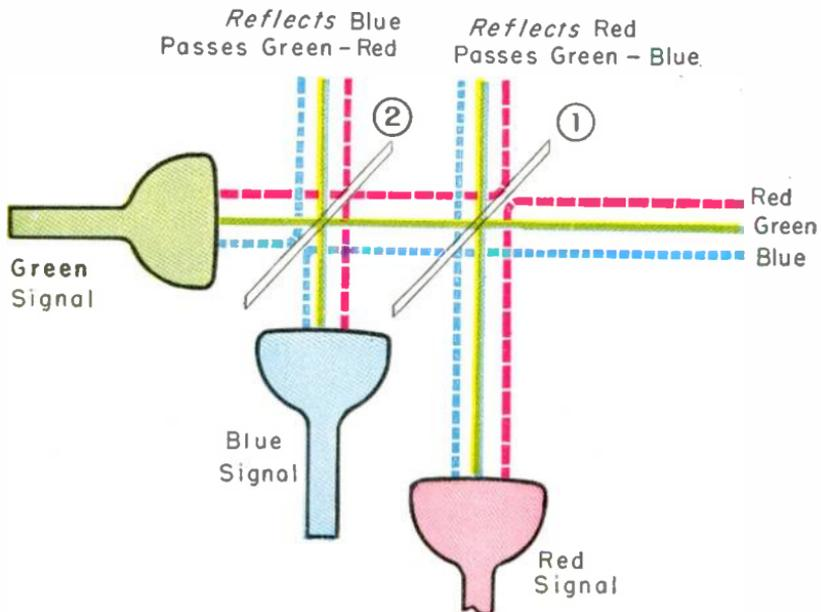
Fig. 18-11.—A direct view system which separates one color band from the light of each tube and combines the bands into a full color image.
