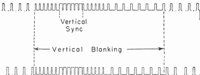
Fig. 1-14.—This is the portion of the television signal which synchronizes travel of the picture tube beam with the picture signals.
