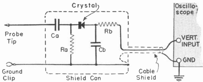
Fig. 2-7.—A detector probe using a crystal diode
