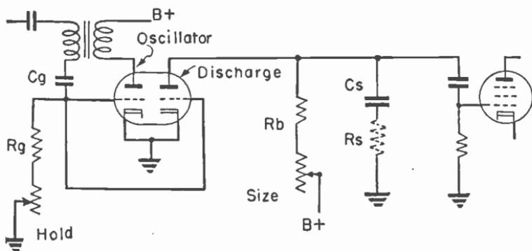
Fig. 12-5.—Blocking oscillator with discharge tube.
