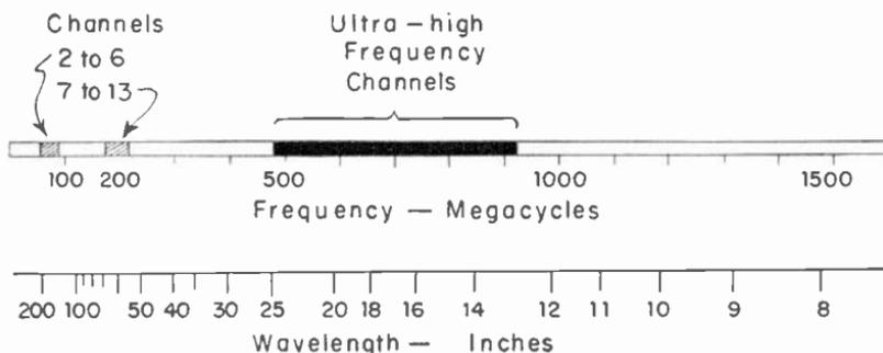
Fig. 18-25.—The relation of uhf television channels to channel 2-6 and 7-13 in the frequency spectrum.
