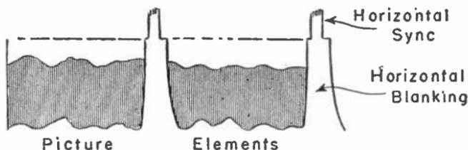
Fig. 9-8.—Signal between video detector output and picture tube input with oscilloscope synchronized for 7,875 cycles per second.
