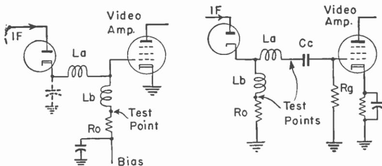
Fig. 9-3.—Video detector circuits in which i-f input is to the plate of the diode.
