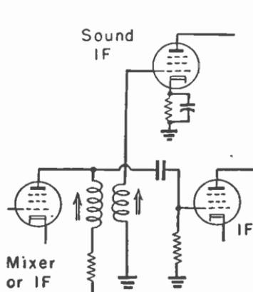
Fig. 4-7.—Tuned sound takeoff from an interstage tuning coil.
