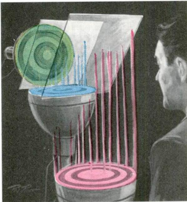
Fig. 18-10.—RCA direct view color reproduction system using three kinescopes and two dichroic mirrors.
