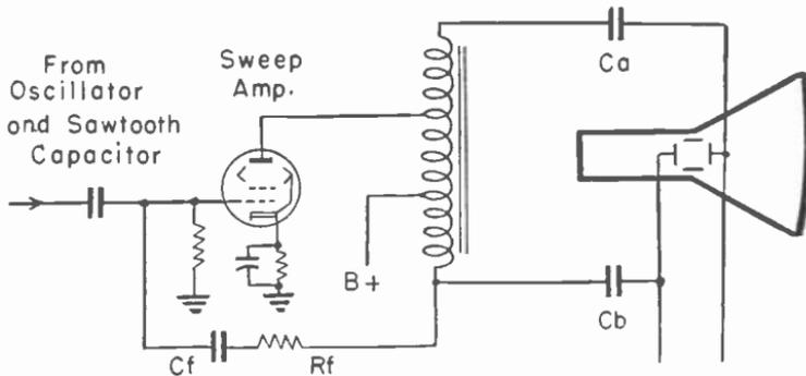
**Fig. 14-4.—Vertical electrostatic deflection with a single amplifier.**
