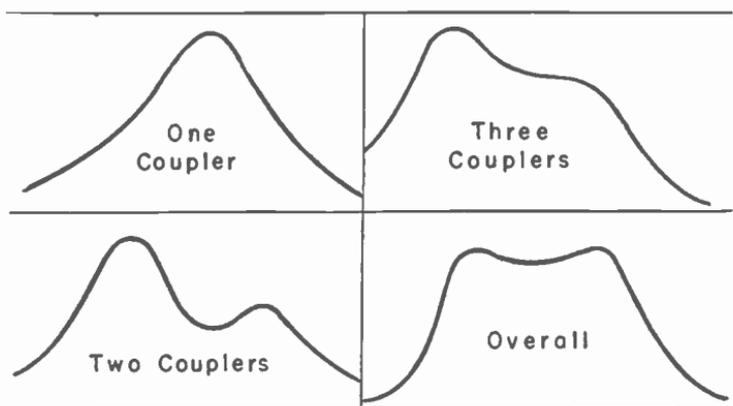
Fig. 6-18.—Typical responses when aligning to include one additional coupler at each successive step.
