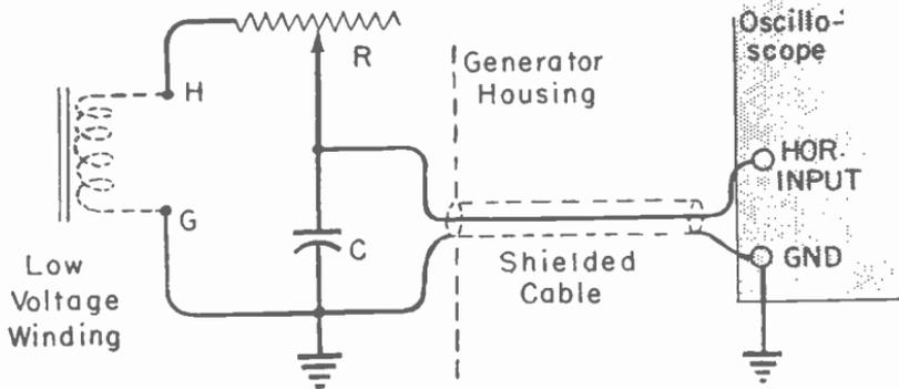
Fig. 2-10.—A circuit for phasing horizontal deflection in the oscilloscope with the sweep of frequency from the generator.
