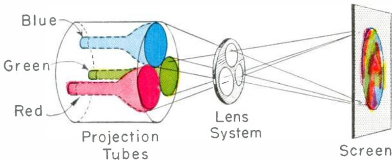
Fig. 18-5.—Three images for the three color bands are combined for reproduction of a full color picture. This is one of many methods used for combination.
