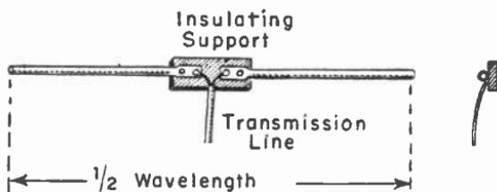
Fig. 17-1.—A simple half-wave dipole antenna for television.
