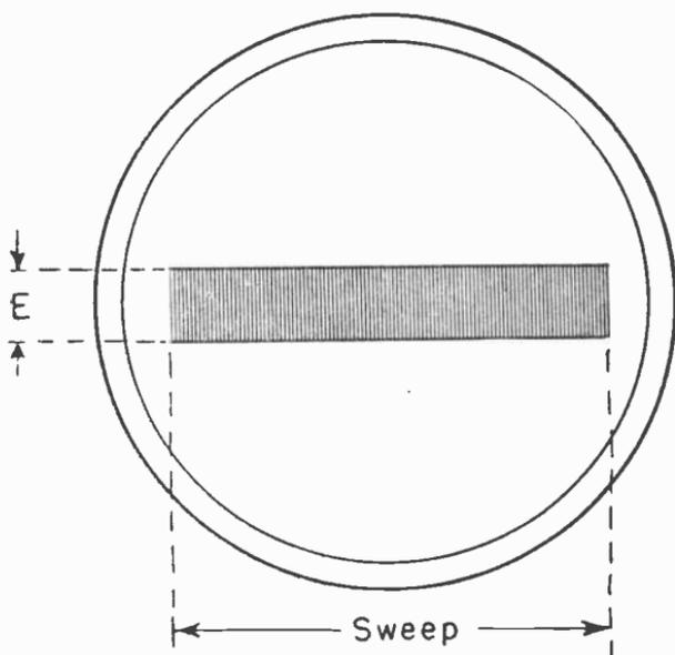
Fig. 2-4.—At very low frequencies the scope trace may show vertical deflection corresponding to sweep generator output voltage.
