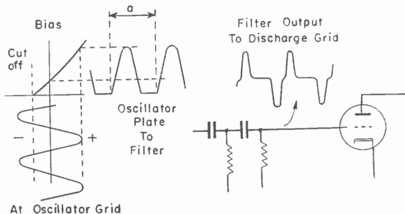
Fig. 13-8.—How the hold control varies the width of square waves from the oscillator, and the time between leading edges of pulses applied to the discharge tube grid.
