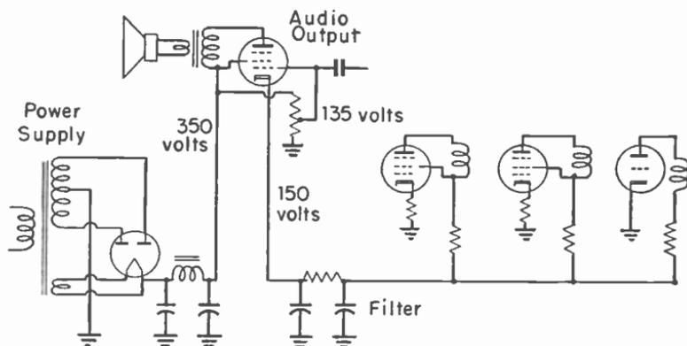
Fig. 16-12.—Three tubes in a parallel connected group which is in series between cathode and ground of an audio output tube.
