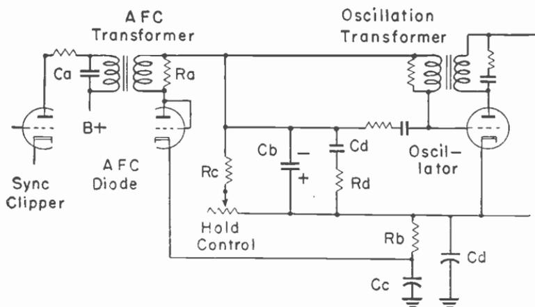
Fig. 13-14.—Horizontal afc system employing a diode-connected triode for varying the oscillator grid voltage.
