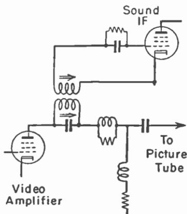
Fig. 4-8.—Takeoff commonly used for intercarrier sound.
