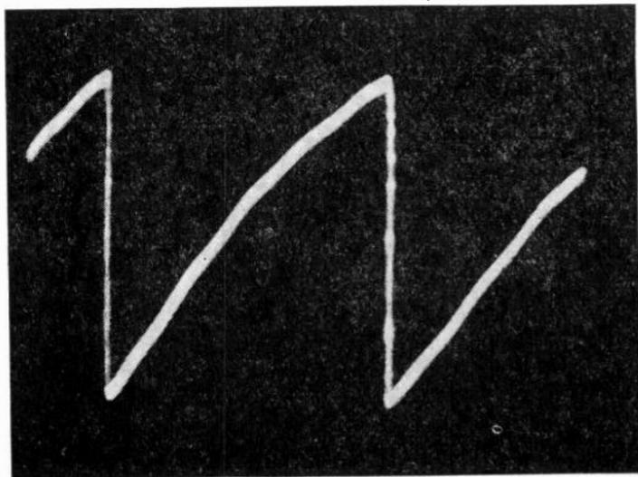
Fig. 1-10.—This trace shows the output of a vertical sweep oscillator. (Courtesy of Motorola Inc.)
