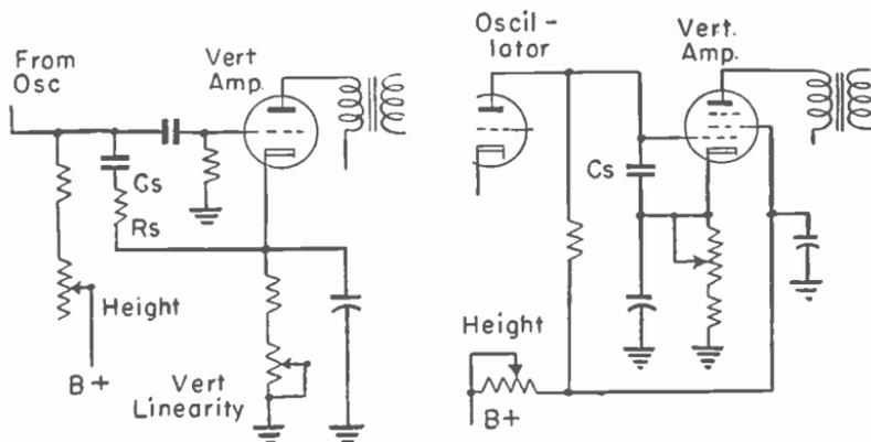
Fig. 14-7.—Circuits for sawtooth capacitors in vertical amplifier systems for magnetic deflection.
