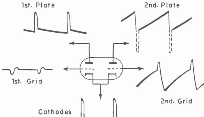
Fig. 12-8.—Waveforms observed at the several elements of a multivibrator used for vertical sweep.
