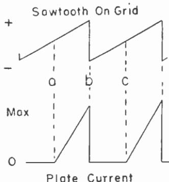
Fig. 14-18.—Pulses of plate current resulting from sawtooth voltage on amplifier grid.
