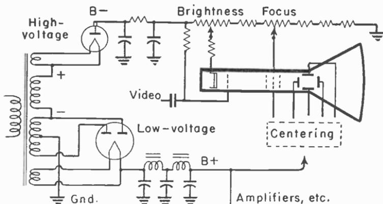
Fig. 16-2.—High-voltage rectifier in series with negative side of low-voltage rectifier.
