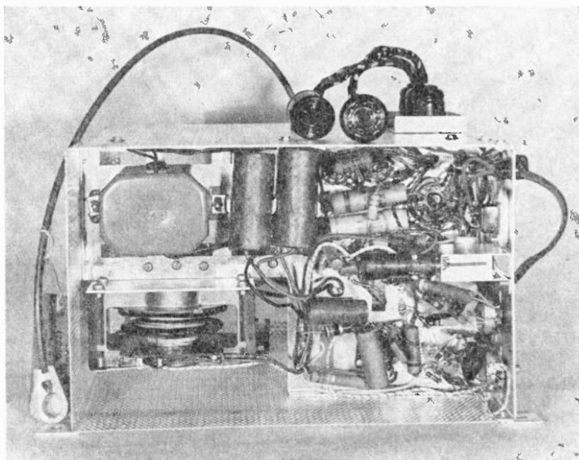
Fig. 16-5.—Bottom view of the Du Mont high-voltage power supply chassis.
