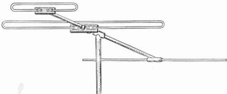
*Fig. 17-7.—Dual antenna with the high-band element in front of the low-band element and with a single reflector at the rear.*
