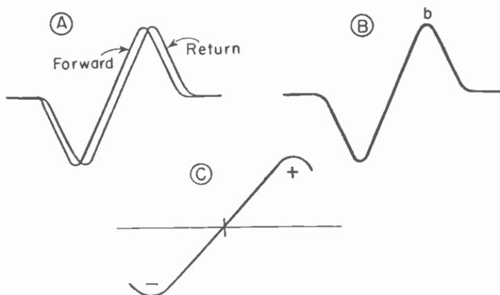
Fig. 7-11.—S-curves obtained when using a synchronized sweep voltage for the horizontal input of the oscilloscope.
