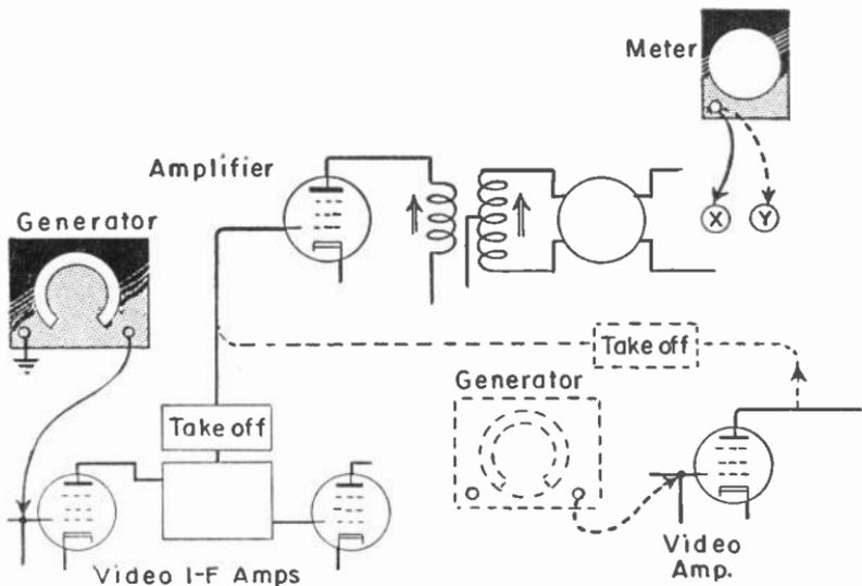
Fig. 7-5.—Generator connections for alignment in sound section.
