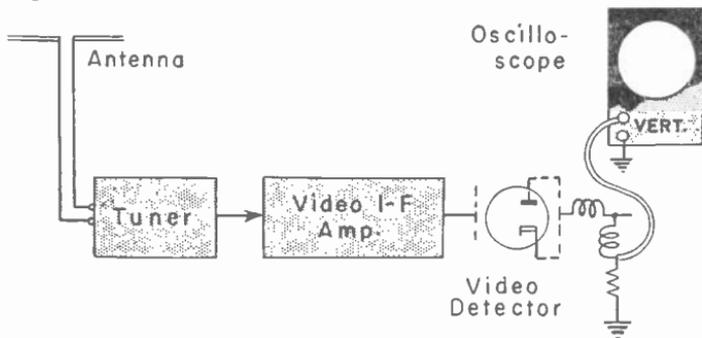
Fig. 9-6.—Connections for observing the signal waveform at the output of a video detector.
