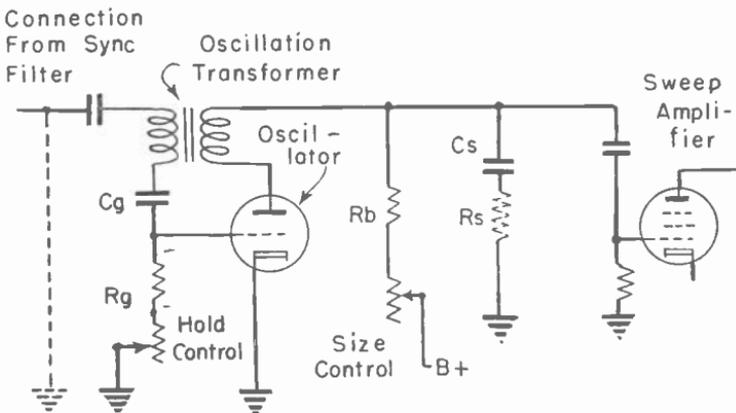
Fig. 12-1.—Connections in the circuits for a blocking oscillator.
