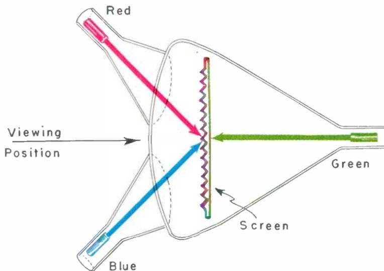
*Fig. 18-13.—Three-color reproduction by means of three electron beams acting on a screen having phosphors which emit the three color bands.*
