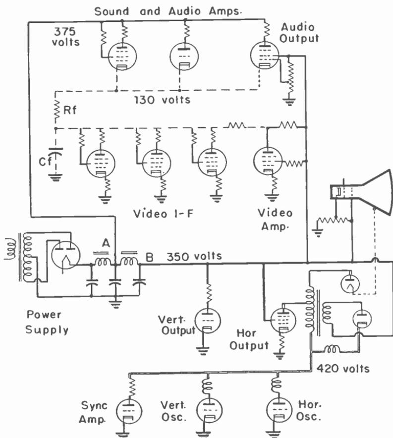
Fig. 16-13.—B-power supply circuits from which a number of different plate, screen, and anode voltages are obtained without voltage dividers.
