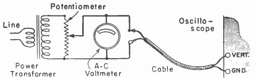
Fig. 2-17.—A unit for providing oscilloscope traces whose height may be translated into applied voltage.
