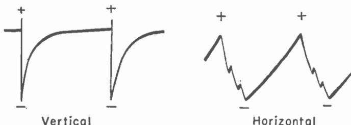
Fig. 12-2.—Traces observed with the oscilloscope connected to the grid of a blocking oscillator.
