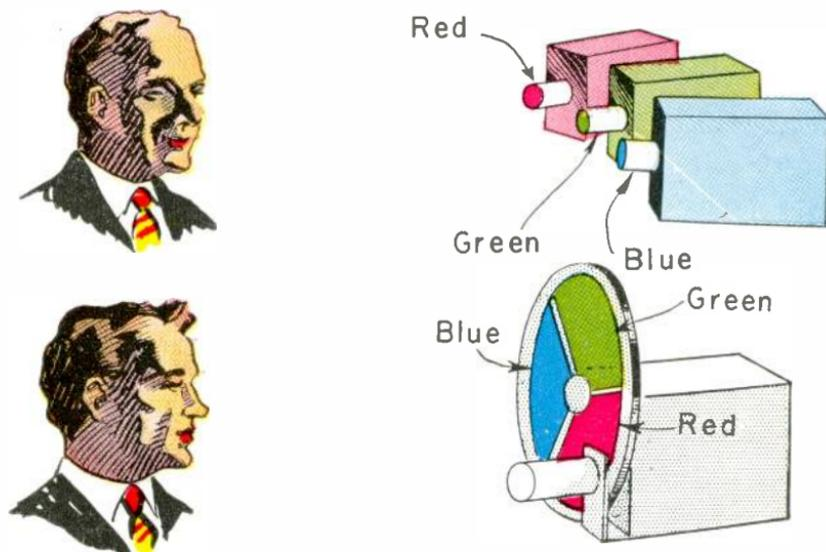
Fig. 18-4.—The three color bands may be picked up by three separate cameras or by a single camera with rotating three-color filter disc.
