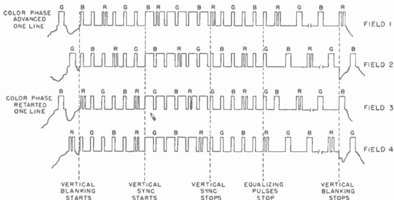
Fig. 18-20.—How a standard signal is modified for color scanning with the CTI method.
