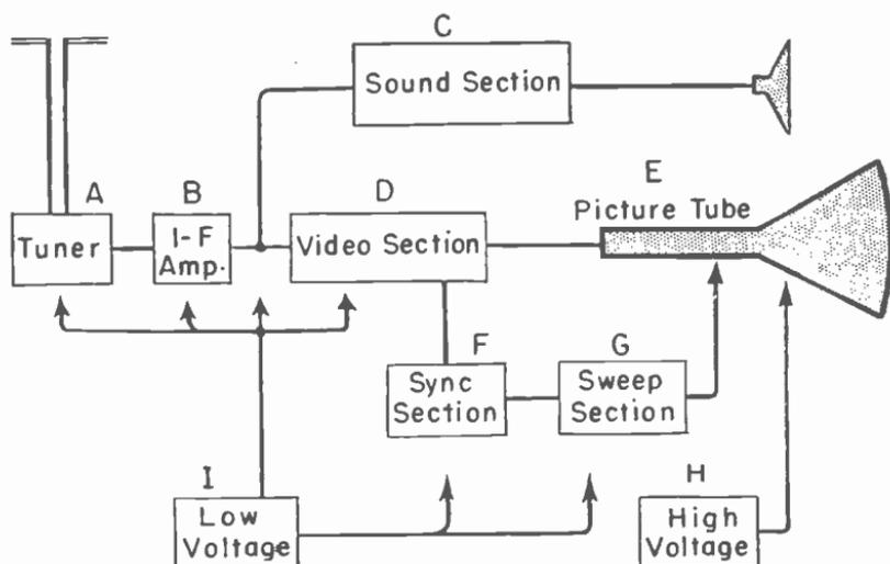
Fig 1-3.—As a first step in trouble shooting we try to localize the fault in some of these major sections.
