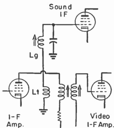
Fig. 4-10.—An inductively coupled sound takeoff.
