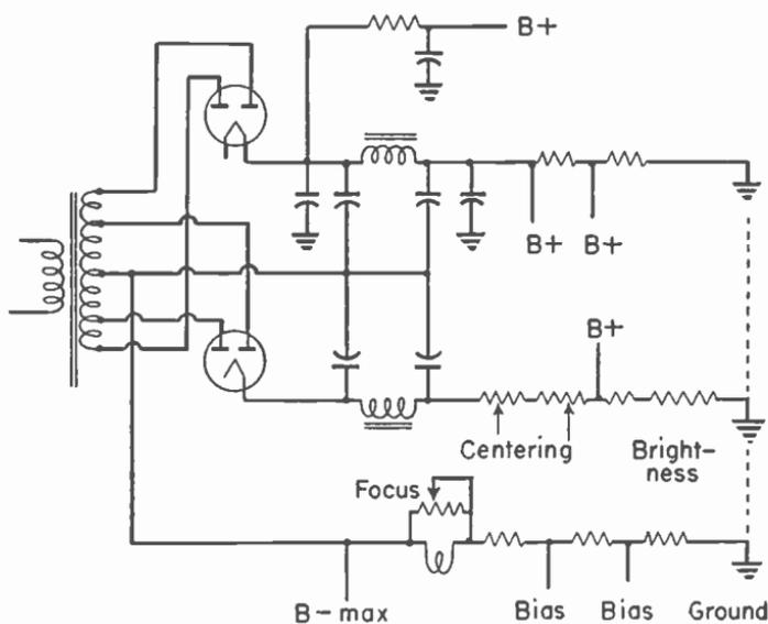
Fig. 16-11.—A low-voltage B-supply employing two rectifiers.
