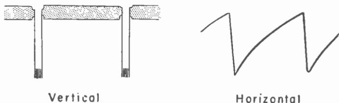
Fig. 11-4.—Synchronizing voltage traces from a restorer plate and from some kinds of takeoff diodes.
