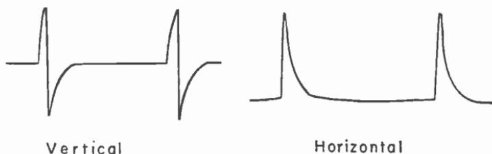
Fig. 11-3.—Triggering voltages for application to sweep oscillators.
