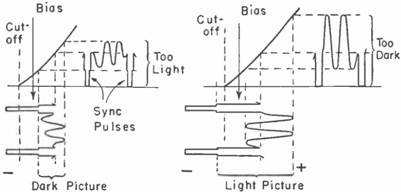
Fig. 10-7.—Effects of darker pictures (left) and of lighter pictures (right) when the picture tube grid bias is not altered.
