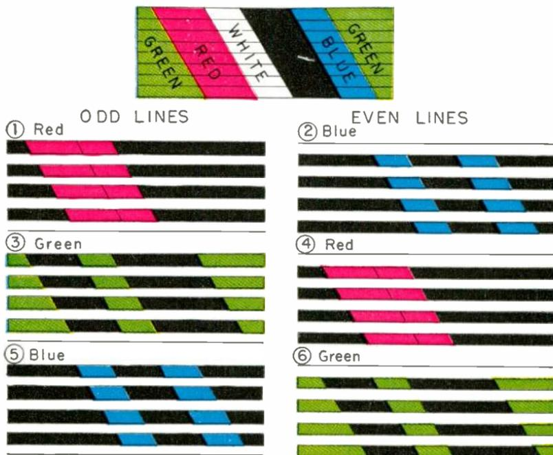
Fig. 18-6.—How the color bands are scanned and recombined to form all hues as well as white and black in the full color picture of a CBS system.
