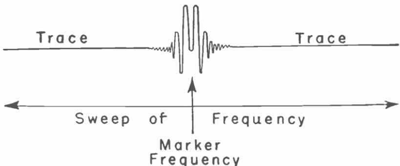
Fig. 2-12.—A marker produced by beating of frequencies from the two generators.
