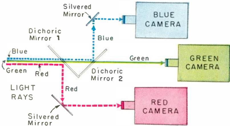
Fig. 18-9.—The principle of three-color separation by means of dichroic mirrors which combine transmission and reflection.
