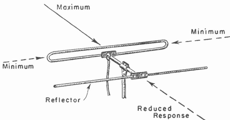
Fig. 17-4.—A folded dipole with reflector element.
