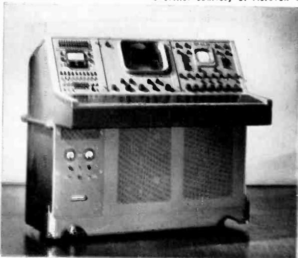
Fig. 18-29.—Cont-ol desk and color monitor for the special equipment designed and developed by CBS for Smith, Kline & French Co. This equipment is being used at medical conventions to bring surgical operations to convention delegates in color. An increasing use of color television in medical schools is predicted in the future.
