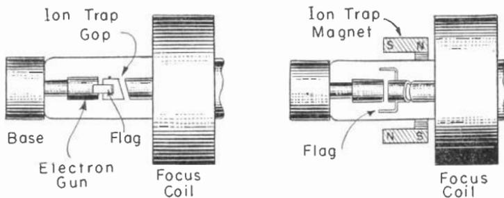
Fig. 15-13.—The ion gap in an electron gun and an ion trap of the permanent magnet type.
