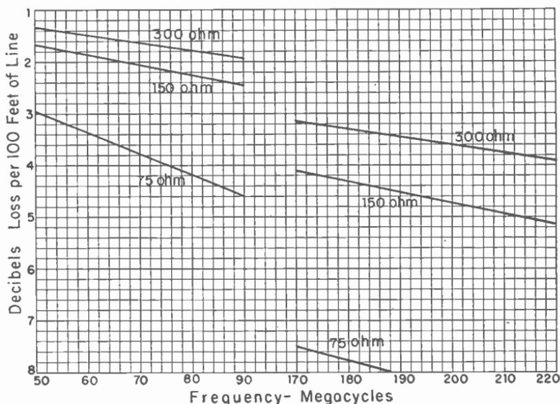
Fig. 17-15.—Losses in three types of twin-lead unshielded transmission line at television frequencies.
