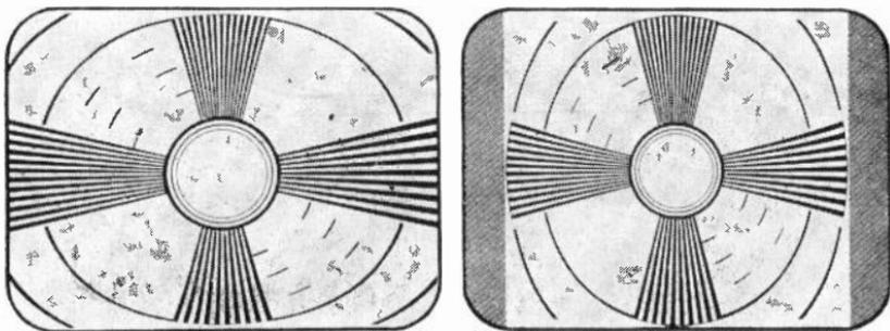
Fig. 14-17.—How the pattern is affected by incorrect adjustment of the width control.
