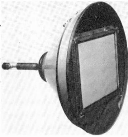
Fig. 1.—Front view shows 18.5-in. color face.
