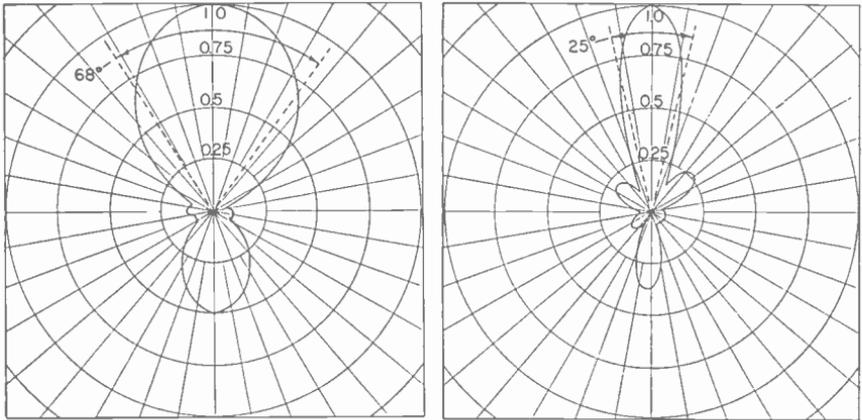
Figs. 2 & 2A. Horizontal and vertical radiation patterns.
