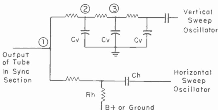
Fig. 11-6.—Typical connections for vertical and horizontal filters which separate the two kinds of pulses.
