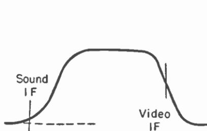
Fig. 4-5.—Video i-f response when intercarrier sound is used.
