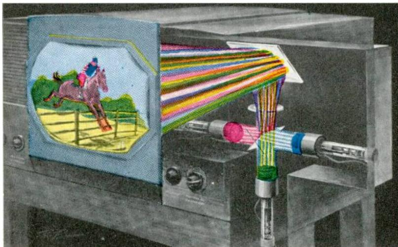
Another view of an RCA color television converter, using small projection kinescopes and refractive optics.
