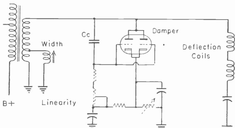
Fig. 14-25.—A twin triode used as the damper tube.
