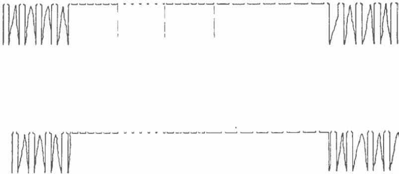
Fig. 1-12.—This is the portion of the television signal which produces pictures.
