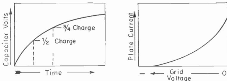
Fig. 14-22.—A non-linear sawtooth charging curve may be compensated for by a non-linear grid-plate characteristic of the amplifier.
