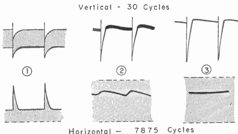
Fig. 11-7.—Oscilloscope traces at various points in a vertical filter.
