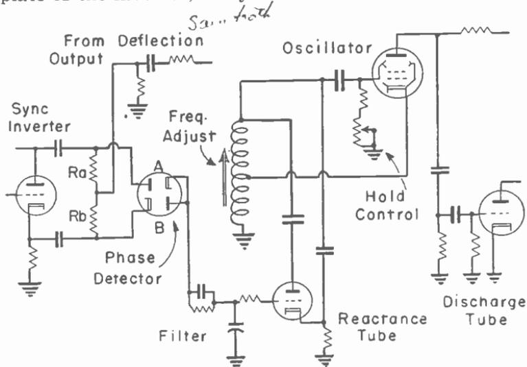
Fig. 13-6.—Horizontal afc system including a phase detector and reactance tube.
