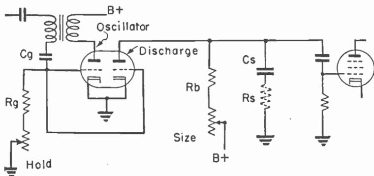
Fig. 12-5.—Blocking oscillator with discharge tube.
