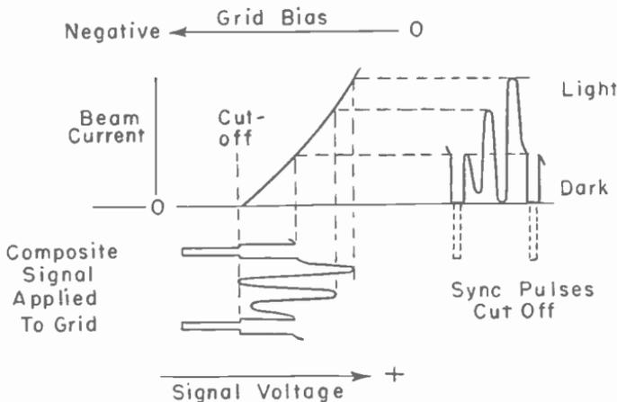
Fig. 10-3.—A composite signal applied to the beam-current grid-voltage characteristic of a picture tube.
