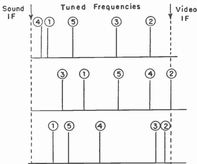
Fig. 5-8.—Some frequencies used with five tuned couplings, as related to the respective sound and video intermediate frequencies.
