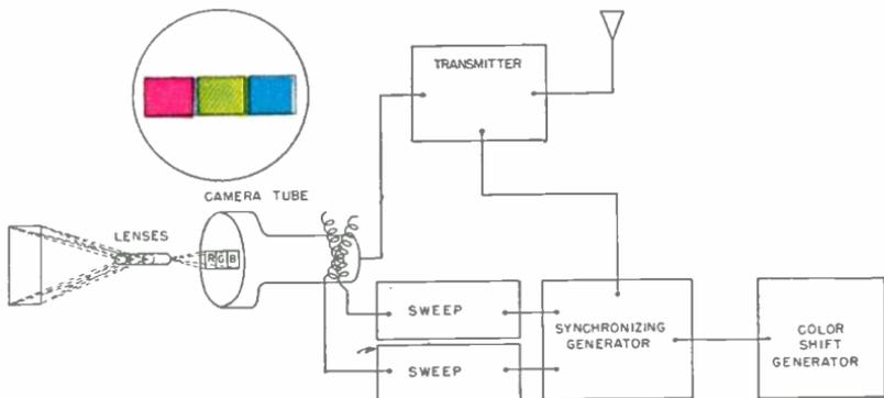
Fig. 18-16.—Principal parts of the CTI color transmitter.
