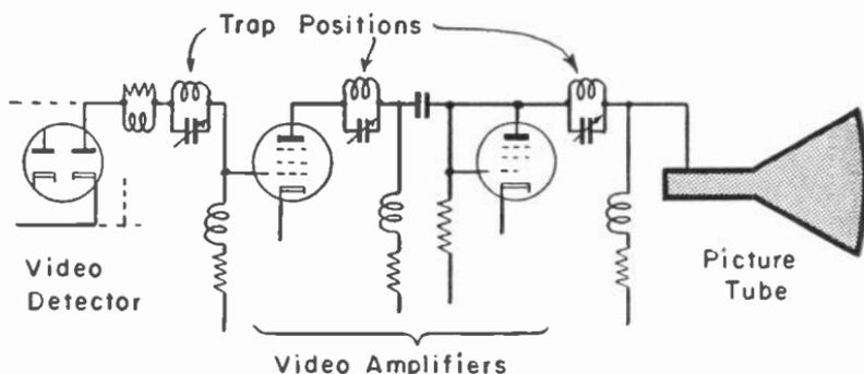
Fig. 5-18.—Traps used for the intercarrier beat frequency.
