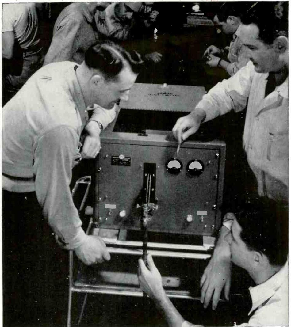
The unit shown above is a commercial High Frequency Induction Heater of the type that is used for soldering and heat treatment of metals.
