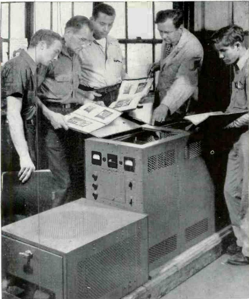
This picture shows students getting instruction on the operation of a Dielectric Heating unit used in plastic moulding and sealing of Vinylite material for raincoats, aprons, tablecloths, etc.
