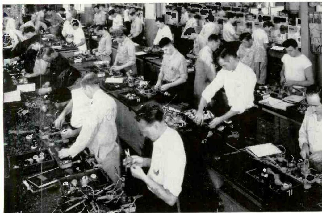
General view of a section of Basic Electricity and Circuits. Notice the large and well lighted shop. The men are wiring and testing light control circuits in their first small conduit layout, and getting real practical experience in the handling of tools and the use of various kinds of switches.
