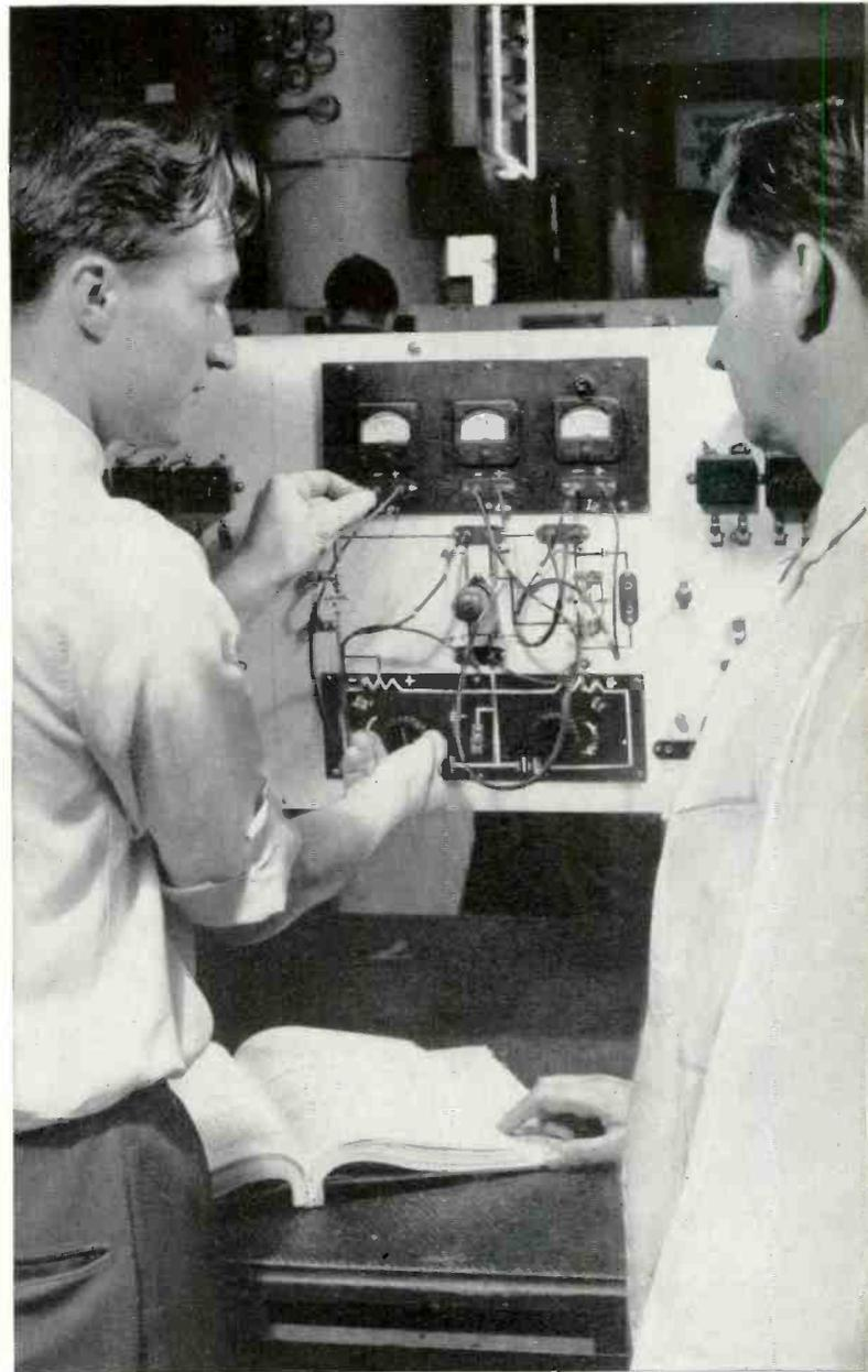
These students are plotting characteristic curves of Vacuum Tubes. In this job, students observe the action of a tube under conditions similar to actual operating conditions to help them understand why a tube will amplify a signal.
