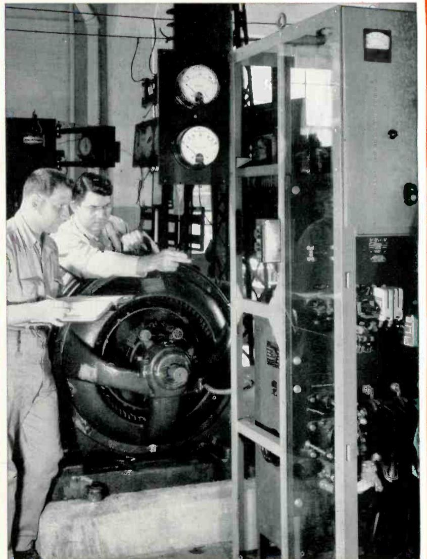
The above photo shows an Instructor explaining the operation and adjustments for synchronous type motor and students preparing to make tests. This unit is used for correcting Power Factor. Every trained maintenance man should be familiar with this type of work.
