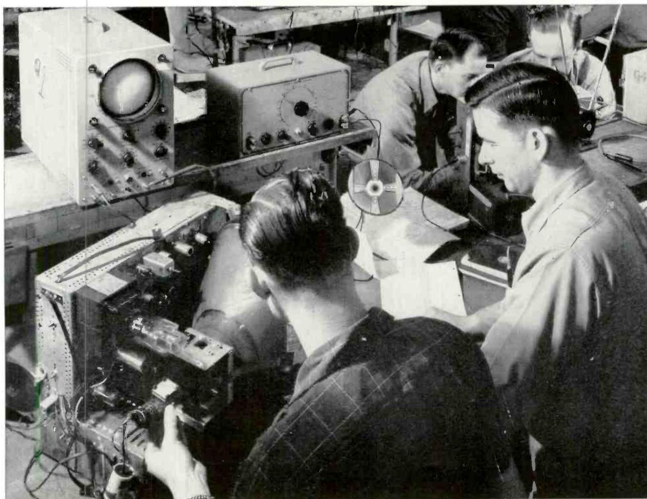
In the job pictured above, students are adjusting the ion trap in a Receiver. In this shop job, students perform the same operations that a serviceman does when installing a new TV set or assembling one after repairs.
