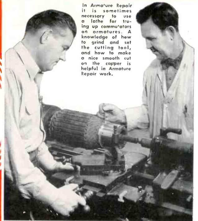
In Armature Repair it is sometimes necessary to use a lathe for truing up commutators on armatures. A knowledge of how to grind and set the cutting tool, and how to make a nice smooth cut on the copper is helpful in Armature Repair work.
