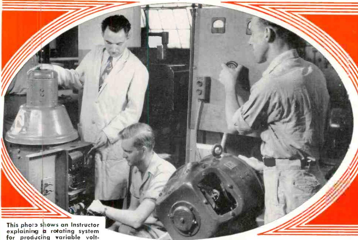
This photo shows an Instructor explaining a rotating system for producing variable voltages used in obtaining a wide range in motor speeds. These units are used extensively in Textile, Food, Metal, Paper, Printing, Rubber, Machine Tool, Wire and Cable industries.
