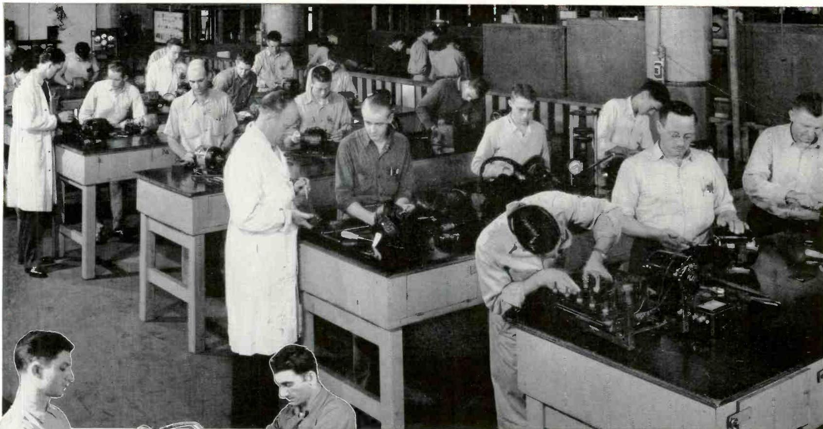
This is a view of the Electric Appliance Repair section showing students getting real practical training on various Testing, Adjusting and Repairing operations on Motors, Controls and other types of Electrical apparatus. This is a profitable field of opportunity to the man in the field, whether he is working for a Service Organization or Operating a Business of his own.
