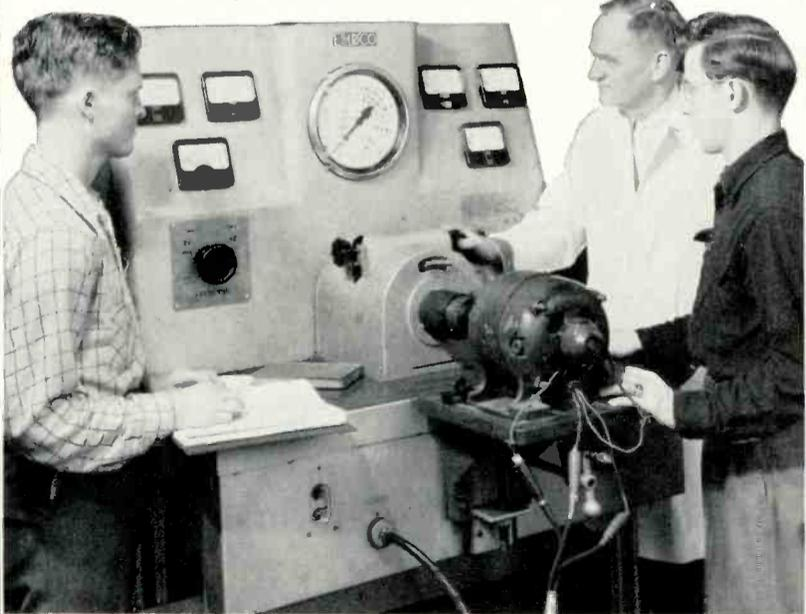
These Coyne students are testing the efficiency of a motor with a modern Dynamometer, a type used extensively in industry for testing A.C. and D.C. motors.
