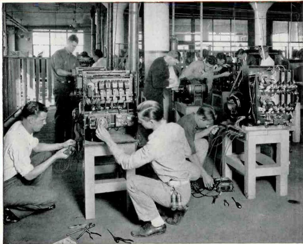
And here we have different types of modern automatic, remote control equipment for A. C. motors. These men are getting acquainted with the care and operation of this type of equipment.
