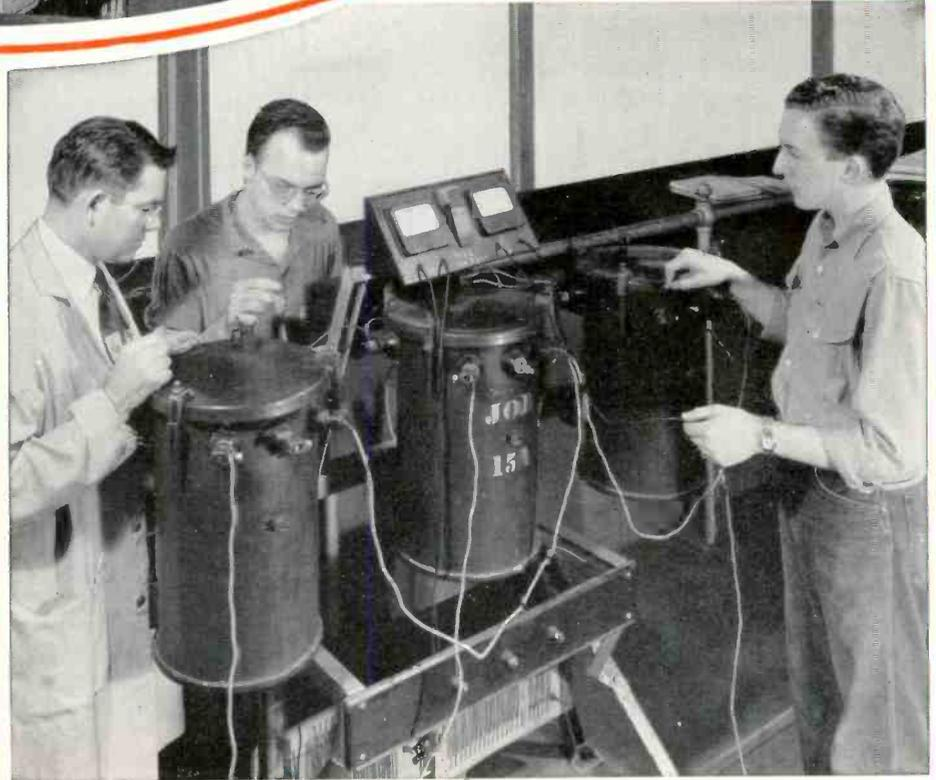
These students are connecting up a bank of power transformers for 3 phase operation, of a type commonly used in outdoor type substations.
