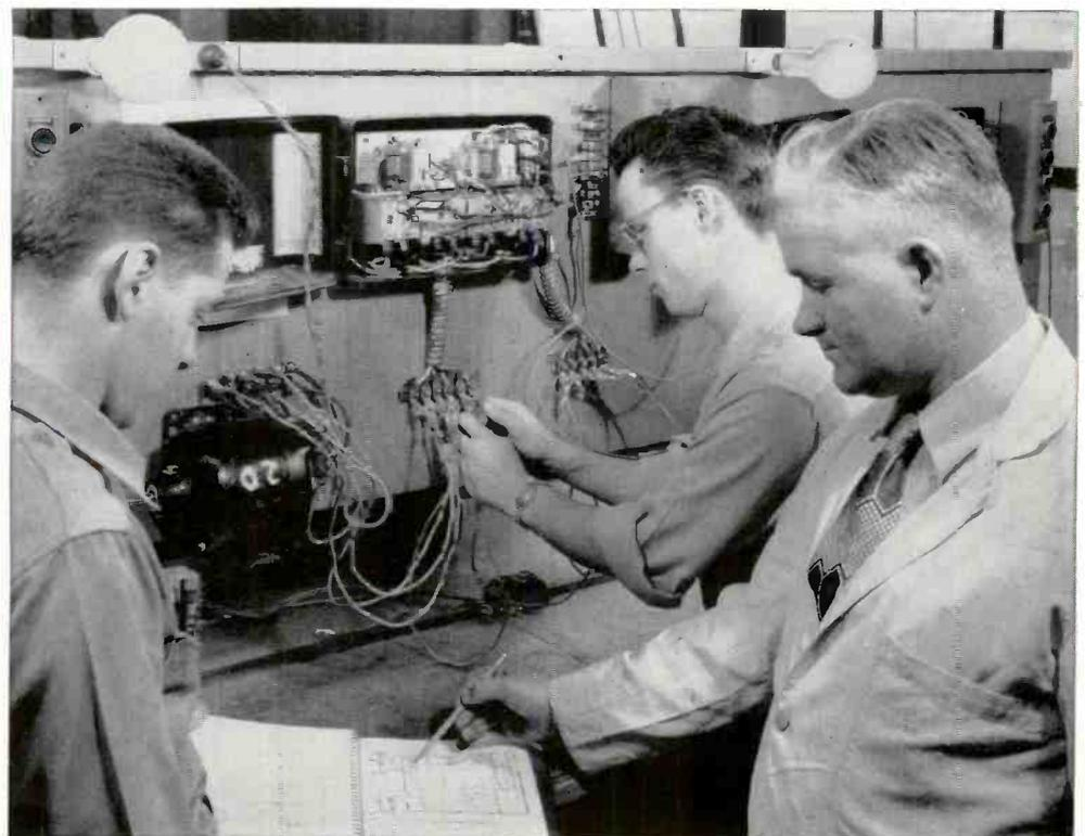
Here you see an Instructor working with a pair of students who are connecting up a reversing type starter for a compound motor, one of the important applications of D.C. equipment in industry.
