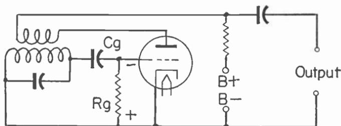
Fig. 3.—A tuned grid oscillator with inductive feedback.
