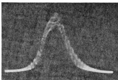
Fig. 31.—Effect of interfering station with frequency-modulated input.
