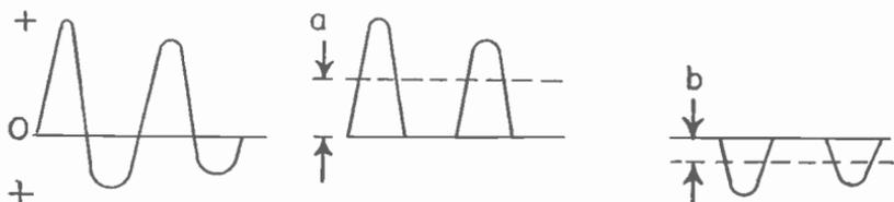
Fig. 13.—An unsymmetrical potential gives potentials depending on which side is rectified.
