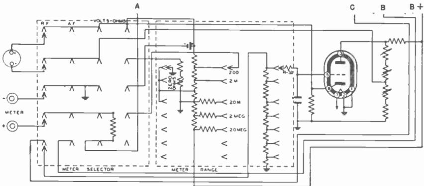
Fig. 7.—The electronic voltmeter used in the Audolyzer.
