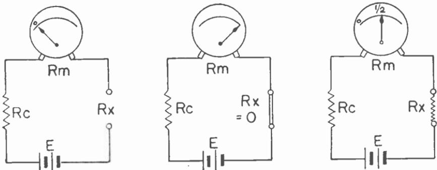
Fig. 4.—The principle of the series-resistance type of ohmmeter.
