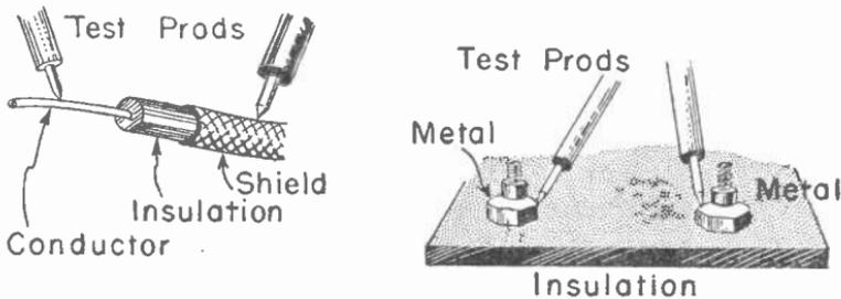
Fig. 4.—Checking the resistance of insulation.
