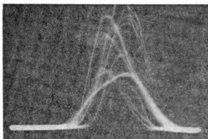
Fig. 30.—Effect of amplitude modulation with frequency-modulated input.
