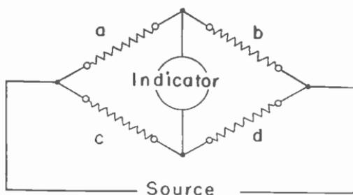
Fig. 6.—The fundamental bridge circuit.
