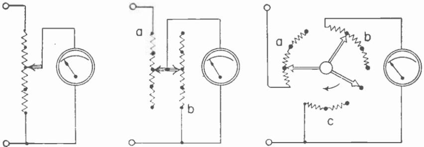
Fig. 10.—Constant impedance range-shifting circuits for output meters.
