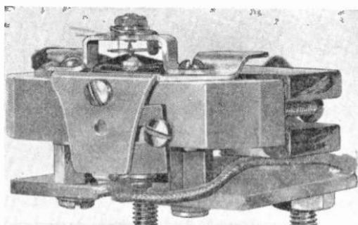
Fig. 17.—Principle of the magnetic shunt.
