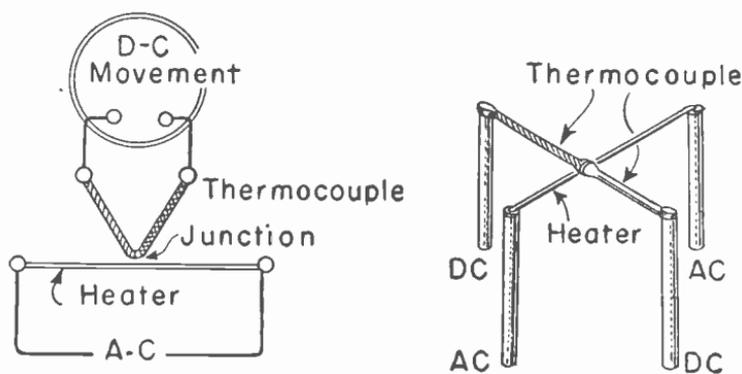
Fig. 20.—The principle of the thermocouple meter.
