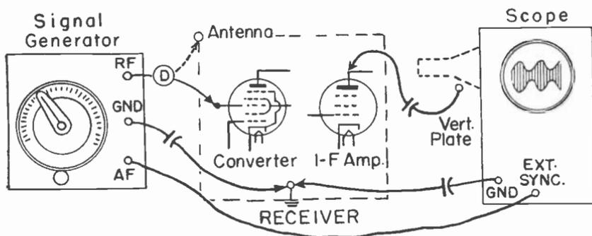
Fig. 12.—Connections for observation of r-f or i-f envelopes, either modulated or not modulated.
