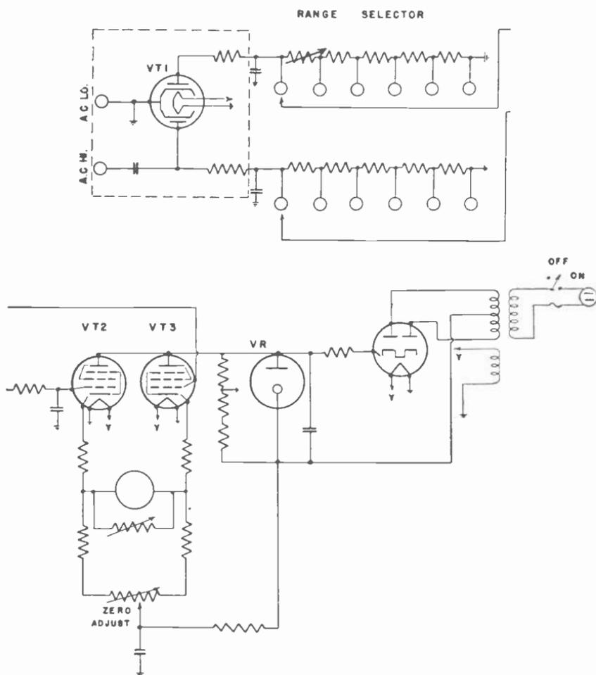
Fig. 18.—One section of the double diode is used to compensate for contact potential in the other section. Reiner electronic voltmeter circuit.
