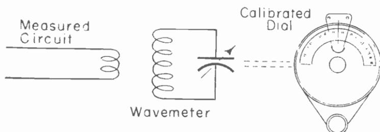
Fig. 13.—The principle of the wavemeter or absorption frequency meter.
