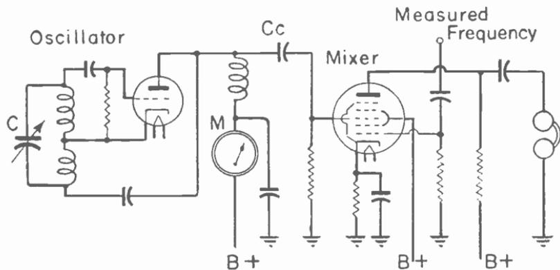
Fig. 18.—Principal parts of a heterodyne frequency meter circuit.
