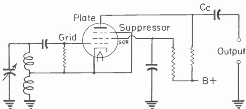
Fig. 10.—One type of electron coupled oscillator.
