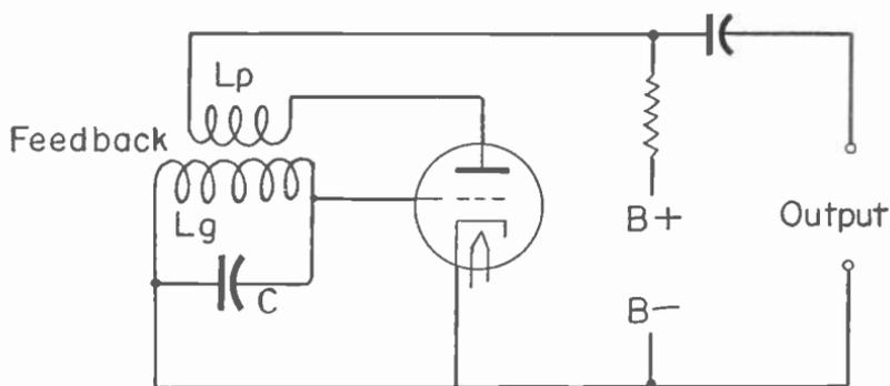
Fig. 2.—The elementary oscillator circuit.
