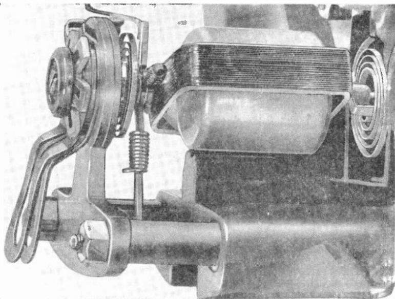
*Fig. 7.—A moving coil with its supports and hair springs at front and rear.*
