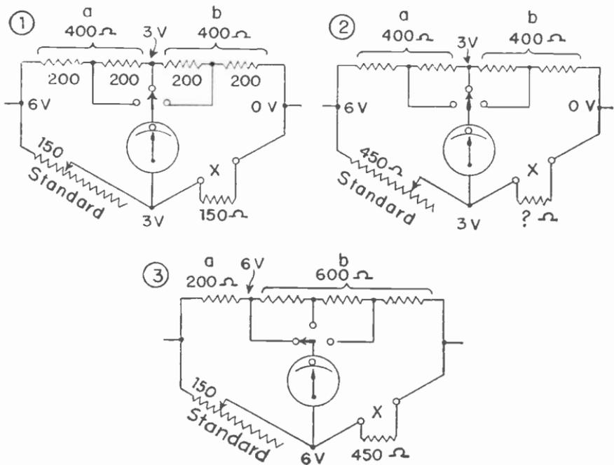
Fig. 5.—Ratio arms, standard arms, and unknown arms on a bridge circuit.
