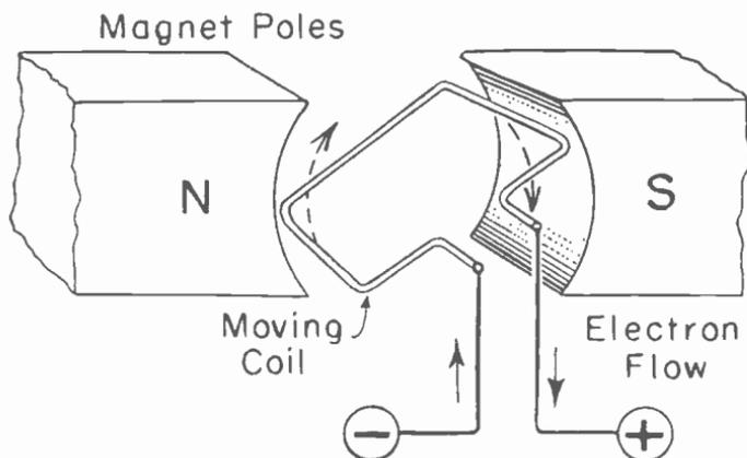
Fig. 5.—Why the coil rotates between the magnet poles.
