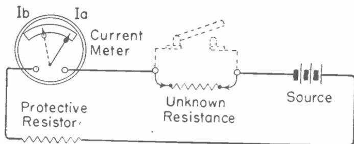
Fig. 2.—Measuring a resistance with a current meter.
