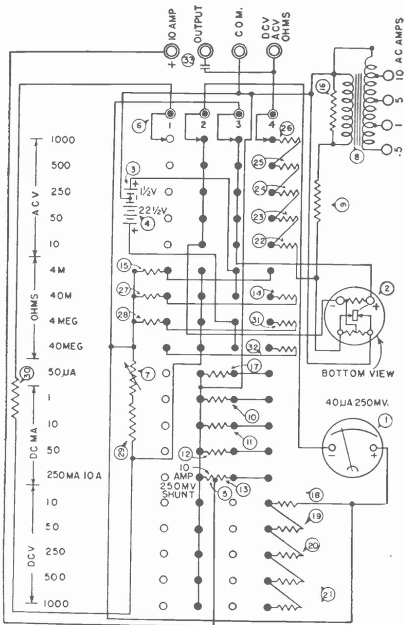
Fig. 17.—Internal connections and switching for a Triplet volt-ohm-millimeter.
