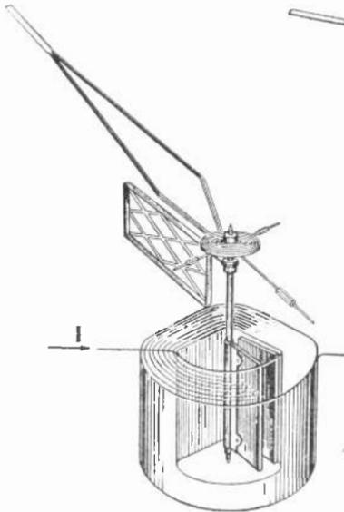
*Fig. 22.—The principle of the iron-vane movement of the repulsion type.
