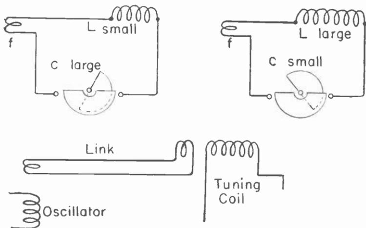
Fig. 6.—Inductance measurement by substitution.
