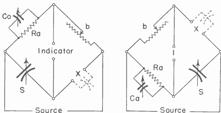
Fig. 14.—A Schering bridge for capacitance measurement.
