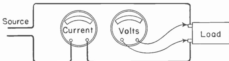
Fig. 12.—Connections for computing power used in a load.
