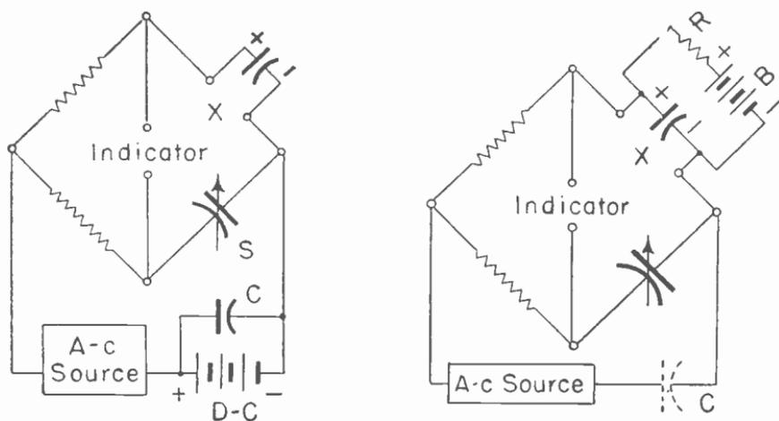
Fig. 15.—Testing electrolytic capacitors on capacitance bridges.
