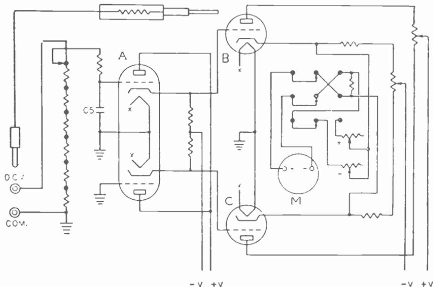
Fig. 19.—Cathode follower bridge circuit as arranged for direct potential measurements in a Triplett electronic voltmeter.
