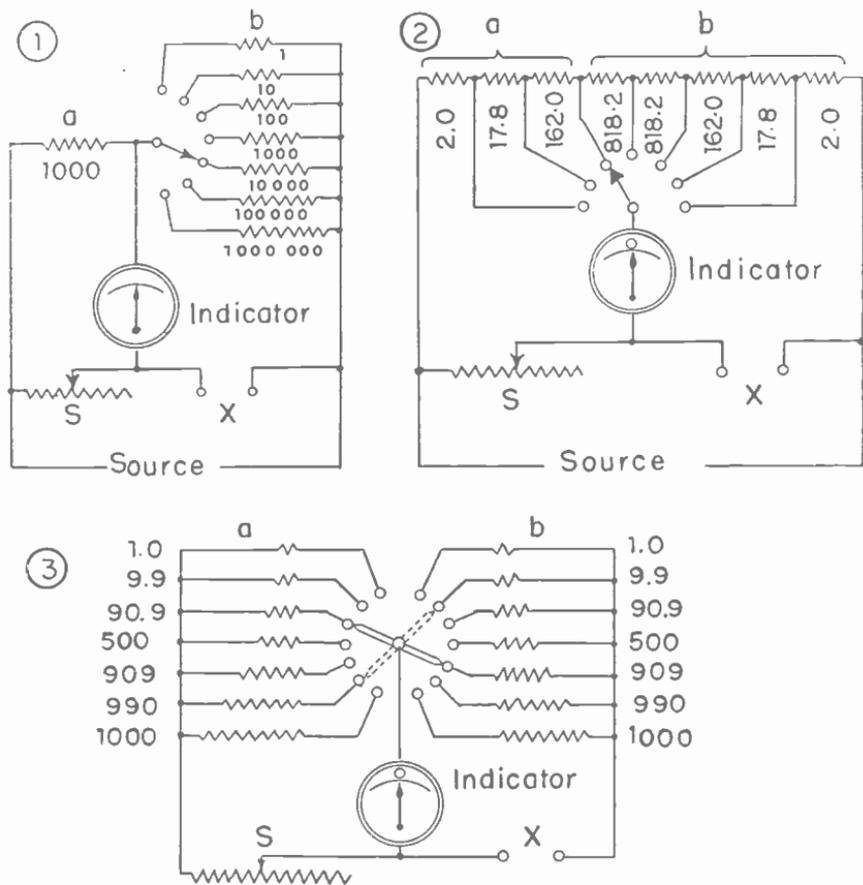
Fig. 7.—Connections and resistance values for ratio arms.
