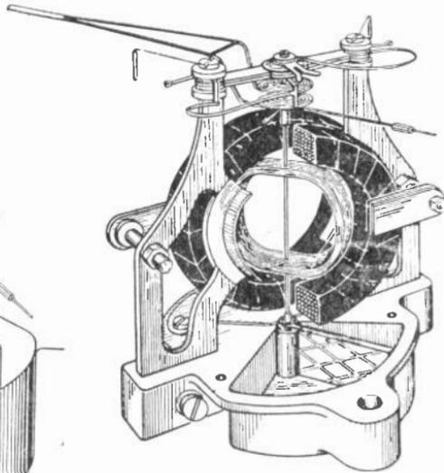
*Fig. 23.—The principle of the dynamometer instrument.
