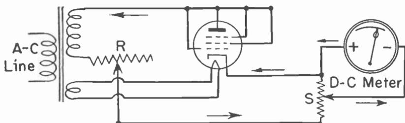
Fig. 4.—A circuit for measurement of cathode emission.
