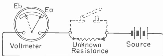
Fig. 1.—Measuring an unknown resistance with a voltmeter.
