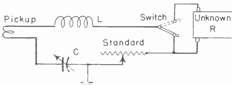
Fig. 11.—Measuring high-frequency resistance by resistance variation.
