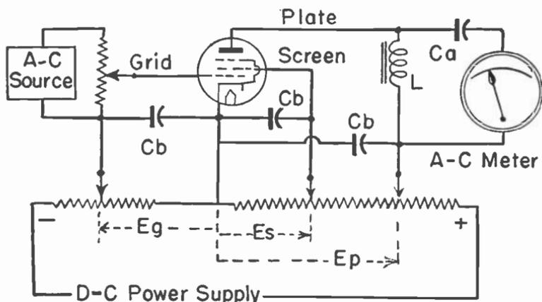
Fig. 3.—A circuit for measurement of mutual conductance.
