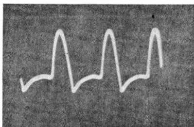
Fig. 6.—Trace inverted by reversing leads to vertical input.
