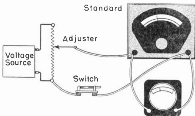
Fig. 11.—Connections for calibration of a voltmeter.
