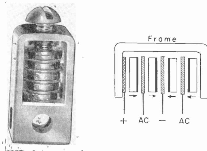
Fig. 18.—A full-wave instrument rectifier, and the arrangement of the discs.
