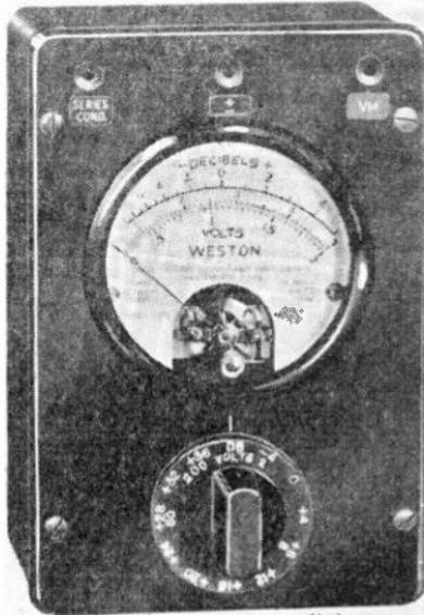
Fig. 13.—A Weston power level meter having 20,000 ohms constant impedance, and reading in volts and decibels.
