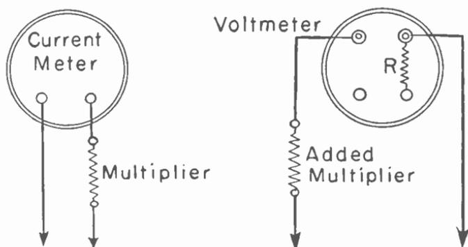
Fig. 13.—Connections of series multiplier resistors for voltmeters.
