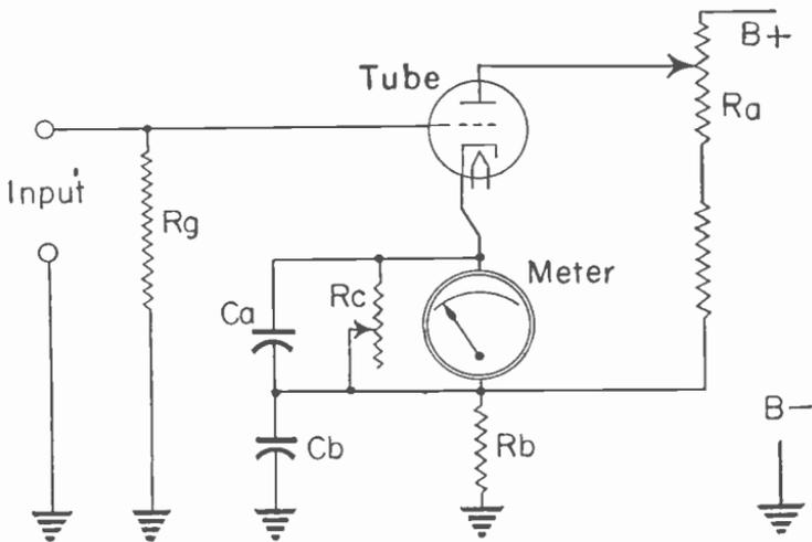
Fig. 6.—The principle of the cathode-bias electronic voltmeter.
