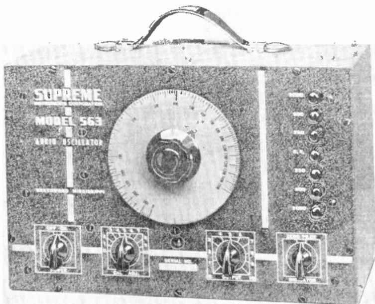
Fig. 19.—Panel controls of the Supreme audio-frequency generator.
