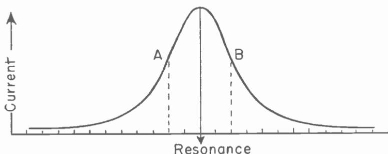
Fig. 5.—There is greater variation of current with frequency slightly off resonance than at resonance.
