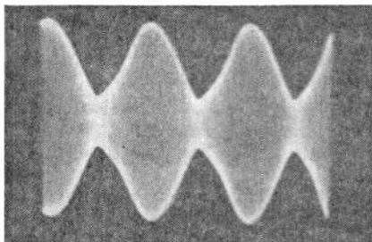
Fig. 13.—High-frequency wave modulated at audio frequency.
