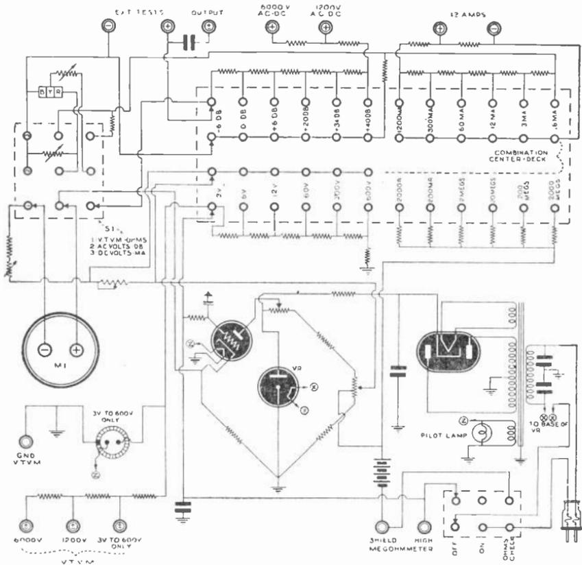
Fig. 9.—Schematic circuit diagram for a Precision Apparatus electronic voltmeter having the meter tube in a bridge circuit.
