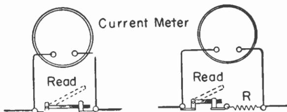
Fig. 4.—Protective devices for current meters.
