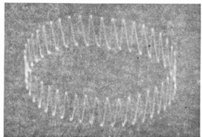
Fig. 21.—Frequency ratio of 43 to 1
