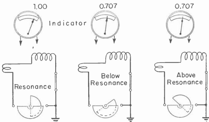
Fig. 12.—High-frequency resistance measured by reactance variation.
