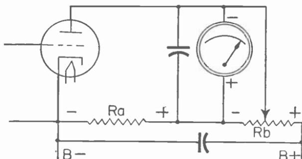
Fig. 4.—One method of bucking the plate current.
