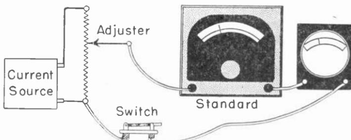
Fig. 10.—Connections for calibration of a current-indicating meter
