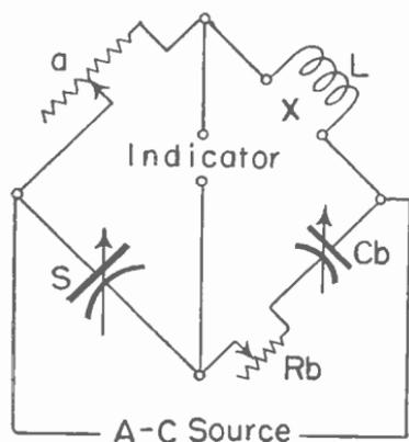
Fig. 18.—The Owen bridge for inductance measurement.
