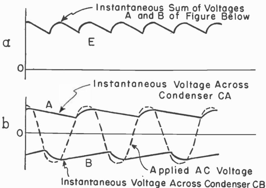
Fig. 21-18.—Potentials in a symmetrical voltage doubler.
