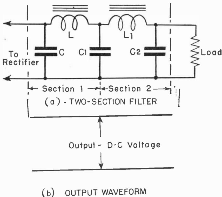
Fig. 21-11.—Two section filter and out-put waveform: (a) Two-section filter
