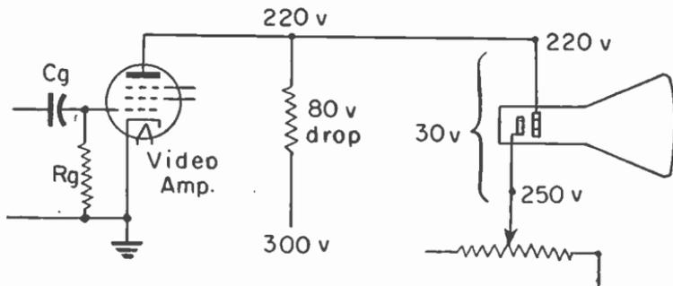
Fig. 15.—D-c reinsertion with automatic (grid rectification) bias on the video amplifier tube.
