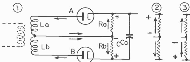
Fig. 8.—The direct-current circuits for the discriminator diodes.
