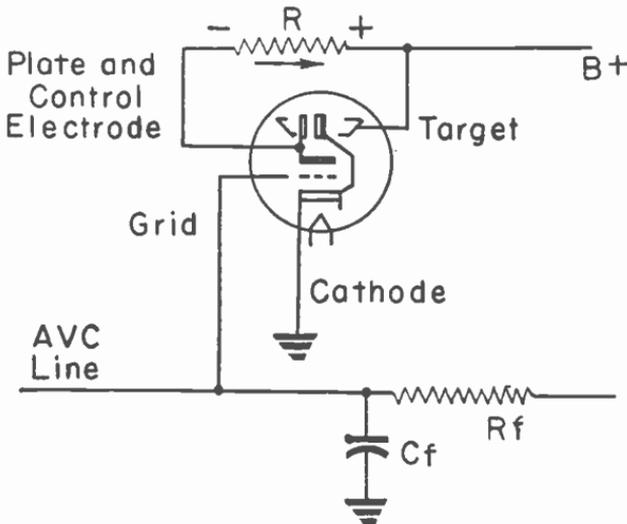
Fig. 17.—Circuit connections for an electron ray tuning indicator.
