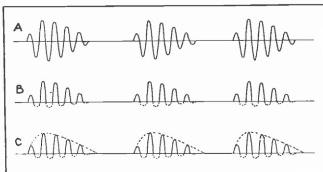
Fig. 22-25.—The curve at "A" represents the alternating current induced by damped wave trains striking the aerial. At "B" is shown the curve for this energy after it has been rectified into pulsating D.C. by the crystal. At "C" the large dotted curves illustrate how each group of pulsations supply line current impulse to the headphones.
