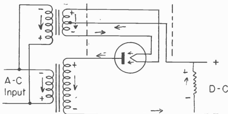
Fig. 21-4.—A rectifier circuit showing use of transformer to get higher output than line voltage.
