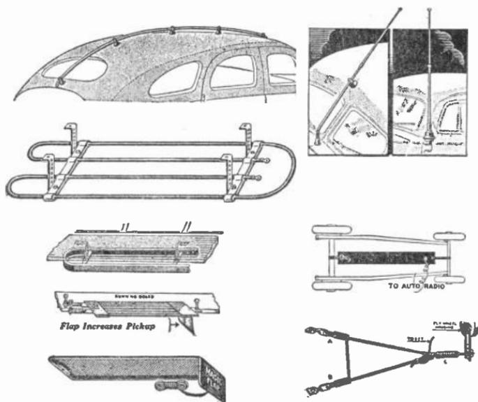
Fig. 2.—Antennas for installation on the top, under the running board, and on the chassis of the automobile.
