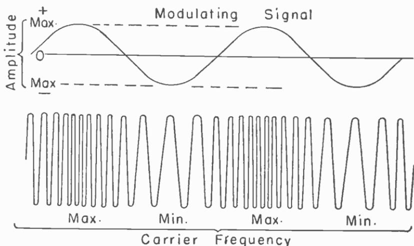
Fig. 3.—Frequency modulation of a carrier wave.
