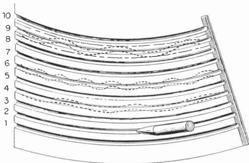
Fig. 16.—Groove sections and undulations on a phonograph record.
