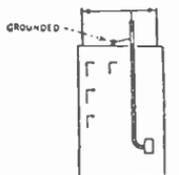
**Shielded Lead-In**—Reduces noise pickup by downlead where this wire must pass through electrically disturbed areas. Good reception on broadcast band but not recommended for shortwaves. In common with other noise-reducing types, must have antenna proper mounted out of noisy area for maximum benefit.
