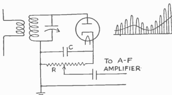
Fig. 22-32.—Using a diode tube for a detector.
