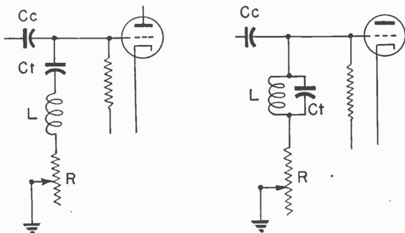
Fig. 22.—Tone controls employing tuned resonant circuits.
