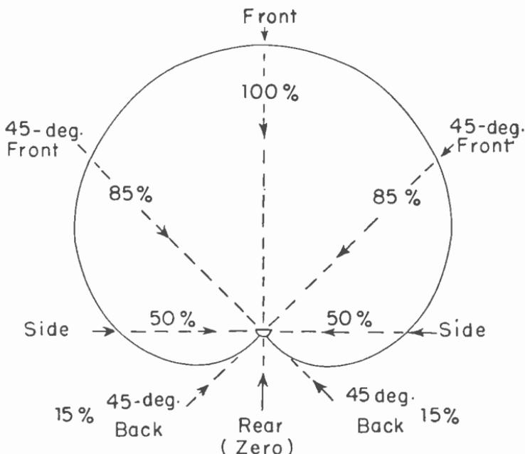
Fig. 14.—The cardioid pattern of microphone response.
