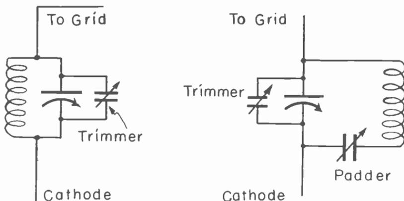
Fig. 11.—Connections for trimmer and padder capacitors.
