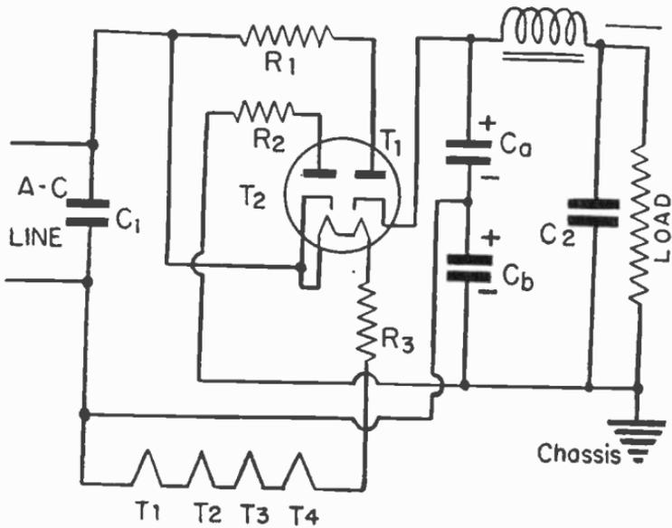
b. SIMPLIFIED DIAGRAM OF DOUBLER CIRCUIT
