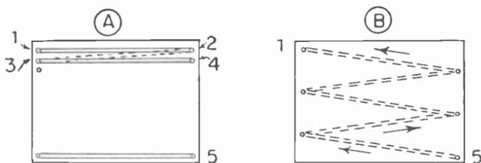
Fig. 6.—How an area is scanned by deflecting the beam sideways and downward.
