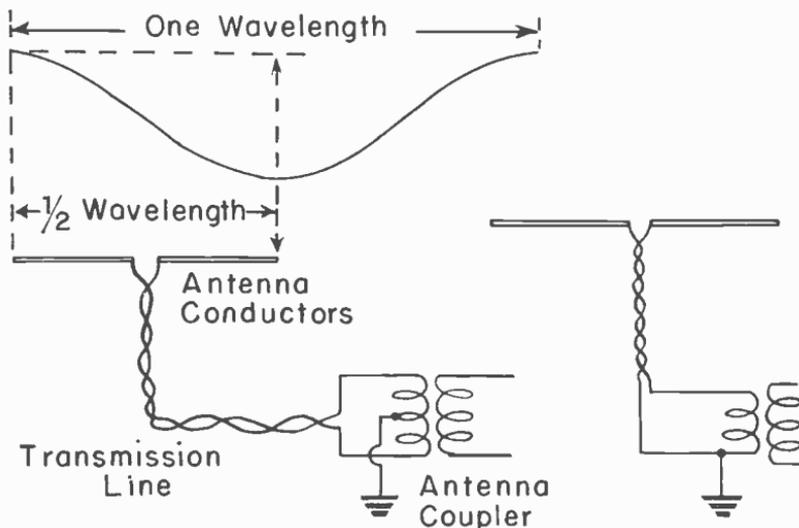
Fig. 14.—The doublet or half-wave dipole antenna.
