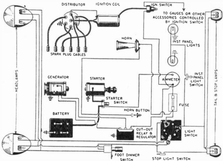
*Fig. 15.—The principal parts and their connections in a complete electrical system for an automobile.*
