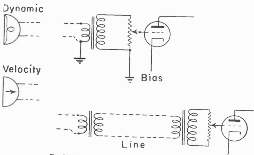
Fig. 13.—Connections from low-impedance microphones.
