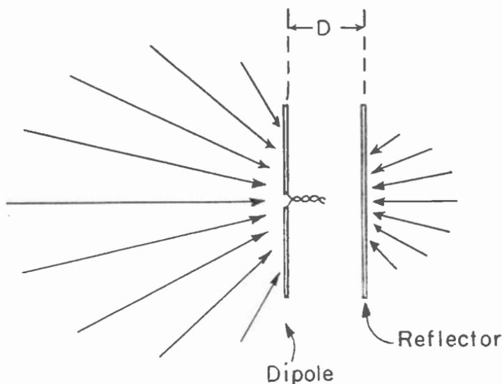
Fig. 16.—A reflector used with a dipole antenna.
