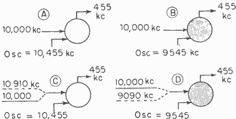
Fig. 12.—Relations between image frequencies and oscillator settings.
