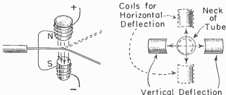
Fig. 8.—The principle of magnetic or electromagnetic deflection.
