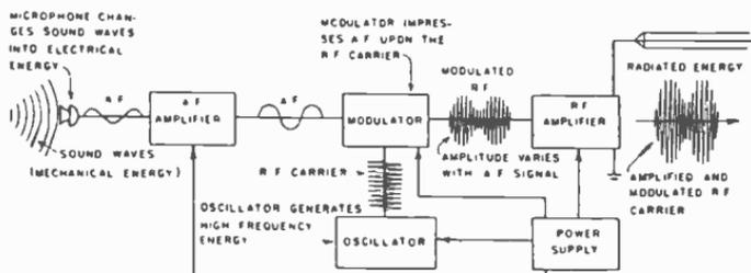
Fig. 22-35.—A radio transmitter from microphone to aerial.
