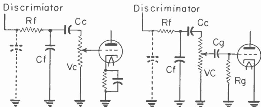
Fig. 19.—Circuits used between discriminator and first a-f amplifier.
