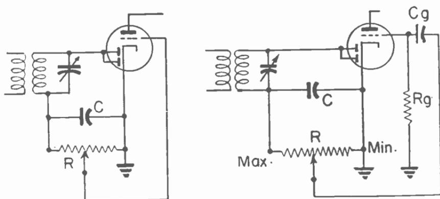
Fig. 5.—Volume controls in diode detector circuits.
