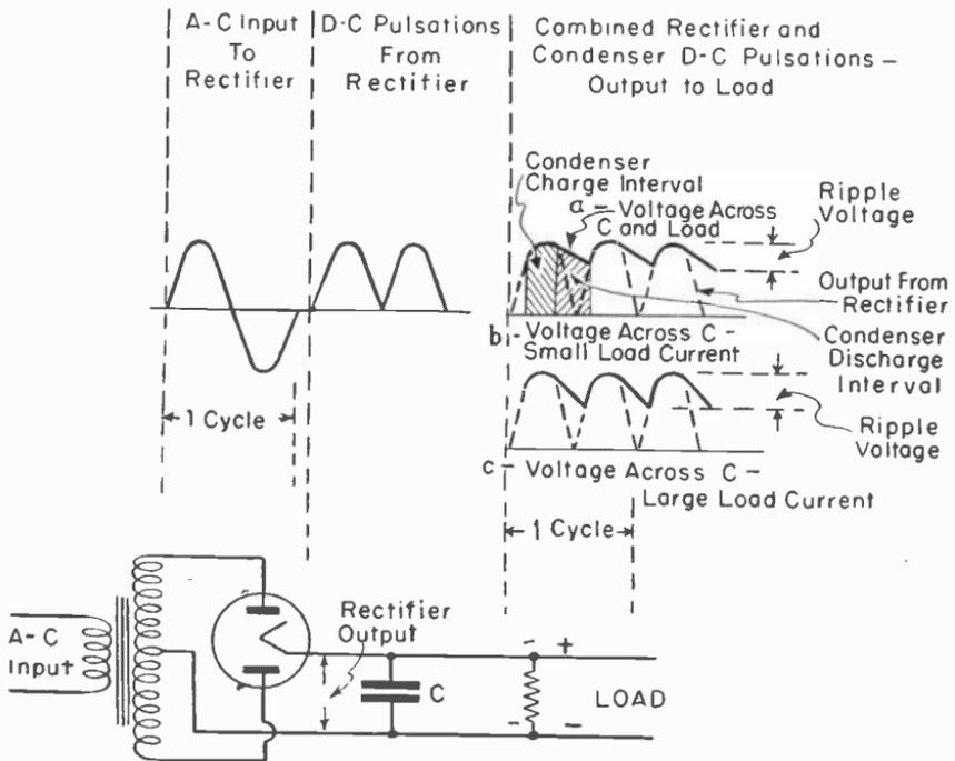
Fig. 21-7.—Condenser input filter and output waveforms with small and large loads.
