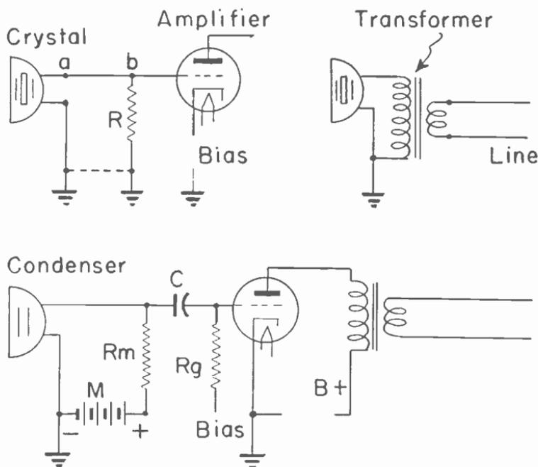
Fig. 12.—Output connections for high-impedance microphones.
