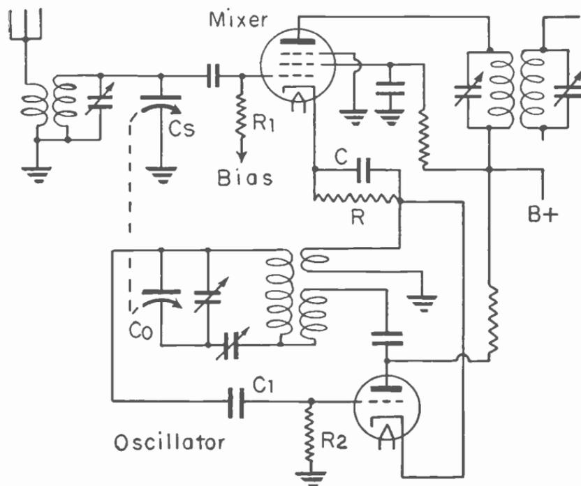
Fig. 14.—Circuits for separate mixer and oscillator tubes.
