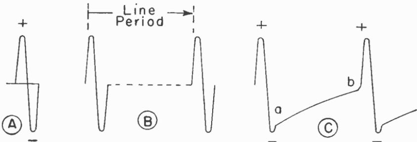
Fig. 21.—The output from a deflection oscillator of the blocking type.
