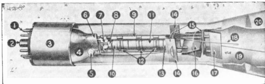
Fig. 4.—The electron gun in one type of DuMont cathode-ray tube. 1, 2 and 3; base collar, base pins, and locating key. 4, 5 and 6; glass stem, getter for gas removal, and glass press. 7 and 8; heater and cathode. 9; supports. 10; control grid. 11; focusing anode. 12; supporting collars. 13; accelerating anode. 14 and 15; supports. 16 and 17; plates for deflecting electron beam. 18 and 19; static shield and connection. 20; glass envelope of tube.
