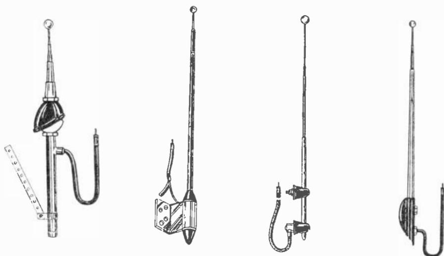
Fig. 1.—Telescoping types of auto-radio antennas. (Spirling)
