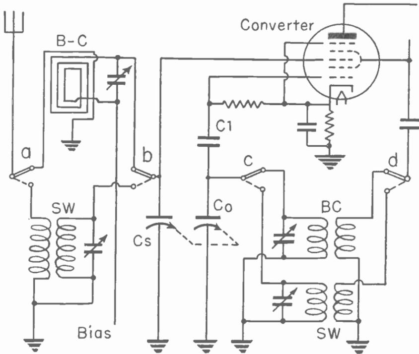
Fig. 12.—Band switching arrangements for a two-band receiver.
