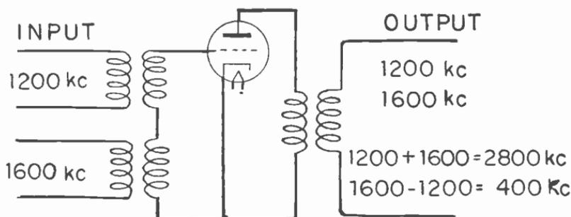
Fig. 2.—Output frequencies produced from two input frequencies.
