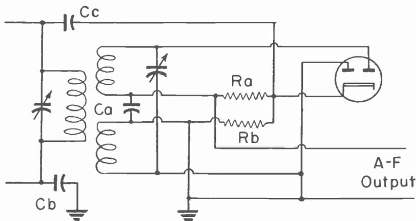
Fig. 17.—A discriminator circuit employing a double-diode tube with a single cathode.
