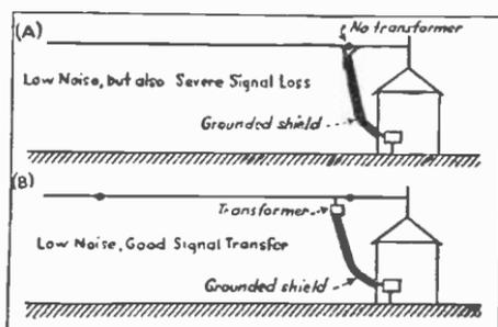
Fig. 22-10-A-B.—Shielded lead ins—poor (A) good (B).
