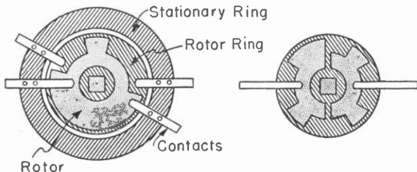
Fig. 3.—One unit of a rotary selector switch.
