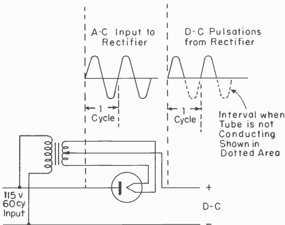
Fig. 21-3.—A half-wave rectifier circuit and its waveforms.
