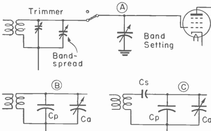
Fig. 6.—Arrangements of tuning capacitors for band spreading.
