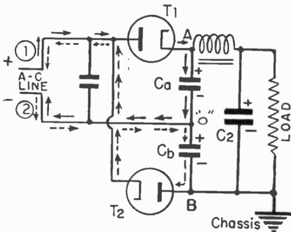
SOLID LINE  $\longrightarrow$  Indicates Direction of Charging Current Flow When (1) is Positive
