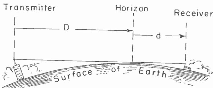
Fig. 5.—Transmission distances and reception distances extend practically only to the visible horizon.
