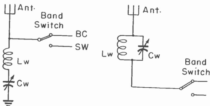
Fig. 11.—Wave traps in the antenna circuit.
