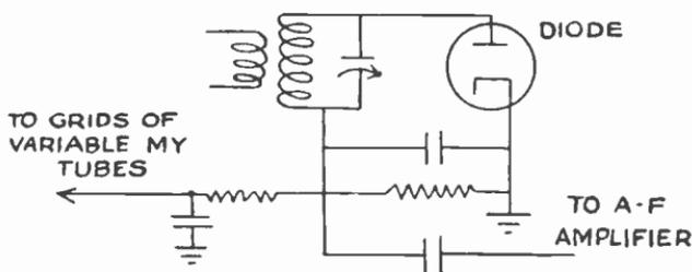
Fig. 22-33.—Automatic volume control voltage for variable- $\mu$  tubes may be taken from the circuit of the diode detector.
