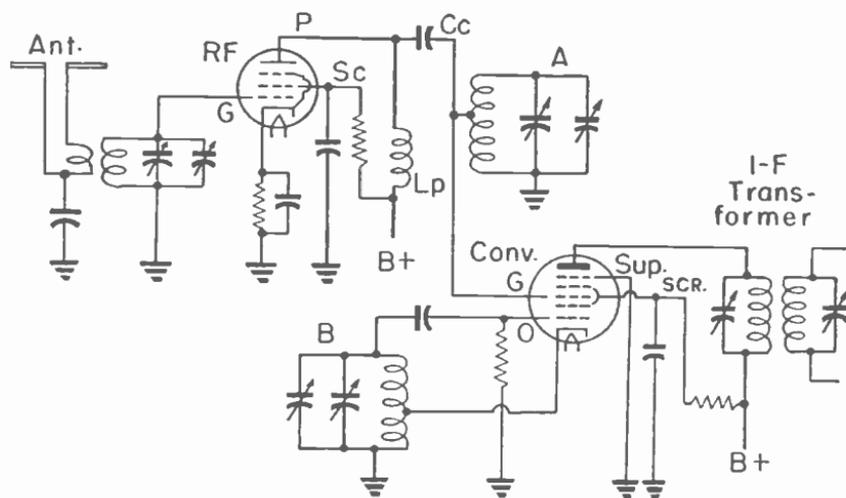
Fig. 13.—Circuits between a dipole antenna and the first i-f transformer.
