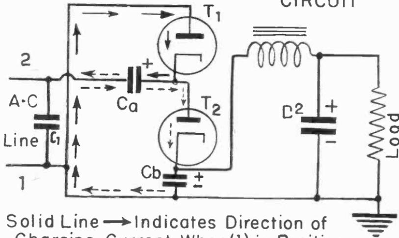
Solid Line  $\rightarrow$  Indicates Direction of Charging Current When (1) is Positive
