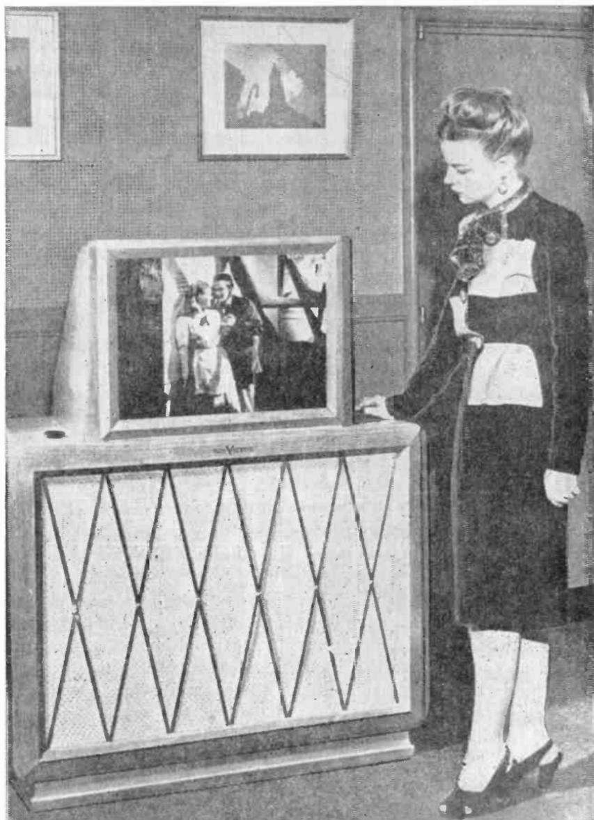
*Fig. 3.—An RCA Victor television receiver with which images from the picture tube are projected through a lens and mirror system to form a reproduction 18 inches high and 24 inches wide.*
