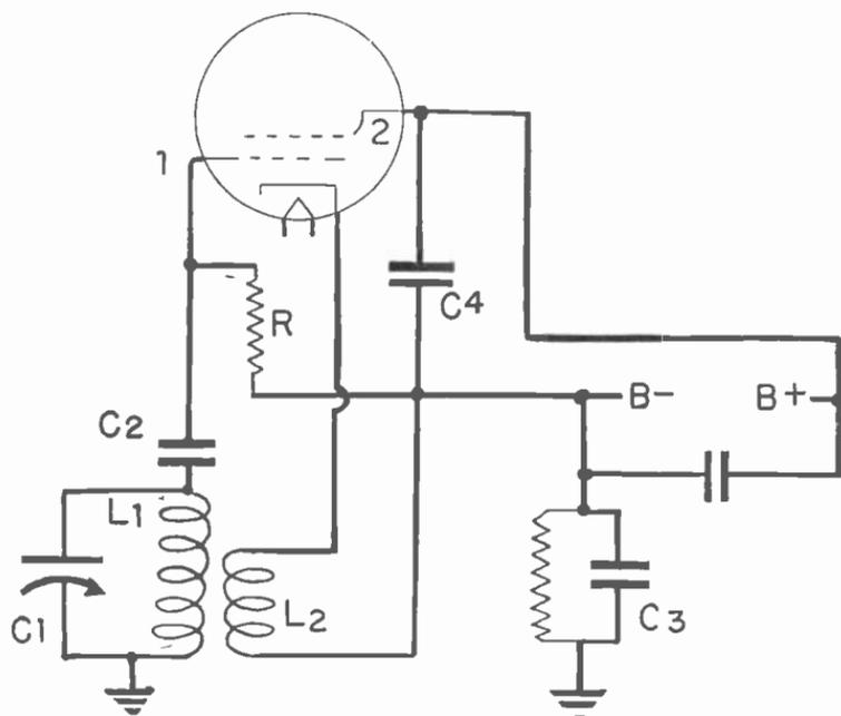
Fig. 6.—The oscillator circuit of the converter.
