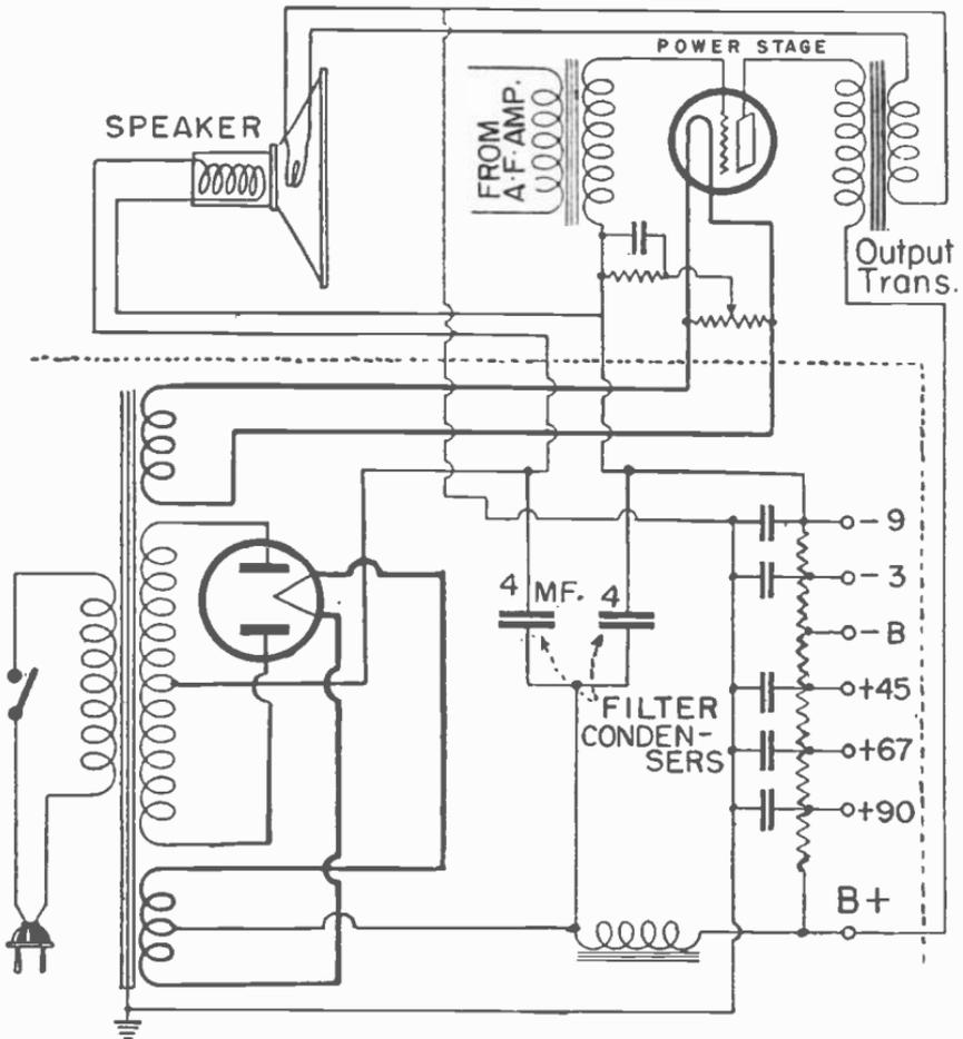
Fig. 23-13.—Diagram of a power supply unit, dynamic speaker, and the last stage of power amplification of a receiver. Note the field coil at the speaker is connected in series with the negative lead of the D.C. plate supply and serves as one of the filter chokes. Also note the connection of the cone coil, or voice coil to the secondary of the output or speaker coupling transformer.
