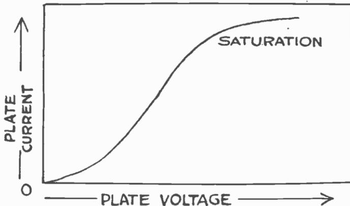
Fig. 22-27.—Plate current increases from zero to saturation as plate voltage is increased.
