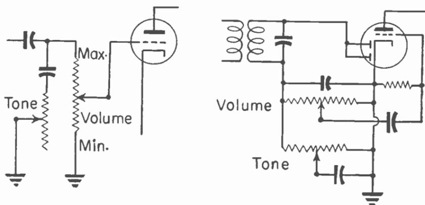
Fig. 20.—Tone controls in the same circuits with volume controls.
