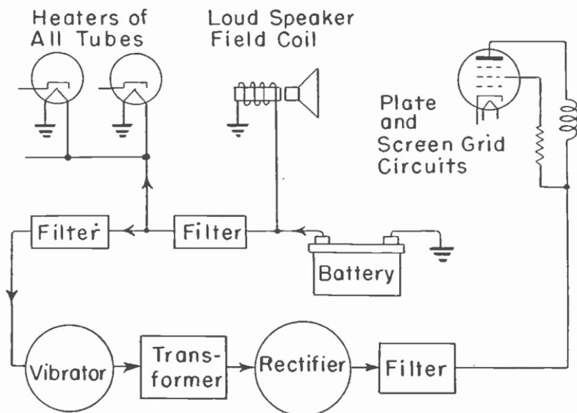
Fig. 7.—Principal units in the power supply system.
