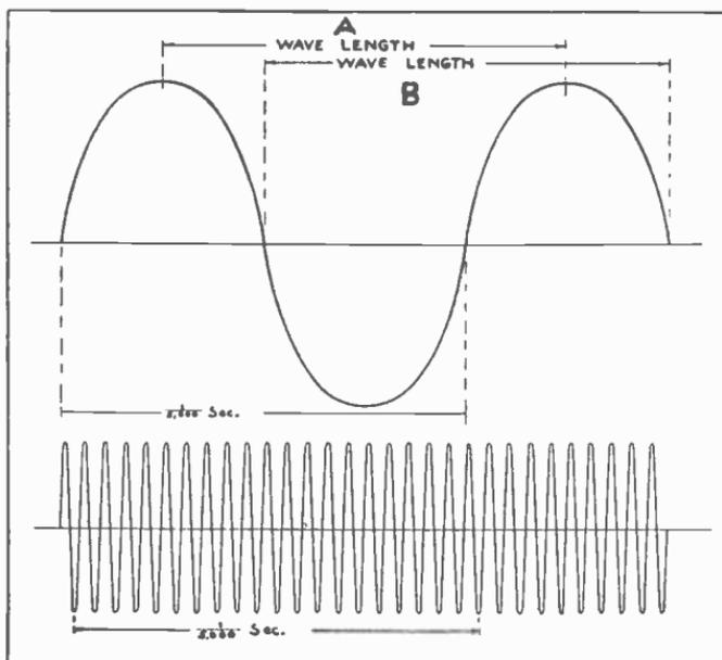
Fig. 22-2.—The above two sets of curves illustrate the difference between the frequency of sound waves and radio waves. The contrast between ordinary 60 cycle alternating current and the radio waves would be still greater.
