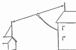
**Simple Doublet**—Reduces noise pickup by downlead where it must pass through noisy areas. Good reception on shortwave band and satisfactory for broadcast reception. Especially efficient at certain frequencies, which may be those most often desired.
