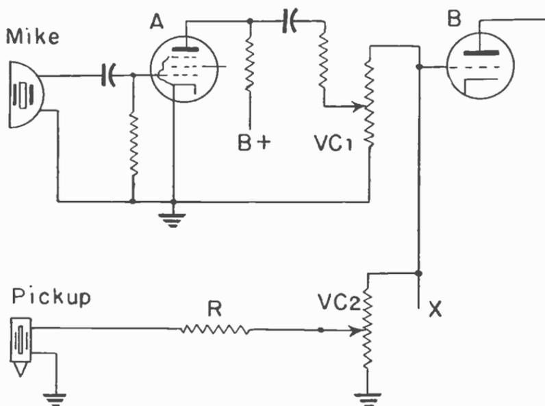
Fig. 20.—An additional amplifying stage for microphone input.
