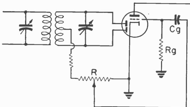
Fig. 8.—Volume control on a full-wave diode detector.
