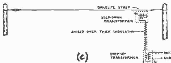
Fig. 22-10-C.—Wiring diagram of lead in.
