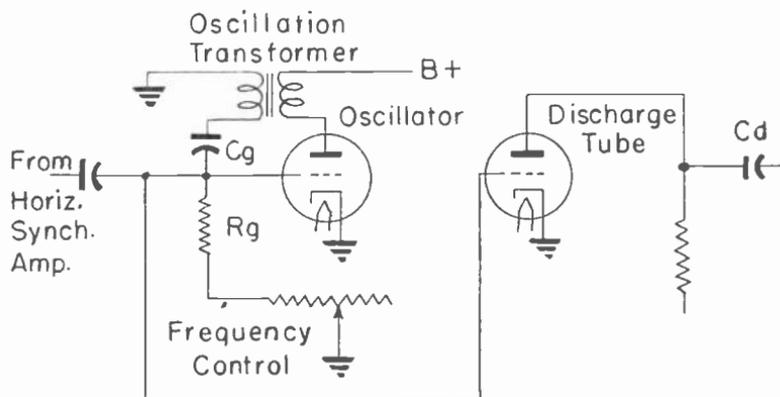
Fig. 20.—A horizontal synch generator including a deflection oscillator and a discharge tube.
