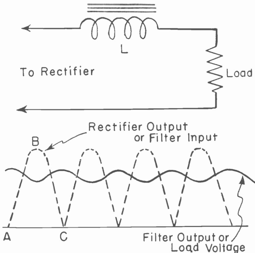
Fig. 21-12.—Choke filter; input and output wavetforms.
