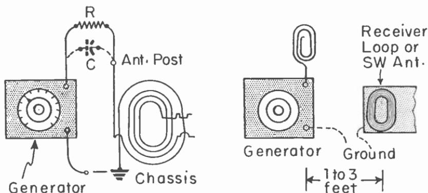
Fig. 13.—Signal generator connections for short-wave alignment.
