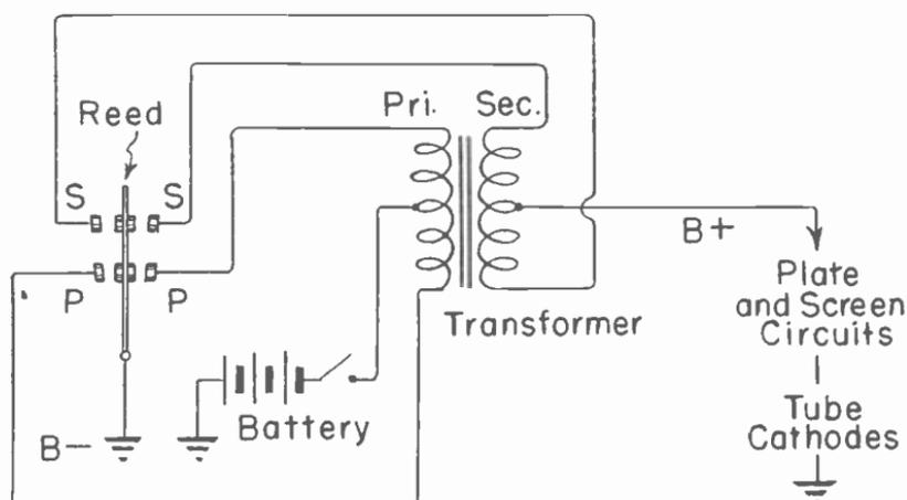
Fig. 13.—Circuit connections for a synchronous vibrator.
