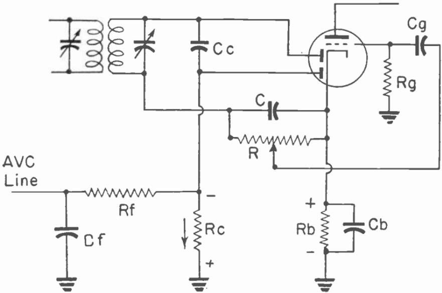
Fig. 13.—A circuit for delayed automatic volume control.
