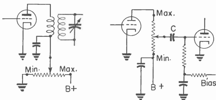
Fig. 3.—Volume controls in amplifier plate circuits.
