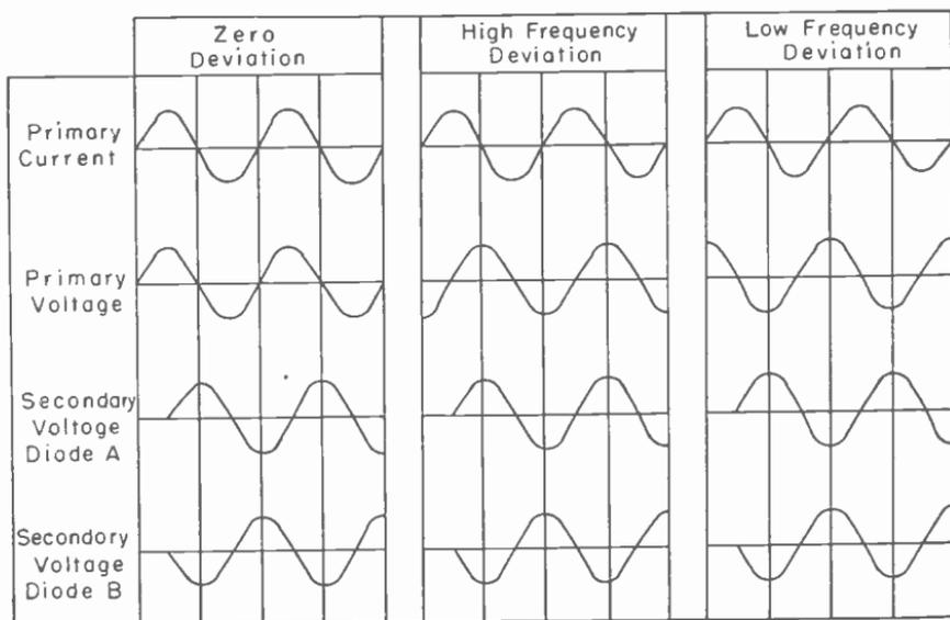
Fig. 11.—The phase relations at the same instants of time in the primary and secondary windings of the transformer, for three degrees of deviation.
