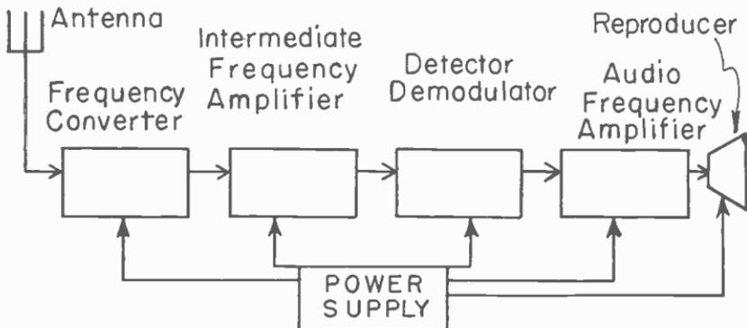
Fig. 1.—Principal parts of a superheterodyne receiver.
