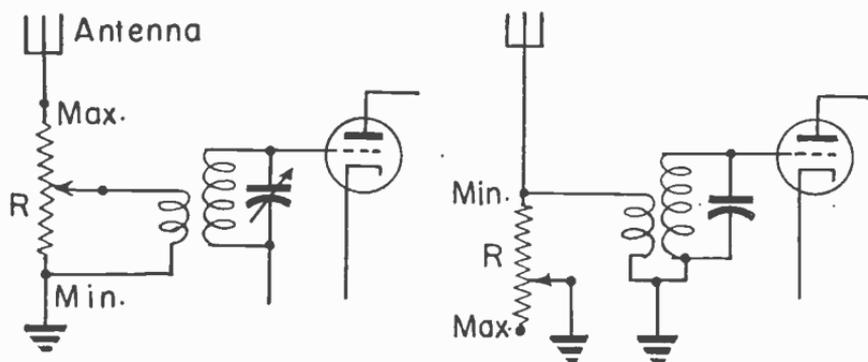
Fig. 1.—Volume controls in the antenna circuit.
