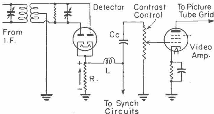
Fig. 9.—A full-wave diode detector circuit.
