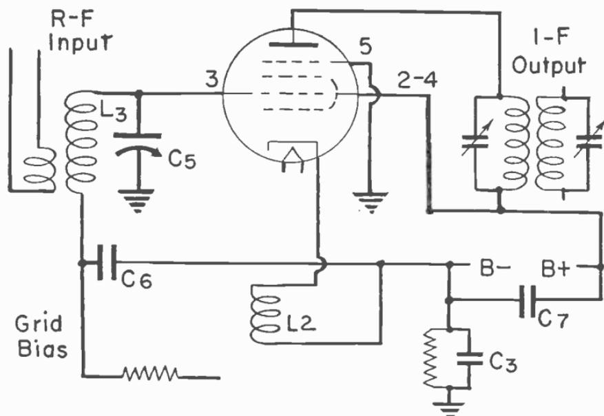
Fig. 7.—The mixer circuit of the converter.
