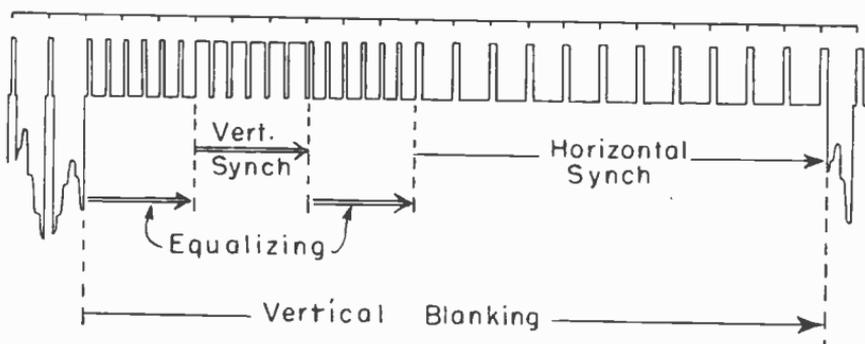
Fig. 16.—Synchronizing pulses which occur in the television signal during one period of vertical blanking.
