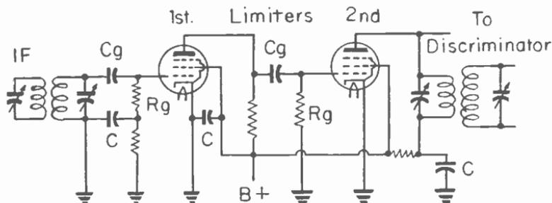
Fig. 6.—Circuits for two limiter stages in cascade.
