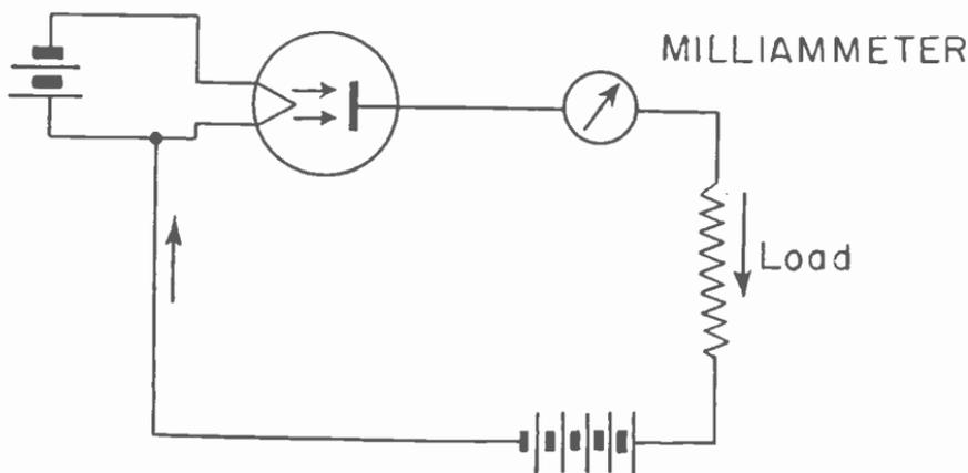
Fig. 21-1.—A diode as a rectifier.
