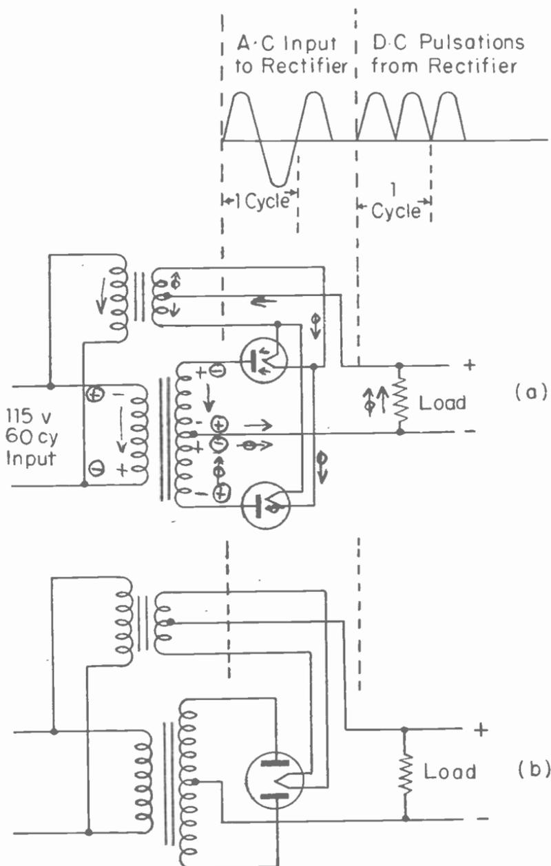
Fig. 21-5.—A full-wave rectifier and its waveforms.
