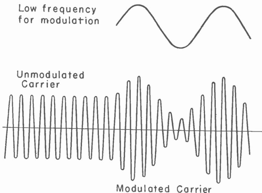
Fig. 2.—Amplitude modulation of a carrier wave.
