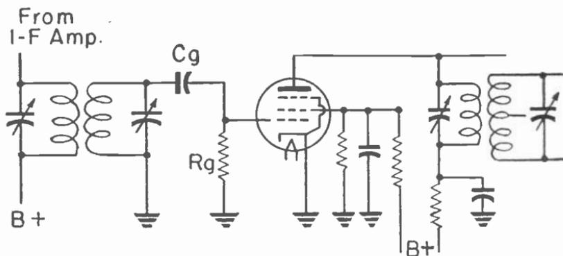
Fig. 1.—The circuit for a limiter stage.
