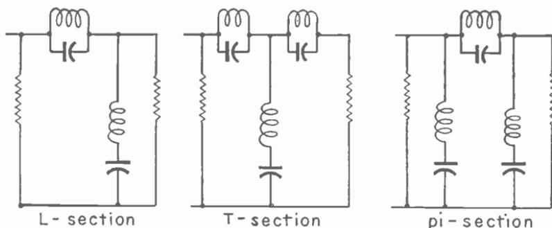
Fig. 28.—Basic stop filters of three different section types.
