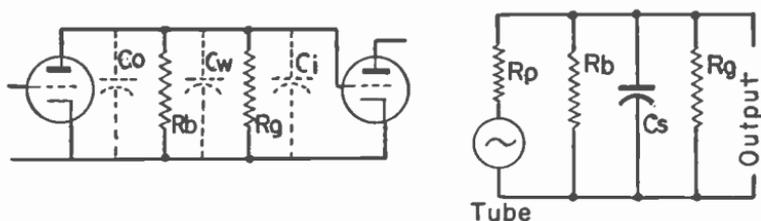
Fig. 9.—Capacitances which affect the gain at high frequencies.
