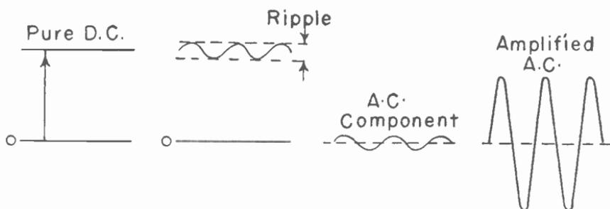
Fig. 13.—Ripple voltage or hum voltage.
