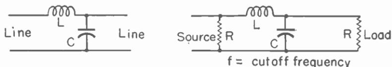
Fig. 22.—A low-pass filter having a single L-section.
