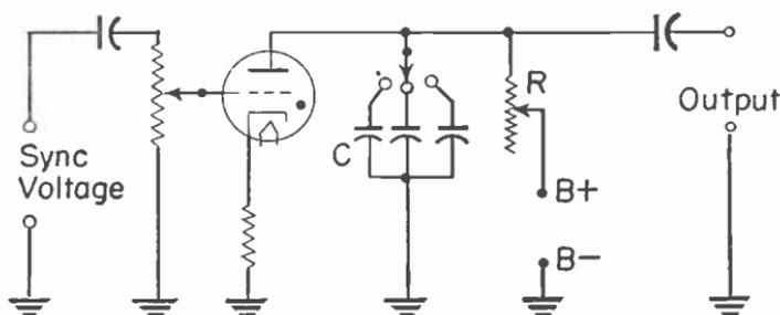
Fig. 16.—The circuit for a gas triode oscillator.
