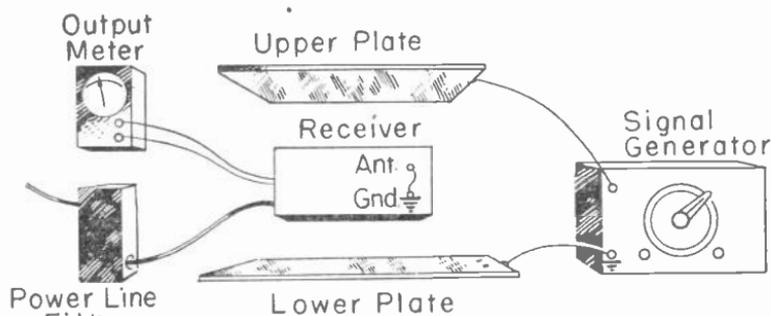
Fig. 11.—Connections for measuring signal pickup in an r-f field.
