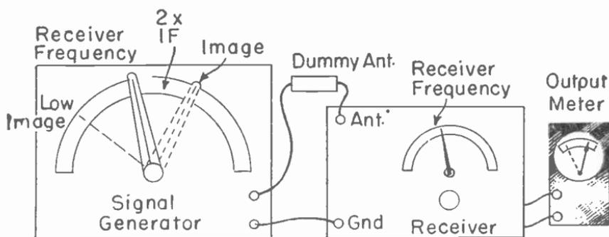
Fig. 10.—Testing a receiver for image frequency response.
