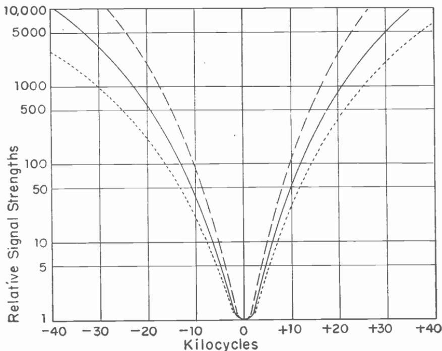
Fig. 4.—Selectivity curves for frequencies near the top, center, and bottom of a band.
