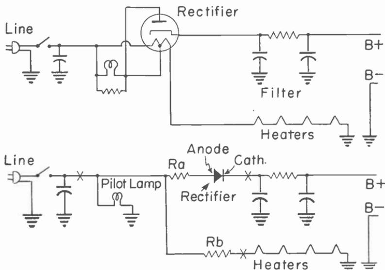
Fig. 4.—D-c power supply with vacuum tube rectifier (top) and with selenium rectifier (bottom).
