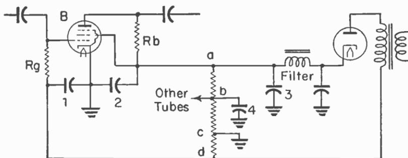
Fig. 3.—Decoupling when there is a voltage divider in the power supply.
