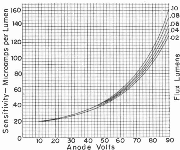
Fig. 14.—How sensitivity of a gas phototube changes with variations of anode voltage and luminous flux.
