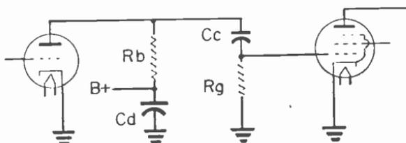
Fig. 5.—The coupling capacitor and grid resistor are in series.
