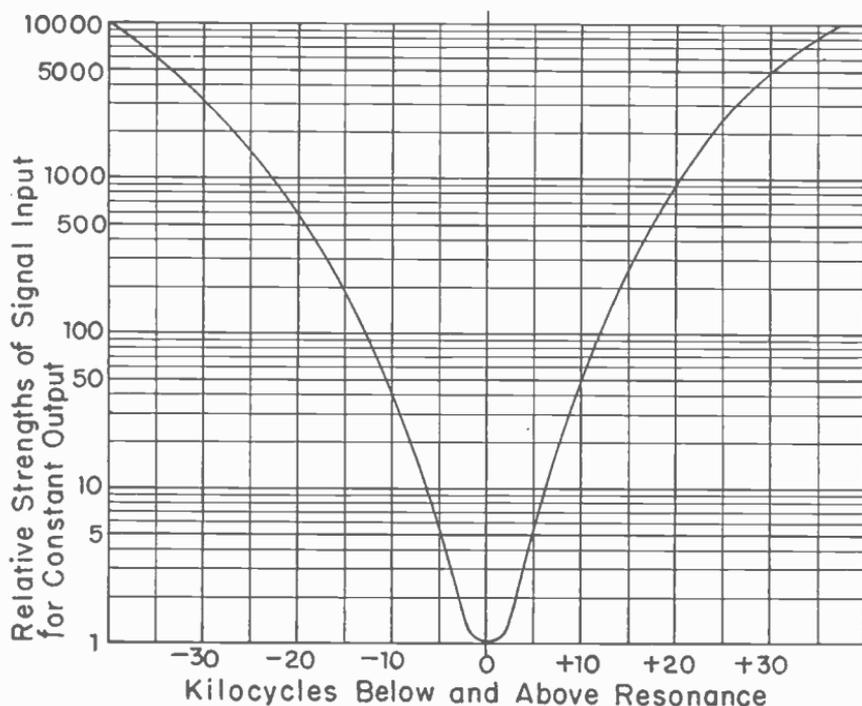
Fig. 2.—Selectivity curve for a typical small receiver.
