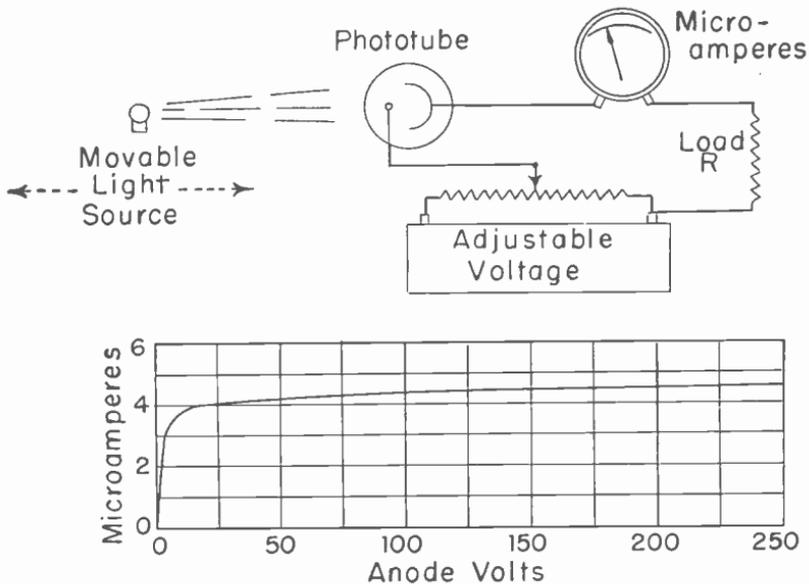
Fig. 10.—Current in a vacuum phototube at various anode voltages.
