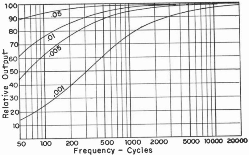
Fig. 7.—Effect of coupling capacitance on low-frequency gain.
