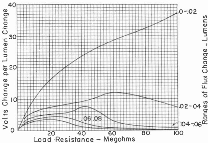
Fig. 21.—Changes of load potential, in volts per lumen of flux change, with a gas phototube.
