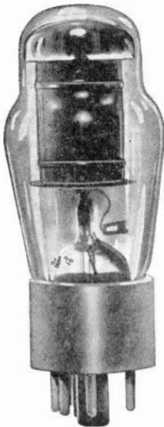
Fig. 4.—One type of voltage regulator tube.
