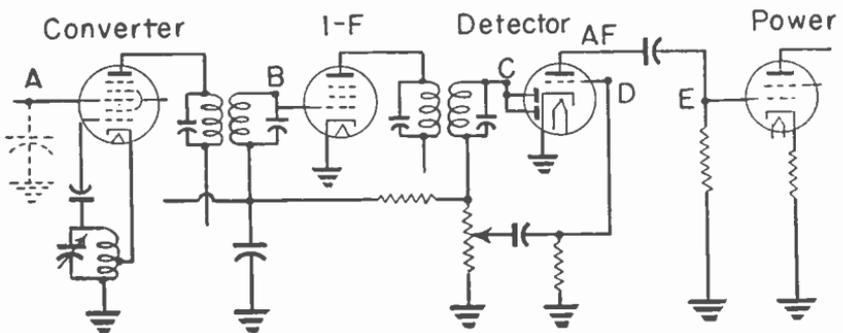
Fig. 16.—Points for grounding stage inputs in locating causes for hum.
