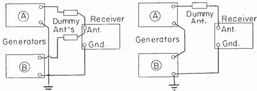
Fig. 6.—Two signal generators in parallel (left) and in series (right).
