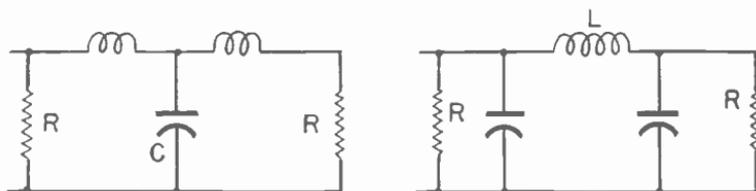
Fig. 24.—Low-pass filters of T-section (left) and pi-section (right).
