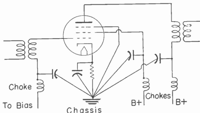
Fig. 7.—Bypassing and filtering for high frequencies.
