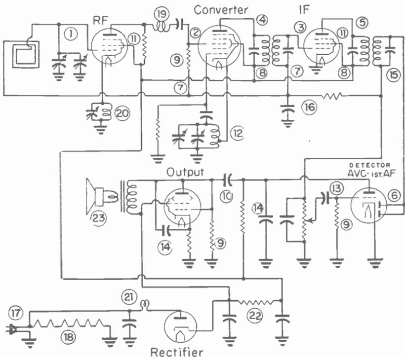
Fig. 13.—Points at which care should be used in dressing wires and parts.
