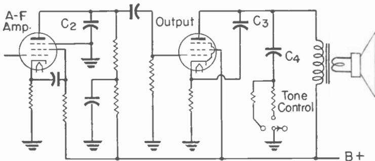
Fig. 11.—High-frequency plate bypasses and a tone control.
