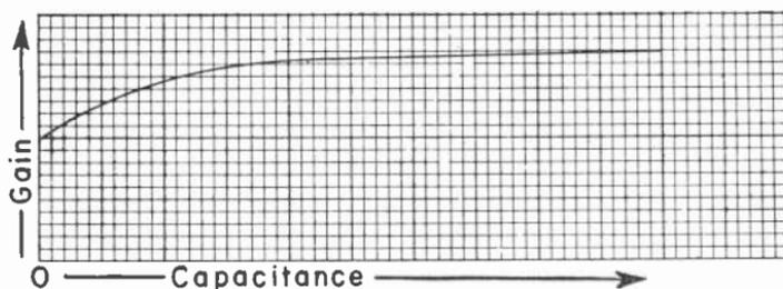
Fig. 14.—Greater bypass capacitance allows increased gain.
