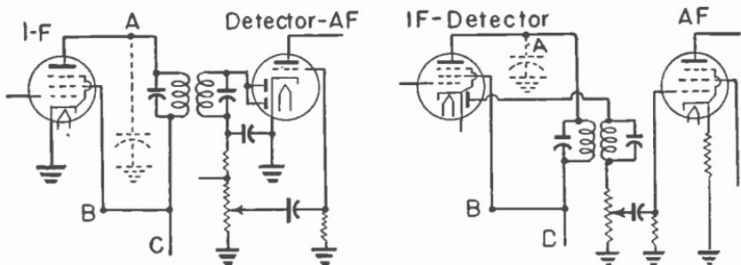
Fig. 18.—Points at which the i-f input to a detector may be cut off.
