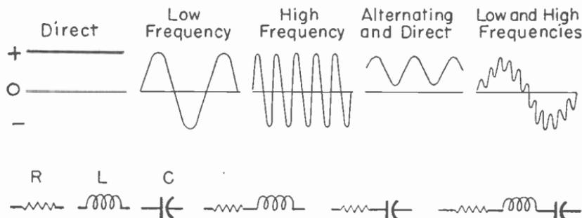
Fig. 4.—Waveforms of currents and potentials, and the elements in which they act.
