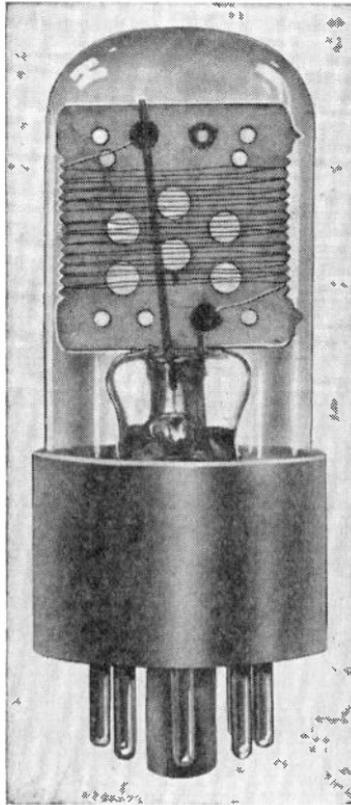
Fig. 23.—A ballast tube mounted on an octal base.
