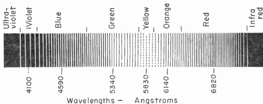
Fig. 4.—Wavelengths of light in the visible spectrum.
