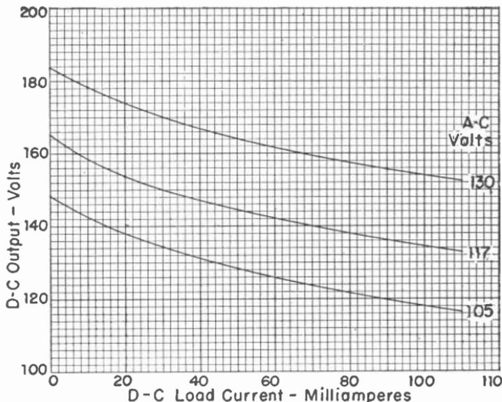
Fig. 3.—Voltage regulation curves for a selenium rectifier.
