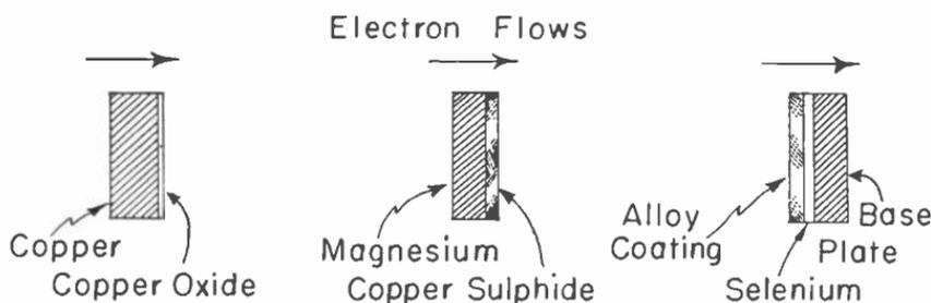
Fig. 2.—Directions of electron flow in contact rectifiers.
