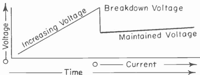
Fig. 3.—The maintained voltage drop in a gas-filled tube is less than the breakdown voltage.
