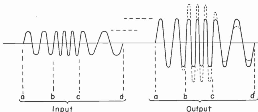
Fig. 8.—Frequency distortion.
