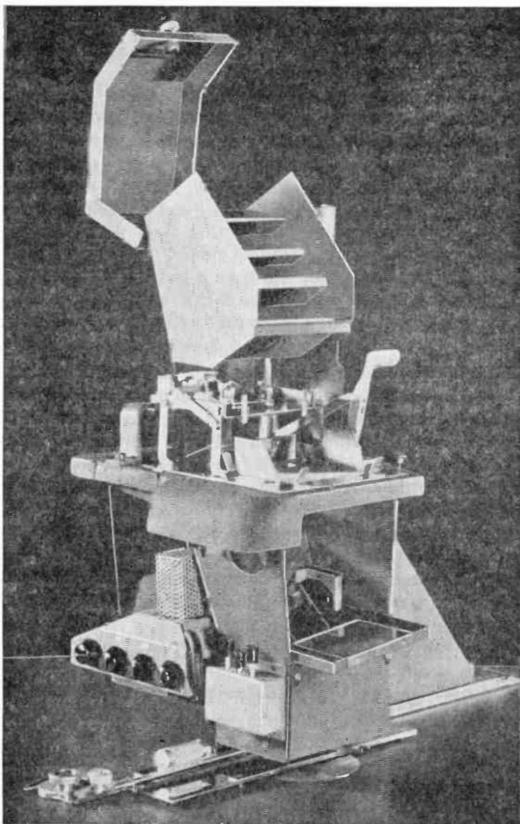
**Fig. 1.—An automatic photographic printer controlled by a phototube.
