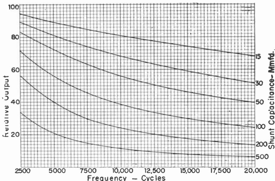
Fig. 10.—How shunt capacitances affect the high-frequency gain.
