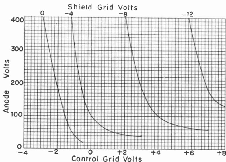
Fig. 20.—Varying the voltage of the shield grid changes the control characteristic of a gas tetrode.
