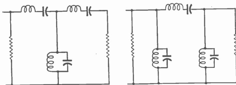
Fig. 27.—Band-pass filters of T-section (left) and pi-section (right).
