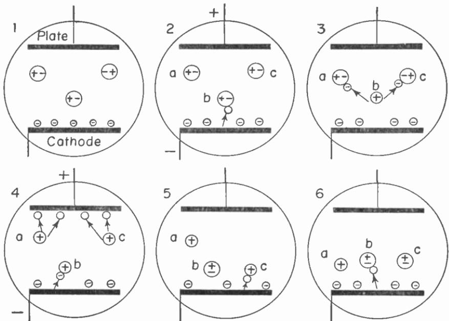
Fig. 2.—What happens during ionization in a tube.
