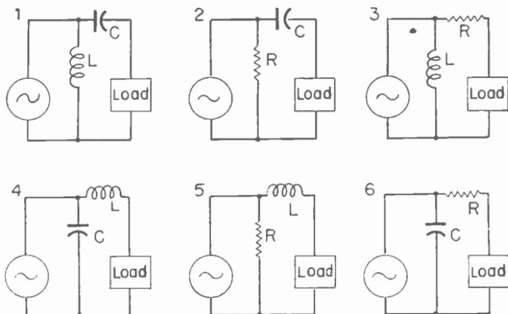
Fig. 5.—Combinations of capacitance, inductance, and resistance in a load circuit.
