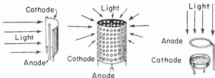
Fig. 3.—Phototube anodes and cathodes.
