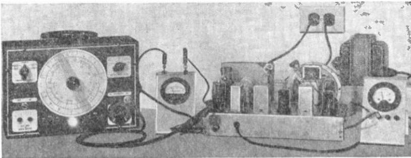
*Fig. 1.—Testing sensitivity by means of servicing instruments.*
