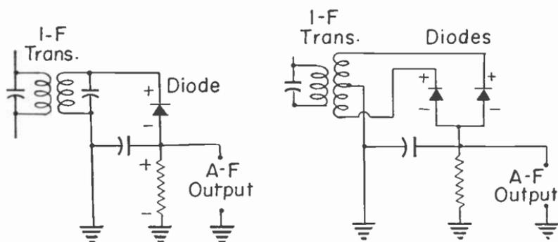
Fig. 9.—Crystal diodes as half-wave and full-wave detectors.
