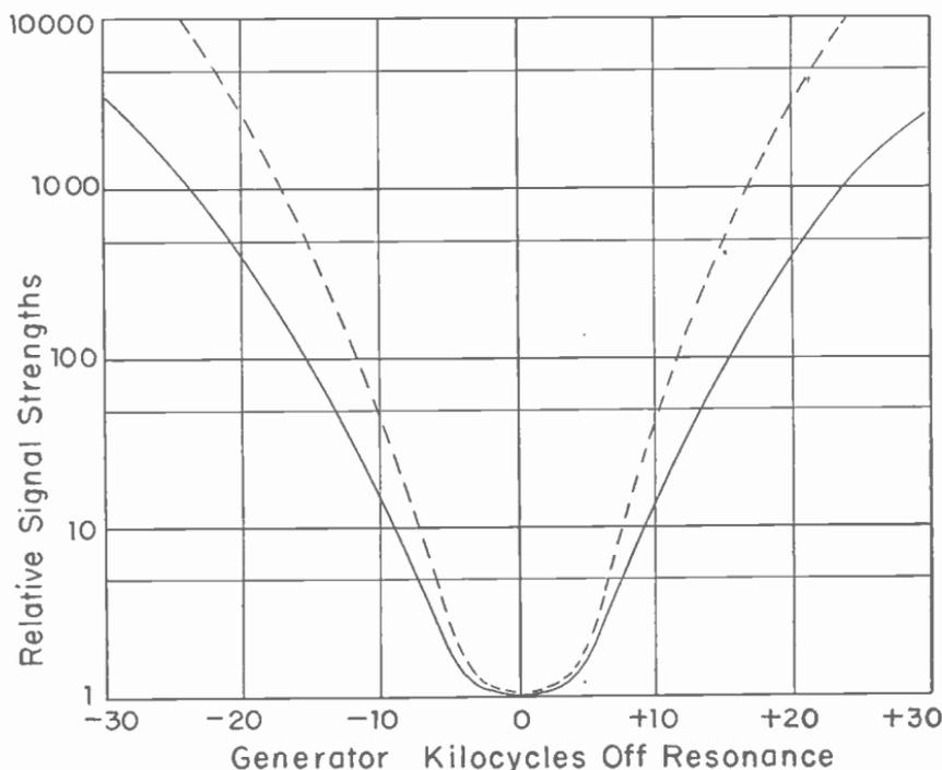
Fig. 9.—Selectivity of an i-f amplifier alone and of the i-f and r-f amplifiers operating together.
