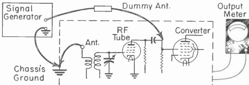
Fig. 8.—Test for selectivity of an i-f amplifier.
