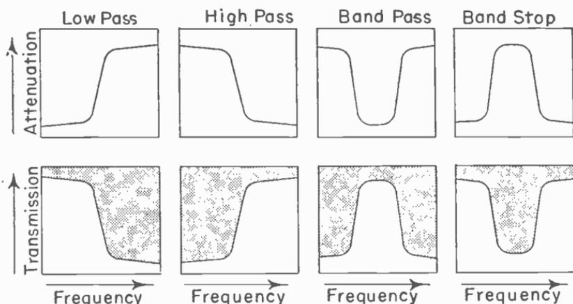
Fig. 20.—Attenuation and transmission characteristics of the four principal kinds of wave filters.
