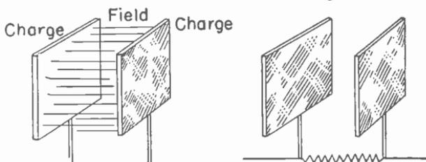
Fig. 17.—There may be capacitive coupling between parts connected through resistance
