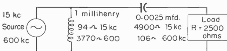
Fig. 6.—The manner in which reactances vary with frequency.
