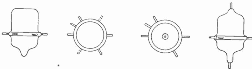
Fig. 4.—Outlines of Acorn tubes, from the side and the bottom.
