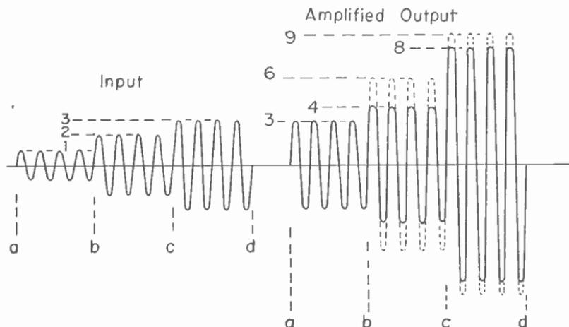
Fig. 2.—Amplitude distortion.
