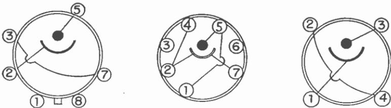
Fig. 8.—Socket and base connections for voltage regulator tubes.
