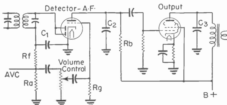
Fig. 10.—High-frequency bypassing in an audio amplifier.
