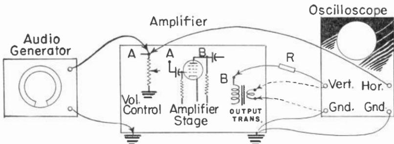
Fig. 13.—Connections of instruments for checking phase distortion.
