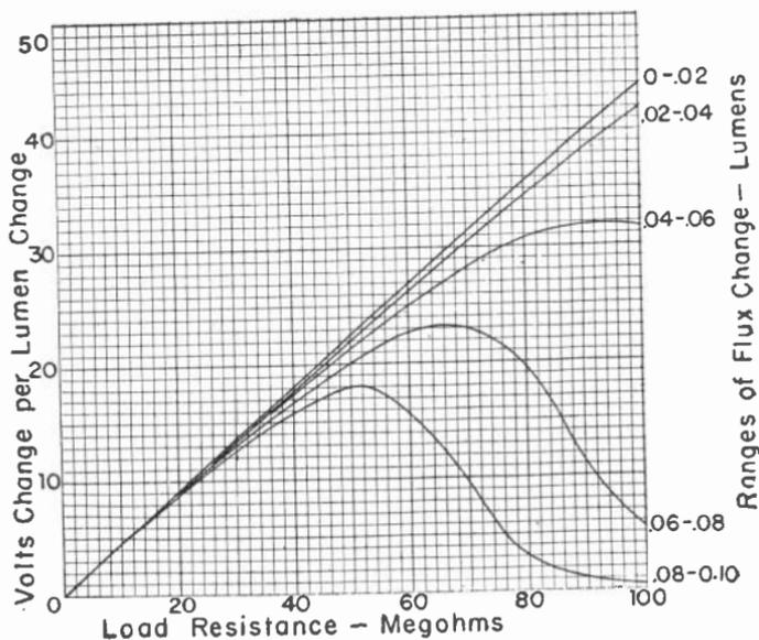
Fig. 17.—Changes of load potential, in volts per lumen of flux change, with a vacuum phototube.
