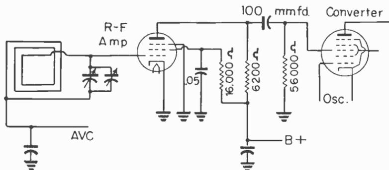
Fig. 15.—Resistance coupling in a radio-frequency amplifier stage.
