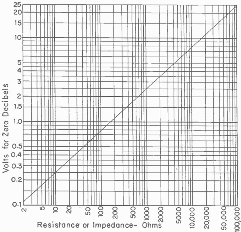
Fig. 7.—Voltages for zero decibels when power is six milliwatts in various values of connected resistance.
