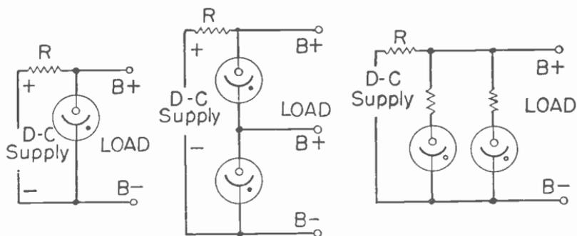
Fig. 9.—Voltage regulator connections; singly, in series, and in parallel.
