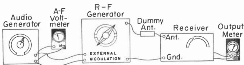
Fig. 10.—Connections of instruments for checking frequency distortion.
