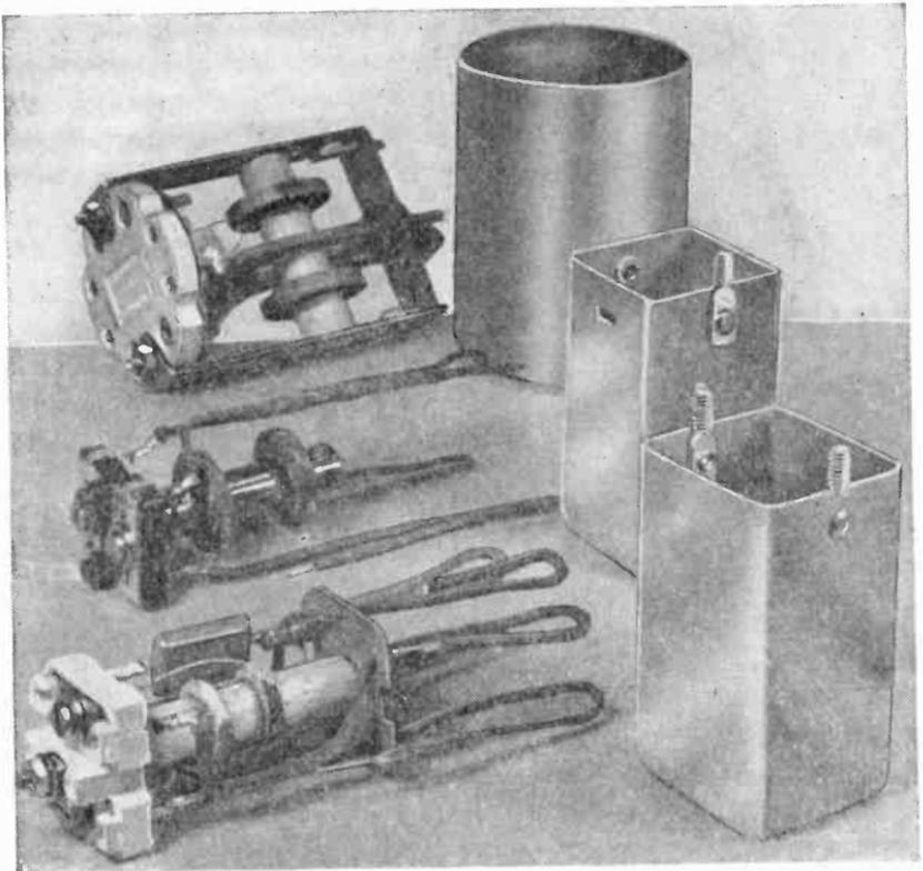
Fig. 16 —Shielding cans and the i-f transformers which they enclose
