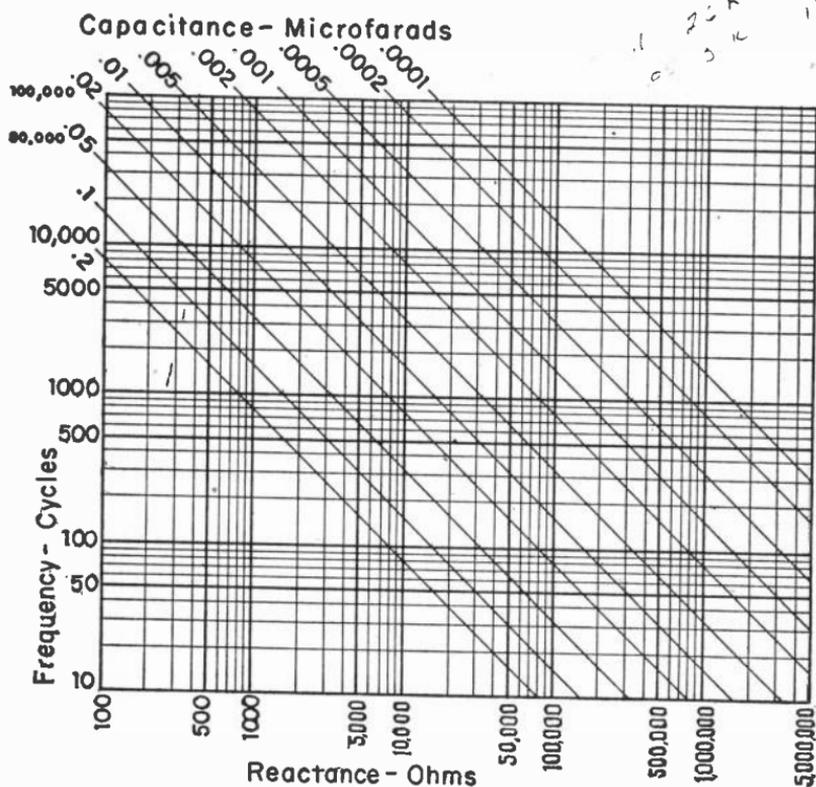
Fig. 6.—Capacitor reactances at audio frequencies.
