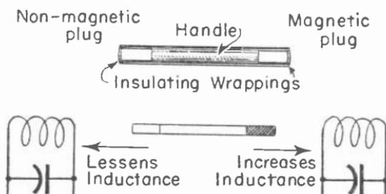
Fig. 10.—Tool for testing tracking of an oscillator.
