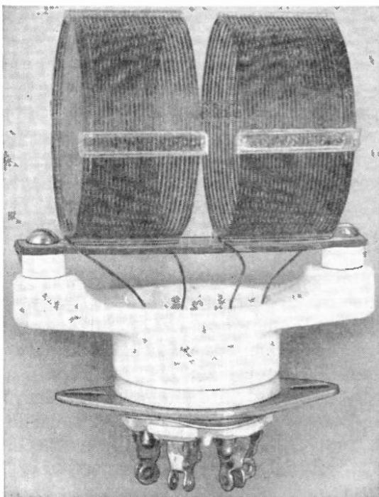
*Fig. 6.—Coils with minimum dielectric in the field space, supported and mounted with polystyrene and steatite.*
