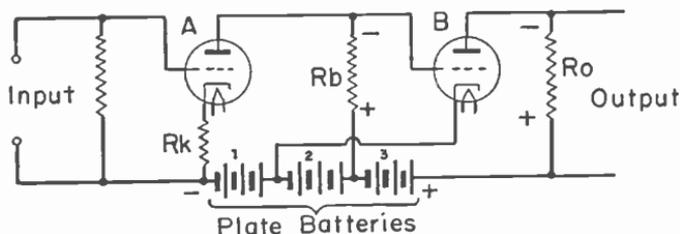
Fig. 19.—An amplifier for direct current or potential.
