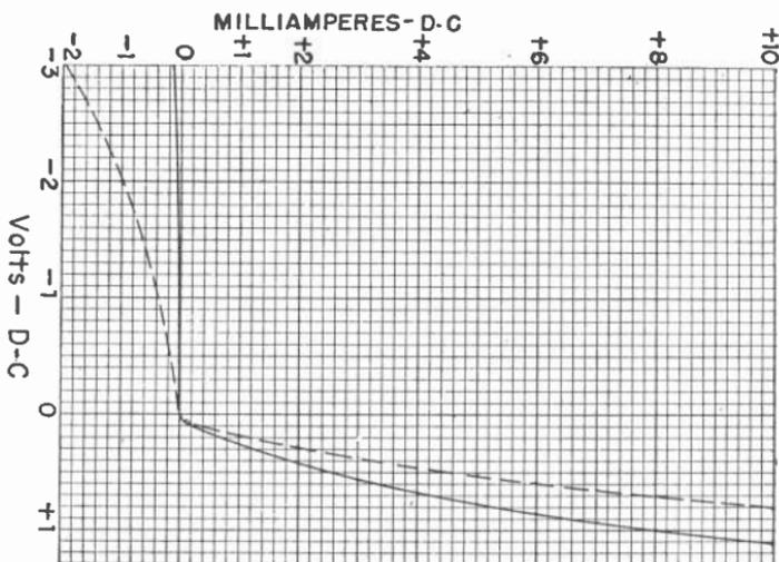
Fig. 8.—Rectification curves for a germanium crystal diode and for a galena detector.
