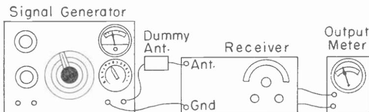
Fig. 11.—Connections for checking sensitivity with signal generator having calibrated output.
