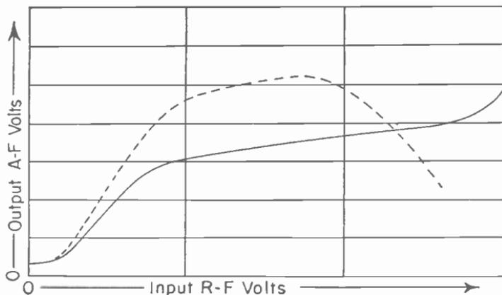
Fig. 15.—Receiver output with and without automatic volume control.
