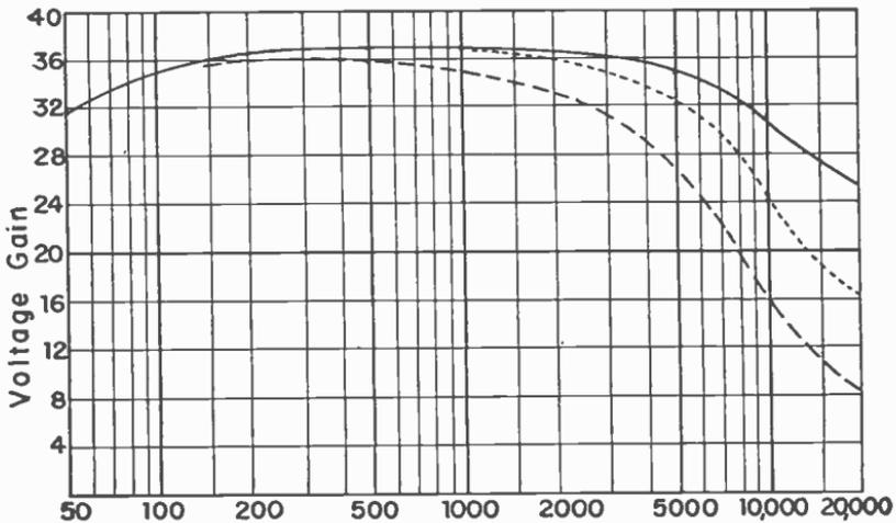
Fig. 12.—Effect of shunt capacitances on overall gain.
