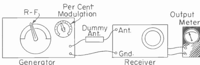
Fig. 3.—Instrument connections for checking amplitude distortion.
