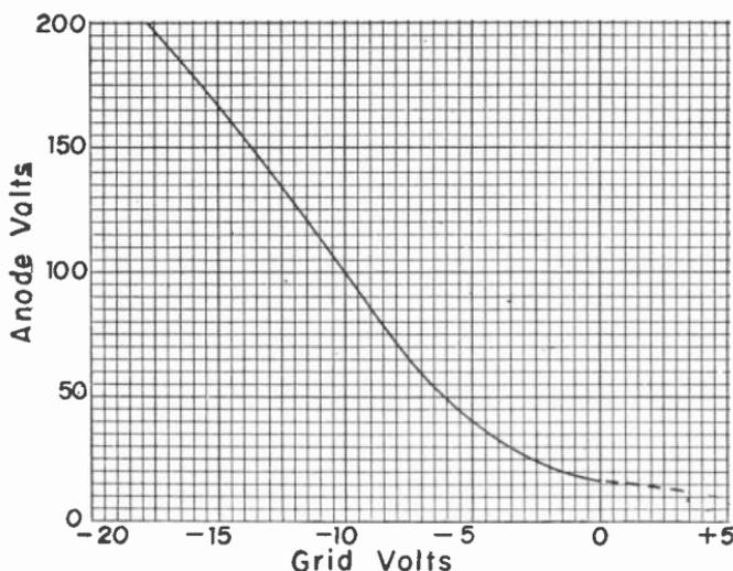
Fig. 14.—Control characteristic for a small gas triode.
