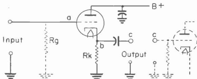
Fig. 16.—Connections for a cathode follower tube.
