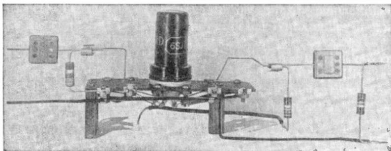
*Fig. 1.—The parts of a resistance-coupled amplifier stage.*
