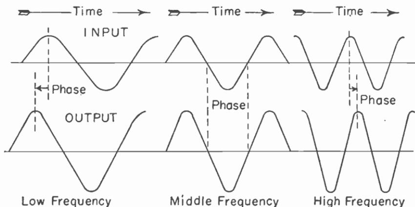
Fig. 11.—Phase distortion.
