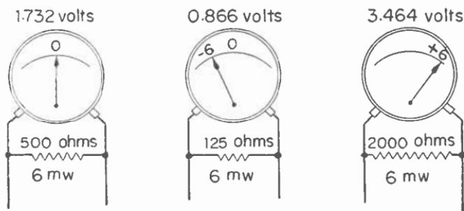
Fig. 8.—Voltages and decibels for a meter connected across various loads.
