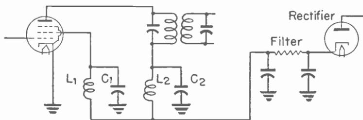
Fig. 12.—Decoupling chokes in plate and screen circuits.
