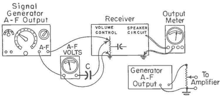
Fig. 17.—Check of variation of gain when the input voltage is changed.
