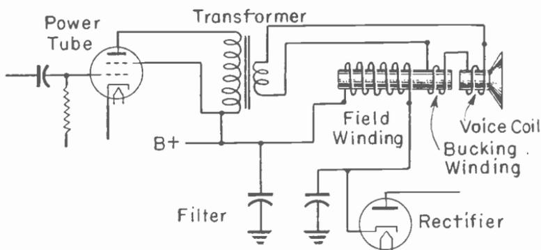
Fig. 19.—Hum bucking with an electromagnetic loud speaker.
