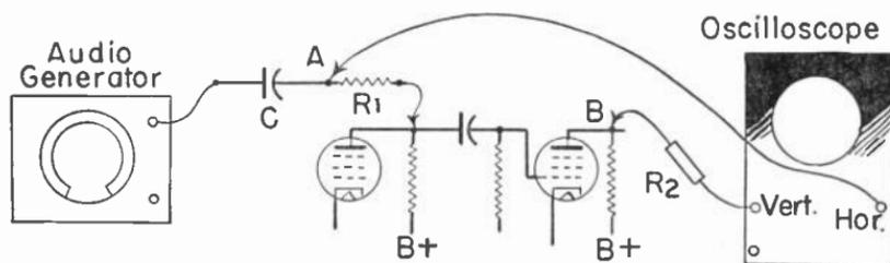
Fig. 14.—Details of connections for the phase distortion test.
