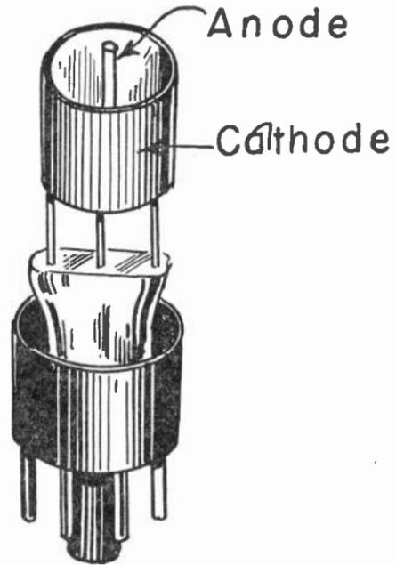
Fig. 5.—The anode and cathode of a voltage regulator.
