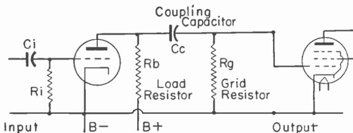
Fig. 2.—Circuit diagram of resistance coupling.
