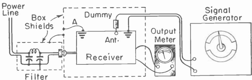
Fig. 3.—How the receiver is protected from interference during selectivity tests.
