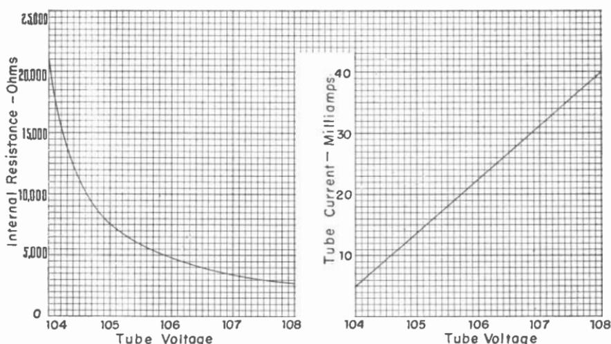
Fig. 7.—Changes of internal resistance and current in a voltage regulator when there are changes of voltage drop.
