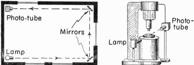
Fig. 29.—A phototube burglar alarm (left) and safety guard for machines (right).
