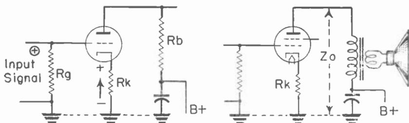
Fig. 5.—Current feedback with a cathode-bias resistor.
