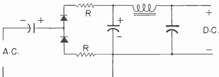
Fig. 5.—Voltage doubler rectifier circuit with two selenium rectifiers.
