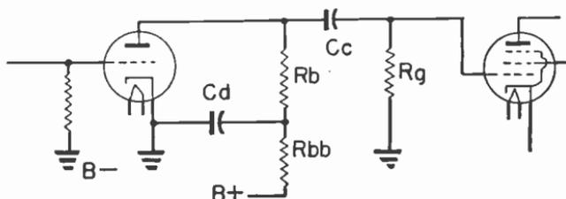
Fig. 4.—Decoupling resistor in series with load resistor.
