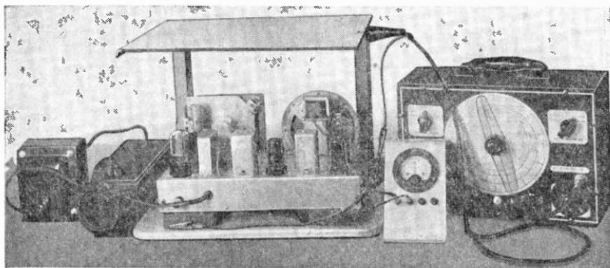
Fig. 12.—A test setup for measuring pickup in an r-f field.
