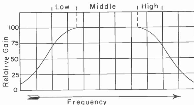
Fig. 3.—Relative gain in various ranges of frequency.
