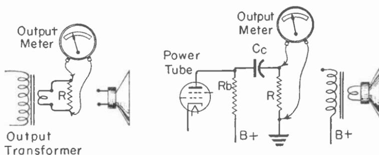
Fig. 4.—Connections for dummy load resistors.
