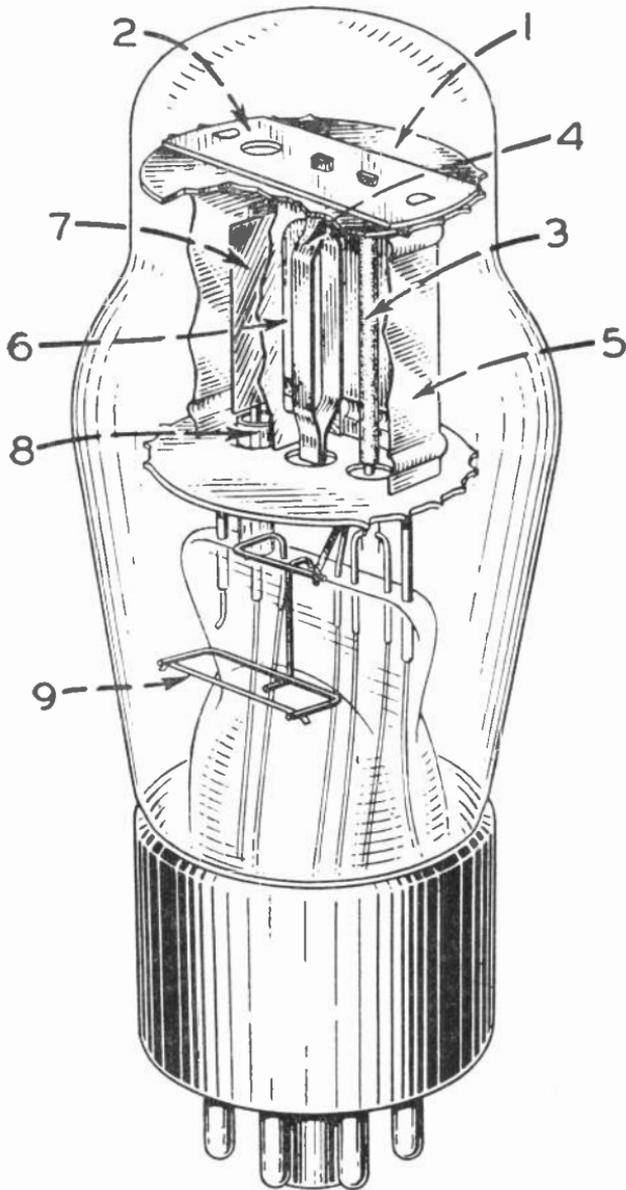
Fig. 18.—The construction of an RCA gas tetrode.
