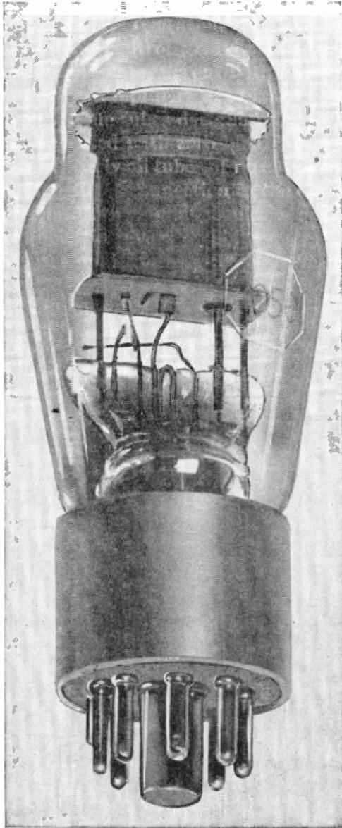
*Fig. 1.—A gas-filled tetrode tube used for control purposes.*
