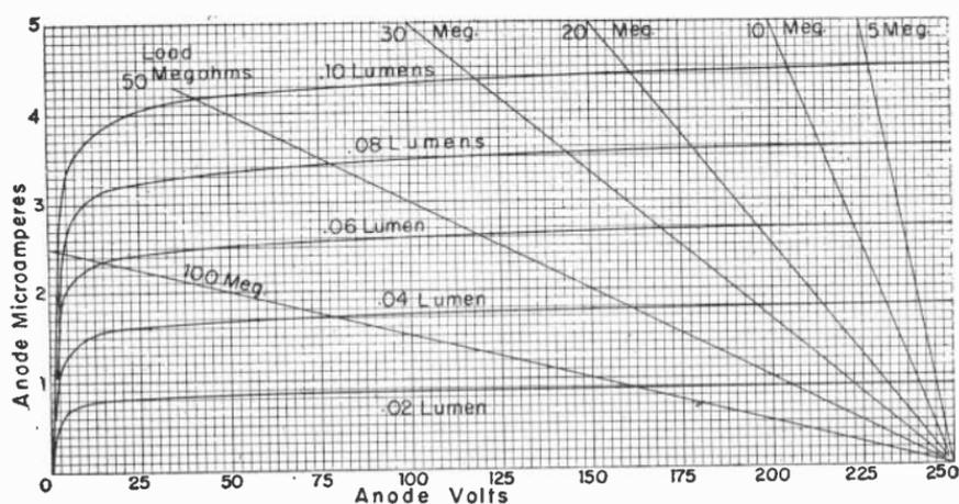
Fig. 15.—Load lines on the anode characteristics of a vacuum phototube.
