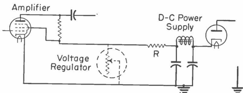
Fig. 6.—The voltage regulator acts like a variable resistance in parallel with the load.
