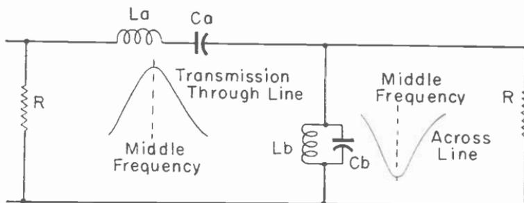
Fig. 26.—The operation of an L-section band-pass filter.
