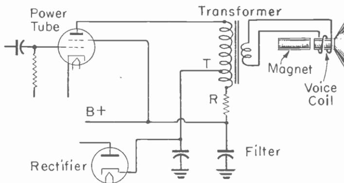
Fig. 20.—Hum bucking with a permanent magnet loud speaker.
