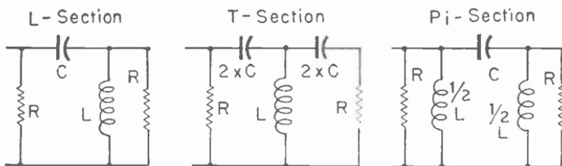
Fig. 25.—Connections for high-pass filters of three types.
