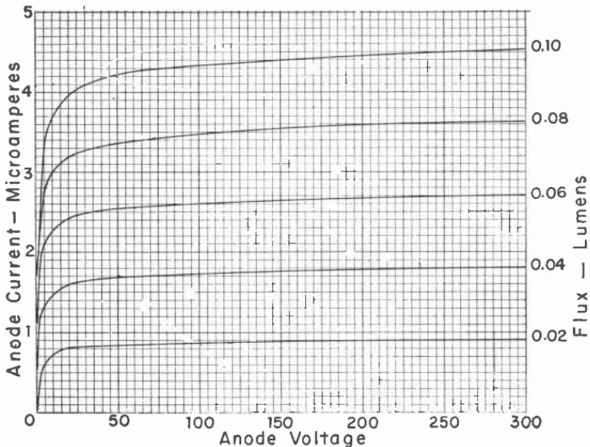
Fig. 11.—A family of anode characteristics for a vacuum phototube.
