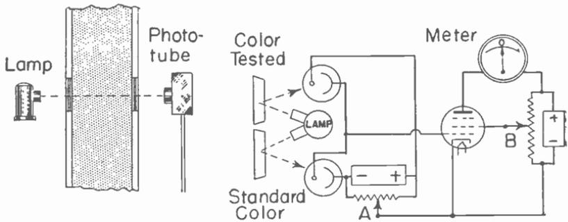
Fig. 32.—Phototube inspection for smoke or translucency in any space (left).
