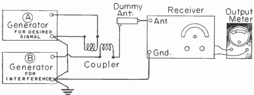
Fig. 5.—Using two signal generators for testing selectivity.
