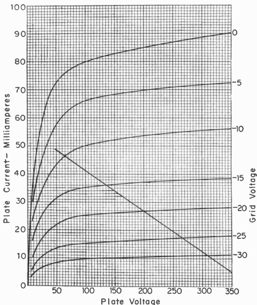
Fig. 19.—The load line used in the example of computing voltage gain.
