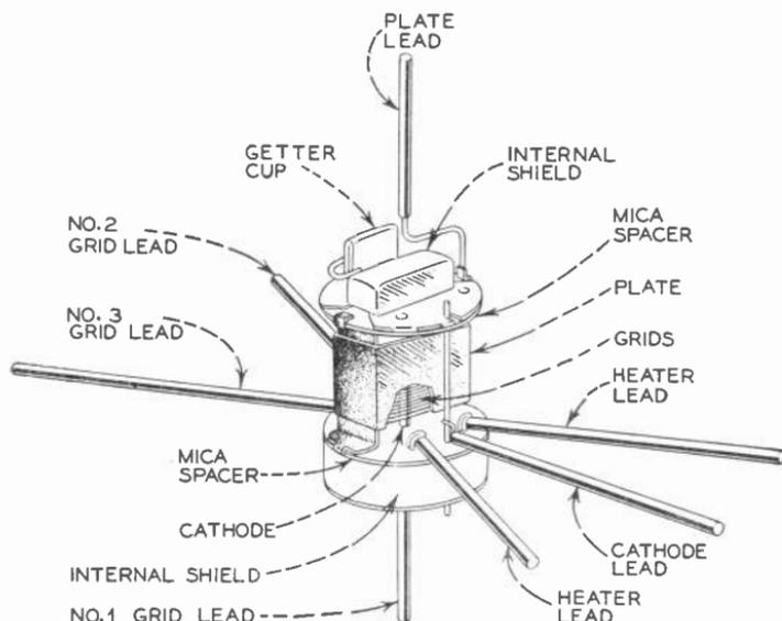
Fig. 5.—The arrangement of elements and pins in an RCA Acorn pentode tube.
