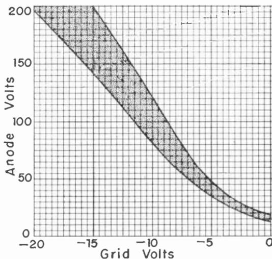
Fig. 15.—Operating limits for a typical gas triode.
