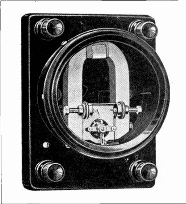
Fig. 104. Very sensitive relays such as shown above are commonly made with the same principal elements used in voltmeters' or ammeters. Relays of this type can be used to open or close various circuits at any set voltage or current values.
