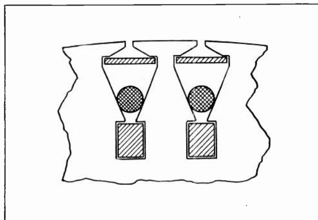
Fig. 201. This sketch shows the slot and bar construction of double squirrel-cage rotors using iron "choker bars" to change the resistance of the field and outer circuits.
