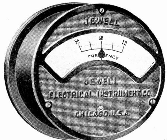
Fig. 74. This photo shows a switchboard type frequency meter, such as commonly used in power plants. The connections to instruments of this type are made to brass terminal bolts which project through the switchboard from the back of the meter.
