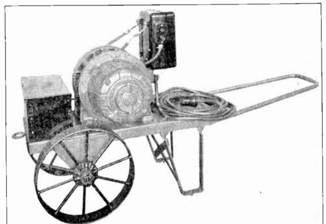
Fig. 210. Portable A.C. induction motor particularly adapted for use on farms and for driving portable machinery. (Courtesy G. E. Company.)
