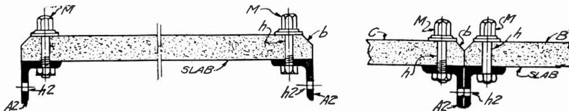
Fig. 62. The above sketches show the method of attaching switchboard panels to the angle iron frame work. Note how the panels are bolted to angle irons, and the angles bolted together between panels. Also note the type of bolts, nuts, and washers used with this construction.
