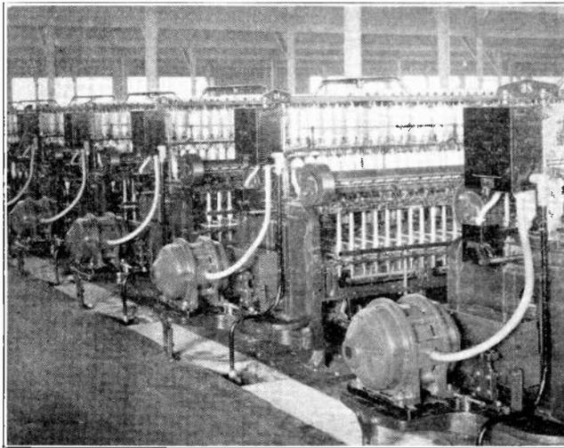
Fig. 5. This view shows a number of A. C. motors being used for individual drive on machines in a textile mill. Thousands of factories and industrial plants use electric motors in this manner for driving their various machines and equipment. (Photo courtesy G. E. Company)
