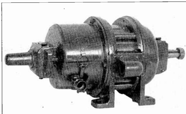
Fig. 158. A. C. induction motor with totally enclosed frame to keep out dust and dirt from the windings and also prevent fire and explosion hazard. (Photo courtesy General Electric Co.)
