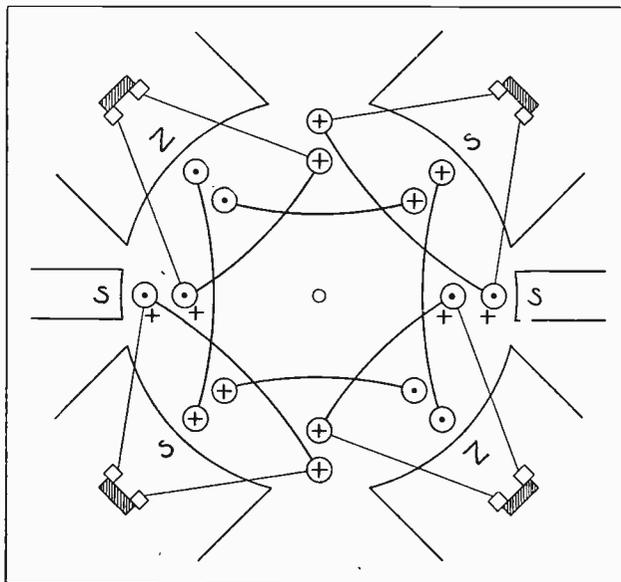
Fig. 56. This simple sketch illustrates the manner in which two interpoles can be used to neutralize self-induction in the coils of a four-pole machine.
