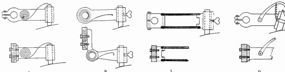
Fig. 17. The sketches on the left show several common types of brush holders. At "A" are two views of box-type holders. "B" and "C" are known as clamp-type holders; while "D" is a brush holder of the reaction-type.
