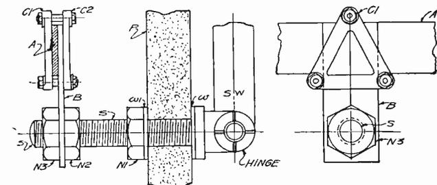
Fig. 73. Two views showing the method of connecting bus bars to the studs of switches and circuit breakers.
