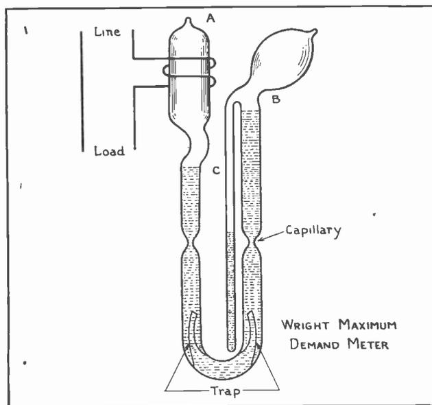
Fig. 98. This sketch illustrates the principle of a common type maximum demand meter which operates by expansion of the air in the bulb "A", when current is passed through the coil around this bulb.
