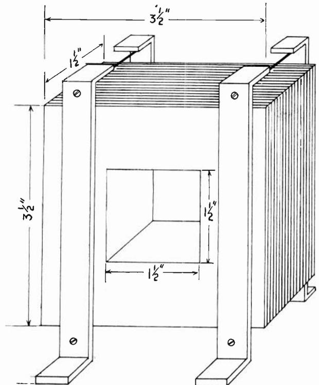
Fig. 153-C. A 50 w. transformer core constructed from strips  $1'' \times \frac{1}{2}''$ . Note the method of binding the strips together.
