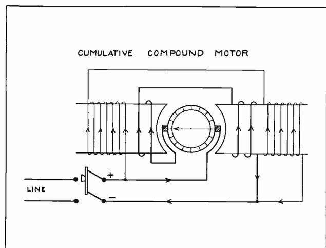
Fig. 113. Diagram of connections for a cumulative compound motor. Note that the series field winding is connected so it will aid the shunt field winding in providing a strong field.
