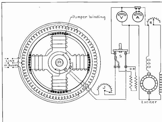
Fig. 91. This diagram shows the connections of the stator and rotor of a three-phase alternator with the exciter-generator, rheostats, meters, and field discharge switch.
