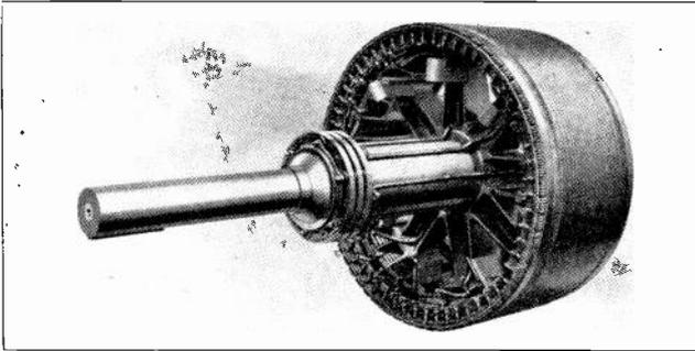
Fig. 181-A. Phase wound rotor of a large slip-ring induction motor. This rotor has heavy bar windings which are not shorted together like those of a squirrel-cage rotor, but instead have connections brought out from each phase to the slip rings.
