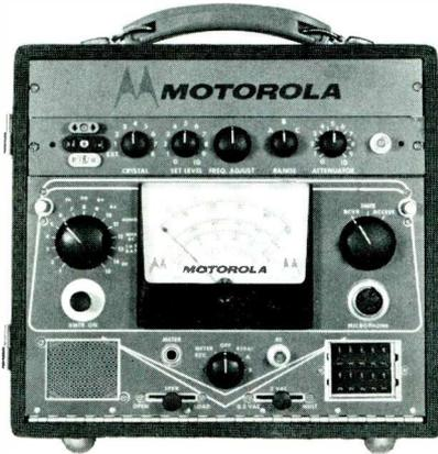
The TU546P Test Set Includes a Peaking Generator, Located on the Upper Panel.
