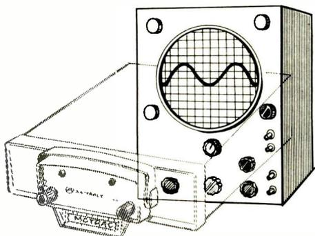
A Scope is Very Useful in Adjusting the IDC Circuit and Trouble Shooting the Audio Section of the Transmitter.
