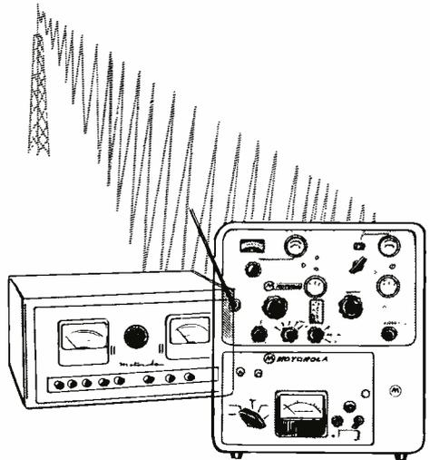
The Motorola Monitor and Frequency Meter will Also Measure the Deviations of an FM Transmission.
