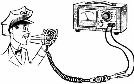
Establishing the Amount of Mike Voltage--As Measured on a Sensitive AC Voltmeter--is Helpful in Diagnosing Modulation Problems.
