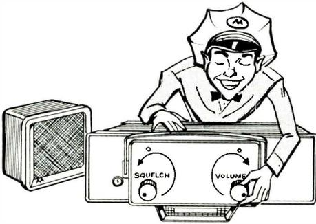
A Quick Check On Receiver Operation is Made by Turning the Volume Full-On and Opening the Squelch.
