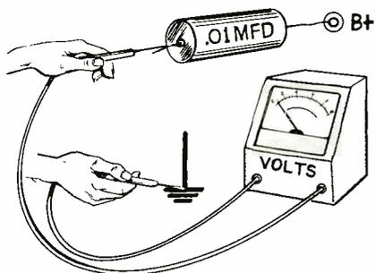
A Voltmeter in Series With a Capacitor and Connected Between B+ and Ground Gives a Reliable Check for Leaky Capacitors.
