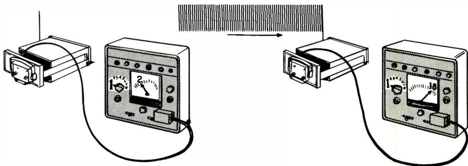
Comparing Meter Readings With and Without a Channel Signal is Very Helpful in Trouble Shooting the Receiver.
