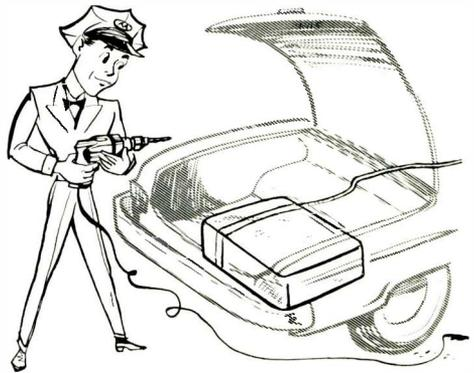
Be Sure to Avoid the Gas Tank, Gas Line and Similar Parts of a Vehicle when Drilling Holes and Mounting Two-Way Radio Equipment.
