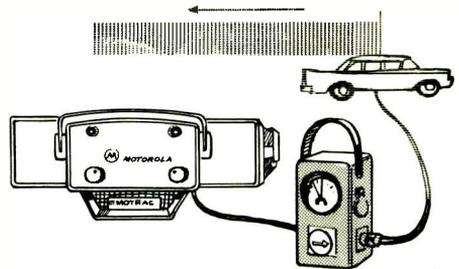
If a Thru-line Output Meter is Used, the Transmission Line Should Terminate into the Antenna.
