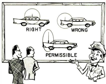
Wherever Possible the Mobile Antenna Should be on the Roof Top. Long (Lo Band) Antennas may be Mounted on a Fender if Necessary.
