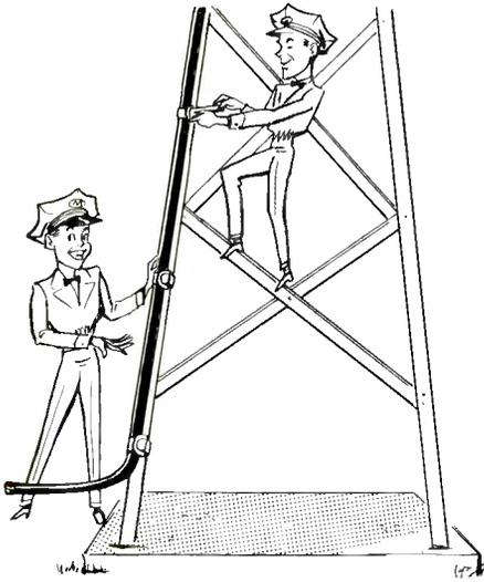
In Base Station Installations the Transmission Line Must be Well Secured to the Tower.
