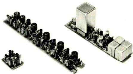
Starting at the Left, We See the Low-Frequency Oscillator, 455-KC IF and High-Frequency Oscillator-Multiplier Sections of a Transistorized Receiver.
