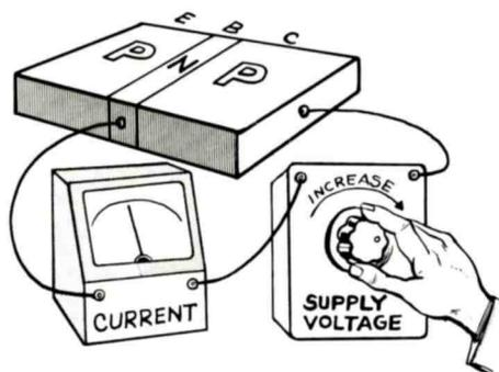
**Increasing the Reverse Collector Bias Produces Little If Any Increase in the Collector Current.**
