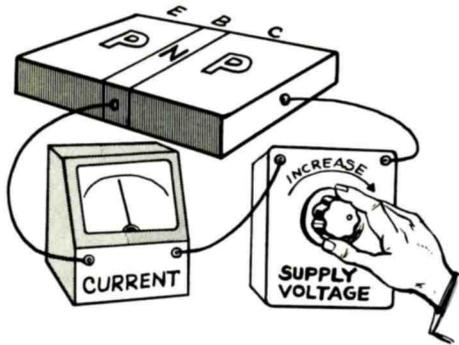
Once Collector Current has been Established in the Transistor, Increasing the Collector Voltage has Little Effect Upon the Collector Current.
