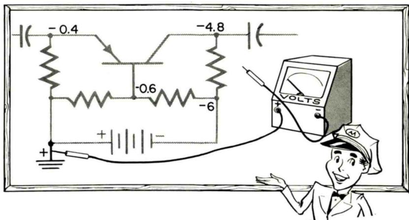
If the Positive Side of the Supply is Grounded, Connect the Positive Test Probe to Ground and Measure Voltages with the Negative Test Lead.
