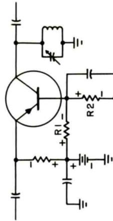
COMMON-BASE BIAS CIRCUIT FOR "NEGATIVE GROUND" SUPPLY
