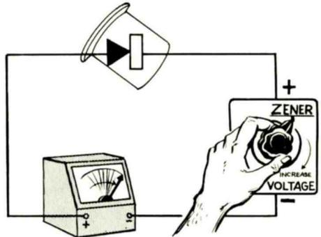
When the Reverse Voltage at the Diode is Increased to the "Zener" Voltage, a Large Current Suddenly Occurs.
