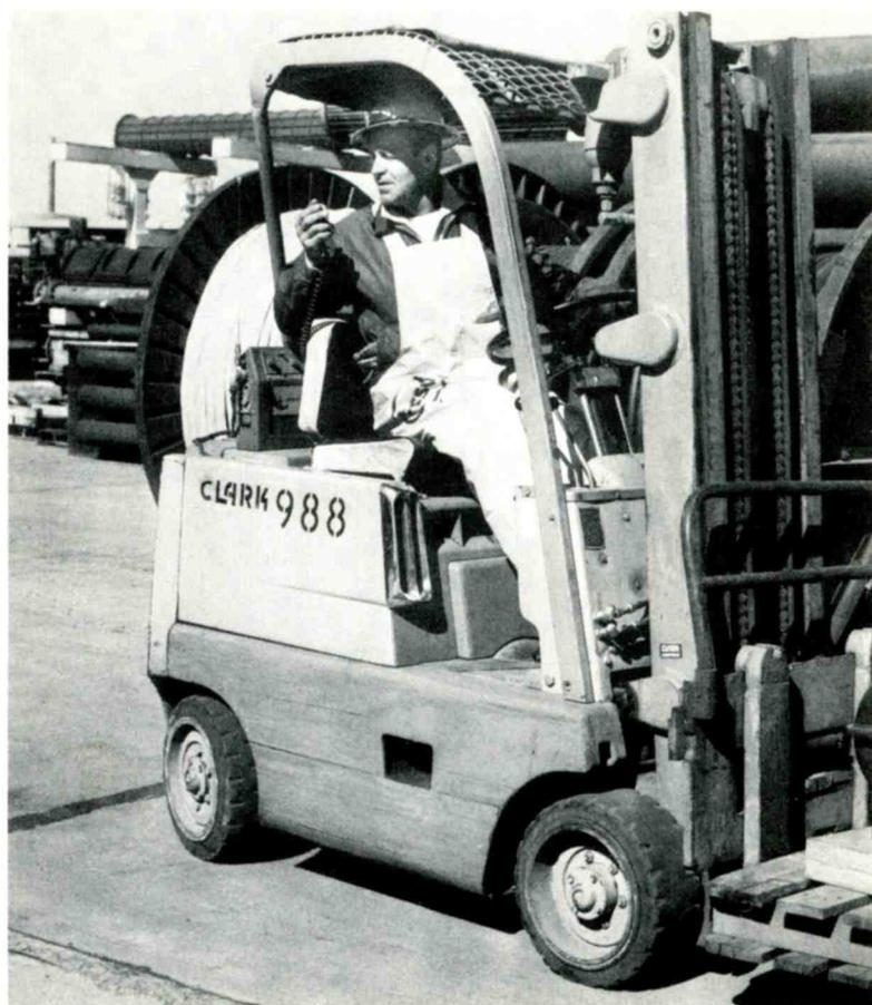
Industrial "Dispatcher" radiophone is designed specifically for use on materials handling vehicles such as this fork truck. Radio control of such trucks greatly increases storage and warehousing efficiency.
