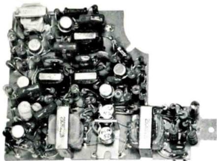
Here We See the Audio and Squelch "Circuit Board" of a Typical Mobile Two-Way Receiver.
