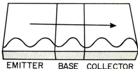
Where the Transit Time of the Carriers Through the Base is an Appreciable Portion of One Cycle, the Transistor Will Not Provide Much Gain.
