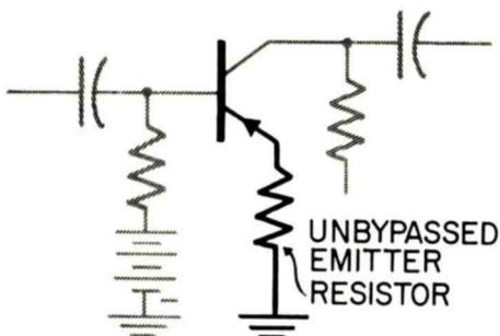
The Unbypassed Emitter Resistor Improves the Frequency Response of an Amplifier and Also Reduces Distortion.
