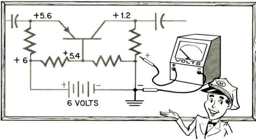
With the Negative Side of the Supply Grounded, All the Circuit Terminals are "Positive." To Make Voltage Checks, Ground the Negative Test Lead.
