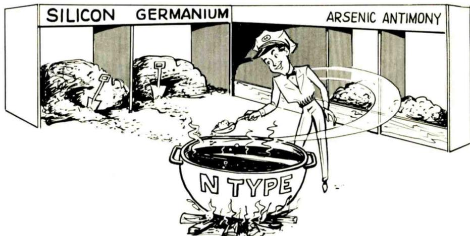
"N-Type" Semiconductor Material is Made by Adding a Small Amount of Arsenic or Antimony--Materials Which Have 5 Valence Electrons--to Germanium or Silicon.
