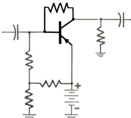
The Collector-Base Resistor Gives Good DC Stabilization, But It Also Introduces Degeneration.
