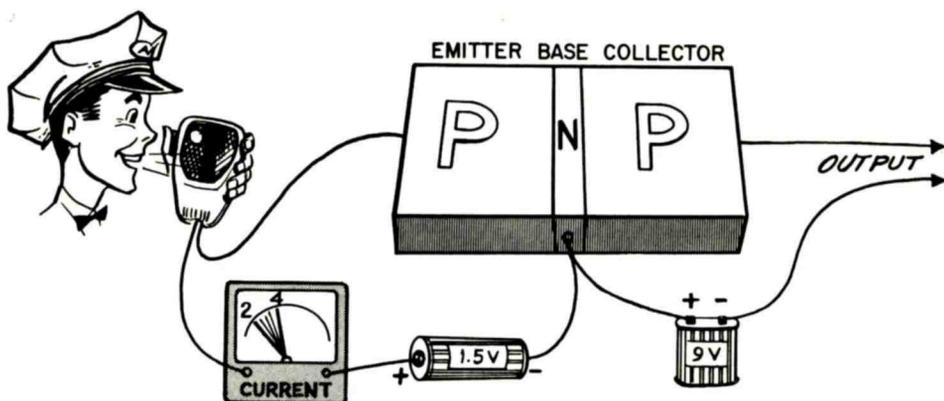
In Transistor Operation, the Current Changes are More Important than the Input Voltages: These Current Changes Control the Output Signal.
