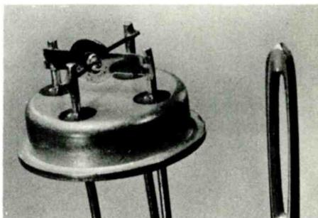
This Photo Shows the Typical Construction of Medium-Low Power Audio Transistors.
