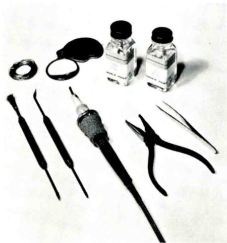
Here We See the Basic Tools Required for Fast and Efficient Service of Transistorized Equipment Using Printed Boards.
