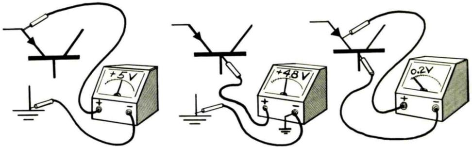
Do Not Measure Emitter Junction Bias Between the Emitter and Base:
