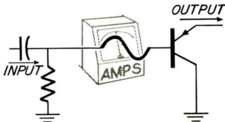
In Analysing the Transistor Amplifier Input, the Important Consideration Is To Provide a Sinusoidal Current Change for an Applied Sinewave Voltage.
