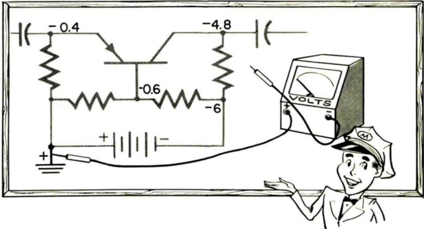
Where the Positive Side of the Supply is Grounded, All the Circuit Terminals are "Negative." Ground the Positive Test Lead of the Meter for Voltage Measurements.
