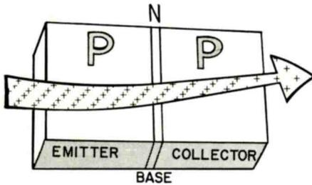
For PNP Transistors, Current is Due Mainly to the Movement of Positive Carriers (Holes) From the Emitter to the Collector.
