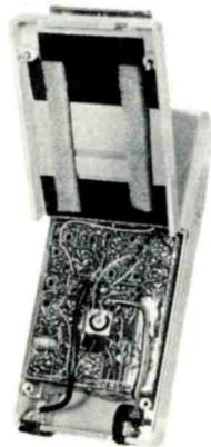
This Photo Shows the Modular Construction of a Motorola Pocket-Size VHF Receiver.
