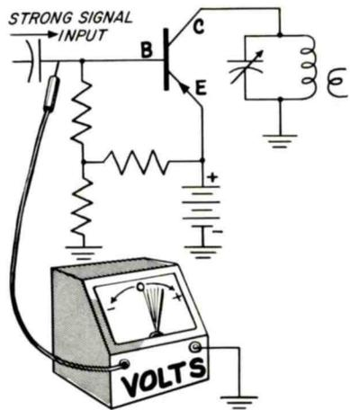
When the Input Signal Overdrives the Input Circuit, the Base-To-Ground Voltage of the Transistor Limiter Stage Varies in the Positive Direction.
