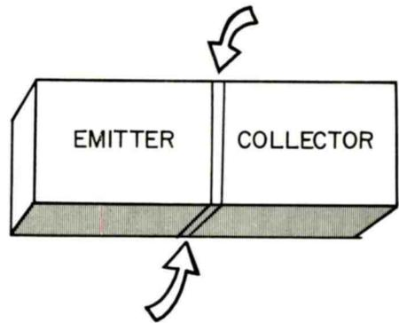
In a Transistor the Base Region Between the Two Junctions is Normally Less Than .001 Inch Thick.
