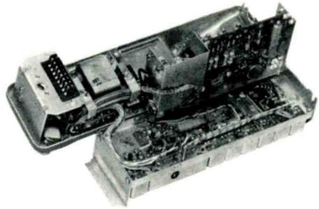
This Photo Shows the Complete Internal Construction of the Motorola Handie-Talkie Transmitter and Receiver.
