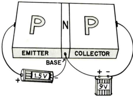
Normal Bias of a PNP Transistor Demands a Positive Emitter and a Negative Collector, Both With Respect to the Base.
