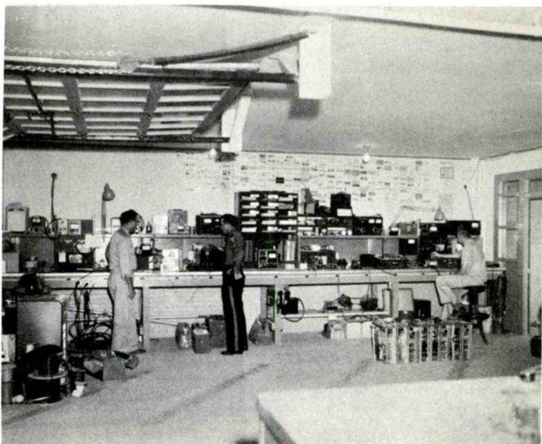
Adequate bench space and equipment is needed for efficient servicing of mobile radios. Reference literature is also conveniently located. This Maintenance Center accommodates several technicians.
