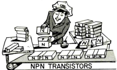
Basically, an NPN Transistor is Made by Sandwiching a Thin Slice of P Material Between Two N Areas.
