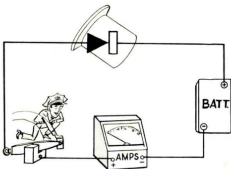
Reverse Bias Applied to the Semiconductor Diode Does Not Produce Current at the Junction.
