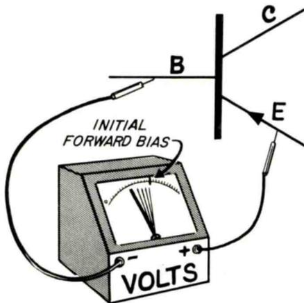
One Test for Limiter, Oscillator and Frequency Multiplier Stages is a Change in Operating Bias at the Emitter Junction.
