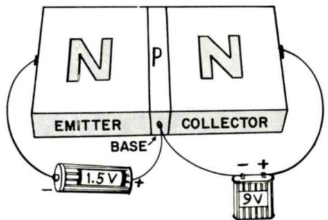
For an NPN Transistor, the Emitter Should be Made Negative to the Base and the Collector Should be Positive.
