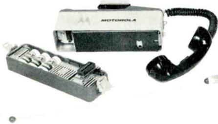
Here We See a Battery Supply for a Portable Two-Way Radio.
