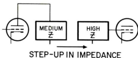
Inter-Stage Coupling Methods in Vacuum-Tube Equipment Must Provide an Impedance Step-Up From One Stage to the Next.
