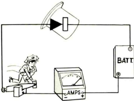
Forward Bias at the Semiconductor Diode Causes Current Through the Junction.
