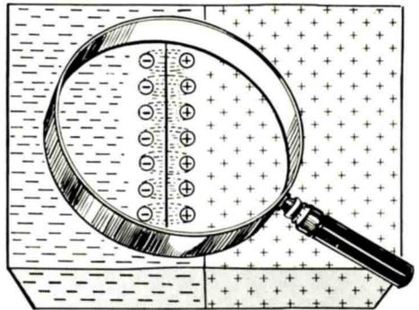
At the P-N Junction, the Fixed Charges Produce a "Barrier Field" Within the Depleted Area.
