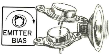
Proper Operation of the "Class B" Push-Pull Audio Amplifier Depends Upon the Correct Emitter Bias.
