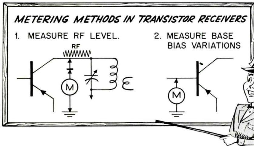
Either or Both of These Metering Methods May Be Encountered in the Transistorized Communication Receiver.
