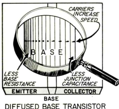
The Diffused-Base Technique is Used Almost Universally in High-Frequency Transistors.
