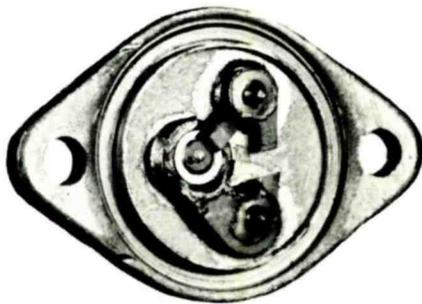
The Power Transistor is Large and Usually Has Its Collector Grounded to the Frame for Efficient Heat Dissipation.
