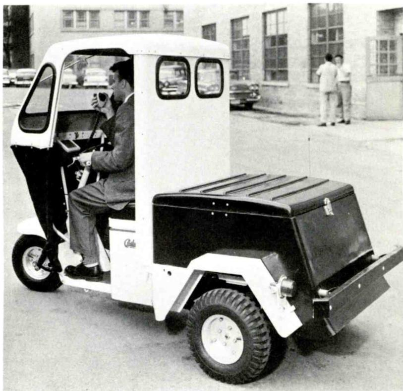
Extensively transistorized two-way units are ideally adapted for use on personnel carriers and other small plant area vehicles. Compactness, reliability, and low battery drain are basic requirements for this application.
