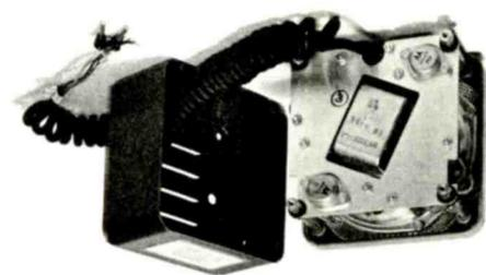
Here We See the Transistors and Heat Sink Chassis of a Motorola Power Voice Speaker.
