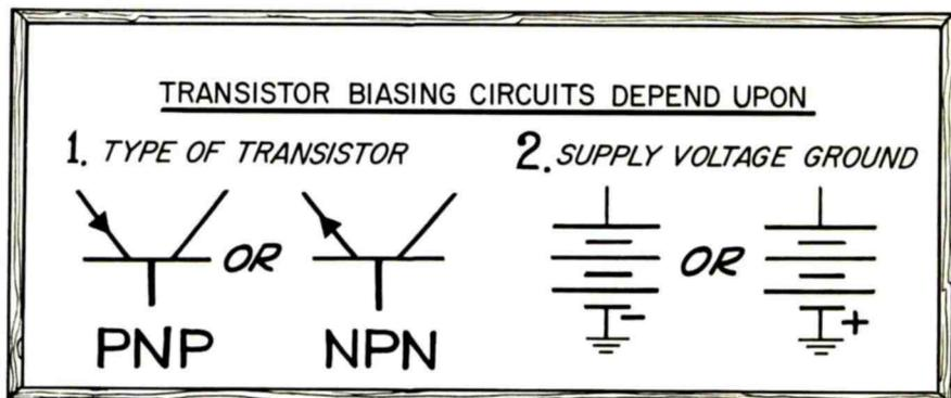
The Biasing Arrangement of the Transistor Circuit Varies With (1) the Common or Grounded Terminal of the Supply and (2) the Type of Transistor.
