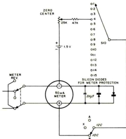
Here We See the Protective Diode Meter Circuit of the Motorola Test Set.
