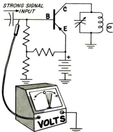
The Signal Strength at the Base of Oscillator, Limiter and Frequency Multiplier Stages May Be Measured by the Change of Base Voltage.
