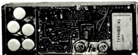
This Modern Two-Way Communications Receiver Includes Two Power Transistors (Lower Right). The Cast Aluminum Frame Makes an Efficient Heat Sink.
