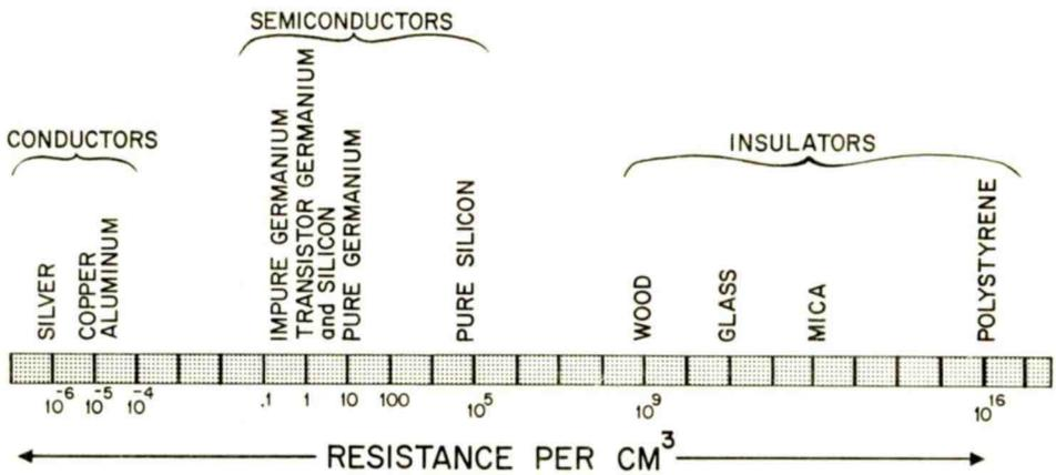
The Elements are Often Classified as Conductors, Semi-Conductors and Insulators, According to their Electrical Resistance.
