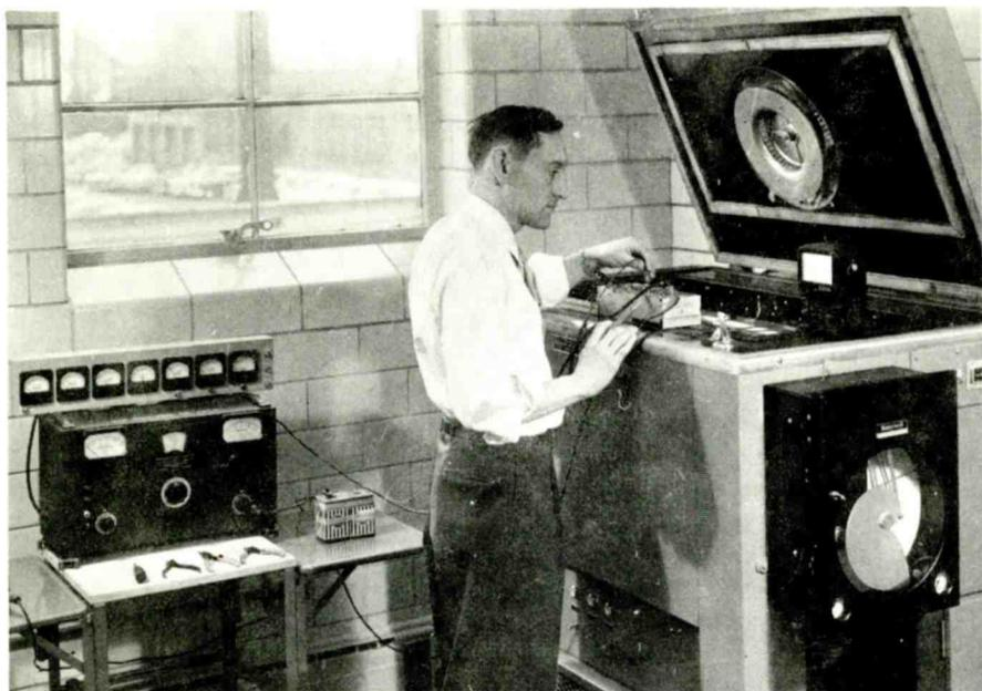
In Designing Transistorized Equipment, It is Important to Check for Operation at All Temperatures.
