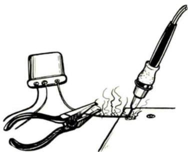
**A Pliers Holding the Lead Between the Transistor and the Soldered Connection Prevents Overheating of the Transistor Junctions.**
