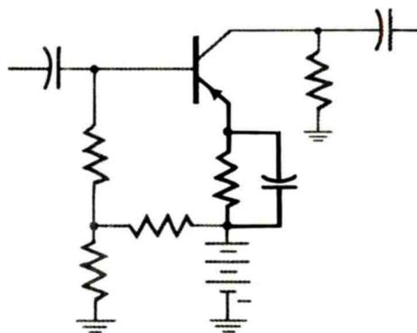
The Emitter Resistor Provides DC Stability to the Transistor Amplifier; the Bypass Avoids Degeneration Due to the Resistor.
