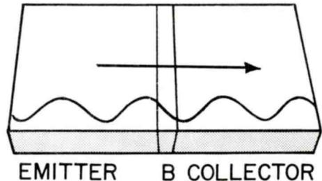
A Narrow Base Area Means a Short Transit Time and the Ability to Amplify at Higher Frequencies.
