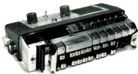
Here We See The Modular Construction of the Transistorized "Dispatcher" Motorola Receiver.
