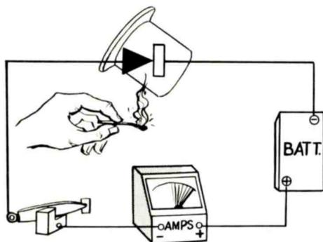
An Increase in Diode Temperature Causes an Increase in Diode Current.
