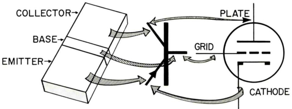
Here We See a Comparison of the Transistor Elements With Those of the Vacuum Tube.
