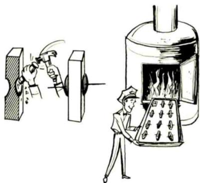
In Actual Transistor Construction, Wells are Made in the Sides of the Base. Emitter and Collector Materials are Next Placed in the Wells. The Entire Assembly is Then Heated to a Specific Temperature for a Predetermined Length of Time.
