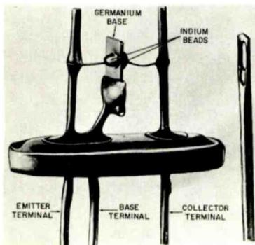
Here We See the Actual Construction of a Low-Power, Low-Frequency Transistor. The Actual Size May be Judged by the Size of the Needle at the Right.
