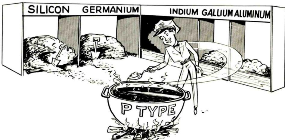
"P-Type" Semiconductor Material is Made by Adding Small Amounts of Indium, Gallium or Aluminum--Materials Which Have But 3 Valence Electrons--To Germanium or Silicon.
