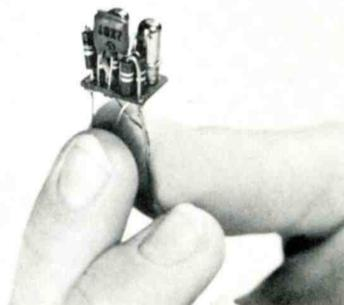
Here We See a Complete Stage (Module) of a Modern Pocket-Size Receiver.
