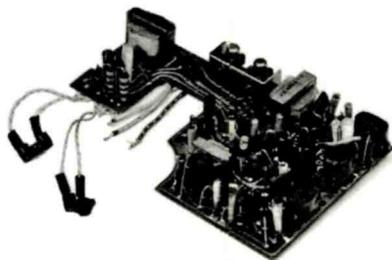
Here We See a Typical "Printed Board." This is the Audio and Squelch Section of a Modern Motorola Receiver.
