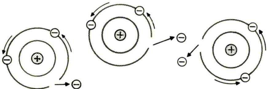
Conduction or Non-Conduction of an Element Depends Primarily Upon the Number of Free or "Valence" Electrons in the Outer Electron Shell.
