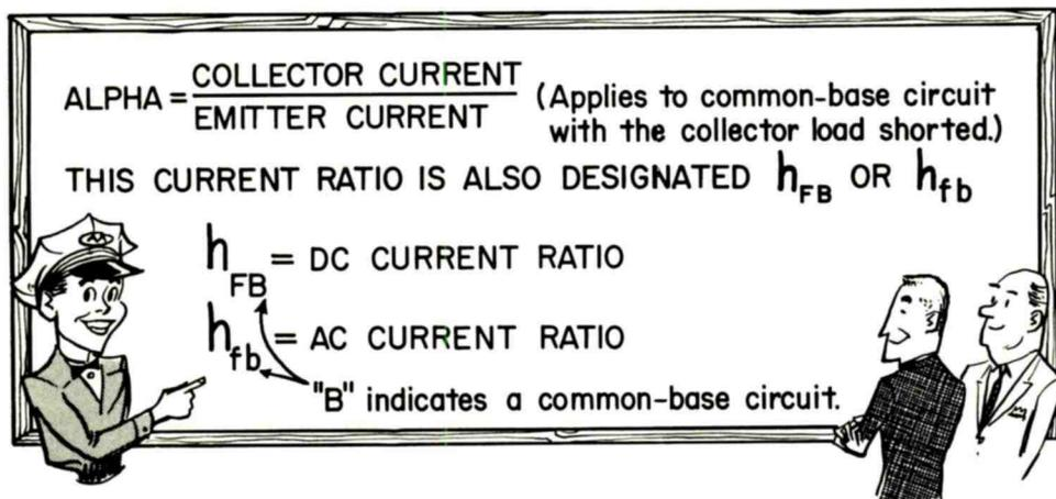
Alpha and " $h_{FB}$ " or " $h_{fb}$ " Ratings Refer to the Common-Base Circuit With the Collector Load Shorted.
