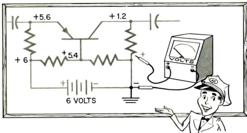
When the Negative Side of the Supply is Grounded, Connect the Negative Test Lead of the Voltmeter to Ground and Take Readings with the Positive Lead.
