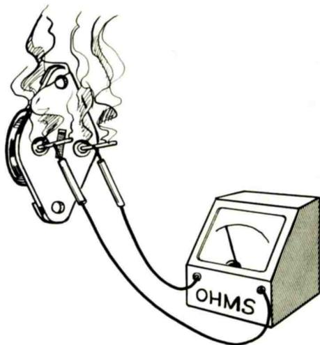
Some Ohmmeters Deliver Considerable Current to the Circuit Under Test. This High Current May Damage Transistors.
