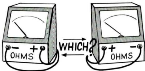
**Intelligent Use of an Ohmmeter Requires the Serviceman to Know the Polarity of the Internal Battery With Respect to the Test Leads.**
