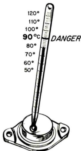
Transistors Can Be Damaged by Excessive Heat.
