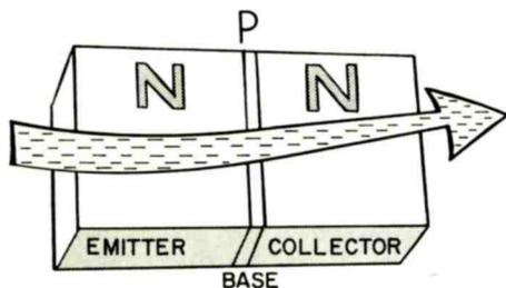
For NPN Transistors, Current is the Result of Electrons Leaving the Emitter and Crossing the Base Into The Collector
