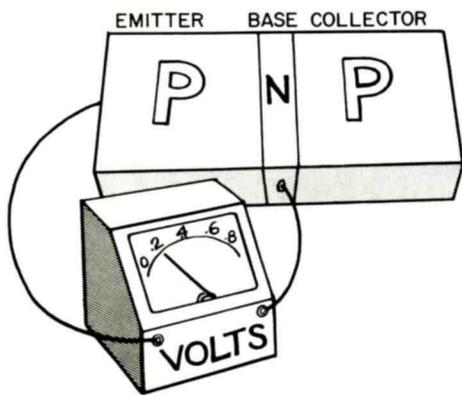
The Average Forward Bias at the Emitter-Base Terminals of a Transistor is About 0.2 Volt.
