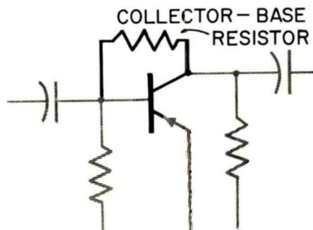
Distortion Can Be Reduced by Connecting a Resistor Between the Collector and Base.
