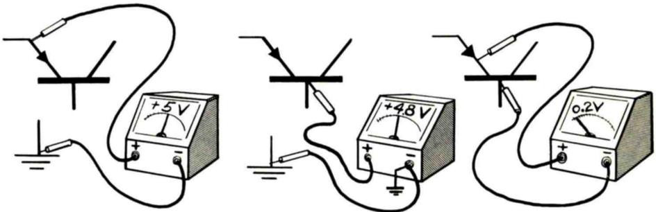
To Determine the Forward Emitter Bias, Measure the Separate Voltages at the Emitter and Base, Both with Respect to Ground. The Difference in the Readings is the Forward Bias. This is Usually More Accurate than a Reading Secured Directly Between the Emitter and Base.
