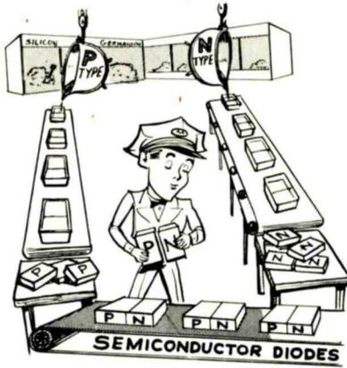
Adjoining Layers of P and N Semiconductor Materials Produce a P-N Junction: this is a Semiconductor Diode.
