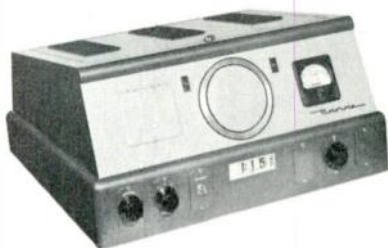
A Typical "Desk Top" Base Station Used for Two-Way Communications.
