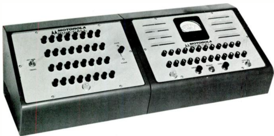
Here We See the 32-Button Accessory Box Connected to the Quik-Call Console.
