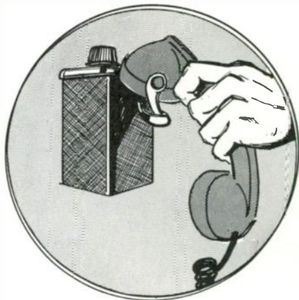
Lifting the Handset from the Hang-Up Box Stops Quik-Call Operation and the Receiver Operates in a Normal Manner.
