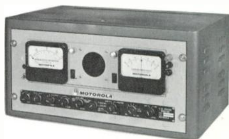
In Addition to Monitoring a Desired Channel, the Motorola Monitor Measures Transmitter Frequency and Deviation.
