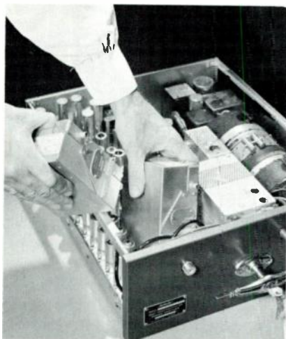
The Permakay Filter in the Motorola Receiver May Be Easily Replaced.
