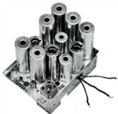
Some Receivers Are Made Up of Subchassis. Here We See an RF and High-Frequency Oscillator Deck.
