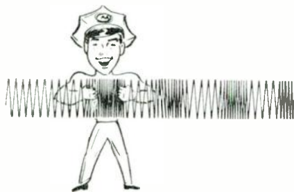
A Strong Audio Modulating Signal Causes Large Frequency Changes in the Carrier.
