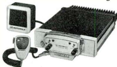
A Modern, Low-Drain Two-Way Radio Having a Completely Transistorized Receiver and Power Supply.
