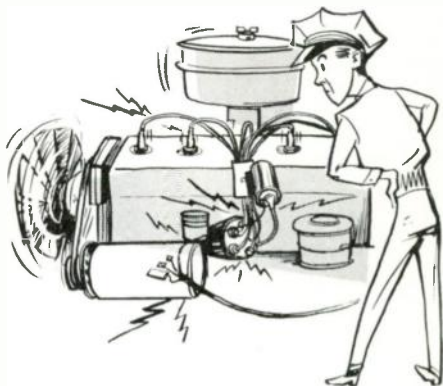
Noise Produced by Ignition Systems Often Interferes with Mobile Two-Way Radio Communications.
