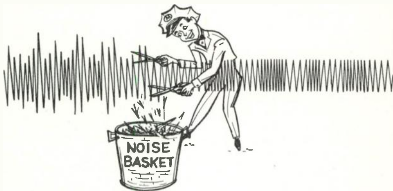
Limiting Removes All of the Noise Peaks from the Waveform, Thereby Producing a Constant-Amplitude IF Wave.
