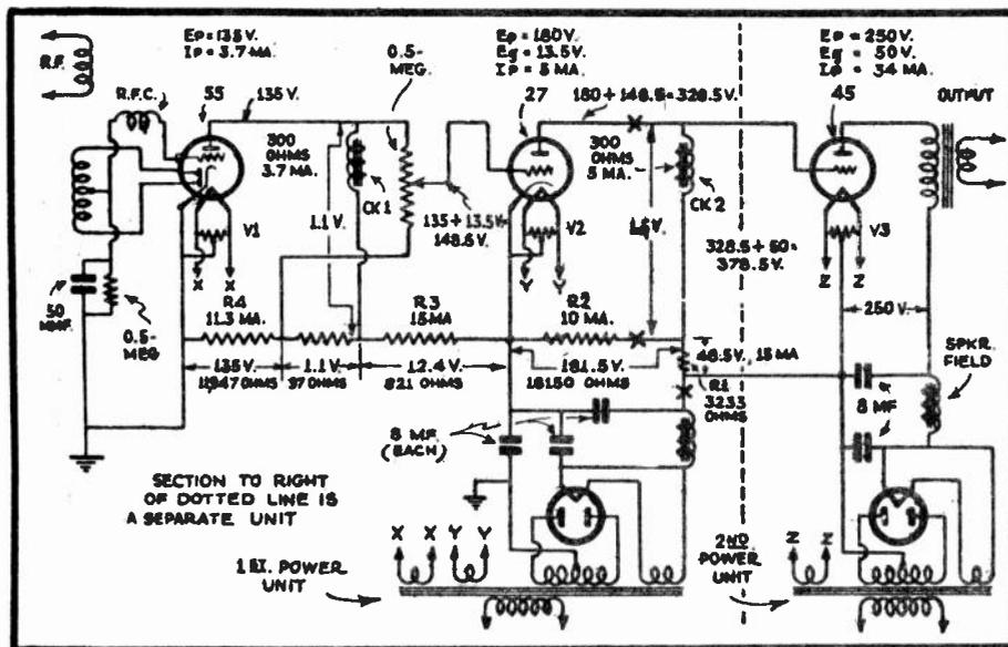
STAGE BY MEANS OF DIRECT COUPLING. SINCE THE AMPLIFYING HALF OF THE 55 TUBE IS DIODE BIASED, THERE IS NO NEED FOR AN AUDIO BY-PASS CONDENSER AND THIS MAKES IT POSSIBLE TO REALIZE A BETTER TONE QUALITY.
