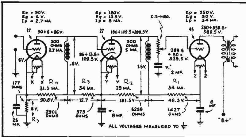
IN FIG. 4 YOU ARE SHOWN HOW THREE STAGES MAY BE CONNECTED TOGETHER BY DIRECT COUPLING AND HOW THE VOLUME MAY BE CONTROLLED IN SUCH A SYSTEM.
