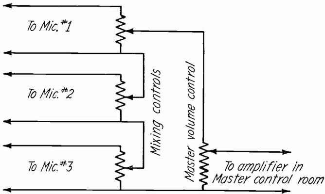
FIG. 5. Schematic Circuit of Mixing and Volume Controls in Monitoring Control Room.
