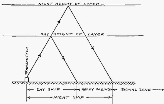
Fig. 7.—Action of the Heaviside Layer in Producing Skip Zones.
