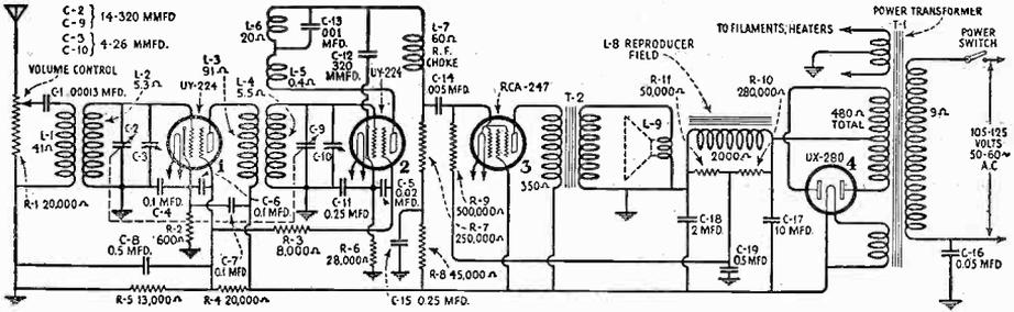
Figure 1—Schematic Circuit Diagram of Model R-5
