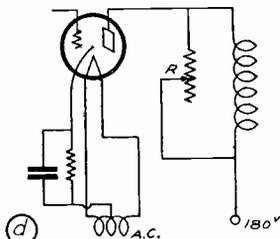
By means of 0-5000<sup>Ω</sup> resistance across primary of r.f. transformer
