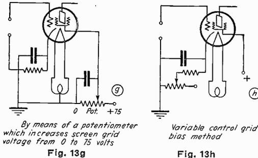
a fixed resistor is placed in series with the variable resistor. This method may be used with any tube and is highly recommended.
