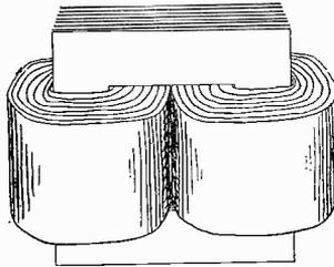
Fig. 14—Core type transformer and winding arrangement.
