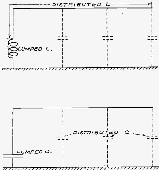
Fig. 9.—"L" Type Antenna Systems Showing Lumped and Distributed Constants.
