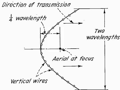
Fig. 20.—View of Parabolic Screen With Radiating Antenna.
