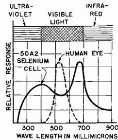
FIG. 9C. Color Response Curve of Acousto-Lite Laboratories Type 50A2 selenium cell.
