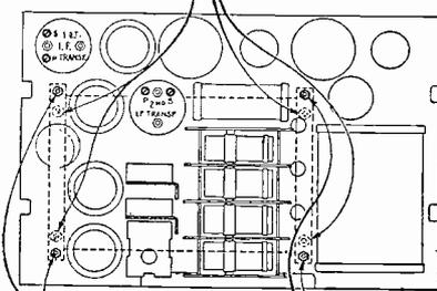
REMOVE FOUR NUTS & LOCKWASHERS TO REMOVE COIL ASSEMBLY.
