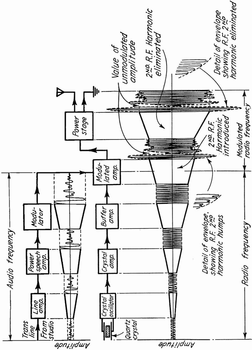
Fig. 13. Functions of Units in a Modern Broadcast Transmitter.
