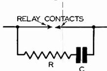
FIG. 13A. A condenser and resistor in series across relay contacts tend to prevent sparking at these contacts.
