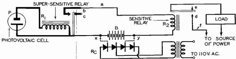
FIG. 15. Typical photovoltaic cell circuit using two relays.
