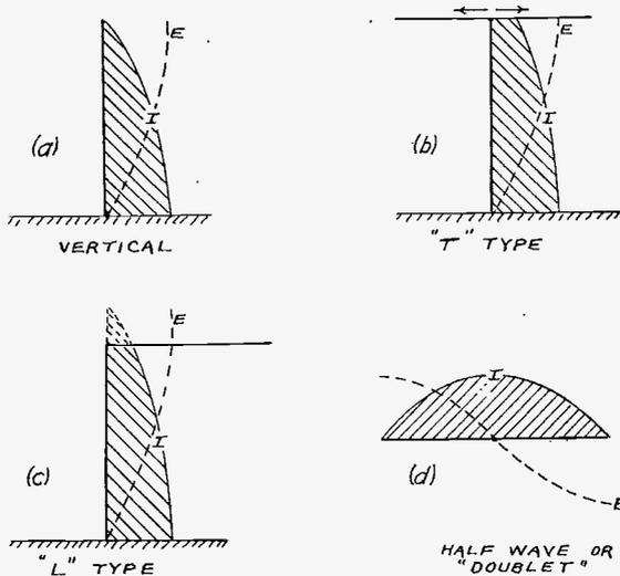
Fig. 3.—Current and Voltage Distributions of Various Antenna Types.
