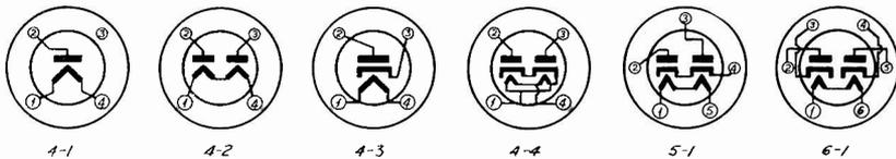
Pin Arrangement—Base Numbers; Bottom view of tube connections
