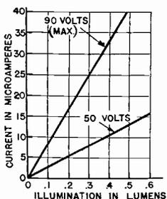
FIG. 6A. Current-Illumination Curves for a typical gas type photocell (General Electric PJ-23 Phototube).
