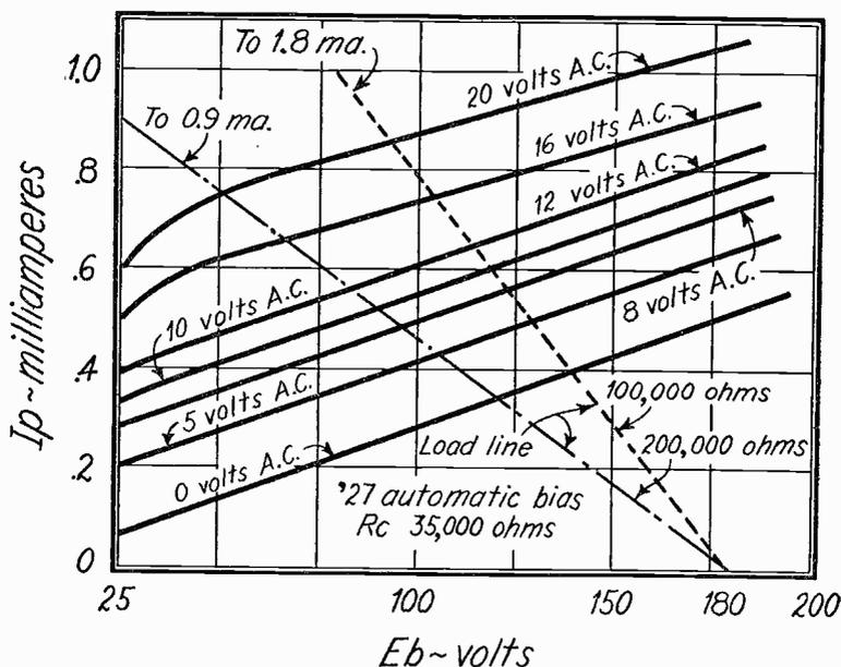
Fig. 14—Characteristics of a typical automatic bias detector of the '27 type.
