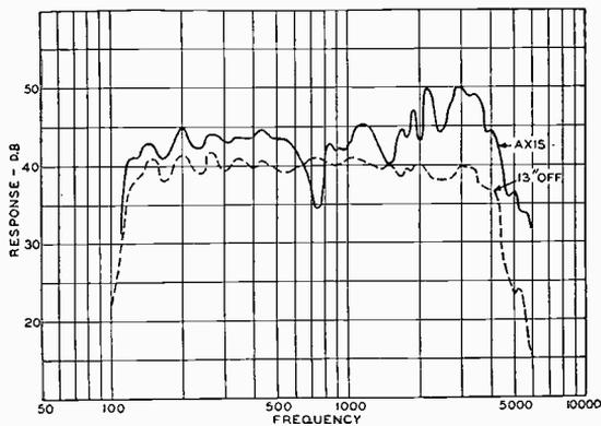
Fig. 12.—Curve marked axis is for sound in front of the cone, 13" indicates the condition 13 inches away from the cone rim.
