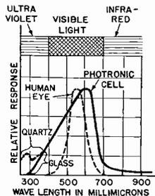
FIG. 13C. Color Response Curve for Weston Photronic Cell.
