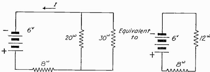
Fig. 11—A combination series-parallel arrangement of resistances.
