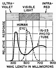
FIG. 6C. Color Response Curve for General Electric PJ-23 phototube. Note peak in ultra-violet region.
