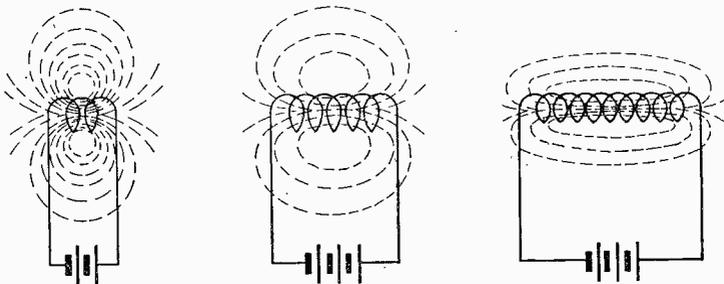
Fig. 3—Magnetic fields around different shape coils carrying a current.
