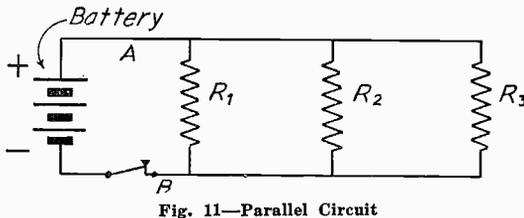
Fig. 11—Parallel Circuit
