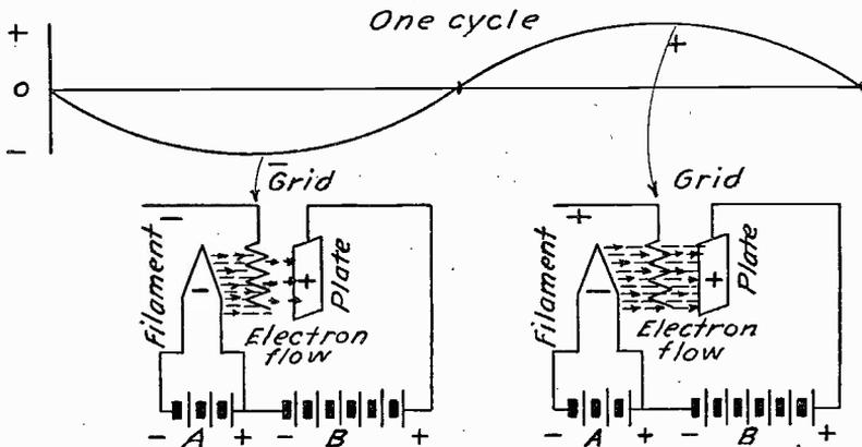
Fig. 13—Illustrating the effect on the electron flow in a vacuum tube when a negative and positive potential is placed on grid.
