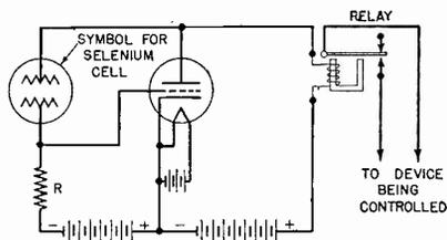
FIG. 8B. Basic circuit for a selenium (photoconductive) cell. Note symbol used to represent this cell.
