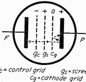
Fig. 13—Illustration showing how the three grids of a pentode tube are arranged.
