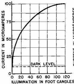
FIG. 9A. Current-Illumination Curve for Acousto-Lite Laboratories Type 50A2 selenium cell.
