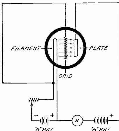
FIG. 1.—Filament, Grid and Plate Circuits of a Triode
