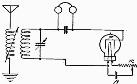
Fig. 7—Receiving circuit using a Fleming valve as a rectifier.
