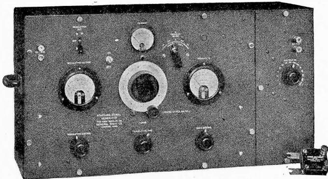
Fig. 6—Typical commercial size generator used in making selectivity, sensitivity and over-all fidelity receiver curves.
