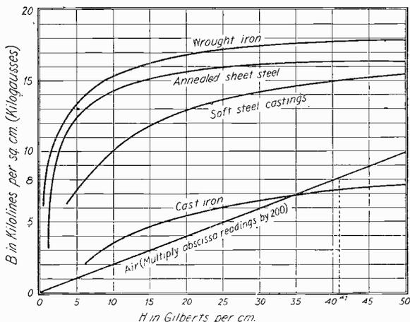
Fig. 10—Characteristic curves of magnetization, or B-H curves \*
