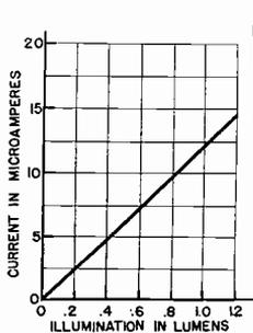
FIG. 5A. Current-Illumination Curve for a typical vacuum type photocell (Westinghouse SR-50 phototube).
