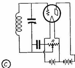
By means of 400<sup>Ω</sup> potentiometer in grid return of r.f. tube
