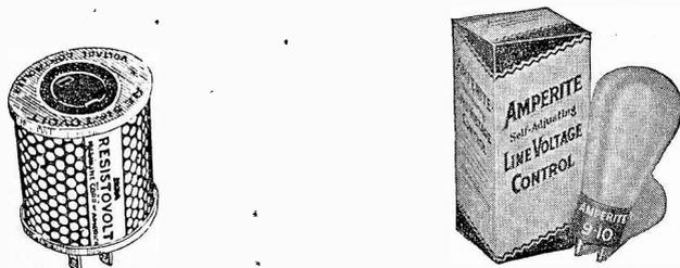
Fig. 26—Typical line ballast resistor which works on the principle that "increased current causes more heat in the resistance element thereby increasing the ballast resistance, resulting in a decrease of line current."
