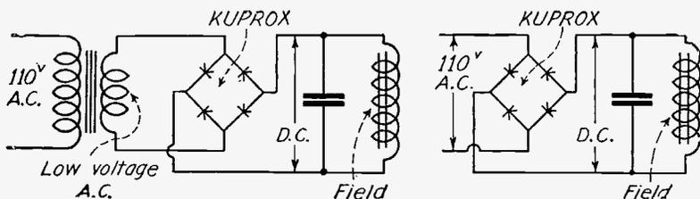
Fig. 26—Step Down and Direct Voltage Supply for A. C. Dynamic Speakers
