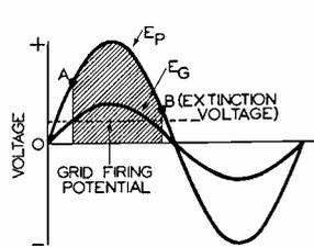
FIG. 21B. When plate and grid voltages of the KU-610 grid-glow tube are in phase, plate current passes for that part of a cycle shown shaded.
