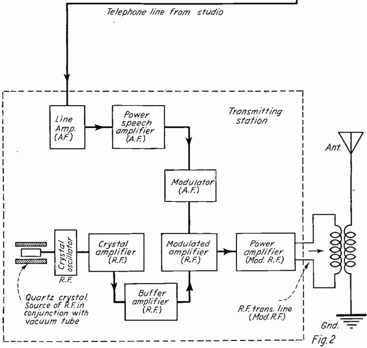
FIGS. 1 and 2. Block Diagrams of Program and Transmitting Circuits for a Typical Broadcast Station.
