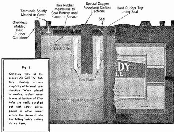
FIG. 1.—Air Cell “A” Battery
