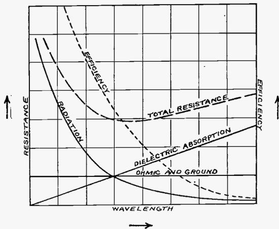
Fig. 11.—Composition of the Total Antenna Resistance at Various Wavelengths and Relative Efficiency.
