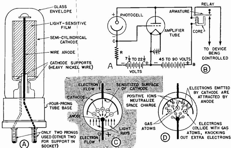
FIG. 4. The construction, the schematic symbol, the theory of electron flow in both gas and vacuum type tubes, and the diagram of an amplifier circuit for a typical photoemissive cell are given here.
