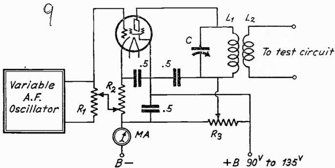
Fig. 27.—Dynatron oscillator circuit in which the percentage of modulation may be varied.
