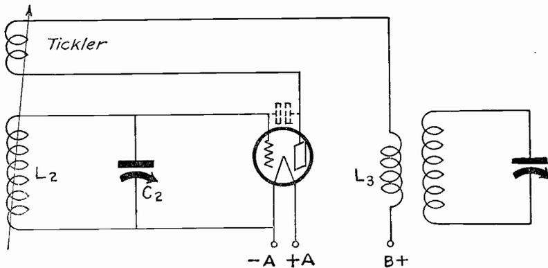
Fig. 13. Regenerative Circuit showing Variable Coupling between Tickler and  $L_2$ ,
