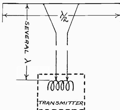
Fig. 17.—Doublet With Voltage Feed.
