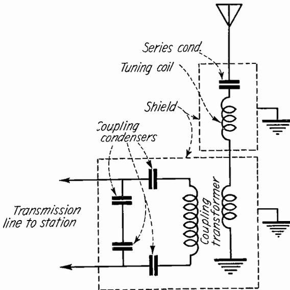
FIG. 16. Schematic of Coupling House Circuits.
