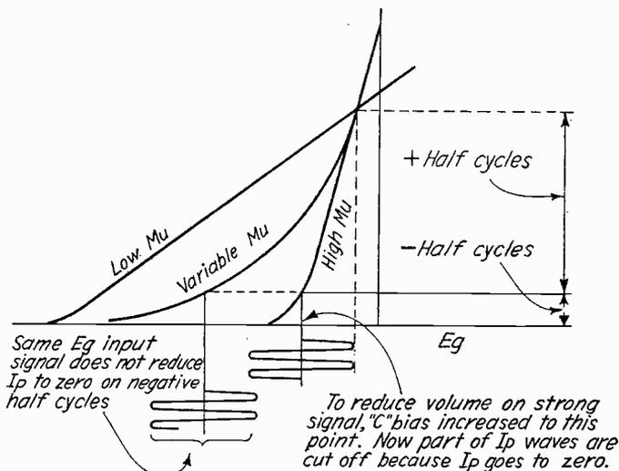
Fig. 15—Comparison of characteristics of high mu tube, low mu tube and variable mu tube. Note the gradual slope and wider grid voltage range of the variable mu tube.
