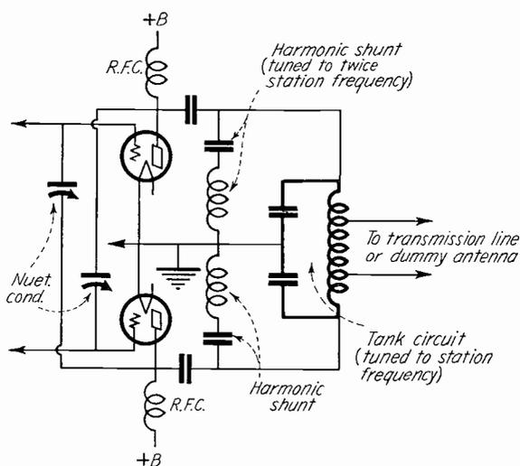
FIG. 14. Schematic of Last Power Stage.
