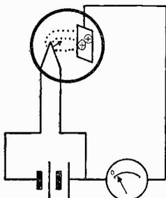
Fig. 2—Illustrating the electron emission from a heated filament to plate of vacuum tube.
