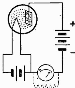
Fig. 3—Illustrating the result of electron emission when a positive charge is placed on the plate.
