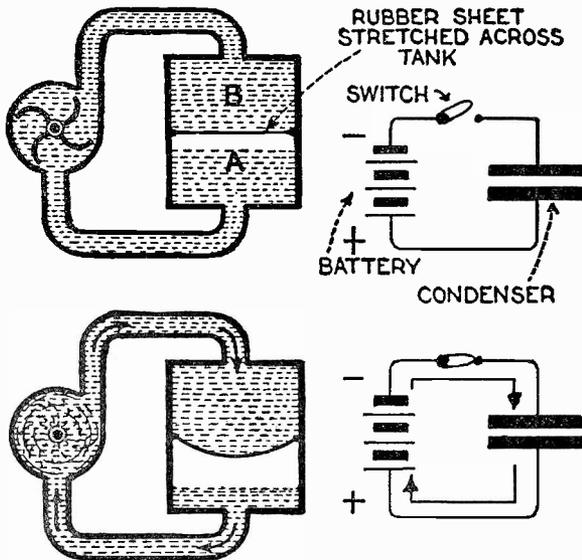
Fig. 7—Hydraulic Analogy Showing How a Condenser Is Charged With Direct Current
