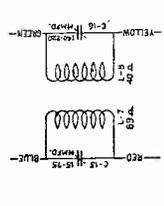
INTERNAL CONNECTIONS OF 2ND I.F. TRANSFORMER
