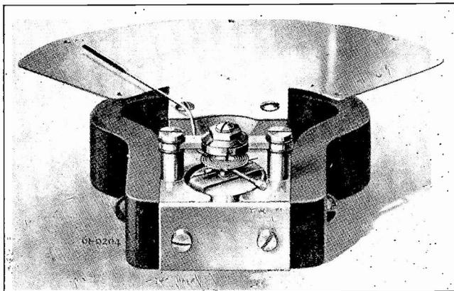
FIG. 8. D'Arsonval D.C. ammeter with case removed
