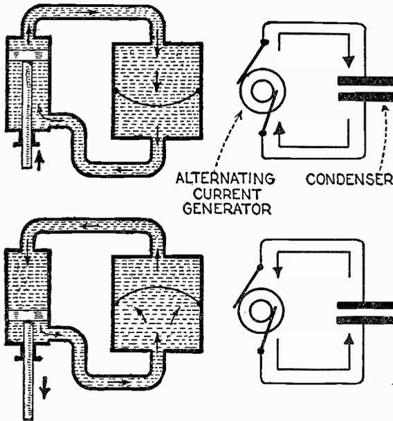
Fig. 8—Hydraulic Analogy Illustrating the Flow of Alternating Current Through a Condenser.
