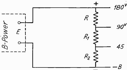
Fig. 13—A voltage divider.
