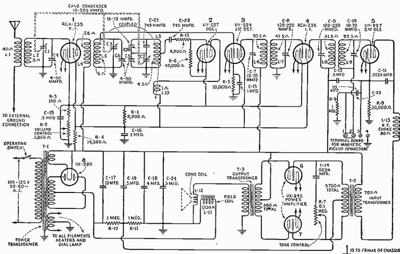
Fig. 17 (a).—Schematic wiring diagram of a typical superheterodyne receiver showing preselector and R.F. amplifier, oscillator, first detector, I.F. amplifier, second detector, push-pull power amplifier and power supply.
