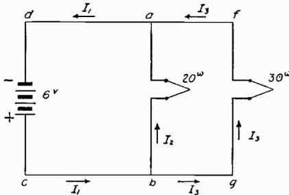
Fig. 8—Two resistances in parallel.
