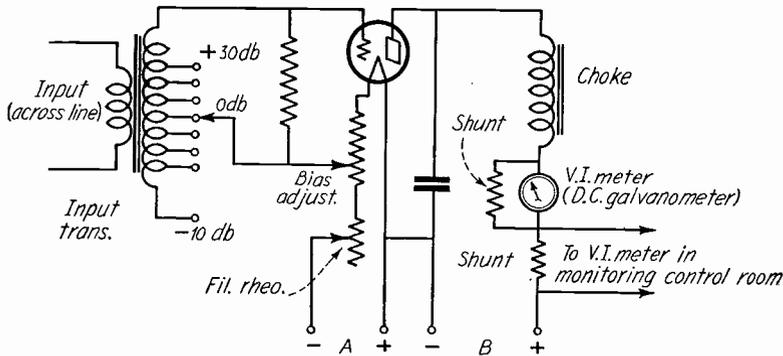
FIG. 9. Schematic Circuit of Volume Indicator.
