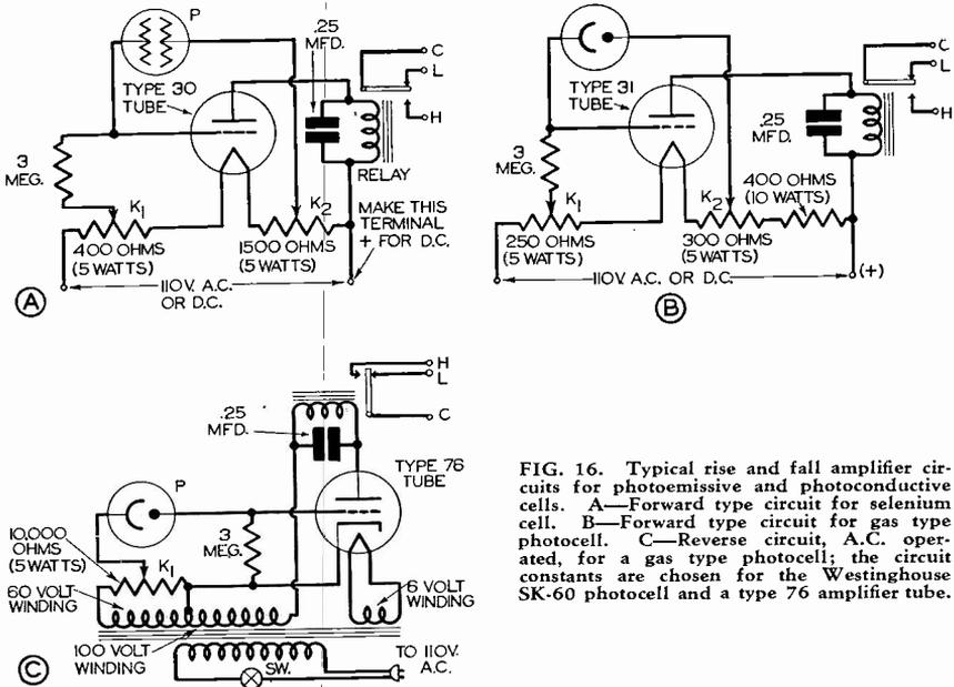
FIG. 16. Typical rise and fall amplifier circuits for photoemissive and photoconductive cells. A—Forward type circuit for selenium cell. B—Forward type circuit for gas type photocell. C—Reverse circuit, A.C. operated, for a gas type photocell; the circuit constants are chosen for the Westinghouse SK-60 photocell and a type 76 amplifier tube.
