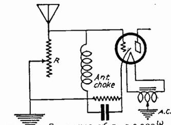
By means of a 0-2,000<sup>Ω</sup> resistance across aerial and ground
