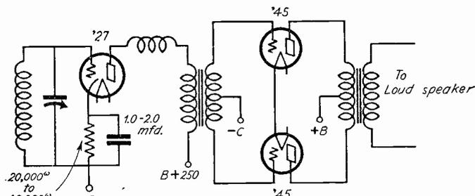
Fig. 12—Circuit of a '27 detector working into a push pull stage.
