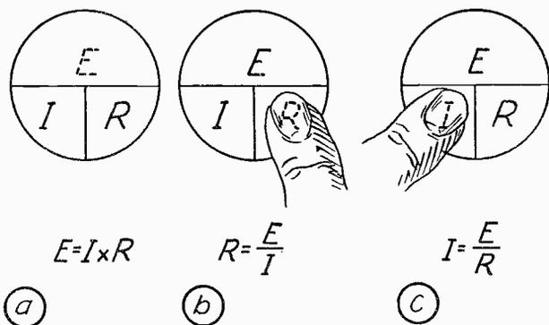
Fig. 3—A simple method for using Ohm's Law in three forms.
