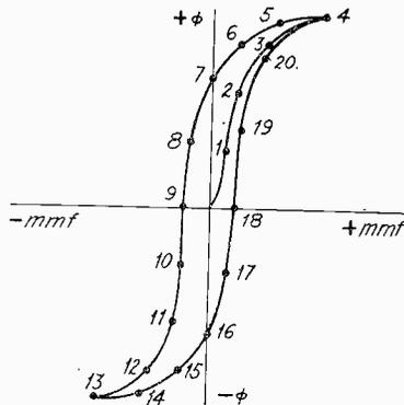
Fig. 13—Typical cycle of magnetization called a hysteresis loop
