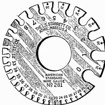
Fig. 15—A pocket wire gauge which can be purchased from any hardware store handling copper wire.
