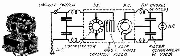
FIG. 23.—The rotary converter, employing a D.C. motor and an A.C. generator winding in the same armature slats. Filter housed in the steel box supporting the rotary converter. Input and output spark filters used.
