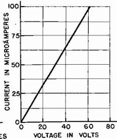
FIG. 9B. Current-Voltage Curve for Type 50A2 selenium cell (with constant illumination).
