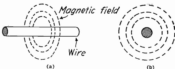
Fig. 1—Magnetic Effect Around a Wire When Current Is Flowing.
