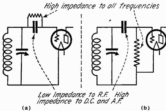
Fig. 17—Two methods of connecting the grid leak in a detector circuit.
