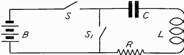
Fig. 12—Fundamental Oscillatory Circuit.
