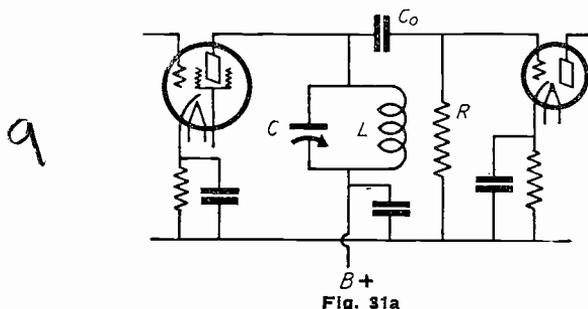
fore, circuit shown in Fig. 31a may be looked upon as an R.F. resistance coupled stage. Condenser  $C_0$  is small as at R.F. frequencies its reactance is low. Quite often  $C_0$  is a small book type adjustable condenser or merely two insulated wires from plate to grid twisted together at the ends, but not making metal contact.
