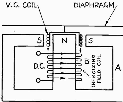
Fig. 6—Moving Coil Unit
