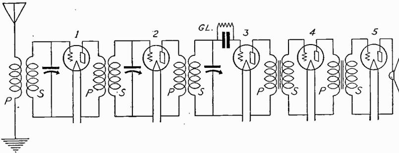
Fig. 21—The circuit of a five tube receiver employing two stages of tuned radio frequency amplification (1 and 2), a detector (3) and two stages of Audio frequency Amplification (4 and 5)
