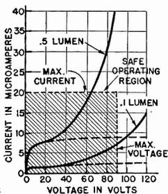
FIG. 6B. Current-Voltage Curve for General Electric PJ-23 phototube, for two different values of illumination.
