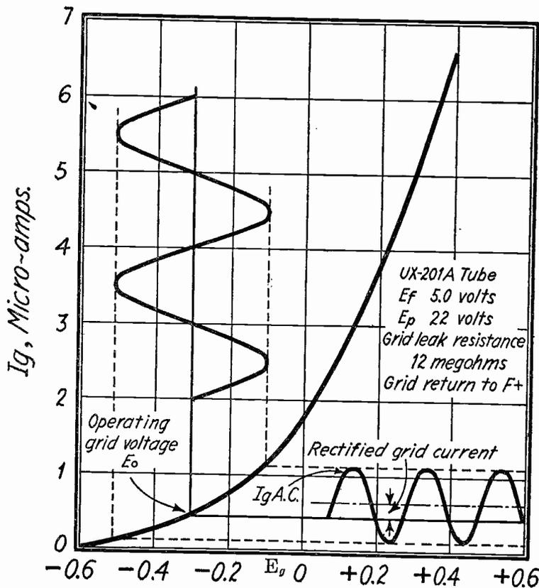
Fig. 15—Grid current-grid voltage characteristic of a tube showing how detection takes place in grid circuit.
