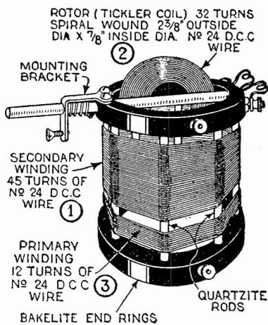
Fig. 6c—Three Circuit Tuner.
