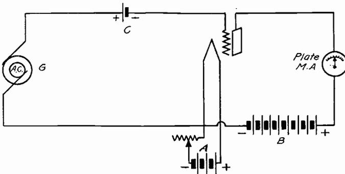
FIG. 4.—Diagram Showing an A.C. Generator (*G*) Connected to the Grid-Filament Input of a Vacuum Tube
