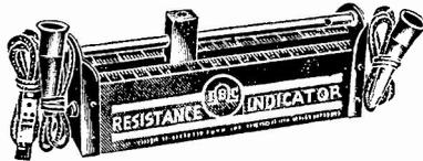
A calibrated adjustable resistor tester which enables a service-man to determine proper replacement values of defective resistors, measure unknown resistors by the substitution method, can be used as a calibrated variable resistor for adjusting voltage, as a potentiometer or voltage divider
