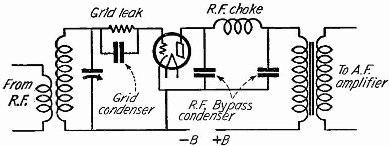
Fig. 16—Grid leak and condenser detector, which also acts as an audio amplifier.
