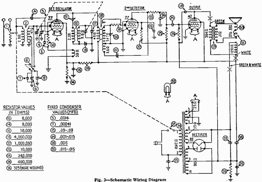
Fig. 2—Schematic Wiring Diagram
