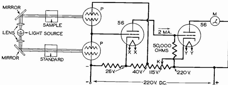
FIG. 19. Typical light differential circuit. The power supply is not shown, but should produce 400 volts D.C.; two separate 2.5 volt secondary windings are needed for XX and YY to prevent leakage reaction between the two amplifier tubes.
