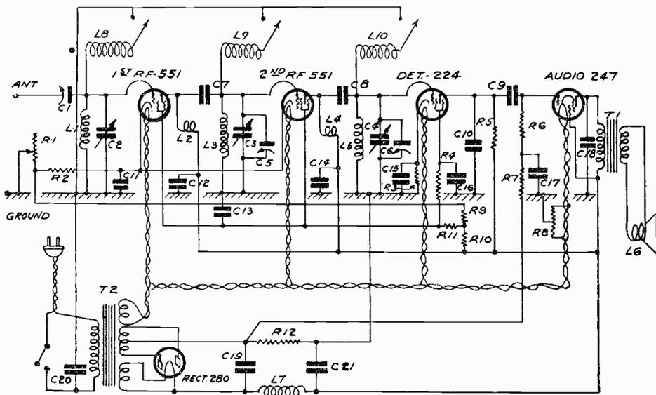
Schematic Diagram of Model 200 Receiver
