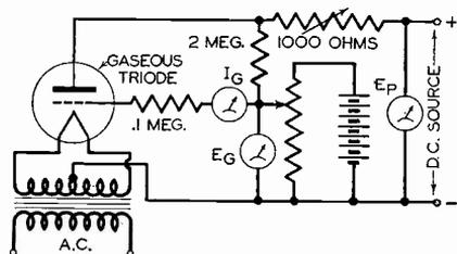
FIG. 20. Characteristic curves of a typical hot-cathode gas filled tube, the Westinghouse type KU-610 grid-glow tube. D.C. starting characteristics for rated anode current are given at the left; the test circuit used appears above.
