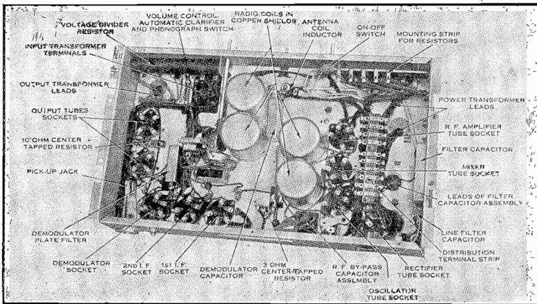
Fig. 2 (a).—Bottom view of the chassis of a typical superheterodyne receiving set with the cover removed.
