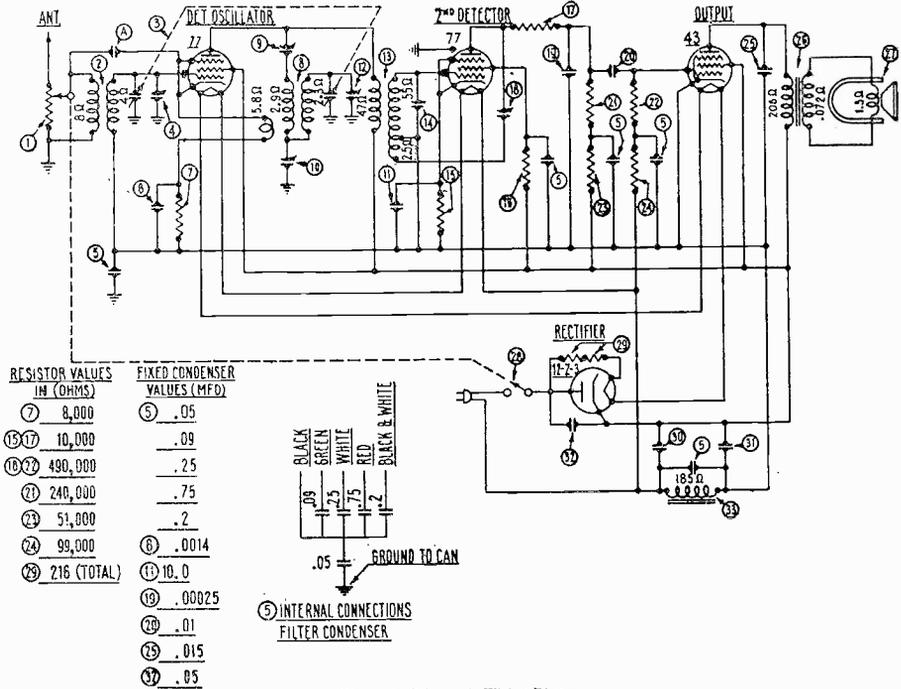
Figure 4—Schematic Wiring Diagram
