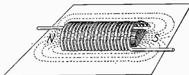
Fig. 6—Magnetic field of a coil of wire having an iron or steel core.
