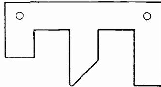
Fig. 17—Shape of one lamination.
