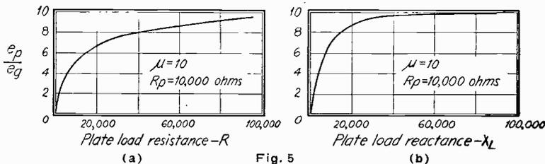
obtain an  $e_p/e_g$  ratio which is 90% of  $\mu$ , the inductance of the load must be, from the formula,  $X_L = 2\pi fL$ :
