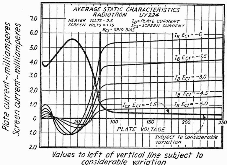
Fig. 6—Plate voltage-plate current characteristics of a screen grid tube. It is worth remembering that the sum of the plate and screen grid current is a constant value for a given screen grid and control grid voltage. The total is the cathode current.
