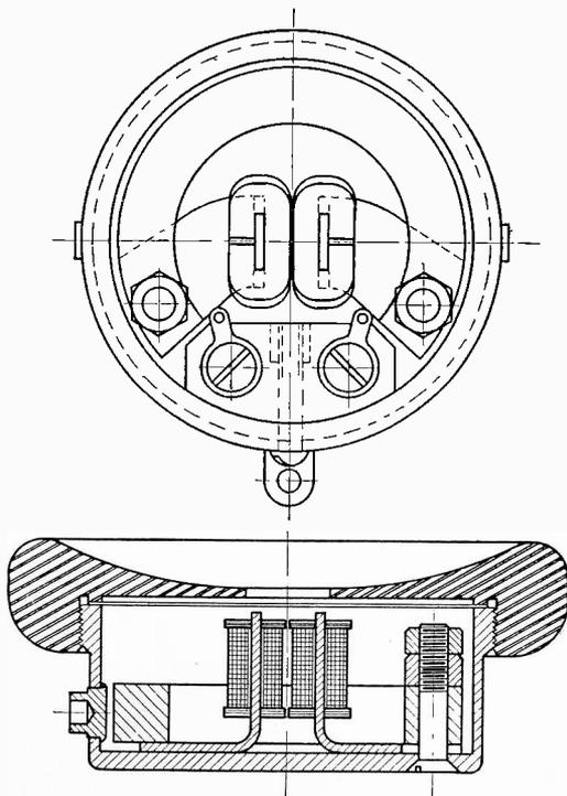
Fig. 1—Illustration Showing Details of the Bi-Polar Type Headphone Unit
