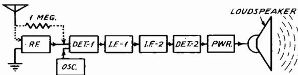
FIG. 2. Block diagram of signal circuits of a superheterodyne receiver. If pulling out *Det-1* produces a click and connecting the antenna to *Det-1* does not result in signals, the *OSC.* is probably defective.
