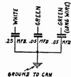
Fig. 3—Internal Connections Filter Condenser
