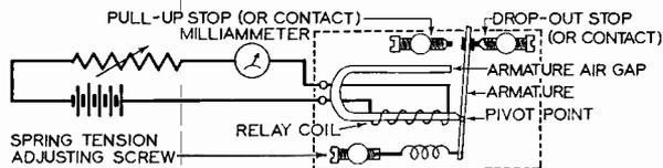
FIG. 14. Test circuit for sending required current through the coil of a sensitive relay when making adjustments.
