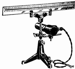
Scale and lamp for semi-portable galvanometer
