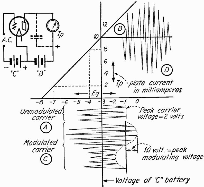
Fig. 2—Modulated and unmodulated carrier signals applied to an amplifier produces in the output a current wave exactly similar to the input voltage wave.
