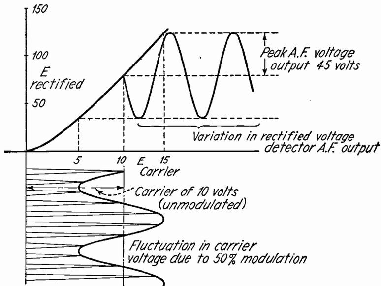
Fig. 12—How modulation of a carrier applied to a linear detector produce modulating frequency currents in the output.
