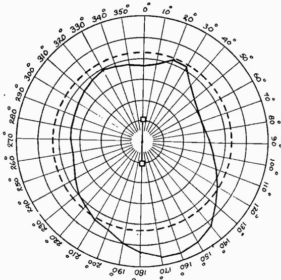
Fig. 8.—Actual and Ideal Field Patterns of a Broadcasting Station.
