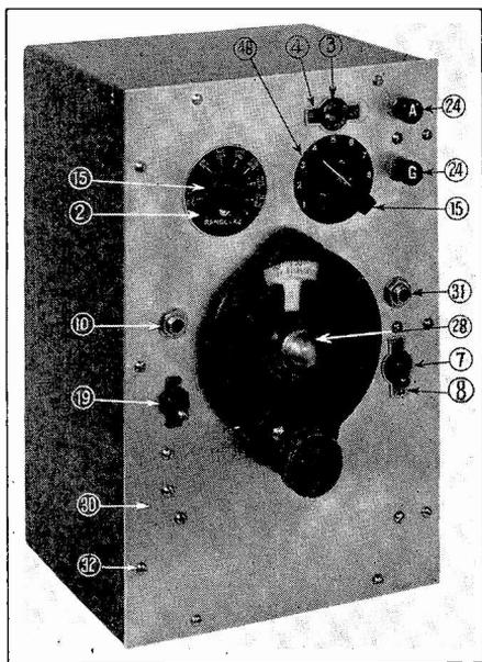
FIG. 1. The completed signal generator, designed and built in the N. R. I. Laboratory, fits into 7" x 10 $\frac{3}{4}$ " x 5 $\frac{1}{2}$ " cabinet.
