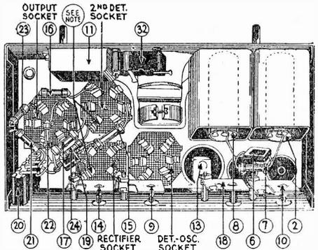
Fig. 3—Bottom View of Chassis, Showing Parts
