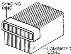
FIG. 6. In order to prevent chatter when relays are operated on A.C., a heavy copper shading ring like that shown here is forced into a slot cut into that end of the laminated iron core which faces the armature.
