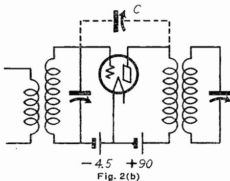
this internal capacity was the screen grid tube. And now that screen grid tubes are so well known and their operation is so clearly understood, it seems strange that the solution was not thought of long ago.
