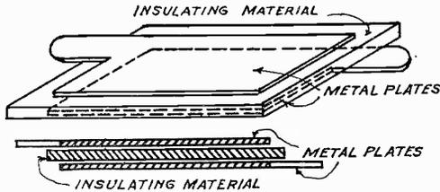
Fig. 1—Constructional Details of a Simple Condenser.
