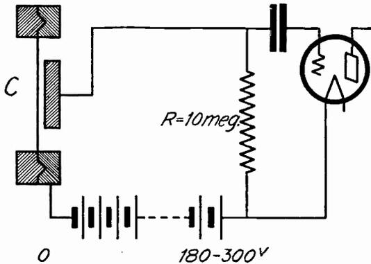
Fig. 4. Schematic Circuit of Condenser Microphone and First Stage.
