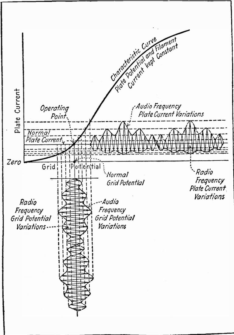
Fig. 4—Detection of sound modulated carrier signal.
