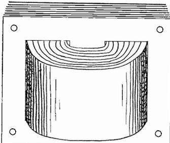
Fig. 16—Shell type transformer.
