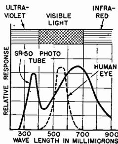
FIG. 5C. Color Response Curve for Westinghouse SR-50 phototube, with response of human eye shown for comparison.
