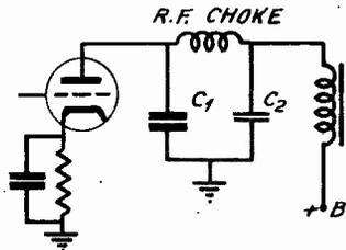
FIG. 3F. If  $C^1$  is shorted, the choke coil may burn out. In this case both  $C^1$  and the choke must be replaced.
