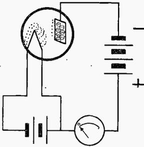
Fig. 4—Illustrating the result of electron emission when a negative charge is placed on the plate.
