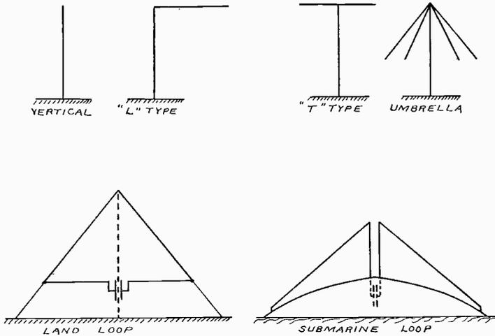
Fig. 1.—Schematic Diagram of Transmitting Antenna Types.
