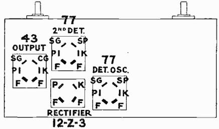
F Filament      SG Screen Grid      K Cathode
