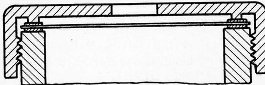
Fig. 12—Illustration Showing How Rubber Gaskets Are Used in Place of the Rubber Tubing
