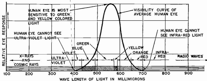
FIG. 3. The relative sensitivity of the average human eye to light of various colors (various wavelengths) is given by this curve.
