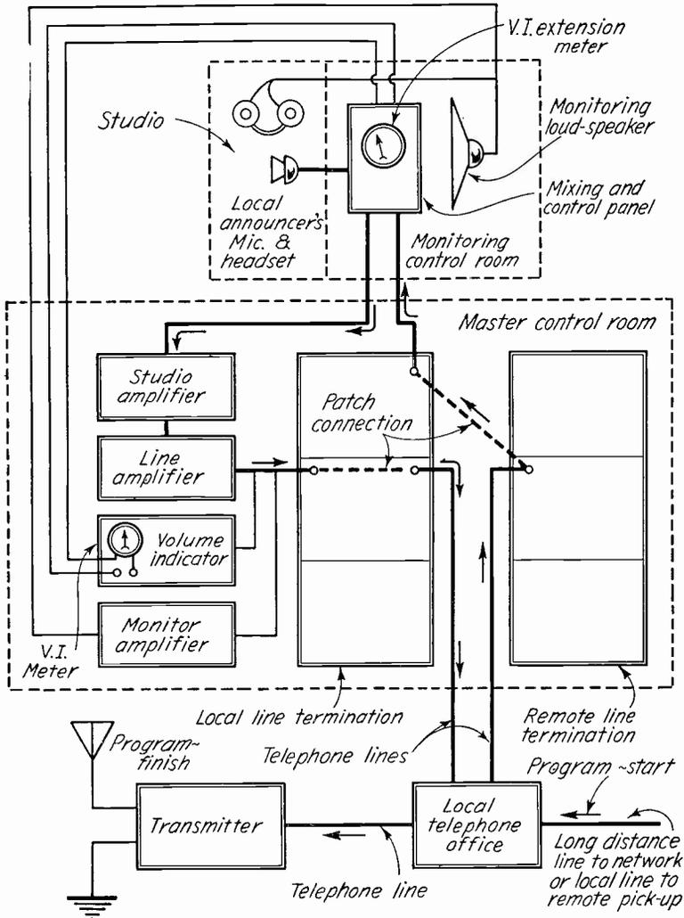
FIG. 7. Setup for Network or Remote Program.
