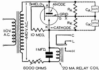
FIG. 23. Basic operating circuit for the Westinghouse KU-618 grid-glow tube. A photoemissive cell or a photoconductive cell of high resistance can be substituted for either of the resistors or condensers connected to the grid. The arrow in the tube symbol represents the cold cathode.
