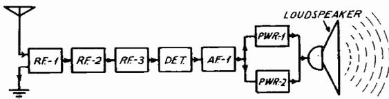
FIG. 1. Block diagram of signal circuits of a T.R.F. receiver.
