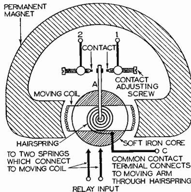
FIG. 1A. The basic construction of a super-sensitive or meter type relay, shown above, is very similar to that of a high quality moving coil type meter.
