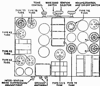
Fig. 1—Top View of Chassis, Showing Tube Locations and Major Parts
