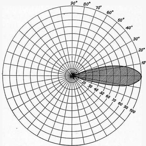
Fig. 21.—Field Patten of Beam Radiation.
