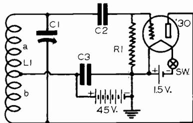
FIG. 8. Circuit for test oscillator.
