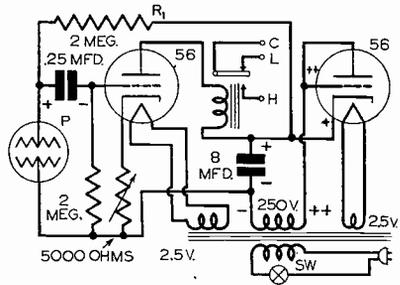
FIG. 17B. Another form of impulse circuit, which uses an extra tube to secure D.C. Here the relay pulls up only when light on the cell is suddenly interrupted, and drops out automatically in a definite time interval. Current flows through the tube circuits only during the half of each cycle for which polarity is as indicated.
