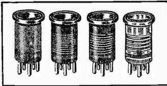
Fig. 16—Above are shown modern plug-in coils used in all-wave receivers, when the receiver is to be used on different radio bands. Each section requires a plug-in coil for each band of frequencies. If two tuning circuits are involved, and tuning in four frequency bands is wanted, eight plug-in coils are required.
