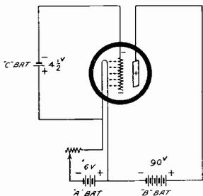
FIG. 2.—This Diagram Illustrates the Action of the Negative Charge on the Grid.
