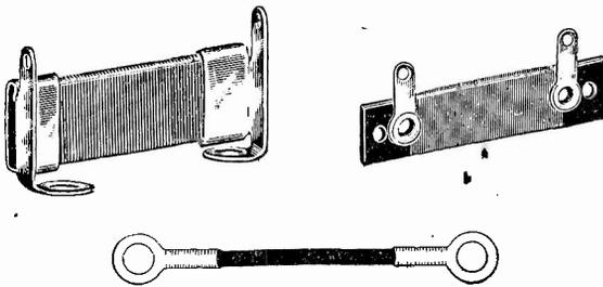
Fig. 20—Low power wire-wound fixed resistors.
