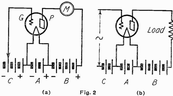
range and for each different value of grid voltage the plate current is observed on a plate milliammeter M. The experimental data thus obtained is plotted in the form of a curve which will appear as shown in Fig. 2c. Such a curve is known as the plate current-grid voltage static characteristic curve of a vacuum tube and gives a complete picture of the effect of input grid voltage change on plate current change for a given plate voltage.
