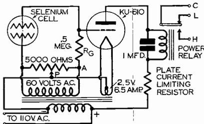
FIG. 21A. A practical photoconductive cell circuit, using a Westinghouse type KU-610 grid-glow tube to operate a power relay directly. Circuit operates entirely from A.C.
