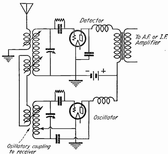
Fig. 18—A heterodyne detector. If the beat frequency is audible this circuit can be either a short or a long wave receiver. If inaudible it may be amplified again and detected to make it audible.
