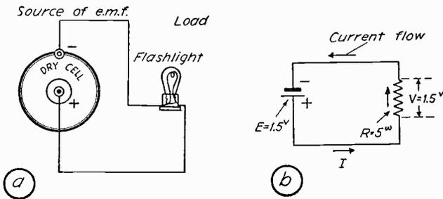
Fig. 1—A simple electric circuit.
