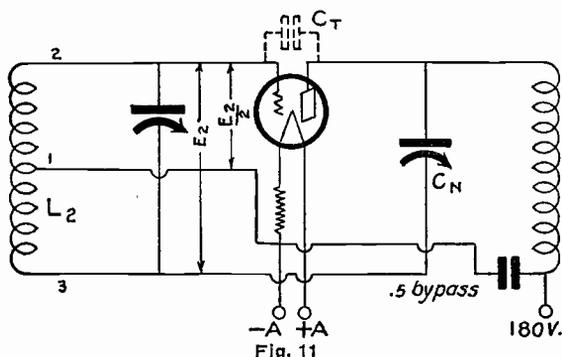
end, through the neutralizing condenser, to the plate. The capacity of the neutralizing condenser is equal to the tube capacity. The voltage across 1-2 is  $180^\circ$  out of phase with voltage across 1-3. Thus, any regenerative voltage fed back to the grid is exactly balanced by an equal and opposite voltage. Any deviation from a condition of voltage balance will cause oscillation.
