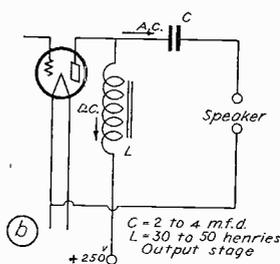
Fig. 16b—Output Stage.
