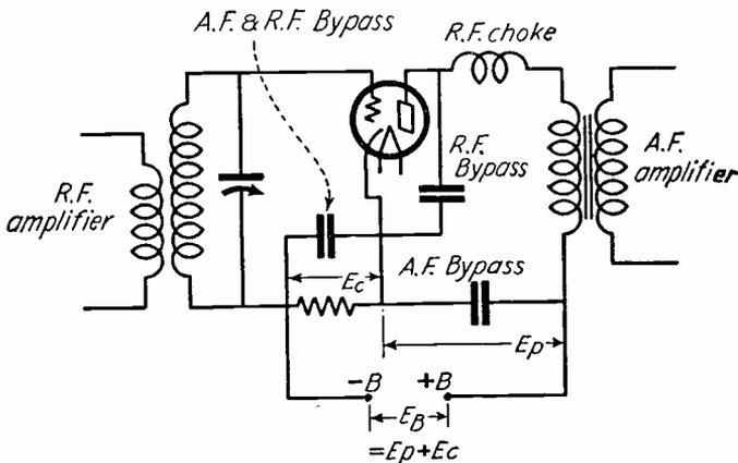
Fig. 13—Typical circuit diagram of an automatic or self-biased detector.
