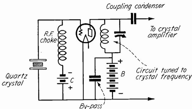
Fig. 12. Crystal Oscillator Circuit.
