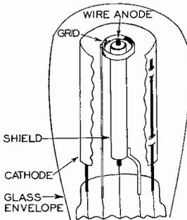
FIG. 22. Cut-away view of a cold-cathode grid-glow tube, showing arrangement of electrodes. The anode is inside a porcelain tube which in turn is surrounded by a metal cylinder, the shield. The grid is simply a thin band or ring of metal surrounding the exposed tip of the anode.
