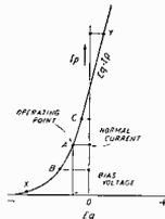
let us say a swing of 300 micro-volts. This is beyond the straight portion of the  $E_g-I_p$  curve and plate rectification takes place, just as in a detector tube.
