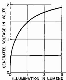
FIG. 13B. Voltage-Illumination Curve for Weston Photronic cell.
