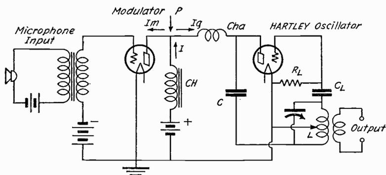
Fig. 18.—Modulated R.F. oscillator using Heising system of plate modulation.\*
