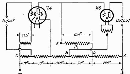
Fig. 10—Circuit showing direct coupled audio amplifier.
