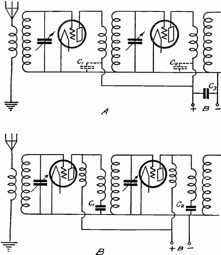
Fig. 5. A. shows a Two Stage R.F. Amplifier with Series Connection for "B" Supply. B. shows the Shunt Connection for "B" Supply.
