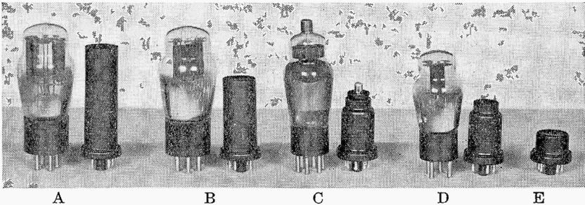
Fig. 25—Four glass-enclosed Radio receiver tubes and corresponding metal-enclosed tubes; and on extreme right "Duo-Diode" tube, available only in metal envelope.
