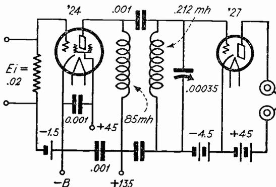
Fig. 7—A stage of screen grid R.F. working into a triode C bias detector.
