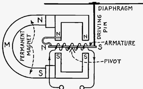
Fig. 4—Balanced Armature Type Unit
