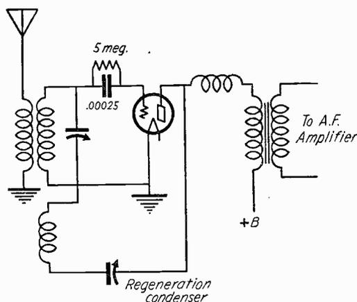
Fig. 19—An autodyne in which the beat frequency is produced in the detector itself.
