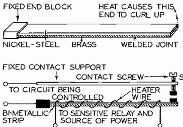
FIG. 12A. Basic principles of the bi-metallic strip type time delay relay are illustrated here. The four connections shown to the relay are often reduced to three by attaching one heater wire to the bi-metallic strip.
