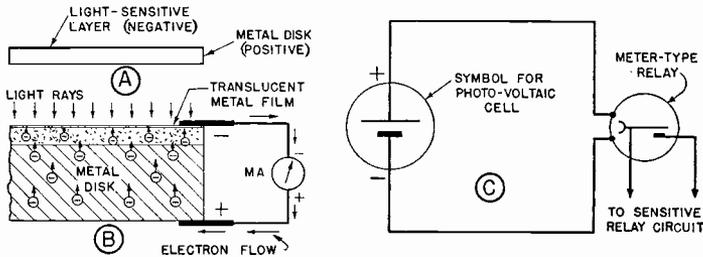
FIG. 11. Basic construction of and basic circuit for the dry photovoltaic (self-generating) cell.
