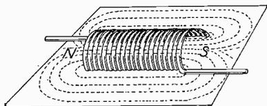
Fig. 5—Magnetic field of an air core coil.
