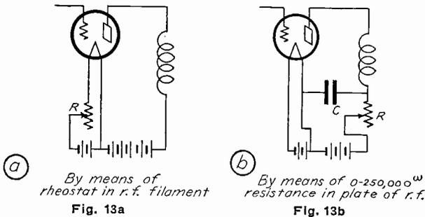
cause of possible distortion and reduced selectivity. Method (d) could be used in place of this. It is not advisable to control volume in audio systems by this method (a) because of the distortion that results. Filaments in A.C. and D.C. sets should be operated at normal, constant voltage.
