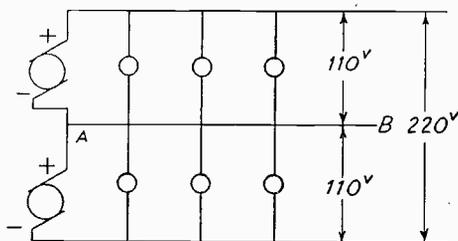
Fig. 13 (b)—Three-wire Transmission System
