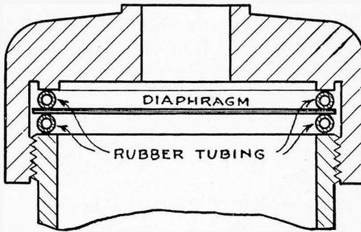
Fig. 11—Illustration Showing How Two Rubber Tubings Are Placed on Each Side of the Diaphragm
