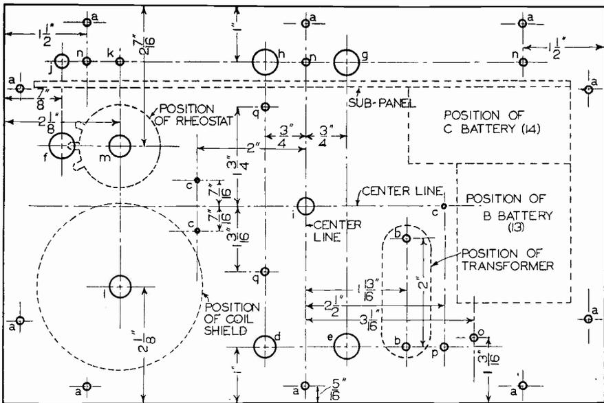
Fig. 2. Layout for 10-13/16" x 7-1/16" aluminum front panel (front view). Refer to dotted lines when mounting parts on the panel. Locate holes "a" 5/16" from outside edges and 1 1/2" from nearest corner.
