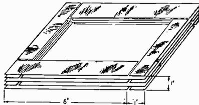
Fig. 15—Illustration showing how a core is built up.
