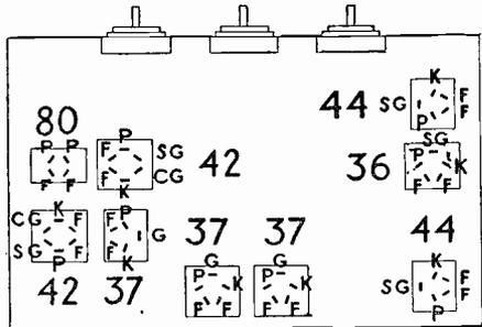
F = Filament      SG = Screen Grid      K = Cathode
