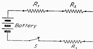
Fig. 10—Series Circuit
