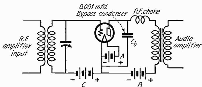
Fig. 8—Detector of the C-bias type.
