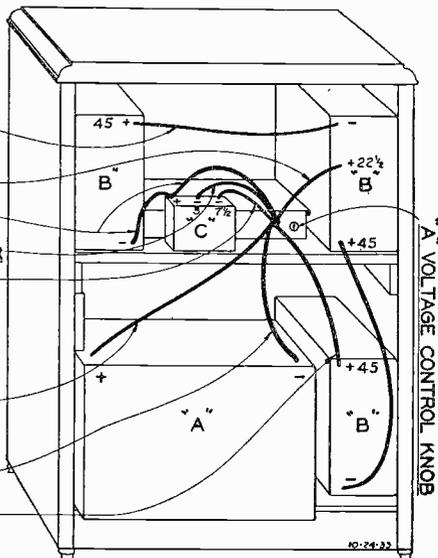
**SPARTON MODEL 82 WIRING DIAGRAM**
