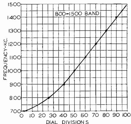
FIG. 9. Sample S.G. calibration chart.
