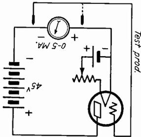
*Theory of Operation:* The fact that current in the grid causes clicks in the phones does not require explanation here. However the effect of a resistance in the grid circuit should be thoroughly understood. Unless there is current flowing through a resistor there is no voltage drop across it. In receivers we often see very high resistances in the grid circuit.
