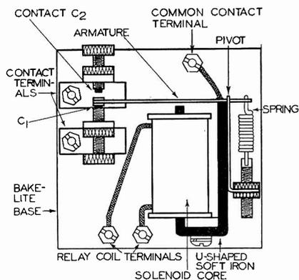
FIG. 3A. Sketch showing construction of a typical sensitive relay. The common contact terminal connects to the armature.
