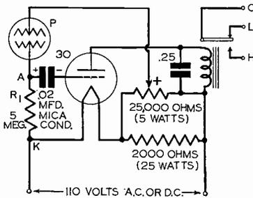
FIG. 17A. One form of the impulse circuit, using a selenium cell and a type 30 amplifier tube. The relay, normally closed, drops out when illumination on the cell is suddenly cut off. The relay remains pulled up for all constant values of illumination, and pulls up by itself at a definite time after each interruption of light.
