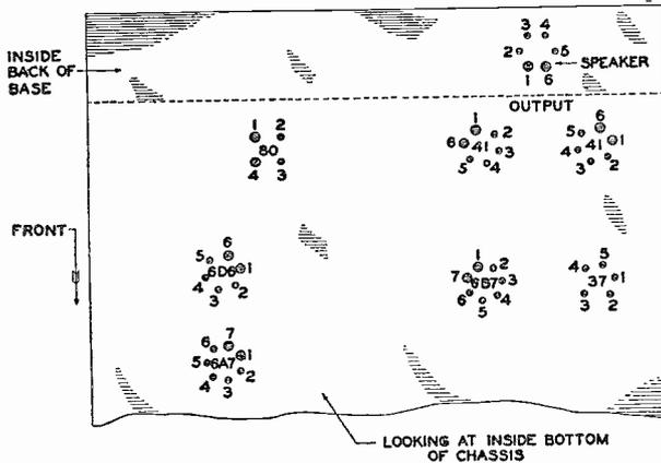
Fig. 2. Terminal Layout for Voltage Measurement Chart.
