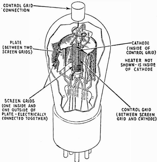
Fig. 4—Cross-sectional view showing the construction of an A.C. screen-grid vacuum tube.
