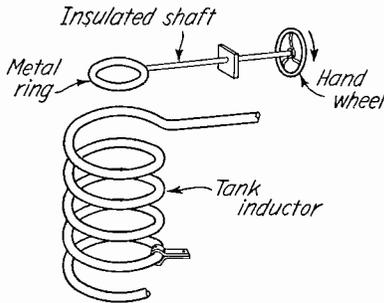
FIG. 15. Method of Tuning Power Tank Circuit.
