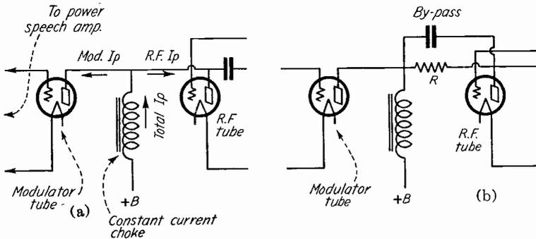
FIG. 11. Heising Modulation. Note: The filaments of the R. F. and Modulator tubes are fed from the same secondary supply.
