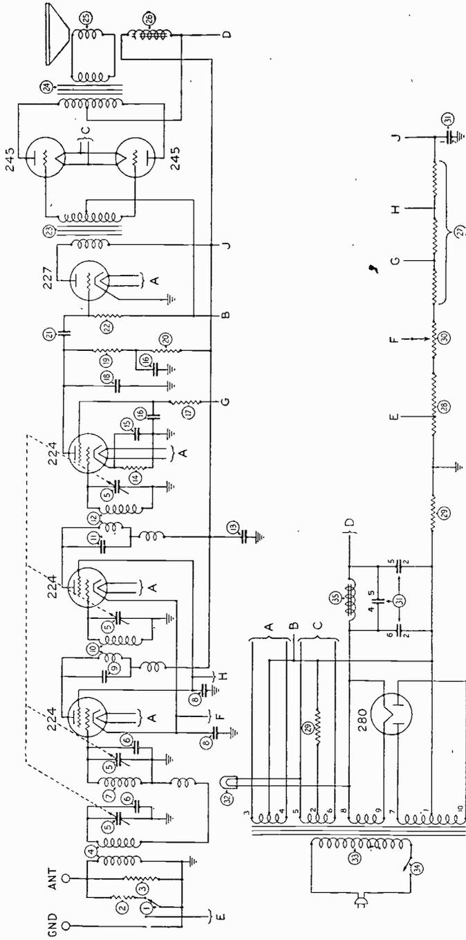
Schematic Diagram of Model 76.
