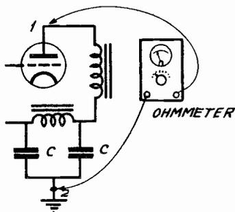
FIG. 3E. If you test continuity in this case, and *C* happens to be an electrolytic condenser, the ohmmeter needle may creep up or down scale. Electrolytic condensers have polarity. Always connect the ohmmeter so the needle creeps up scale.
