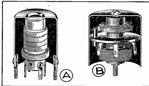
Fig. 14—Radio frequency coils in a metal shield to prevent other coils in the receiver from affecting their operation. A is a tuned secondary transformer; B is a self-tuned secondary, depending on its own capacity for tuning.
