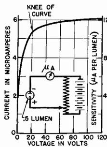
FIG. 5B. Current-Voltage Curve for Westinghouse SR-50 phototube, obtained with constant illumination of .5 lumen.
