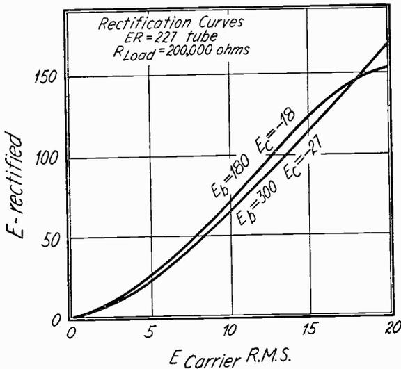
Fig. 11—Voltage measured across load resistance of detector as various carrier voltages are applied.
