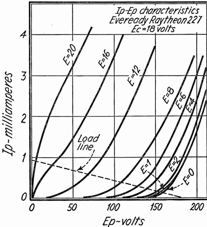
Fig. 10.—Plate current ( $I_p$ ) of detector controlled by plate voltage ( $E_p$ ) and carrier input signal voltage ( $E$ ).
