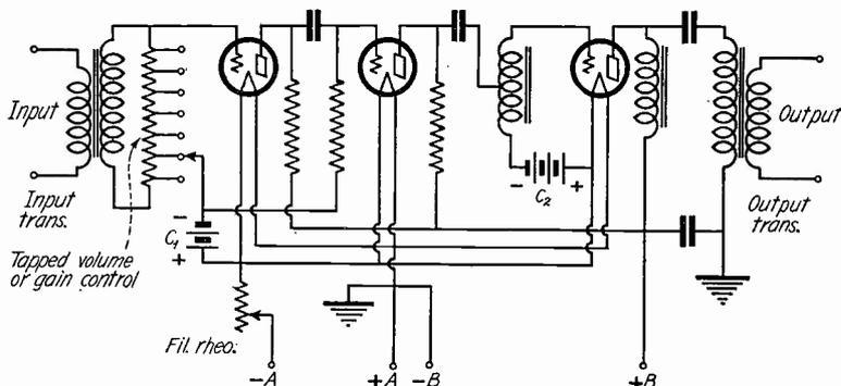
FIG. 8. Wiring Diagram of Line Amplifier.
