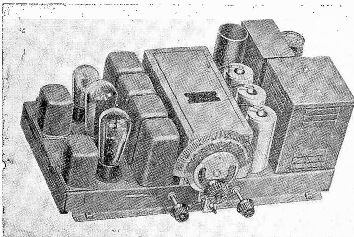
Typical chassis of a screen grid T.R.F. receiver showing shielding. This is what the radiotician or service man see when he removes the chassis from the cabinet.
