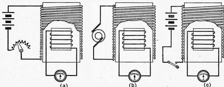
Fig. 3—Sketch showing three methods which can be used for inducing a voltage in a secondary coil when a varying D.C. current, alternating current or an interrupted current is applied to the primary coil.
