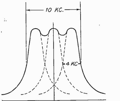
*Over-all resonance curve when one R.F. stage is adjusted slightly above, and one slightly below resonance.*
