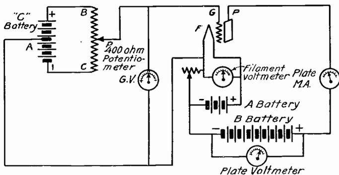
Fig. 5.—Circuit Diagram of Testing Set for Obtaining Tube Characteristics
