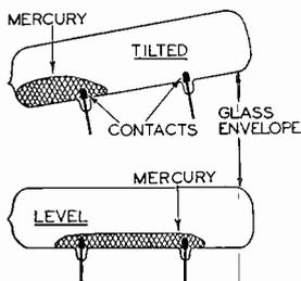
FIG. 11A (above). Tilted and level positions of a simple mercury switch, where a globule of mercury makes electrical connection between the two contacts.
