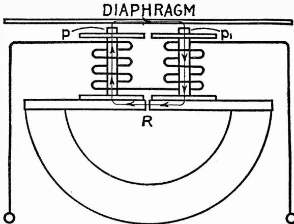
Fig. 3—Addition of Reluctance Gap to Bi-Polar Unit
