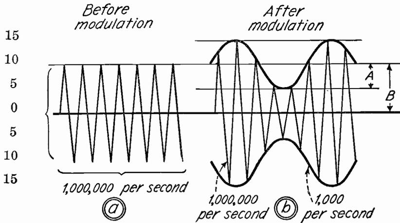
$A$  = peak value of modulating current or voltage.
