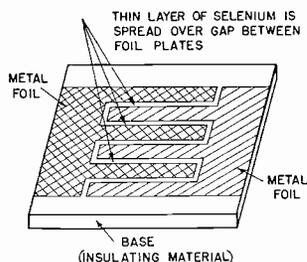
FIG. 8A. The basic construction of a simple selenium cell is illustrated in this sketch.
