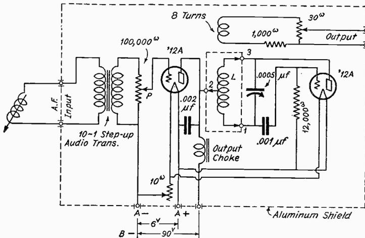
Fig. 21—Audio modulated signal oscillator (Hartly type)
