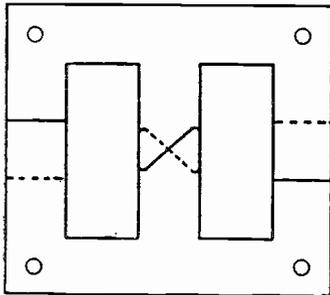
Fig. 17(a)—Laminated core, each lamination reversed and then alternately reversed.
