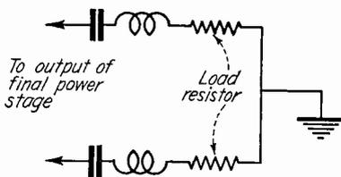
Fig. 17. Dummy Antenna Circuit.
