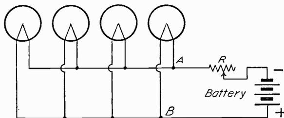
Fig. 8—Four Vacuum Tube Filament Circuits Connected In Parallel.
