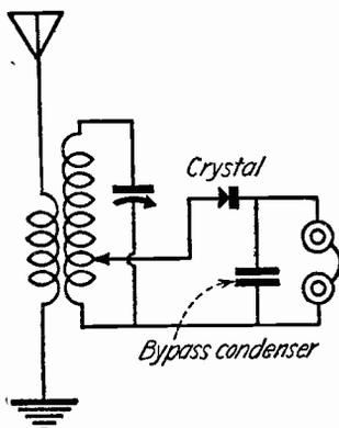
Fig. 6—Crystal detector receiving circuit.
