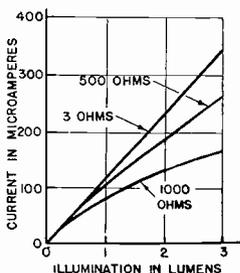
FIG. 13A. Current-Illumination Curve for Weston Photronic cell.
