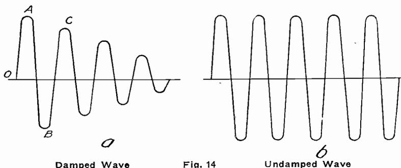
The coil and condenser act in a very similar manner, as we have seen. The energy in the spring may be likened to the charge (or voltage) of the condenser. The coil takes the part of the weight. The up and down motion of the spring and weight is like the to and fro motion of the electrons in the electric circuit.
