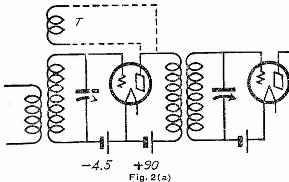
erties. The maximum amplification possible with a triode is 30—in the case of the '40 type tubes—but '40 tubes can only be used as A.F. amplifiers. They oscillate much too readily for use in R.F. stages. It was known for a long time that if this internal capacity could be eliminated, tubes could be constructed to have high amplification factors. The result of efforts to reduce
