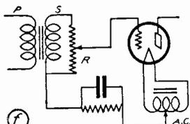
By means of a 0-500,000<sup>Ω</sup> potentiometer placed across secondary of audio transformer
