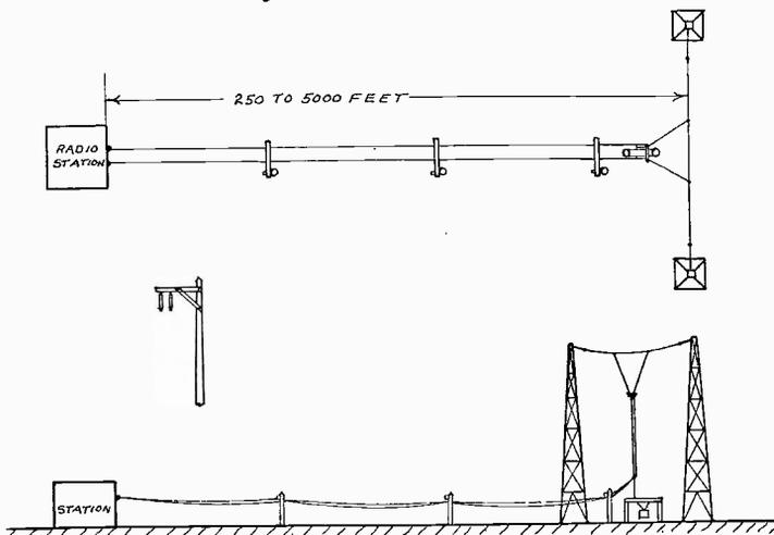
Fig. 13.—Typical Arrangement of Radio Station With Antenna Energized by a Transmission Line.
