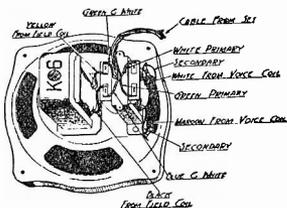
Fig. 2—Speaker Connections—121 Code
