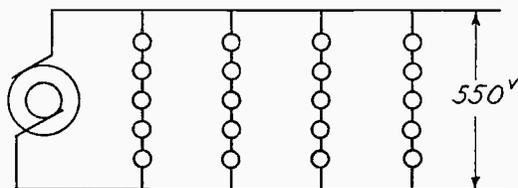
Fig. 13 (a)—Series-Parallel Circuit
