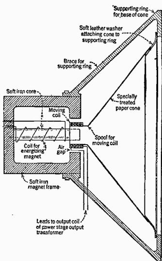
Fig. 20—Construction of the Moving Coil Type of Dynamic Speaker
