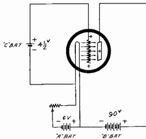
FIG. 3.—The Action of the Positive Charge on the Grid
