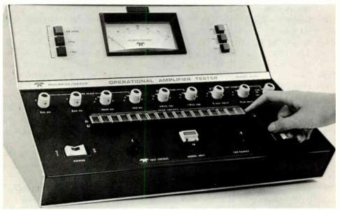
Courtesy Philbrick/Nexus-Teledyne Fig. 50. An automatic operational amplifier tester.
