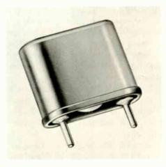
Fig. 20. A quartz crystal in its holder.
