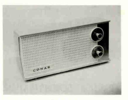
In this kit you build this complete five-transistor, line-operated AM radio receiver and conduct experiments on it.
