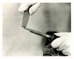
Fig. 7. File the opposite surface at the same angle as the first surface, as shown.
