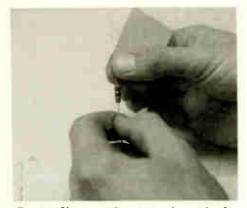
Fig. 16. Using sandpaper to clean a lead.
