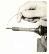
Fig. 9. How to apply solder to tin the tip of the iron.
