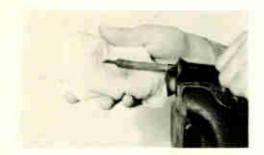
Fig. 10. Wiping excess solder from the iron with a piece of cloth.
